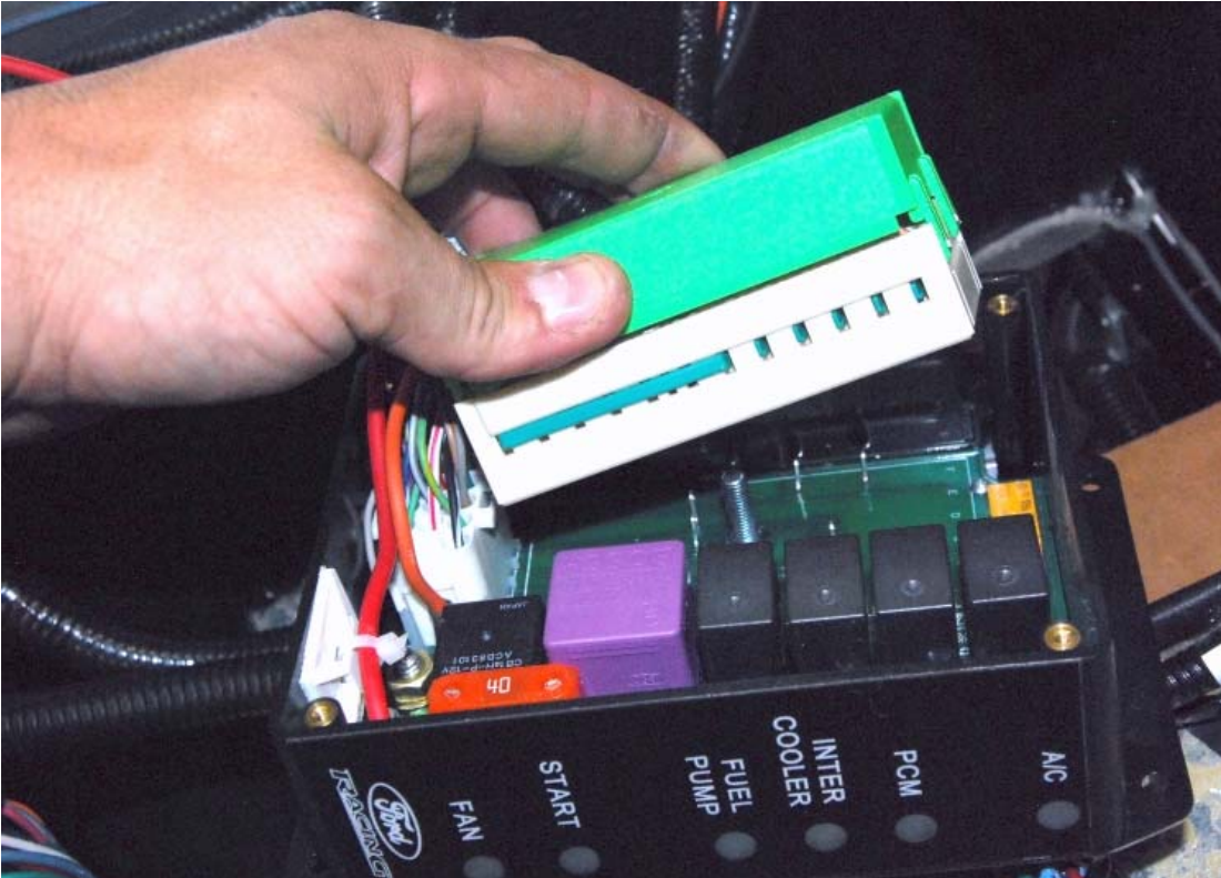
Connect the green power plug inside the box. It gets attached using a large Philips head screwdriver through the bottom of the box.
