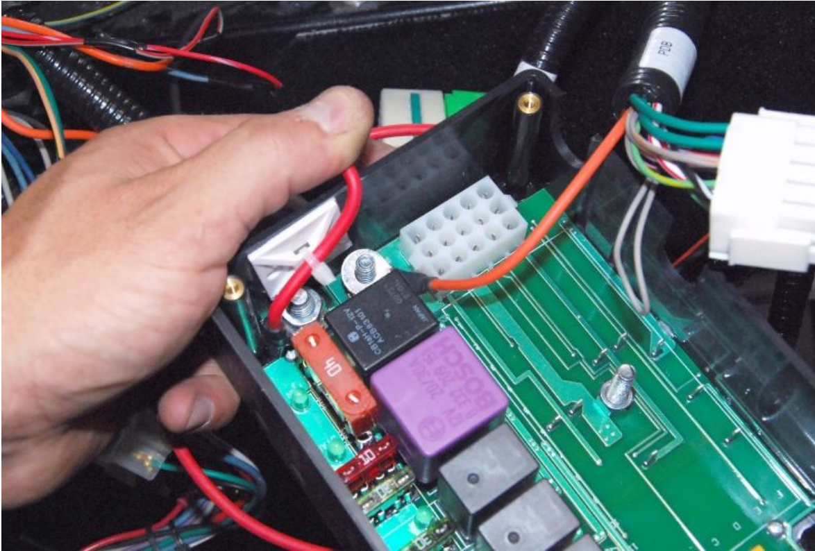
Put the orange wire ring connector onto the post.
