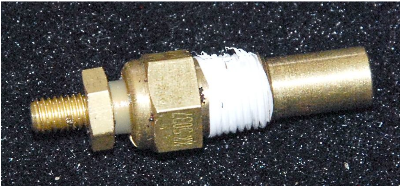
Put Teflon tape on the sending unit.
