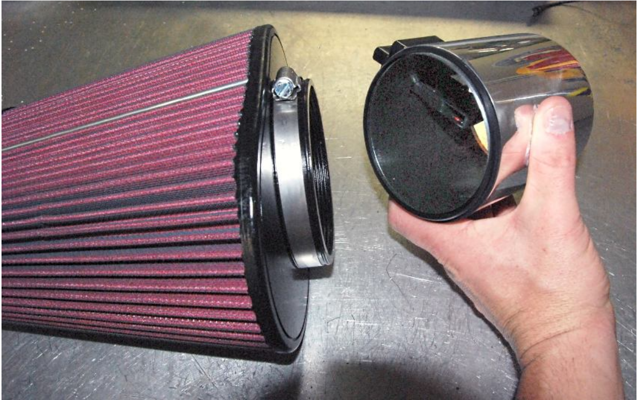
Slide the Mass Air Meter tube flat sensor side first (Spectre writing) into the air filter.
