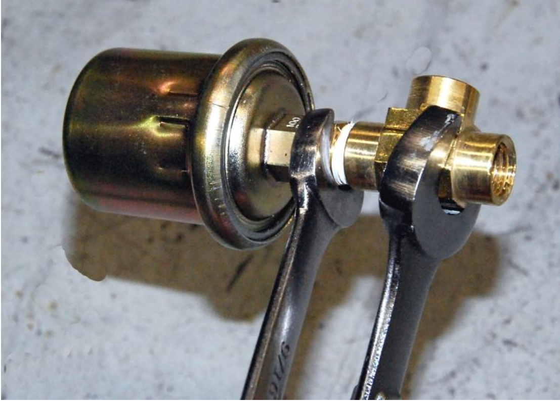
Put Teflon tape on the adapter then screw on the “T” adapter fitting.
