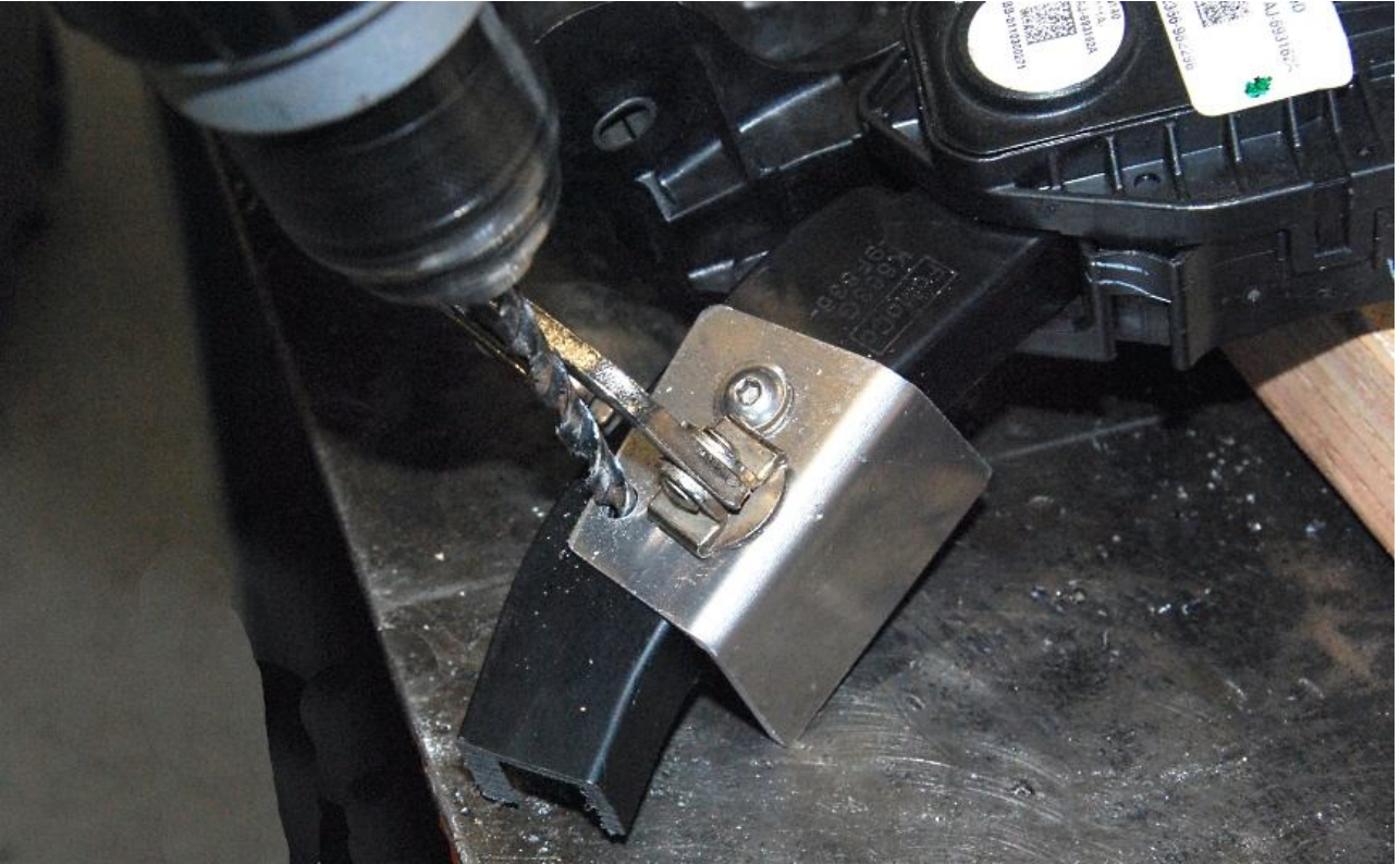
Drill the second hole out in the stalk to ¼”.
