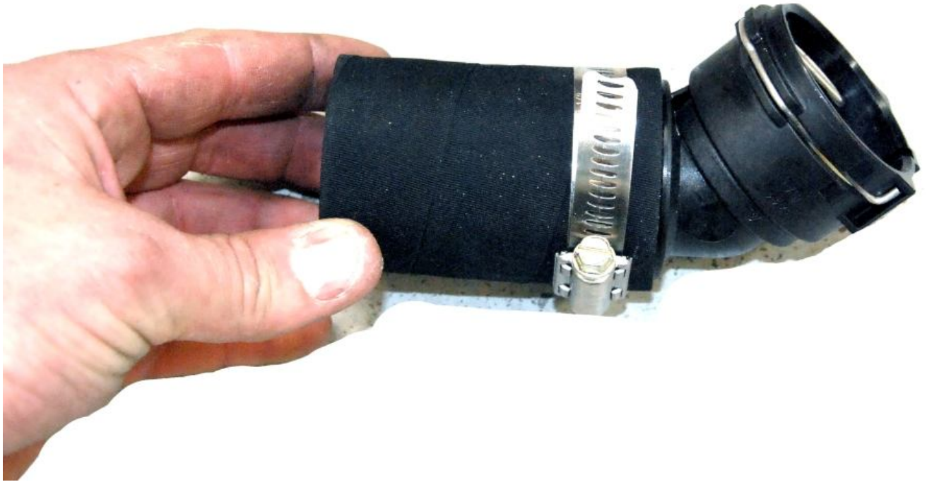
Attach one of the kit hose adapters to the plastic adapter
