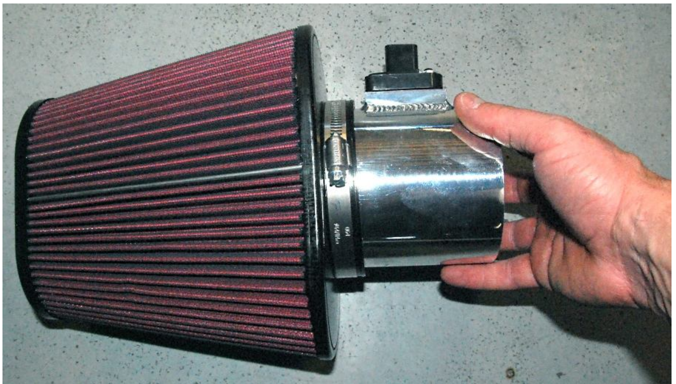
Adjust the Mass air meter so that the mass air plug is on the far side as the Ford Racing instructions recommend.
