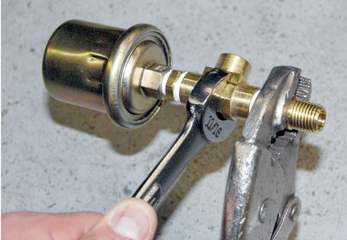
Use vise grip pliers to attach the 1.50" tube to the sender assembly.
