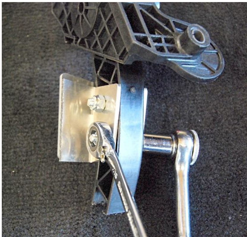
Bolt the two brackets to the stalk.
