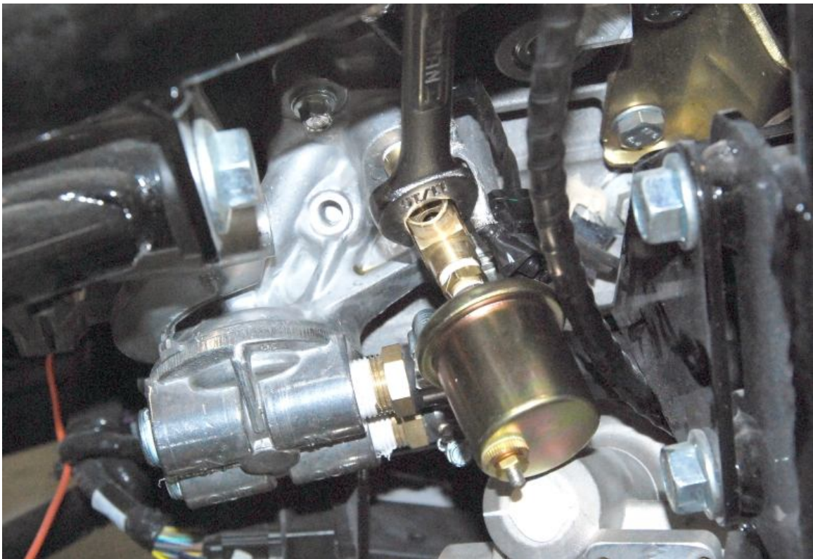
Use Teflon tape and install the pipe fitting assembly in the oil pressure location on the engine so that the side port faces up for now.
