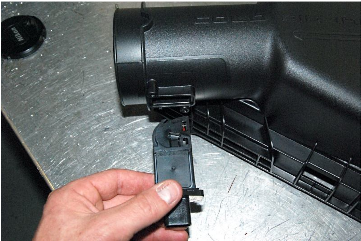
Remove the sensor and note the direction of the curved part of the sensor.
