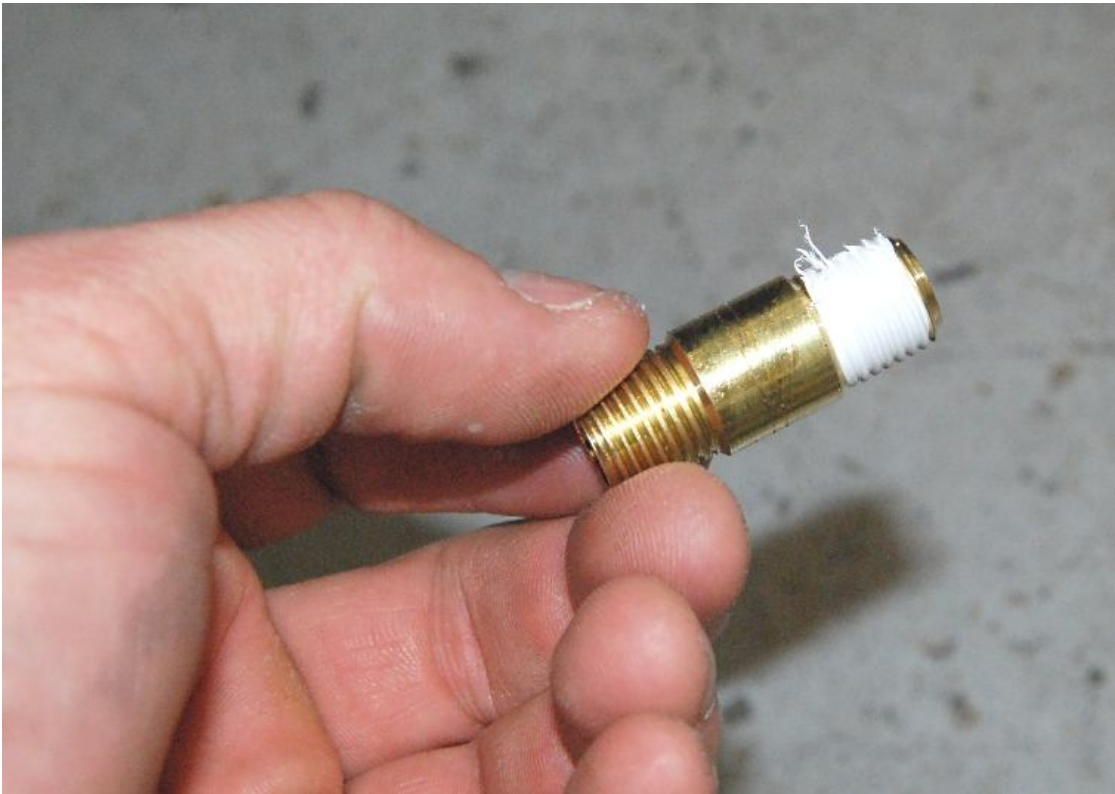
Put Teflon tape on the 1.50” NPT tube.
