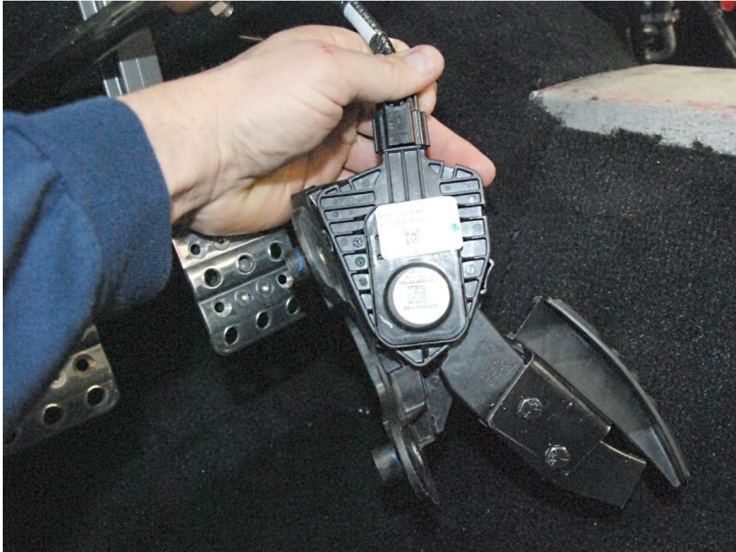
Connect the harness plug to the pedal.
