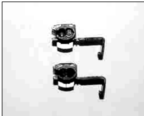
Upper connector has blockage, lower is drilled.
