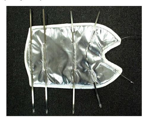
3. From the top of the car in the engine bay push the heat shield down so that the "V" area is in the bend of the pipe near the exhaust header.
