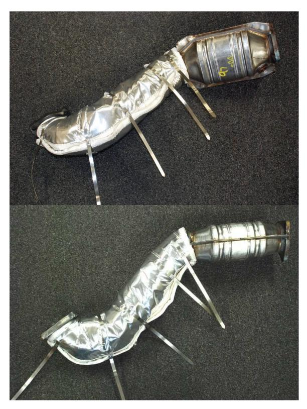
5. Starting at the header end of the pipe, pull the heat shield tight around the tube overlaping the material then while holding the material tight with one hand, pull the strap tight using a pair of pliers.
