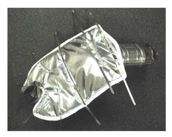
4. From under the car, pull the heat shield around the pipe and insert the straps into each other. Leave the straps a bit loose so that the heat shield can be pulled tight and adjusted. The top two straps near the catalytic convertor are easier to get to from the top in the engine bay. Note that the straps are like zip ties, once they are together they will not come apart.
