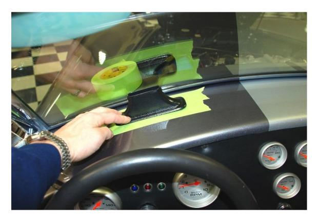
d. Use a pen to lightly draw around the outside of the duct and remove the duct.
