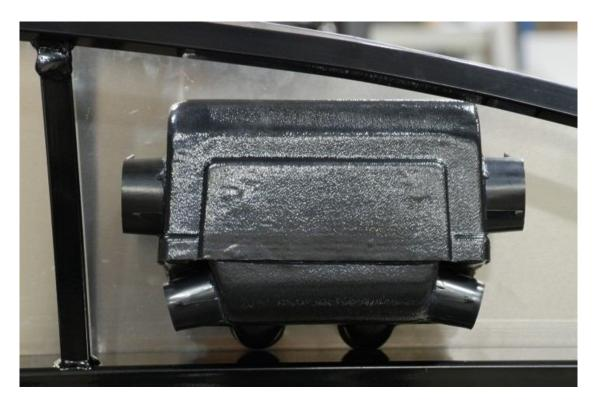
14. Insert the heater core tubes into the small holes and push the grommets into the holes.
