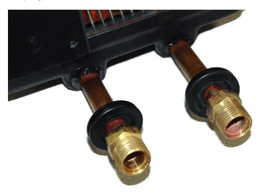
12. To prevent any air leakage between the heater box and the firewall, use some high temp RTV silicone just above the heater core tubes as shown in the picture below. Make sure you use enough so that it will seal against the firewall.
