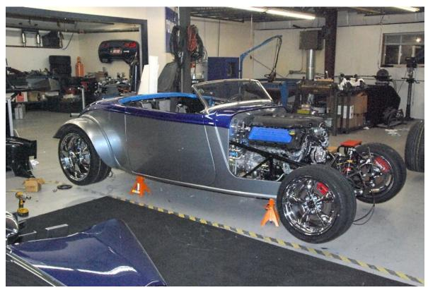
Jack the rear end up so that it is at ride height and check the fitment of the wheel in the fender. Make sure there is no interference.
