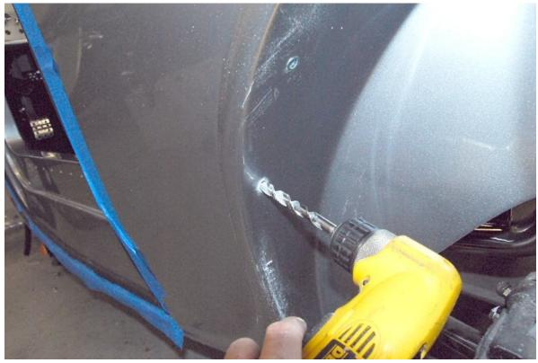
Remove the fender and enlarge the hole in the body to  $^{25}/_{64}\!\!\!^{\prime\prime}$
