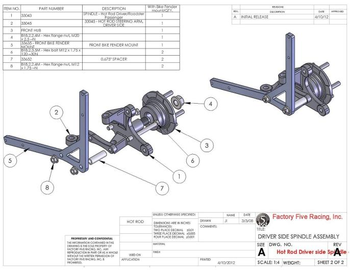
Install the long steering arm bolts, spacers and front fender mount bracket. Leave the locknuts loose for now.
