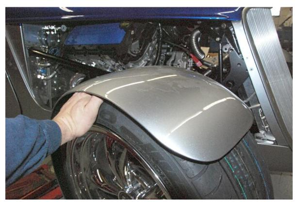
Recheck clearance between the fender and tire.
