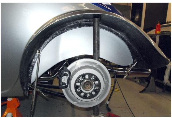
Position the rear fender on the body so it fits tight on the inside, hold it in place with a 2x4 on a jack stand or similar.
