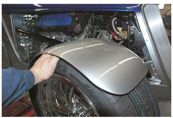
Make sure that ther is at least a hand clearance between the fender and tire at all positions under the fender.
