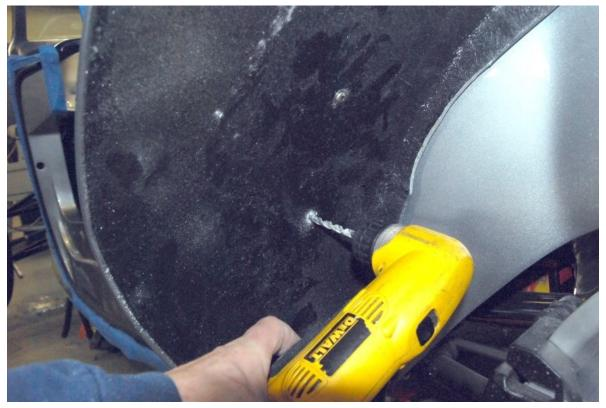
Drill a  $^{3}/_{16}$ " hole straight up making sure it goes through the fender and the body.
