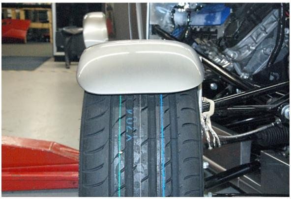
Clamp the fender to the mount so that the fender is between the tire and mount and is positioned around the tire as desired.
