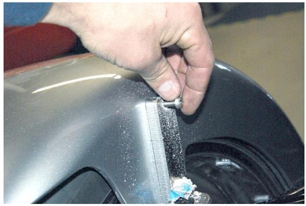
Reclamp the fender in place using the 1/4" mounting screws to locate the fender.
