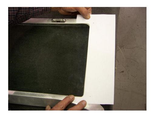
• One more snap is required on the outboard portion of the dash, install using the supplied template. This is a directional snap, it can only be taken of in one direction. Pick up in front and pull backwards.
