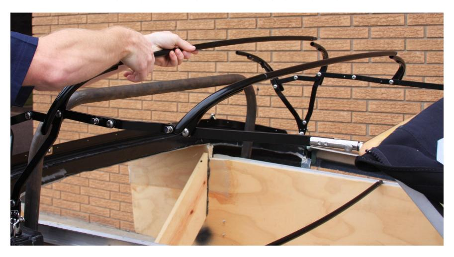
Now install the adjustable links into the pocket on the back side of the 4 bows and lightly tighten.
