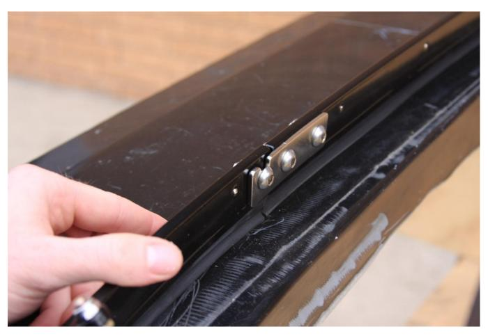
☐ Install the rear adjustable links to the ball sockets on the belt bow and lay on the body.
