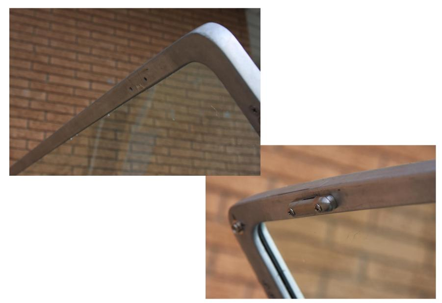
☐ Place the wooden header on the windshield and <u>adjust latches to</u> <u>crush seal about 1/4"</u>.
