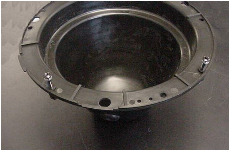
Adjustment screws installed.
