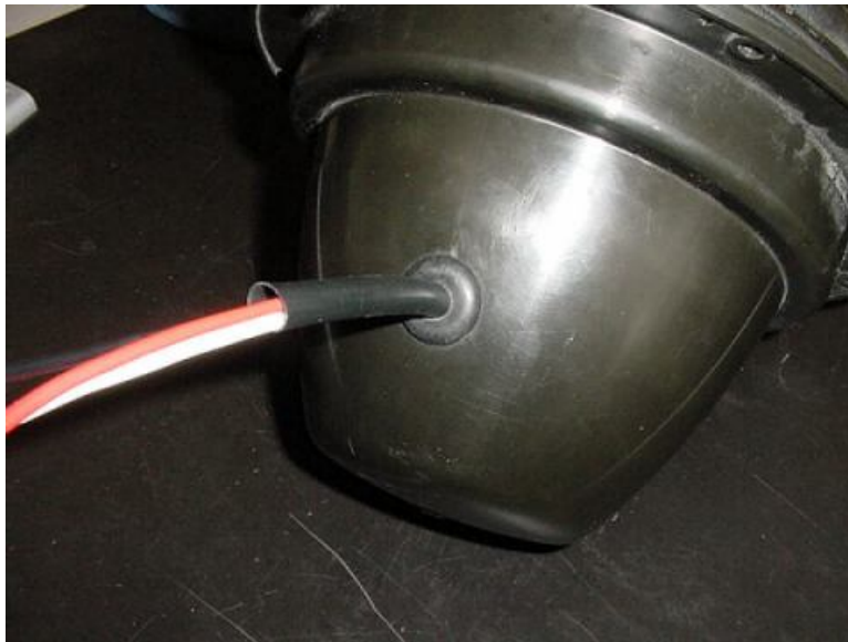
Pigtail wires and covering pulled through grommet.
