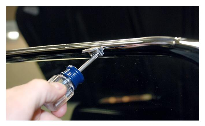
Slide the sun visors onto the brackets and tighten the pedestals with the  $\frac{3}{32}$ " hex key.
