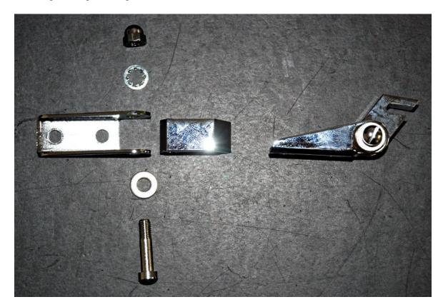
Attach the hinges to the sun visor using the shorter screws along with the flat washers, lock washers and acorn nuts. Use a small amount of Loctite<sup>™</sup> on these screws because they can work loose over time from positioning of the visors.
