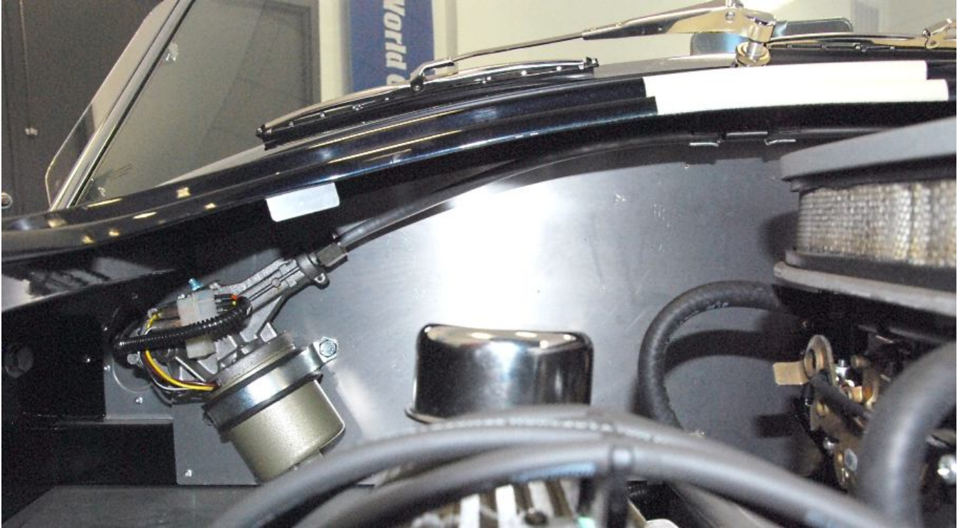
Wiper motor installed on firewall.
