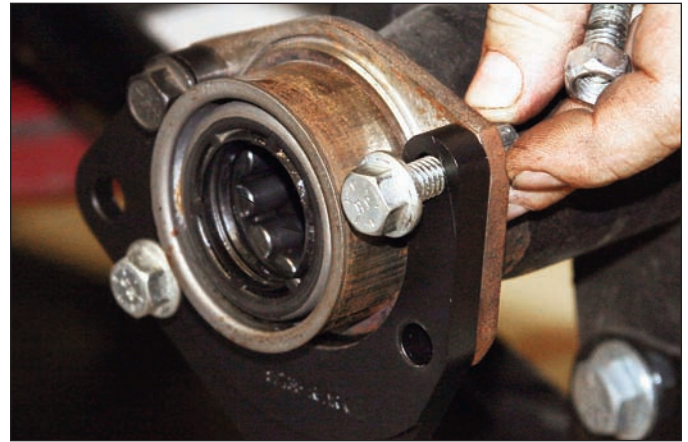
Sequence 11: Install the flat housing mount caliper bracket onto the axle hub using bolts, washers, and nuts with the "U" opening in the up position and the mounting ears facing toward the front of the vehicle. NOTE: The bracket must fit squarely against the housing flange. Inspect for interference from casting irregularities, burrs, etc. Grind as necessary.
