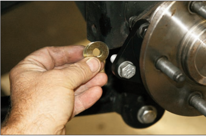
Sequence 13: Slide the caliper bracket mounting bolts thru the ears of the flat bracket from the outboard side. Initially place two shim washers between flat bracket and the caliper mounting bracket.
