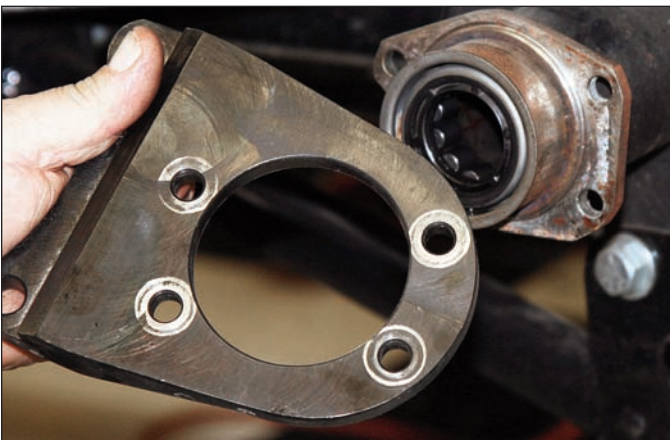
Sequence 9: Remove the OEM caliper mounting bracket from the axle hub.
