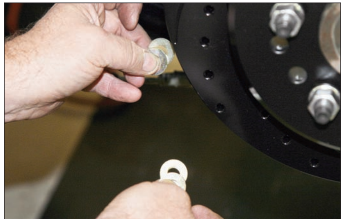
Sequence 18: Lubricate the caliper mounting studs with lightweight oil. Initially place two shim washers on each stud between the caliper mounting bracket and caliper.
