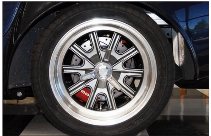
Sequence 23: Install the wheel and torque the lug nuts to manufacturer's specification. Rotate the wheel and check for any interference. Reinstall the replica knock-off's. Bed in the brake pads and rotor in a safe location before general use driving.
