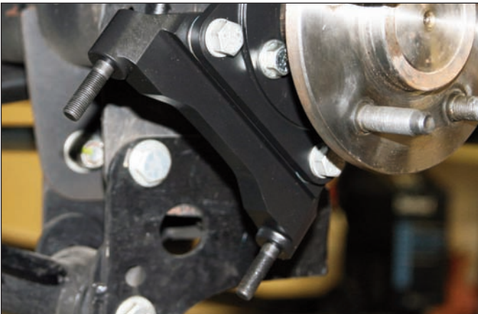
Sequence 14: Attach the caliper mounting bracket to the backside of the flat bracket. Temporarily tighten the mounting bolts. Do not Loctite at this time.
