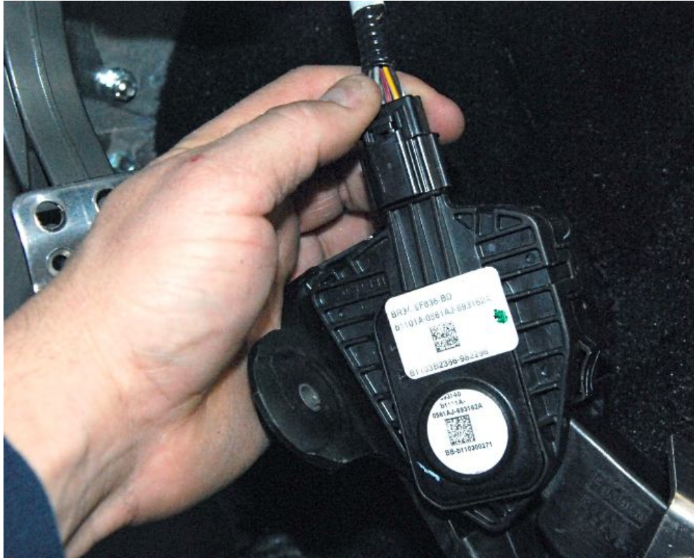
In the footbox, attach the plug to the pedal.
