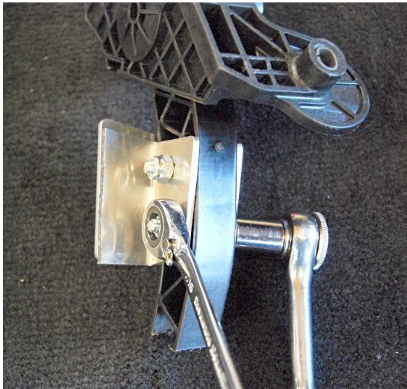
Bolt the two brackets to the stalk.
