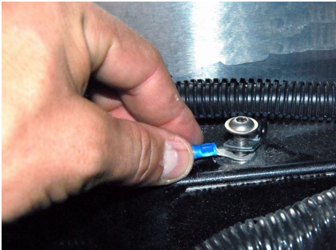
Attach the ring connector to ground.
