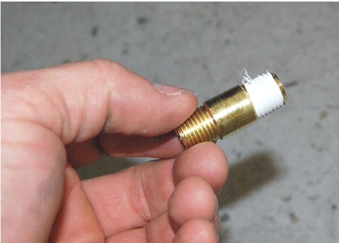
Put Teflon tape on the 1.50” NPT tube.
