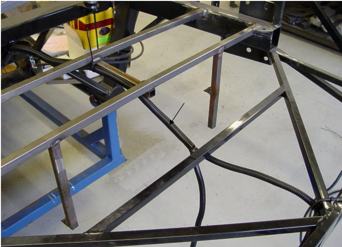
Rear harness going to back of frame.
