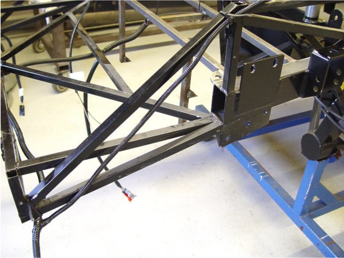
Rear harness running up to the top of the trunk.
