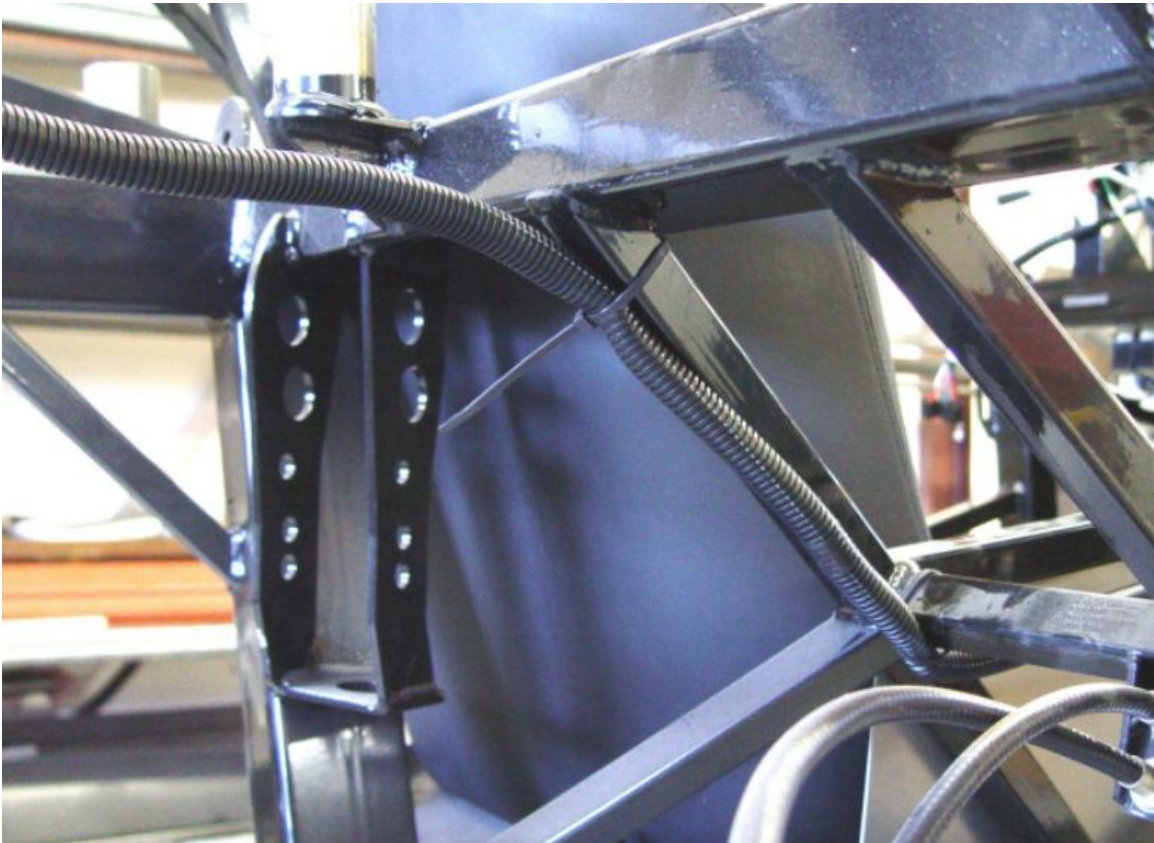
Rear harness going up to 2"x 3" tube.
