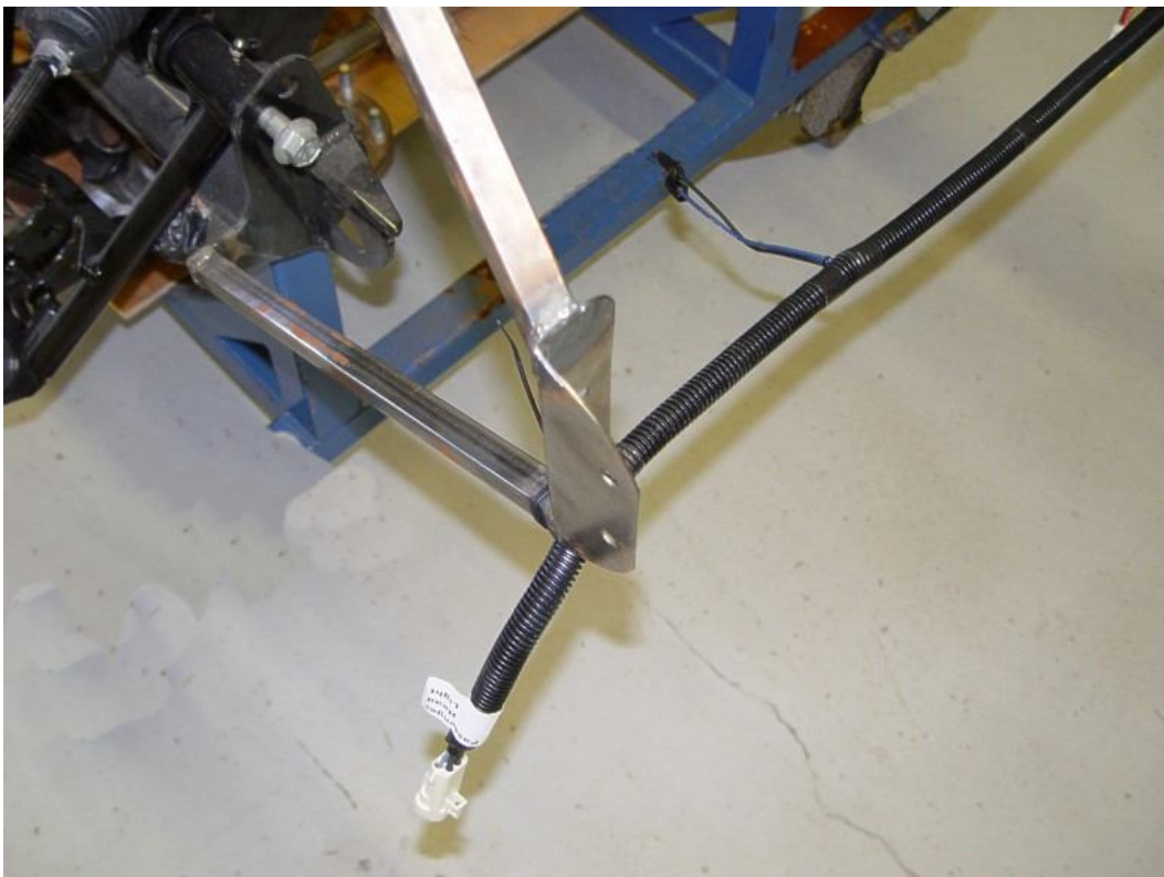
Front harness passenger side. Note fan wires also shown.
