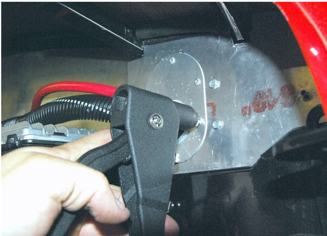
Silicone and rivet the block-off cover to the firewall extension.
