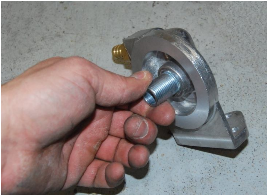
Screw the threaded nipple into the relocater.
