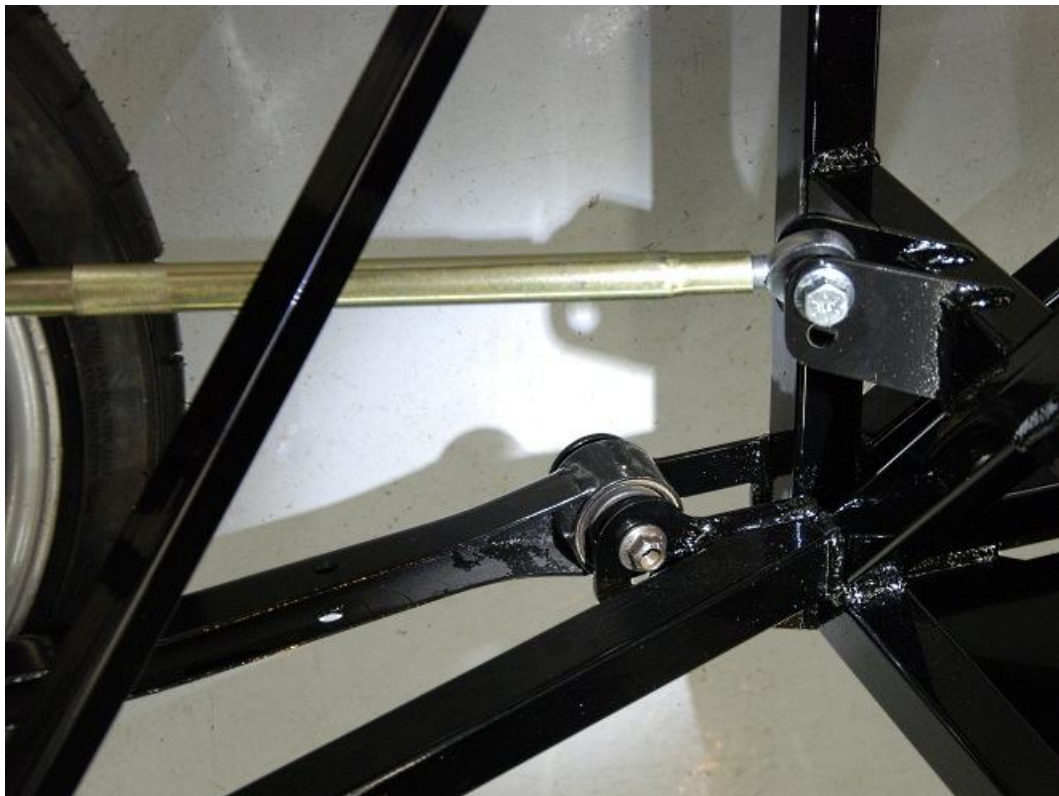
Upper and lower trailing arms mount in the upper mounting holes.
