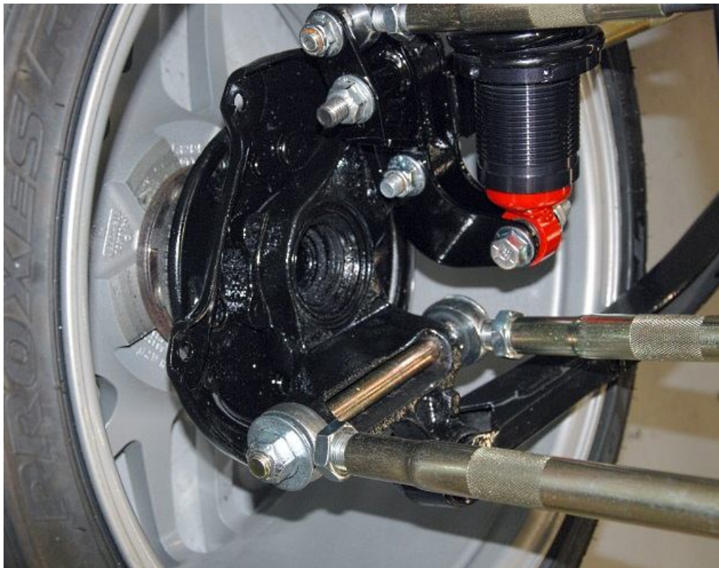
Bolt the outer end of the lower links to the spindle using the long \frac{5}{8} inch bolt. Because these rod ends are mounted on the outside of the spindle use washers that are bigger than the inside roller on the rod end for safety. (In the event of a rod end separating, the arm is still captured)
