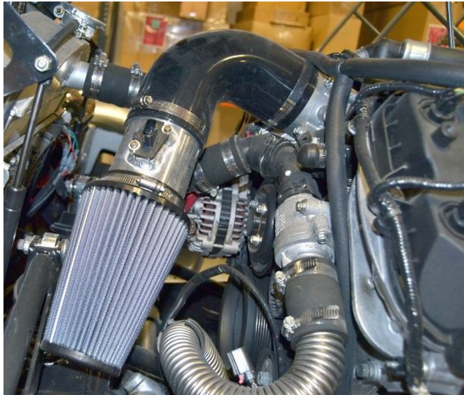
Push the mass air plug onto the mass air meter.
