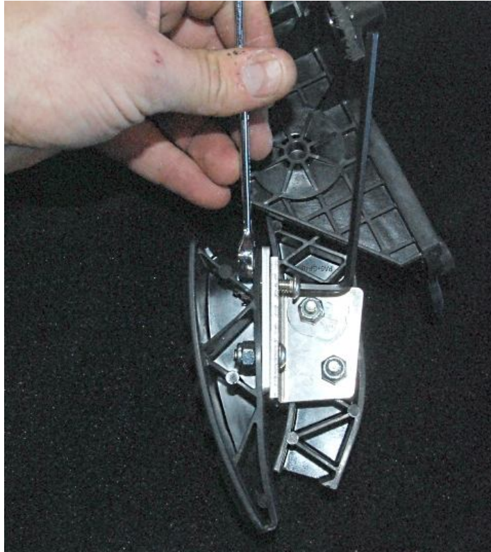
Attach the pedal pad to the mount brackets
