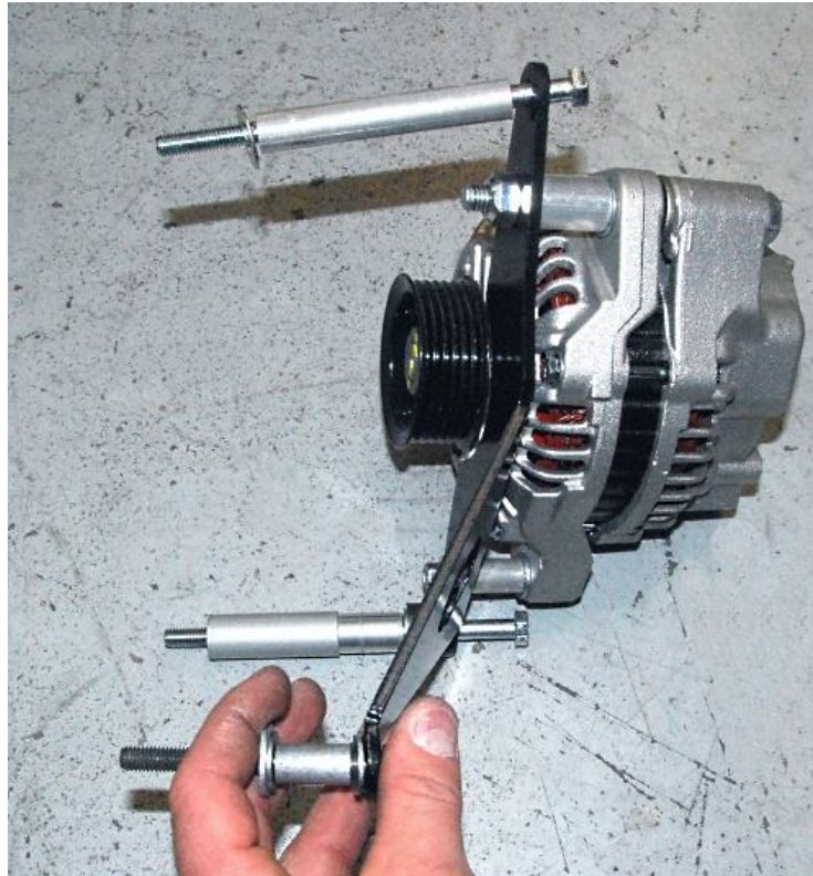
Run the bracket mounting bolts through the bracket and put the spacers on the bolts.
