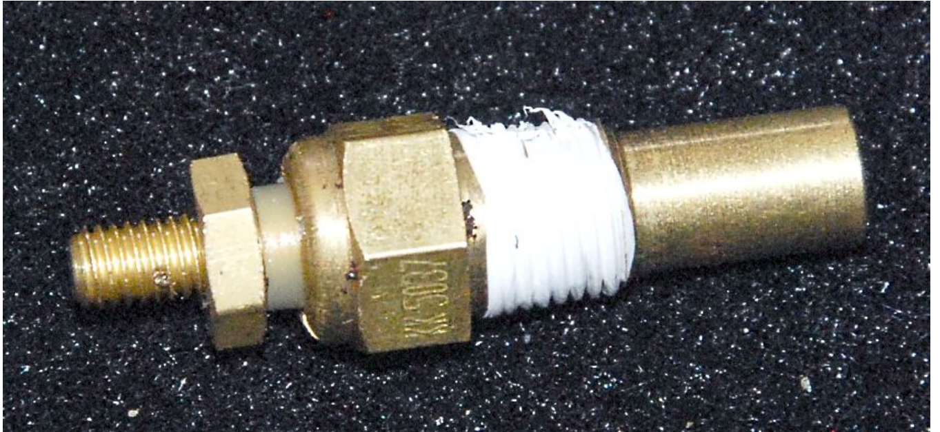
Put Teflon tape on the sending unit.
