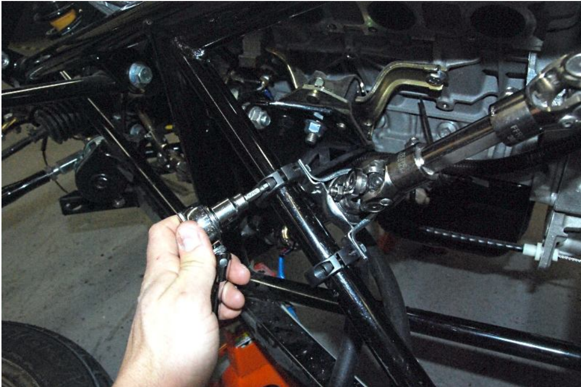
Locate the tube clamps on the tube so that the shaft is as straight as possible and then tighten the clamps.
