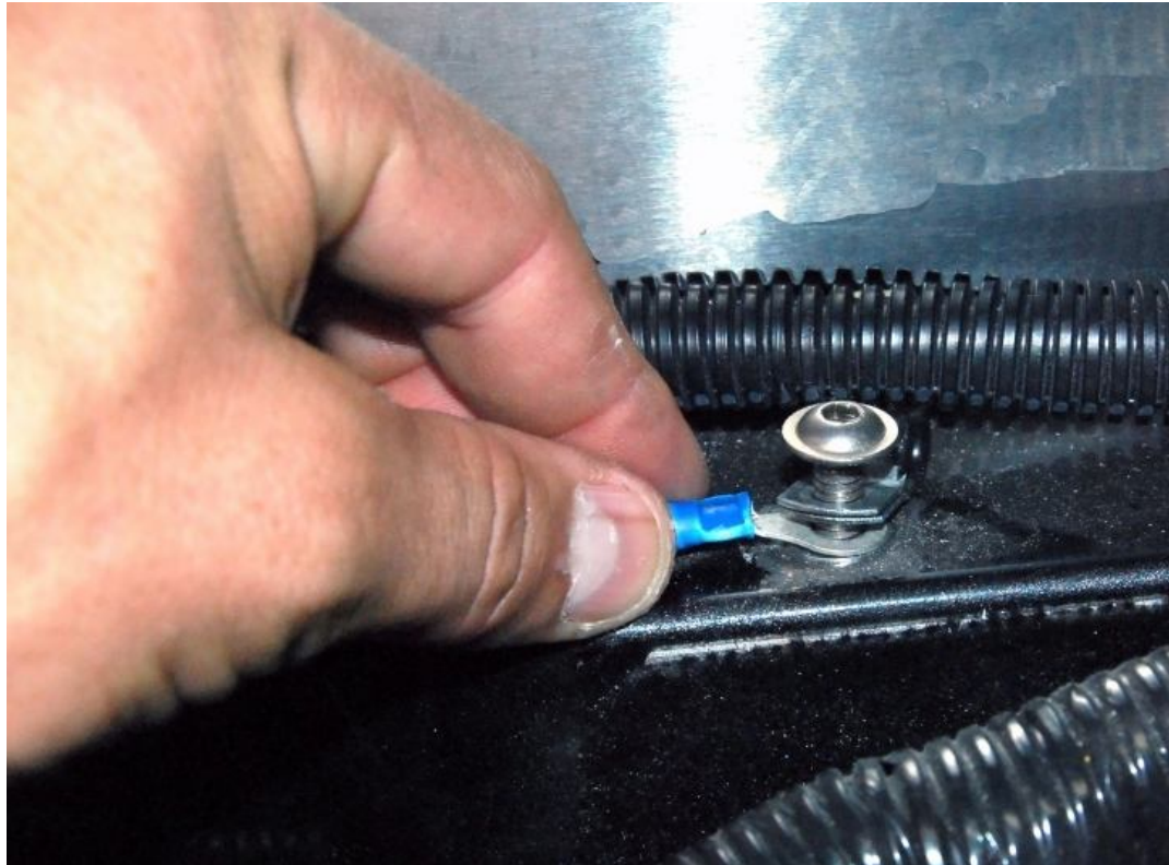
Attach the ring connector to ground.
