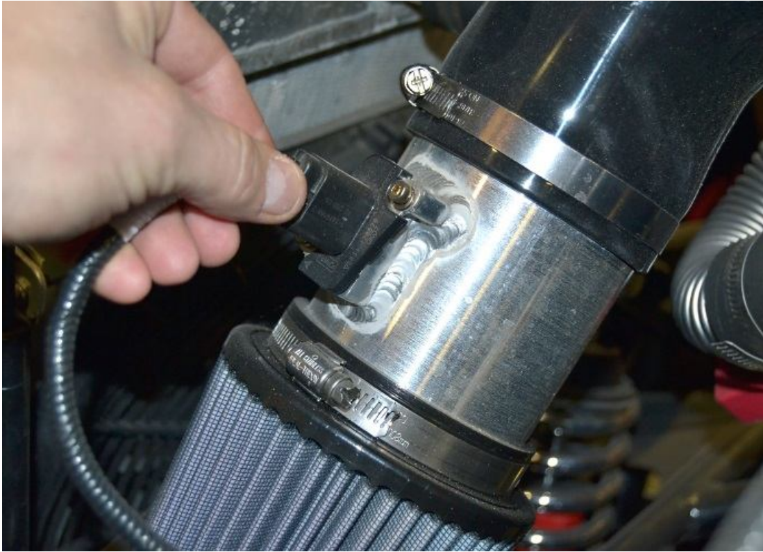
Push the mass air plug onto the mass air meter.
