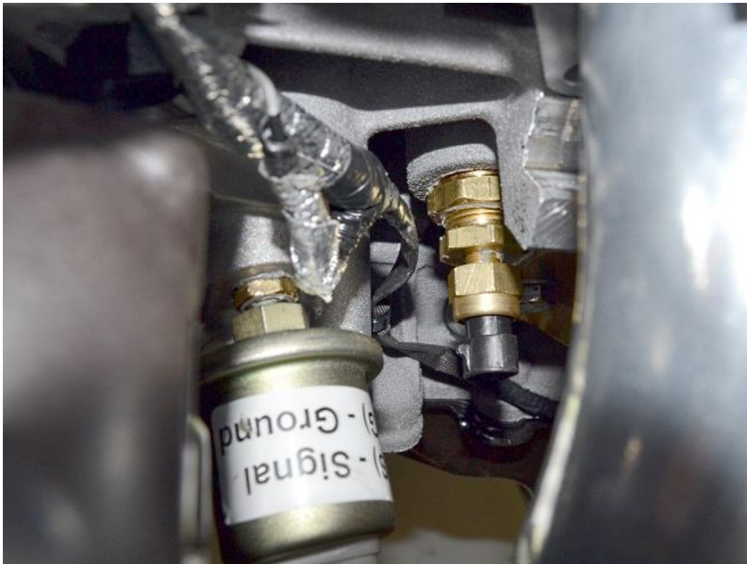
Use a 12mm deep socket to screw the sender into the adapters.
