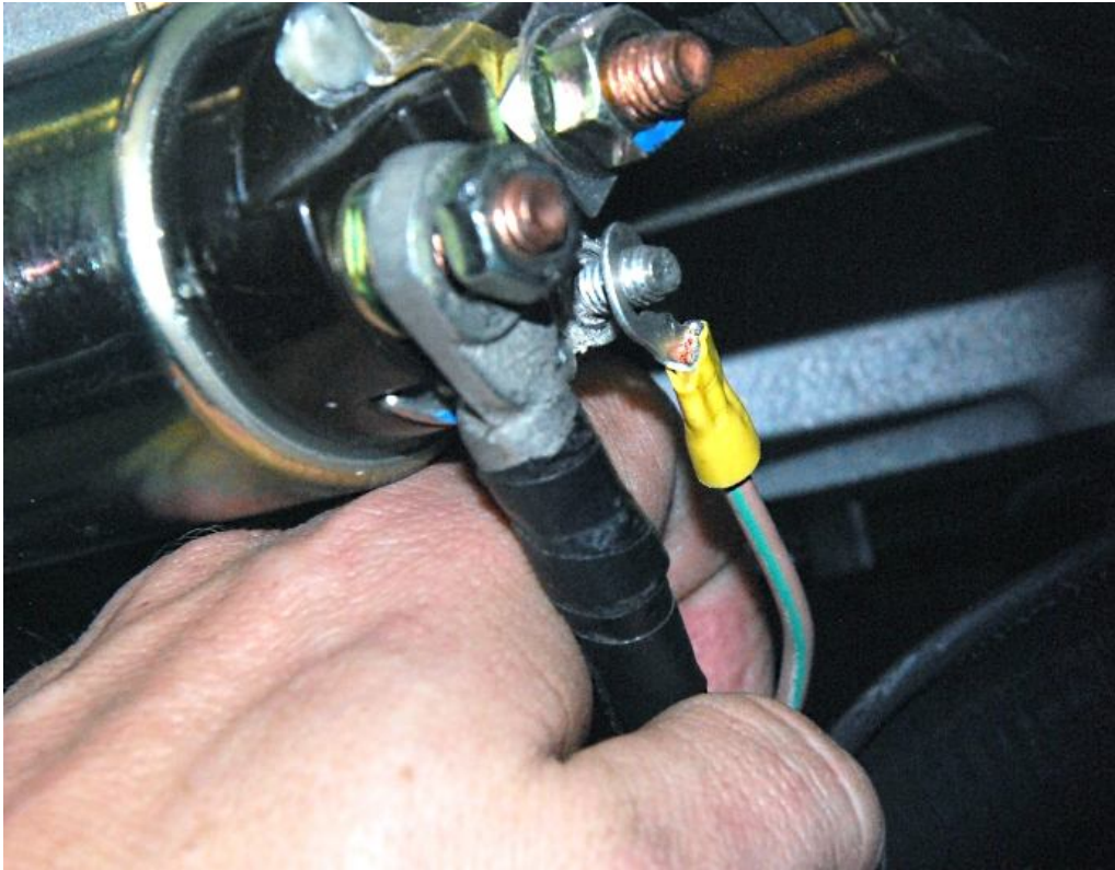
Attach the tan/green wire to the starting post on the solenoid.
