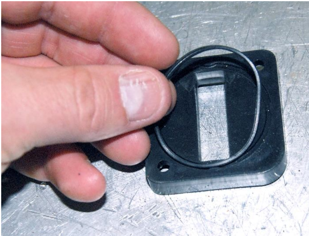
Install the rubber ring into the intake mount.
