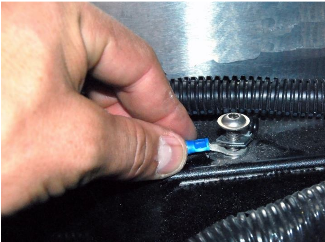
Attach the ring connector to ground.
