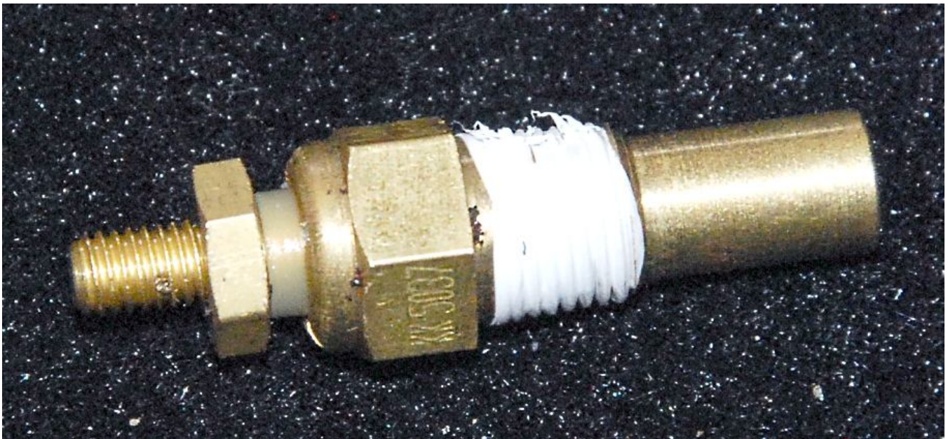
Put Teflon tape on the sending unit.
