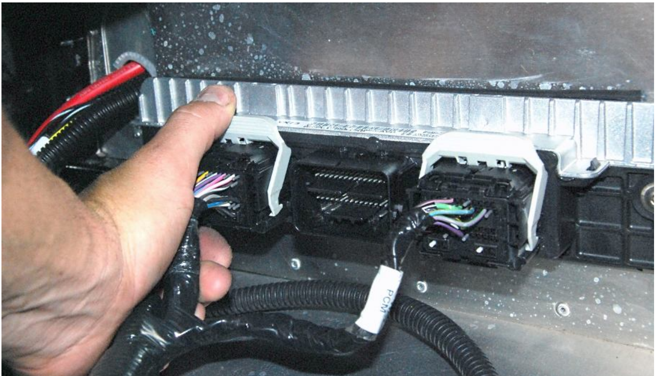
Plug the two engine harness plugs into the computer.
