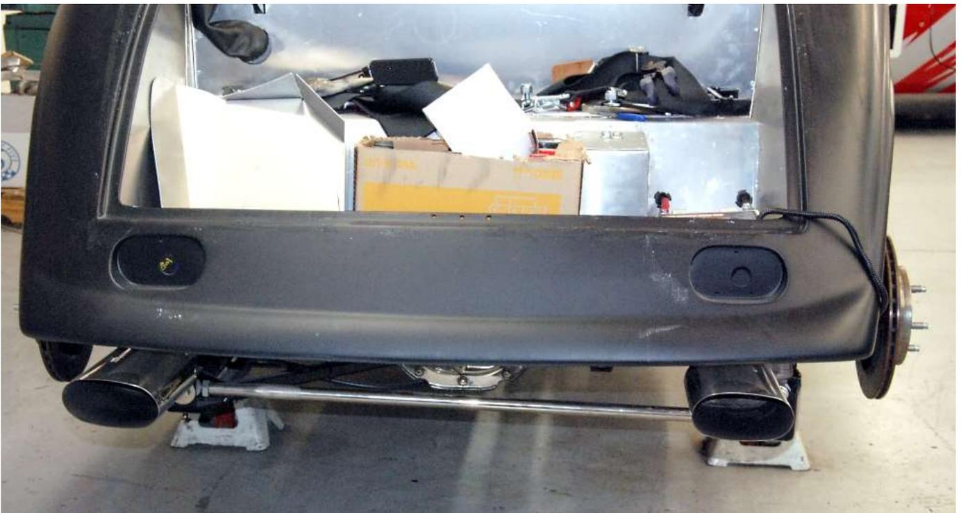
Attach the exhaust tips and locate them so that they are below the tail lights. Move the rubber hanger if necessary.
