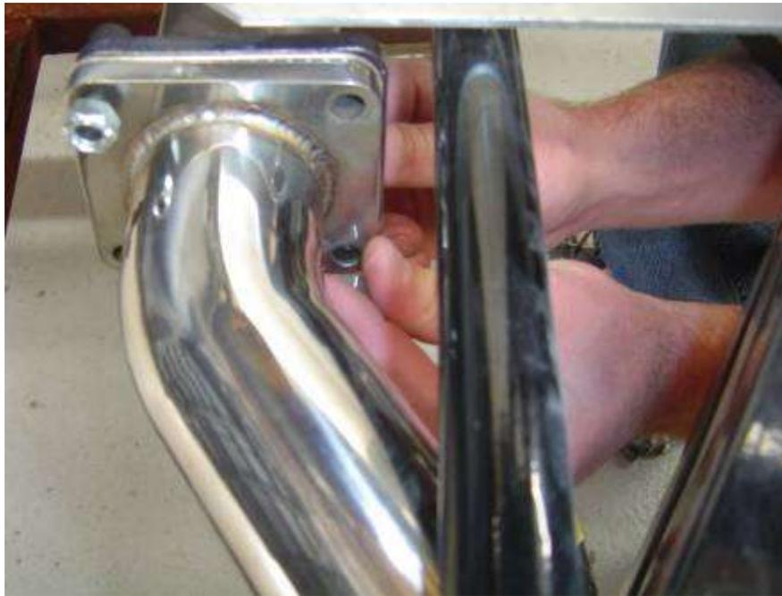
Attach the front exhaust pipe assembly to the shorty pipe with the supplied  $\frac{3}{8}$ " hardware. Make sure to install the supplied gasket (FFR# 33369) between the two square flanges.
