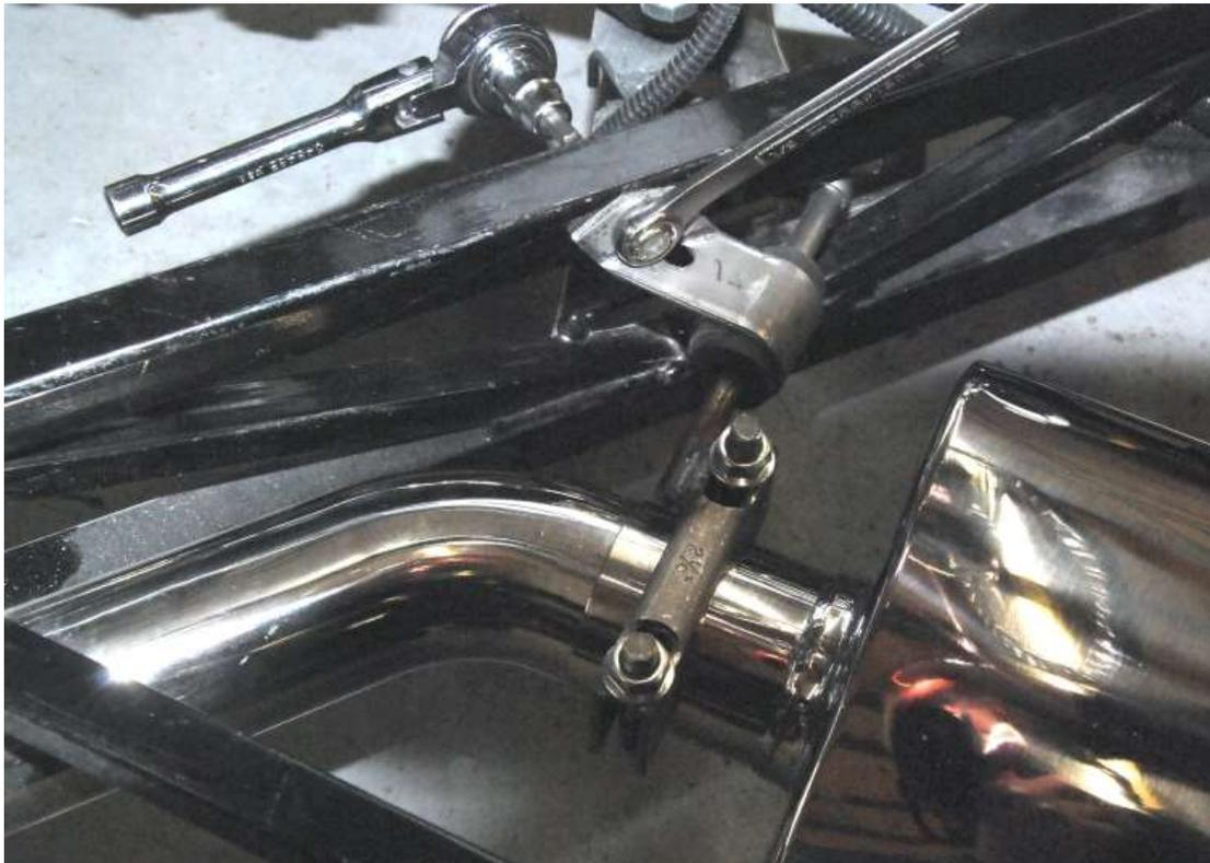
Re-install the brackets and attach them to the frame with the  $\frac{3}{8}$ " hardware provided.
