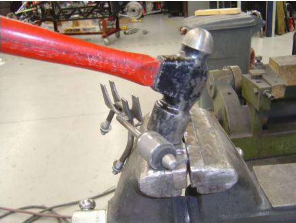
Remove the exhaust mounts and clamp them into a vise. Using a hammer, bend the tab over to a 90° angle.
