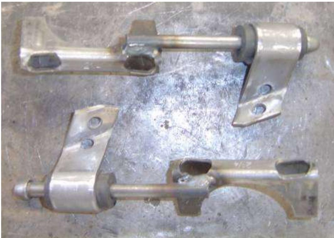
Grind the corners of the brackets which protrude past the surface of the floor.
