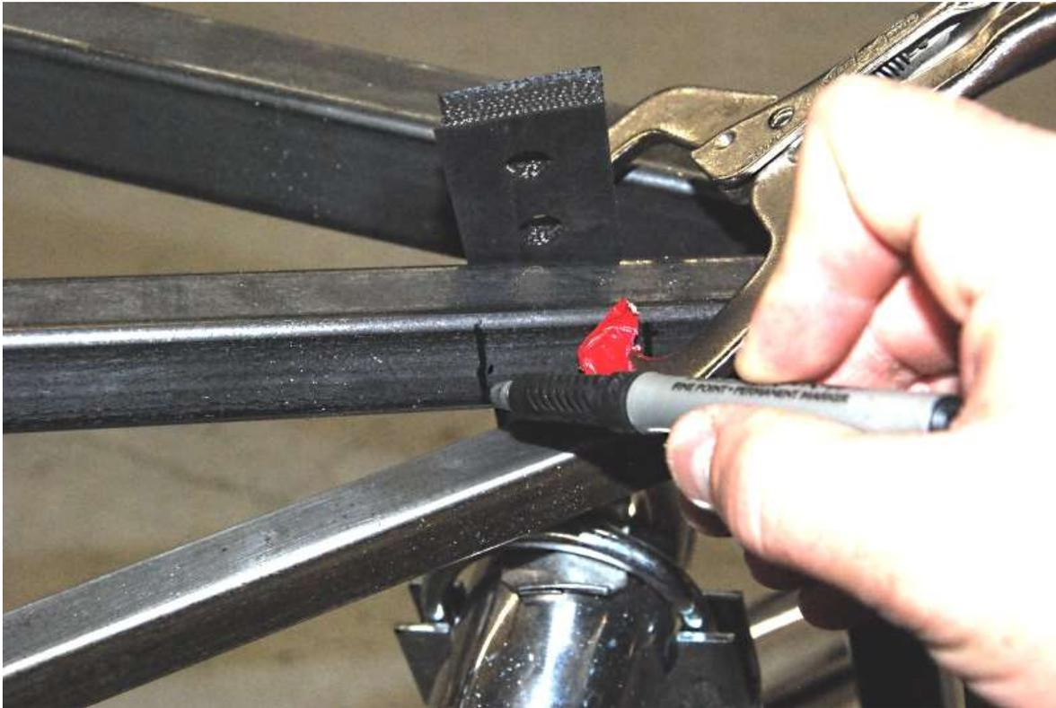
On the front side of the tube, mark the side locations of the rubber.
