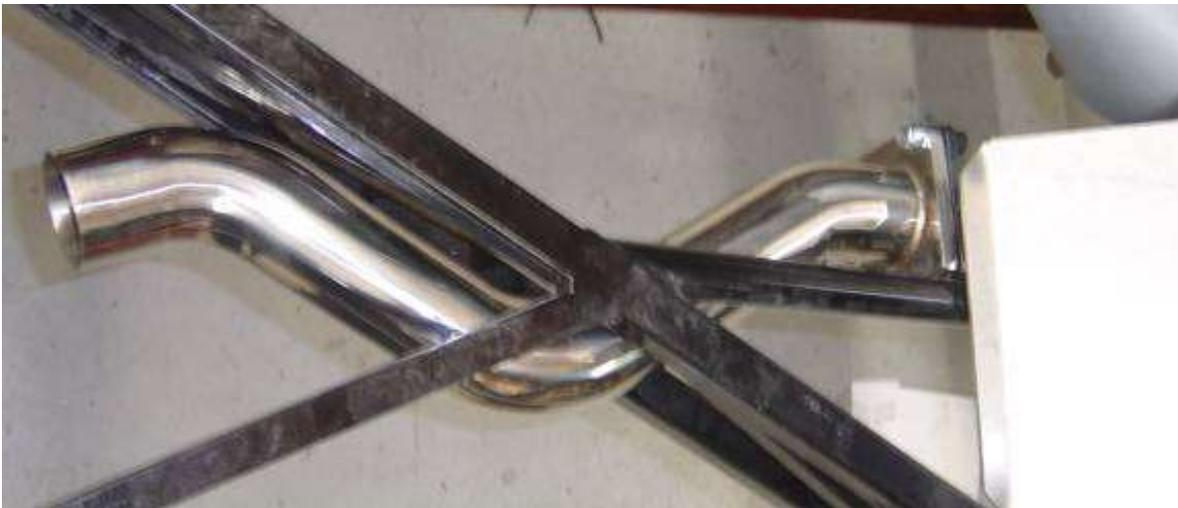
Pass the front exhaust assembly through the frame from the front so that the flange is at the front and will match up with the shorty pipe
