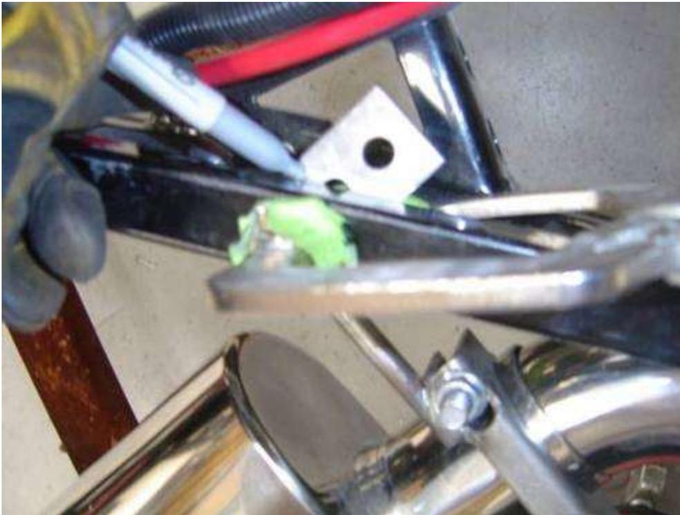
The mount tabs for the exhaust mounts have the ability to slide on the rubber bushing. Position the mount tabs so that they overhang the frame rails. Mark the location of the frame on the mount tab so that you can bend it up at a 90° angle to mount to the frame so that the bolt holding it to the frame is in shear if possible.
