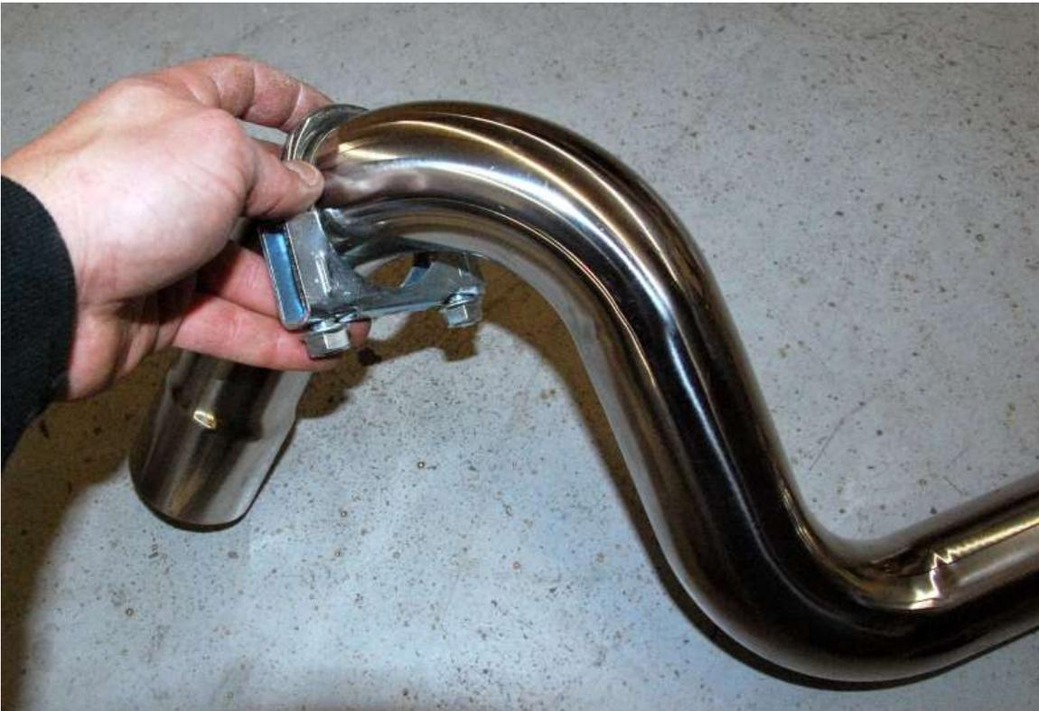
Slide one of the clamps onto the rear tube up near the top of the bend.
