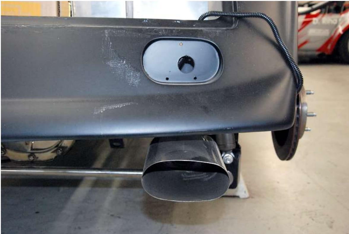
👉 The optional rear exit exhaust runs the exhaust back under the tail lights.
