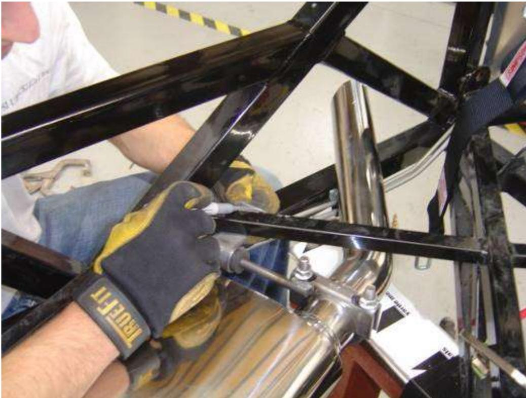
Also mark the location of the brackets that protrude past the surface of the frame where the aluminum floor sits.
