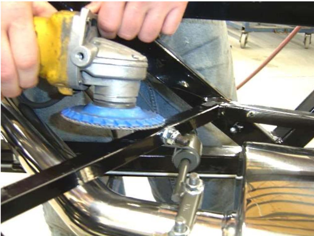
Check to make sure none of the bracket or hardware is above the top surface of the frame rails. If need be, grind anything that is sticking past this leading edge where the aluminum floor must sit.
