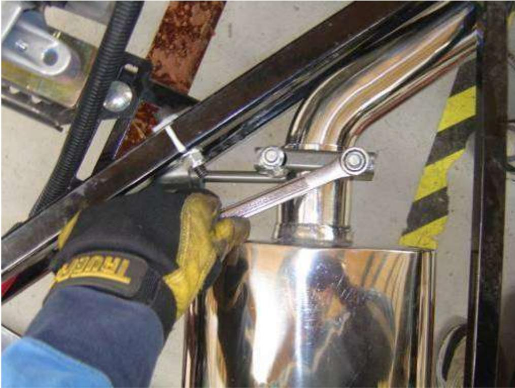
Once you are happy with the placement of all the exhaust components, tighten all of the fasteners holding the exhaust in place.
