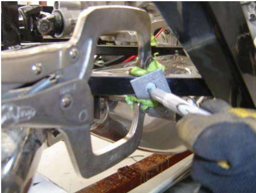
Re-install the exhaust brackets on the frame and mark the locations for the mount holes on the frame.
