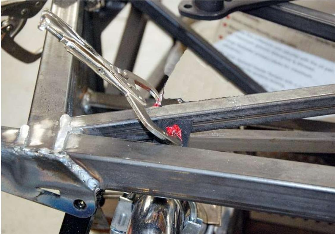
Clamp the hangers so that the lowest hole is on the back side of the tube shown in the pictures above.
