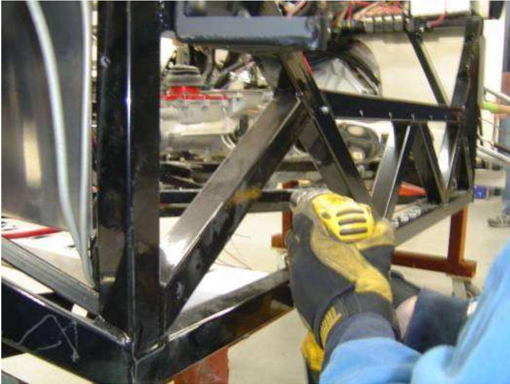
Remove the exhaust mounts and drill the frame where you just marked with a  $\frac{3}{8}$ " drill bit.
