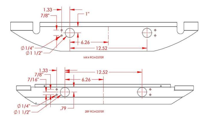
Drill the large holes with a 1.5" hole saw and the center of the small holes with a 0.25" drill bit. Install the oil cooler assembly from the underside of the car into the holes made. MK4 Roadster - Attach the oil cooler to the aluminum floor using the (4)  $\frac{1}{4}$ " button head screws, nylon spacers, washers and lock nuts in the order shown below.
