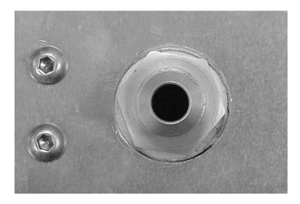
Attach the O-ring AN fittings to the Oil Cooler.
