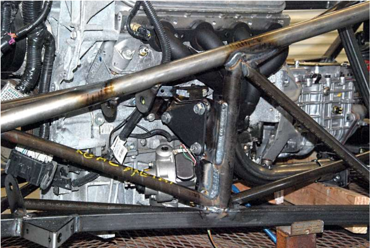
Attach the connector pipes to the kit exhaust system.
