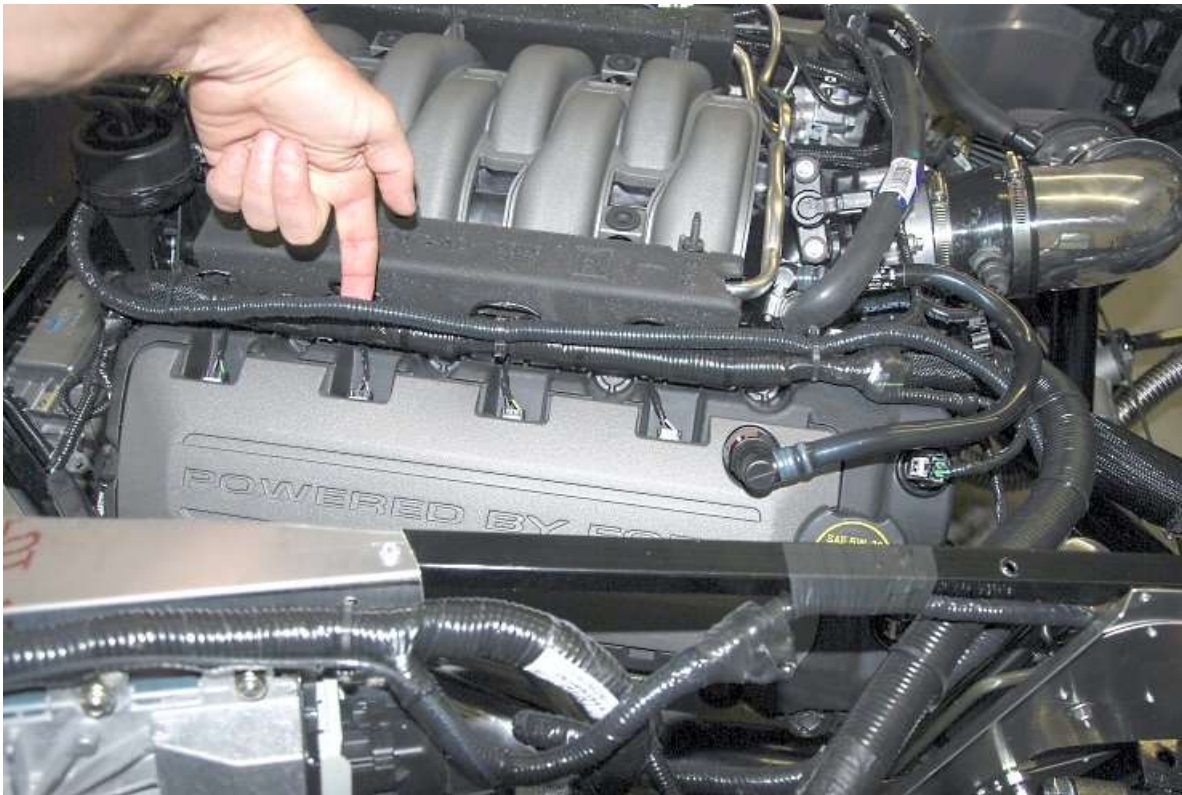
Run the BB harness leg to the back of the engine and across the back.
