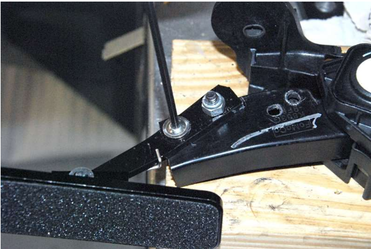
Use one of the flanged \frac{1}{4} "-20 x \frac{3}{4} " screws in the lower hole.
