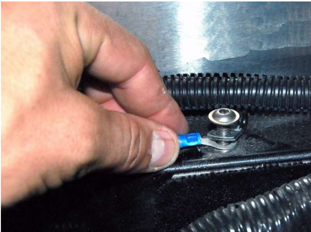
Attach the ring connector to ground.
