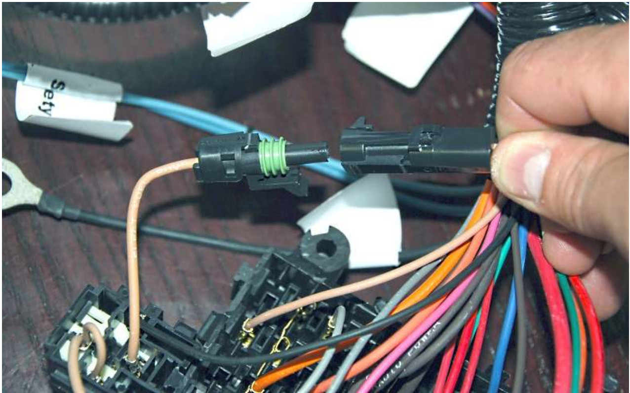
Disconnect the fuel pump wire at the relay.
