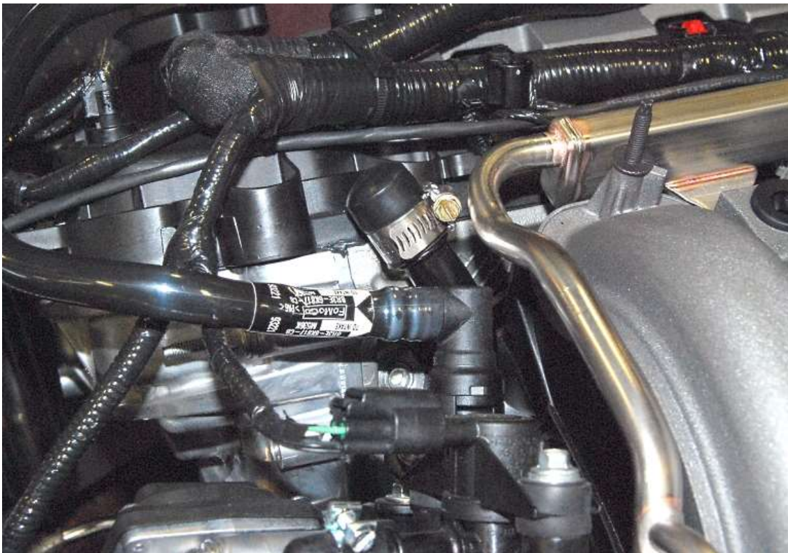
Cap and hose clamp the 3/4" coolant.
