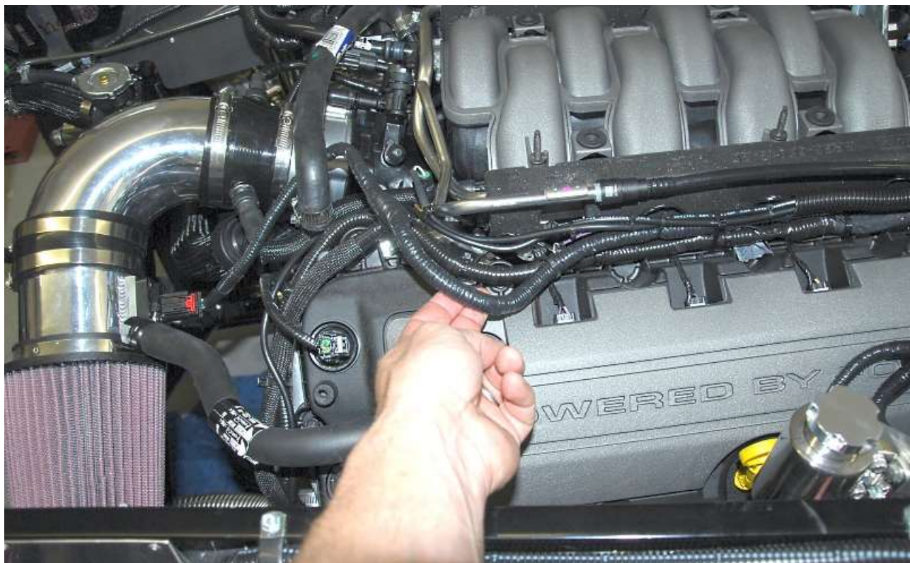
Run the BB harness leg back to the front of the engine on the left side.
