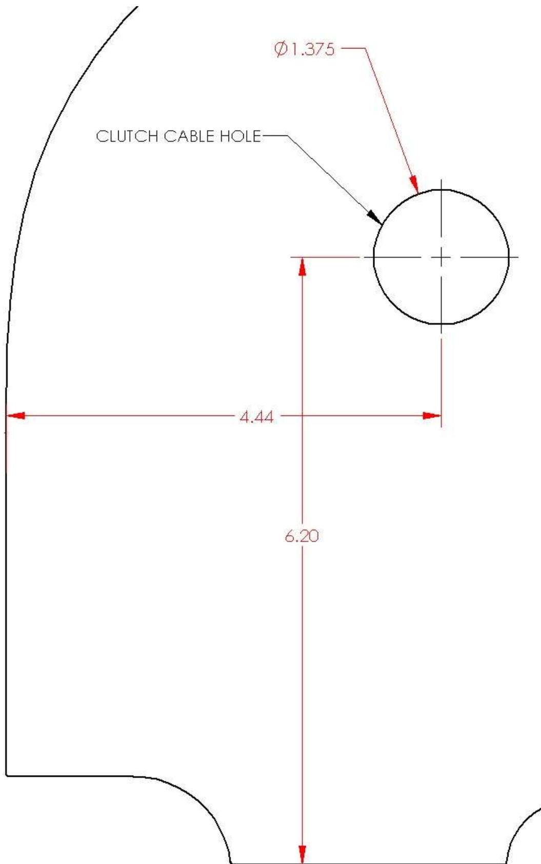
Drill the center mark with a  $\frac{3}{16}$ " drill bit
