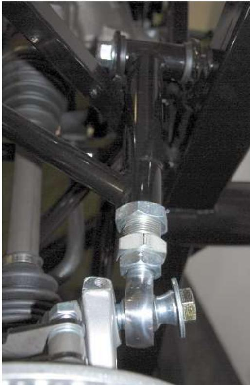
Check the angle of the upper control arm rod end, make sure that the rod end is not touching the spindle and that it is aligned with the upper control arm.
