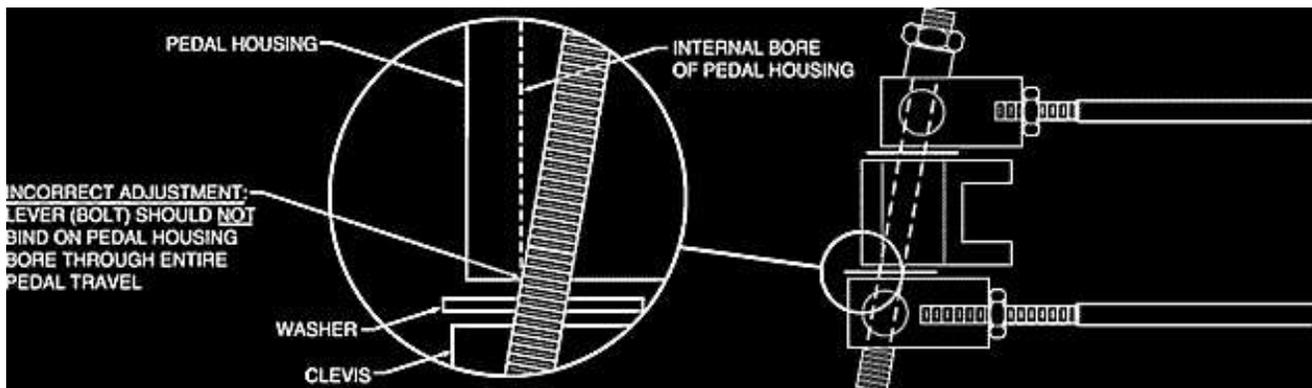
It is important that the operation of the balance bar functions without interference by over adjustment. This can occur when a clevis jams against the side of the pedal or the lever (bolt) hits the pedal bore during any point of pedal travel.
