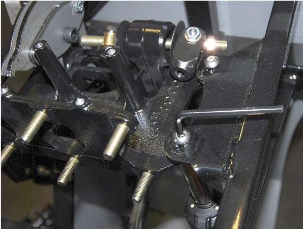
Attach the pedalbox to the underside of the frame brackets using the  $\frac{5}{16}$ " x 1" button head screws, locknuts,  $\frac{3}{16}$ " hex key and  $\frac{1}{2}$ " socket.
