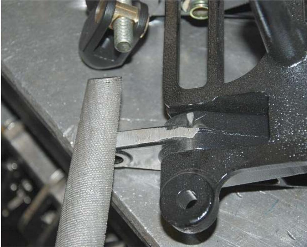
If necessary use a file to remove the forging centerline so the  $\frac{3}{8}$ " bolt can go through the clutch pedal hole.
