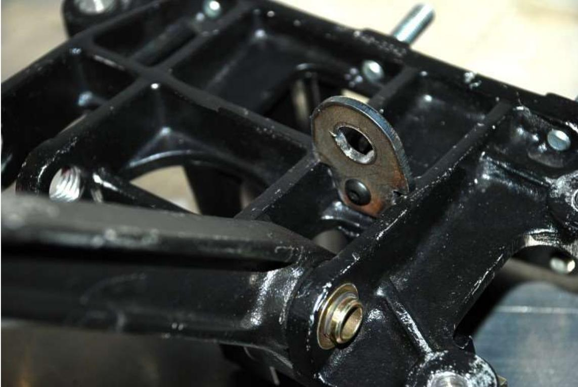
Place the brake switch mount between the brake pedal mount tabs on the side closest to the brake pedal pivot holes and drill a  $\frac{3}{16}$ " hole through the brake switch mount hole and the pedal box.
