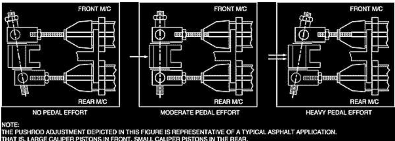
Sometimes this will lead to a “cocked” balance bar when the pedal is in the relaxed position, “no pedal effort”. This is acceptable as long as each master cylinder pushrod is completely free of pressure when the pedal is relaxed.
