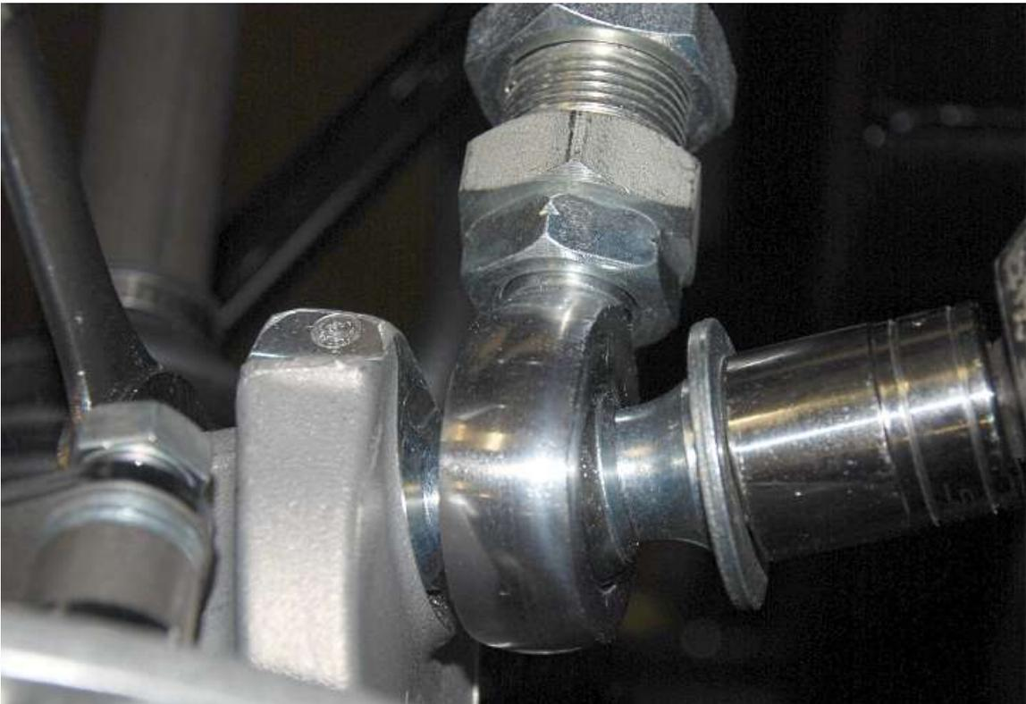
Use a  $\frac{15}{16}$ " wrench,  $\frac{15}{16}$ " socket and ratchet to tighten the locknut.
