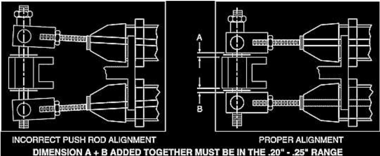
Make sure that the master cylinder pushrods remain true in relationship to the cylinder during entire pedal travel; pushrods should not be pushing master cylinder pistons at an angle.
