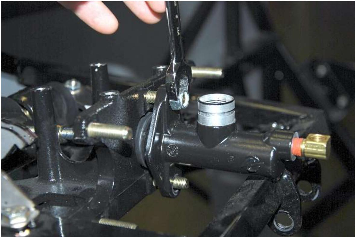
✎ Attach and tighten the locknuts using a 1/2" wrench holding the master cylinder to the pedal box then repeat for the other master cylinder.
