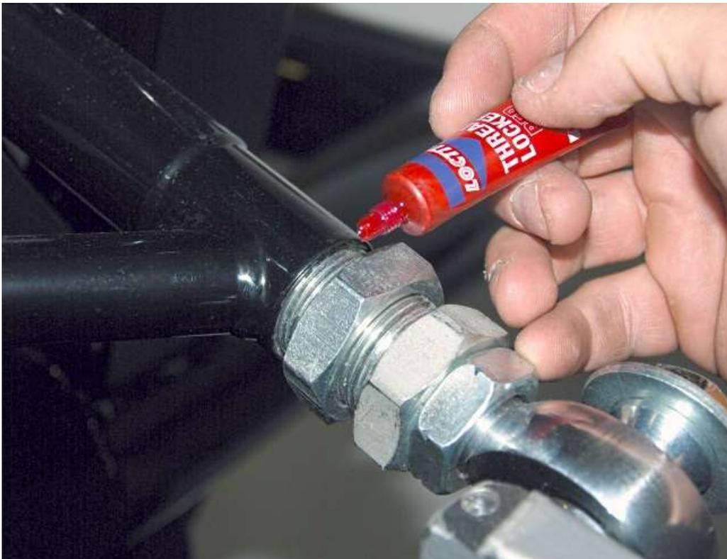
Once the car has been aligned, use a  $1\frac{5}{8}$ " wrench to loosen the upper control arm large jam nut and put some Loctite on the threads where the jam nut will sit.
