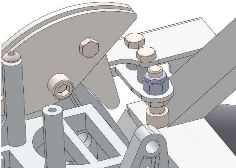
Install the aluminum spacers between the frame and the clutch quadrant stop bracket and fasten using  $\frac{1}{4}$ "-20 x 1.25" screws.
