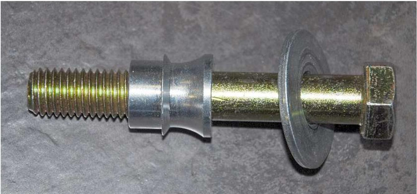
Reuse the  $\frac{5}{8}$ " washer that was on the old bolt and place it on the new  $\frac{5}{8}$ " x 4.25" bolt along with a misalignment spacer.
