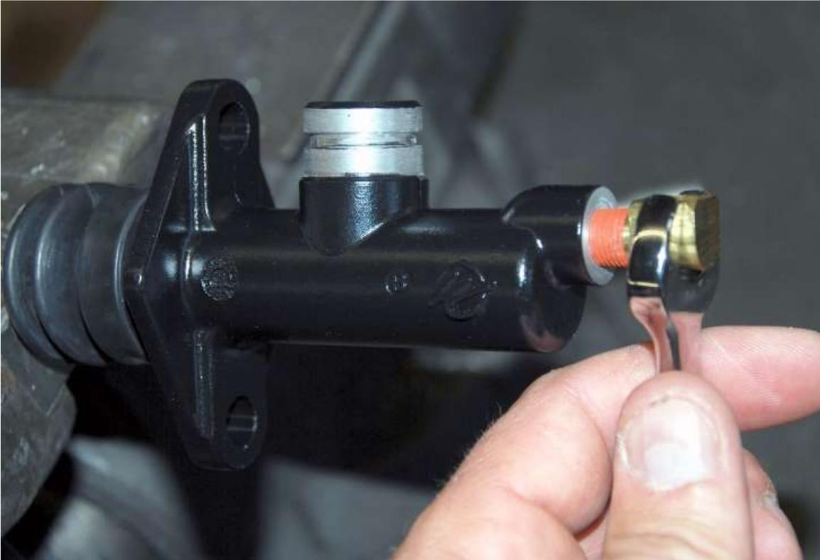
Screw the 90° brake line adapter into the end of the master cylinder making sure that the opening points up when tight.
