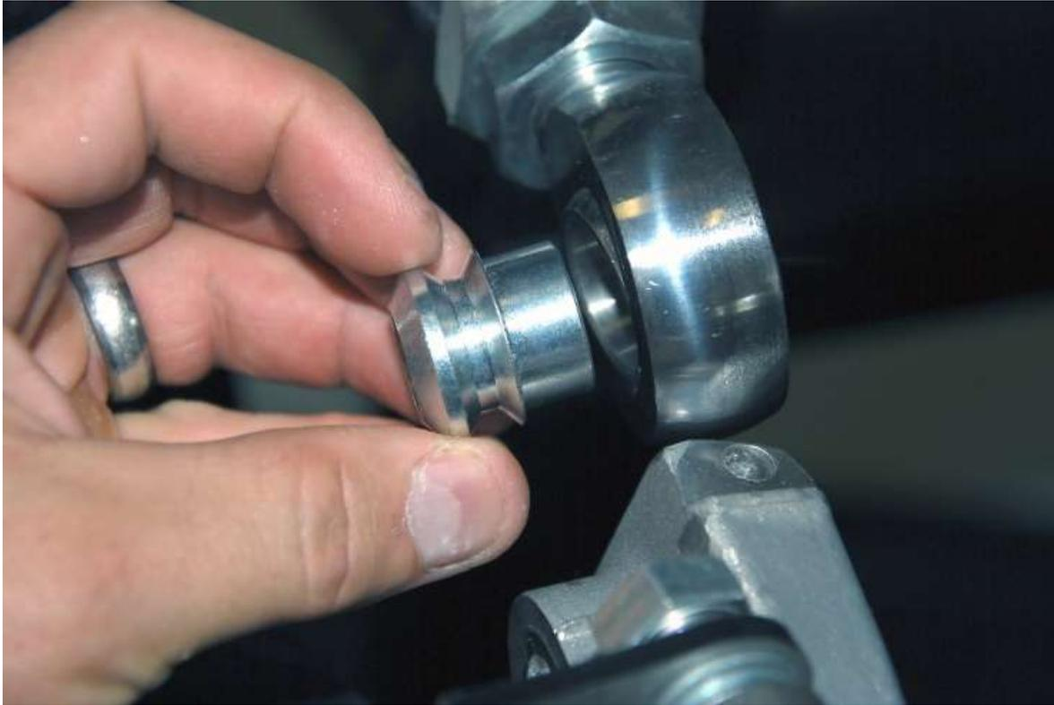
Insert the angled mount adapter into the upper arm rod end.
