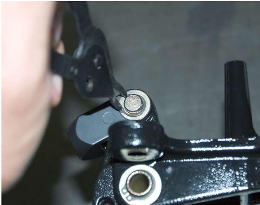
Use snap ring pliers to remove the clevis at the top of the clutch pedal.
