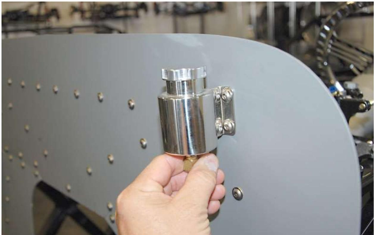
The reservoir can either be mounted in the engine bay on the firewall or on the inside of the firewall depending on personal preference.
