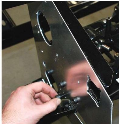
Insert three  $\frac{3}{8}$ " x 1" socket head screws from the pedal box hardware assembly and the one included in this pedal assembly through the front of the footbox and through the pedal box mount.
