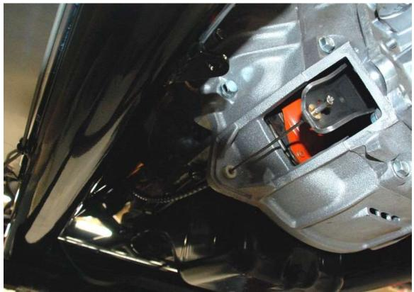
Connect the clutch cable to the bellhousing and the clutch fork.
