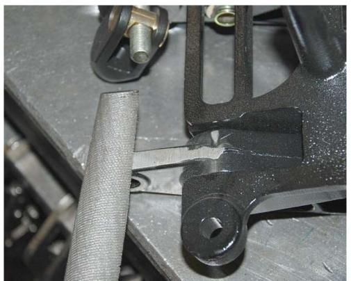
If necessary use a file to remove the forging centerline so the 3/8" bolt can go through the clutch pedal hole.
