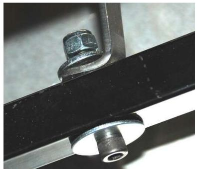
Reinstall the pedal box assembly in the driver's footbox; use the  $\frac{1}{4}$ 'x 1.50" screws from the pedal box fastener assembly with a fender washer next to the head. Leave all the hardware hand tight.
