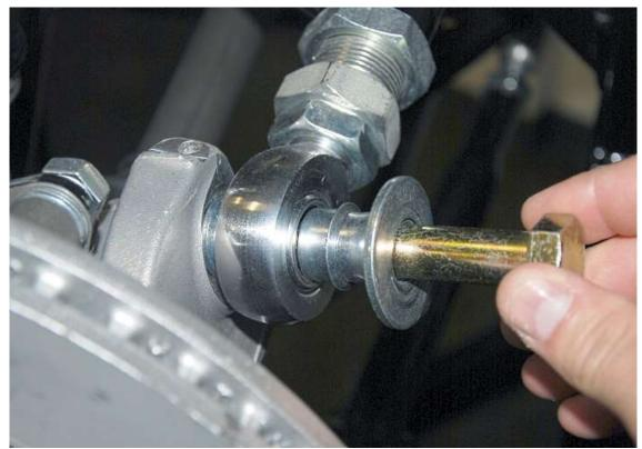
Attach the upper control arm to the spindle using the bolt with the misalignment spacer.
