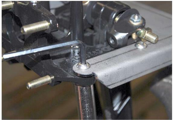
Attach the Wilwood pedals to the underside of the mounting bracket using four  $\frac{5}{16}$ " Button head screws, locknuts,  $\frac{3}{16}$ " hex key and  $\frac{1}{2}$ " wrench.
