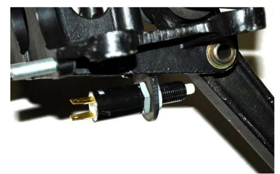
Attach the brake switch mount to the pedal box using the black #10 screw and locknut.
