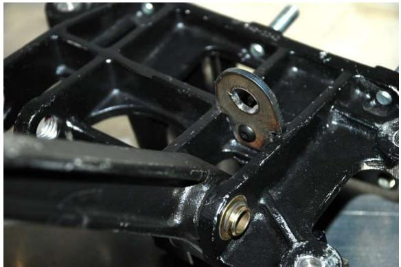
Place the brake switch mount between the brake pedal mount tabs on the side closest to the brake pedal pivot holes and drill a  ${}^{3}/{}_{16}$ " hole through the brake switch mount hole and the pedal box.
