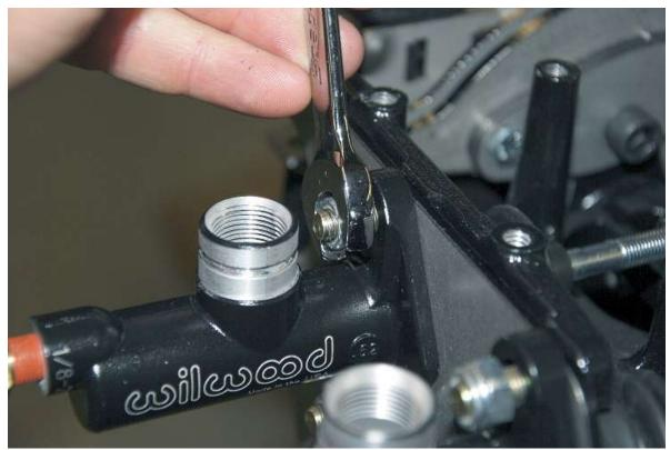
Attach and tighten the locknuts using a  $\frac{1}{2}$ " wrench and  $\frac{1}{2}$ " deep socket holding the master cylinder to the pedal box then repeat for the other master cylinder.
