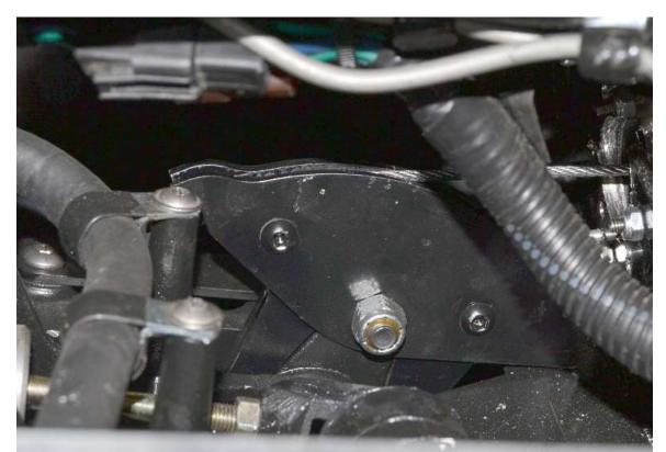
Slide the clutch cable boss through the firewall spacer and loop the cable over the quadrant.
