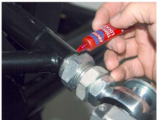
Once the car has been aligned, use a  $1^{5}/_{8}$ " wrench to loosen the upper control arm large jam nut and put some Loctite on the threads where the jam nut will sit.
