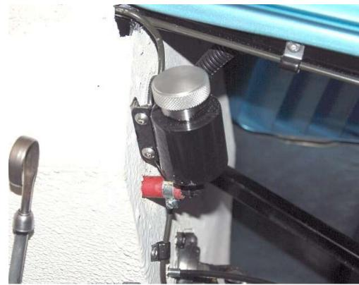
The brake reservoir mounts to the front of the footbox just inside the hood opening. Take the reservoir with cap and line it up so the top is in line with the top of the hood support tube and mark the holes.
