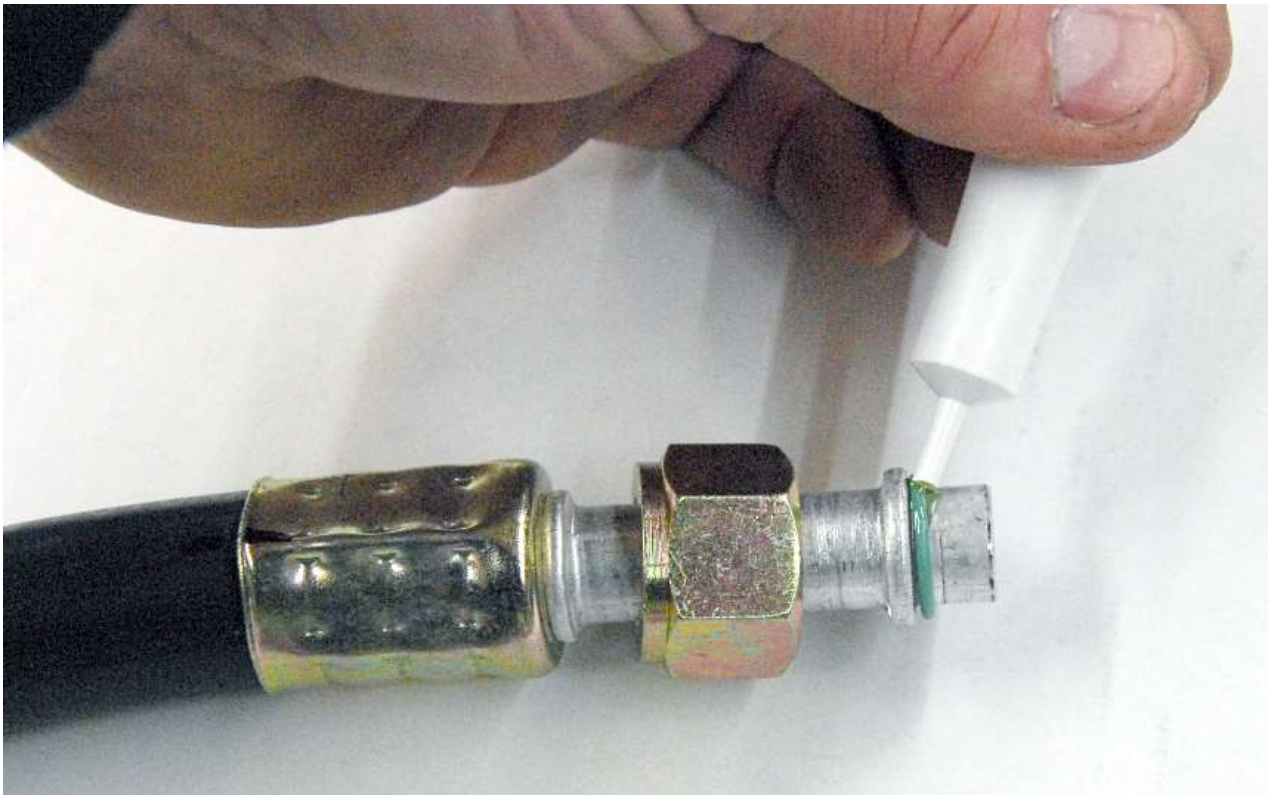
Lubricate the o-ring with the oil included.
