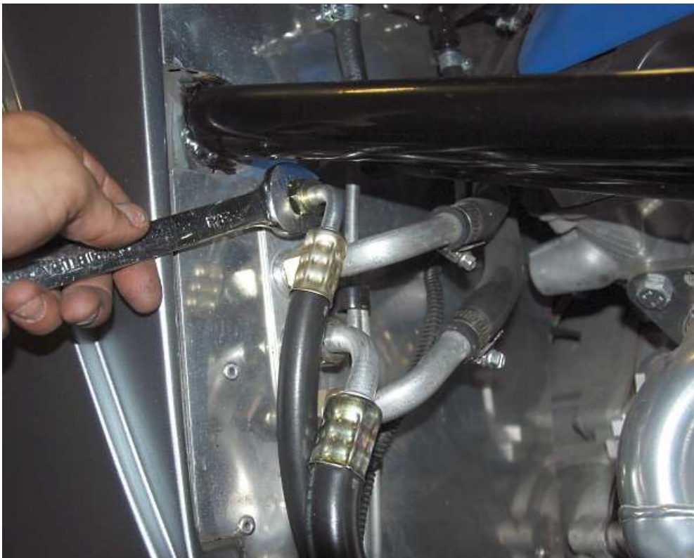
Reconnect and tighten the engine bay firewall hoses.
