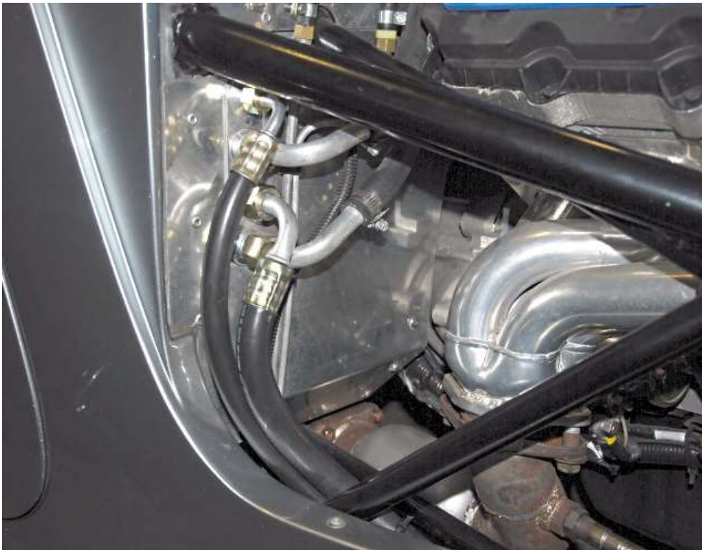
Cut and insert the heater control valve in one of the heater hoses.
