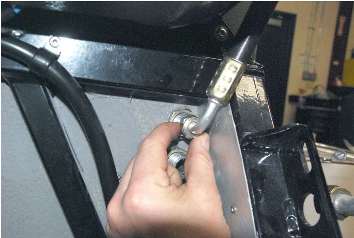
Screw on the top inside A/C fitting by hand then tighten using a \frac{3}{4} " wrench.
