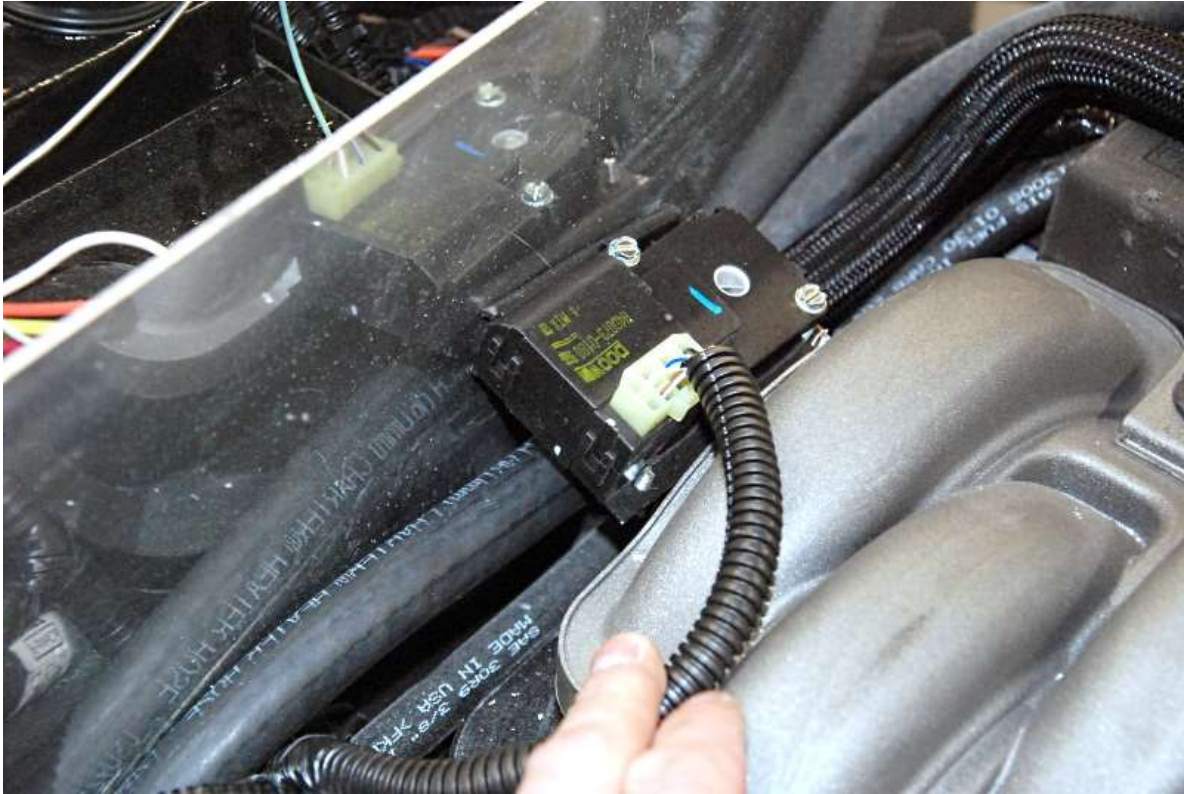
Cut and insert the heater control valve in one of the heater hoses.
