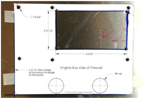
Drill all of the holes indicated and 1/8" holes in the corners of the large rectangular hole.
