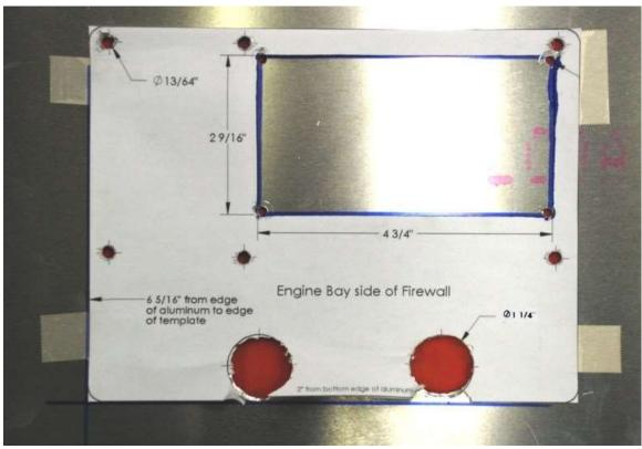
Use a 1<sup>1</sup>/<sub>4</sub>" hole saw to cut the two 1.25" holes marked.
