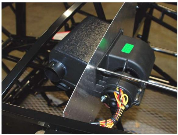
Re assemble the heater with the blower motor in the engine bay and the heater core in the passenger compartment using the screws taken off before.
