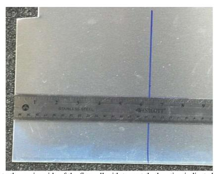
Attach the template to the engine side of the firewall with tape at the location indicated on the template.
