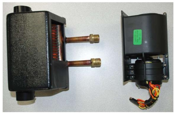
Take the heater unit apart so that the blower motor is separate from the rest of the heater box by removing the six Philips head screws holding the motor onto the heater box.
