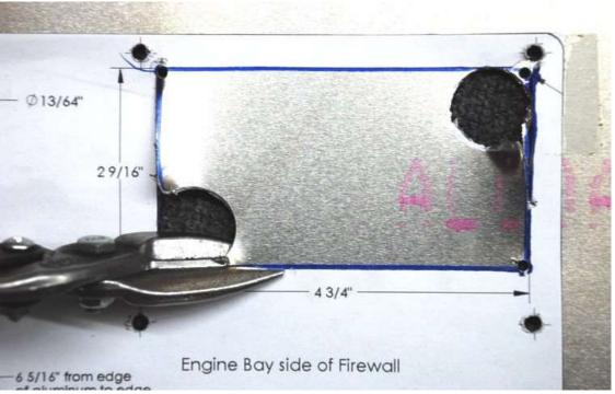
Cut the large hole with tin snips.
