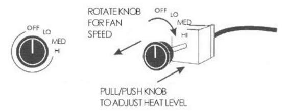
Check the operation of the switch. Full counter clockwise is off.
