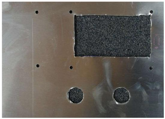
Remove the template from the firewall and use some brake or Carb cleaner to remove the marker lines.
