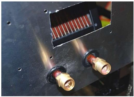
Insert the heater core tubes into the small holes and push the grommets into the holes.
