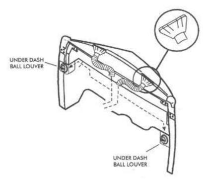
Route duct hose up to the defroster ducts and push them onto the plastic defroster ducts.
