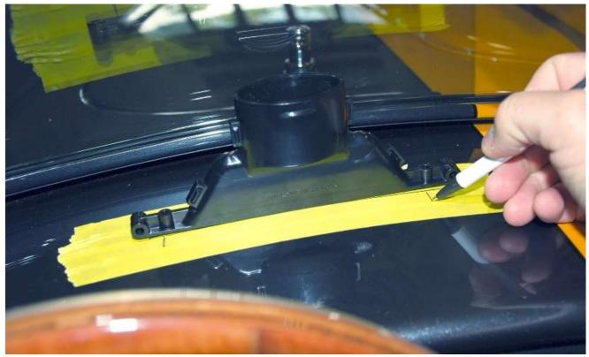
Use a pen to lightly draw a line on the side of the duct closest to you and where the mounting holes are.
