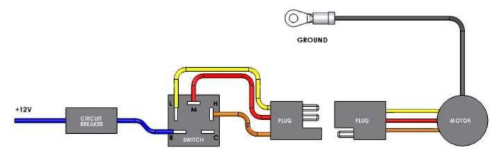
Connect the power wire shown below to an open +12v switched power source in the fuse panel.
