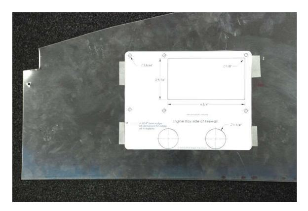
Mark the edge of the large hole using a marker.
