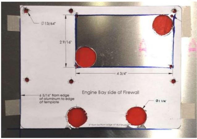
Use the 11/4" hole saw in two opposite corners of the large rectangular hole so that the edge of the saw lines up with the two sides.
