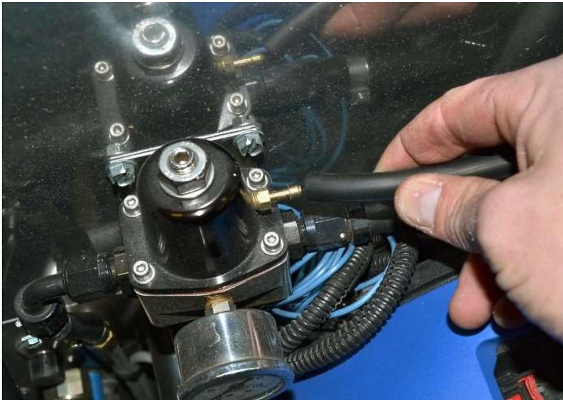
Run the vacuum line to the fuel pressure regulator and push it onto vacuum barb.
