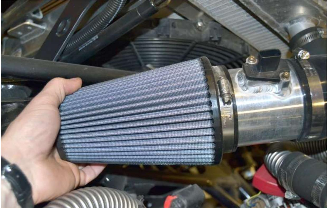
Push the FFR filter onto the Mass Air meter making sure that the meter is facing the correct direction.
