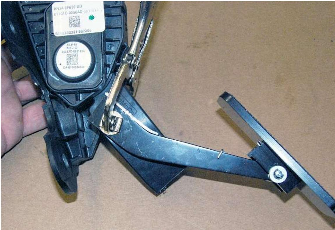
Remove the pedal from the car and check the alignment of the two pedals with the line you just drew.
