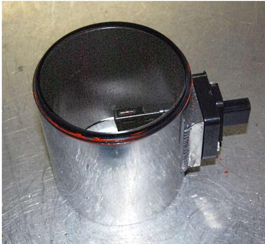
Turn the mass air meter over so the Reducer is on the top and let the RTV dry overnight.
