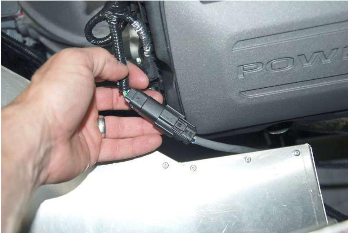
Attach the right O<sub>2</sub> sensor to the connector at the back of the head.
