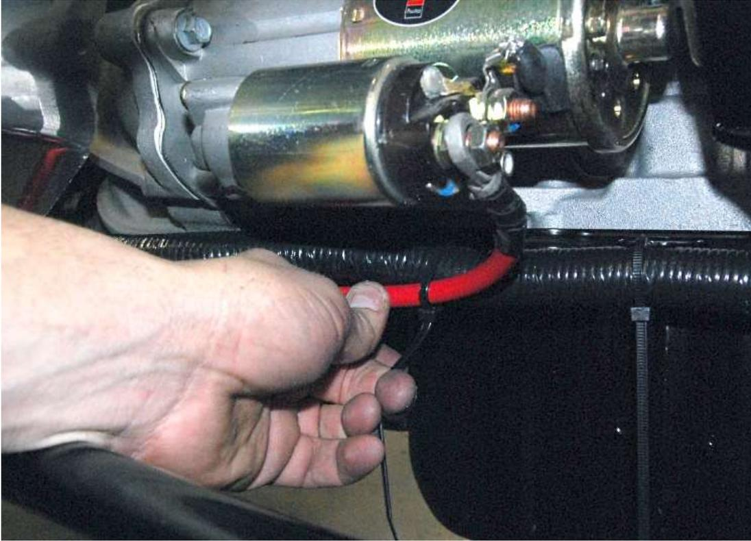
Attach the battery cable to the starter solenoid.
