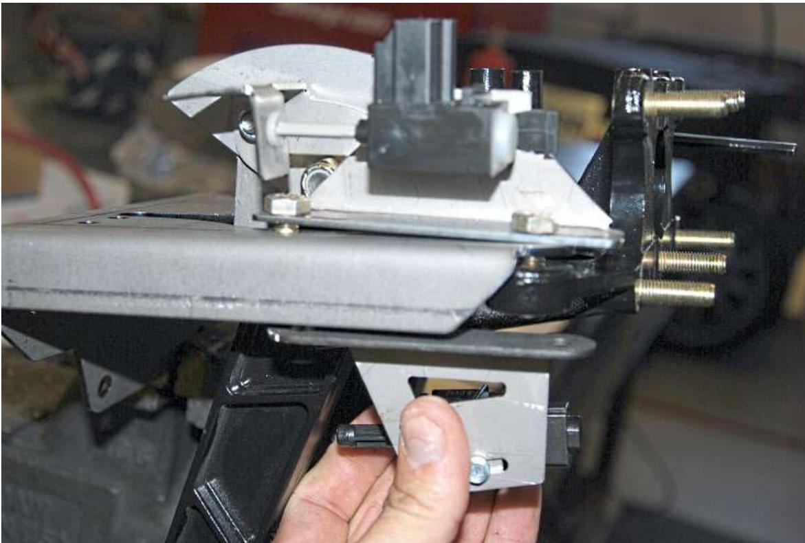
Attach the top travel clutch switch bracket to the bottom of the bolts.
