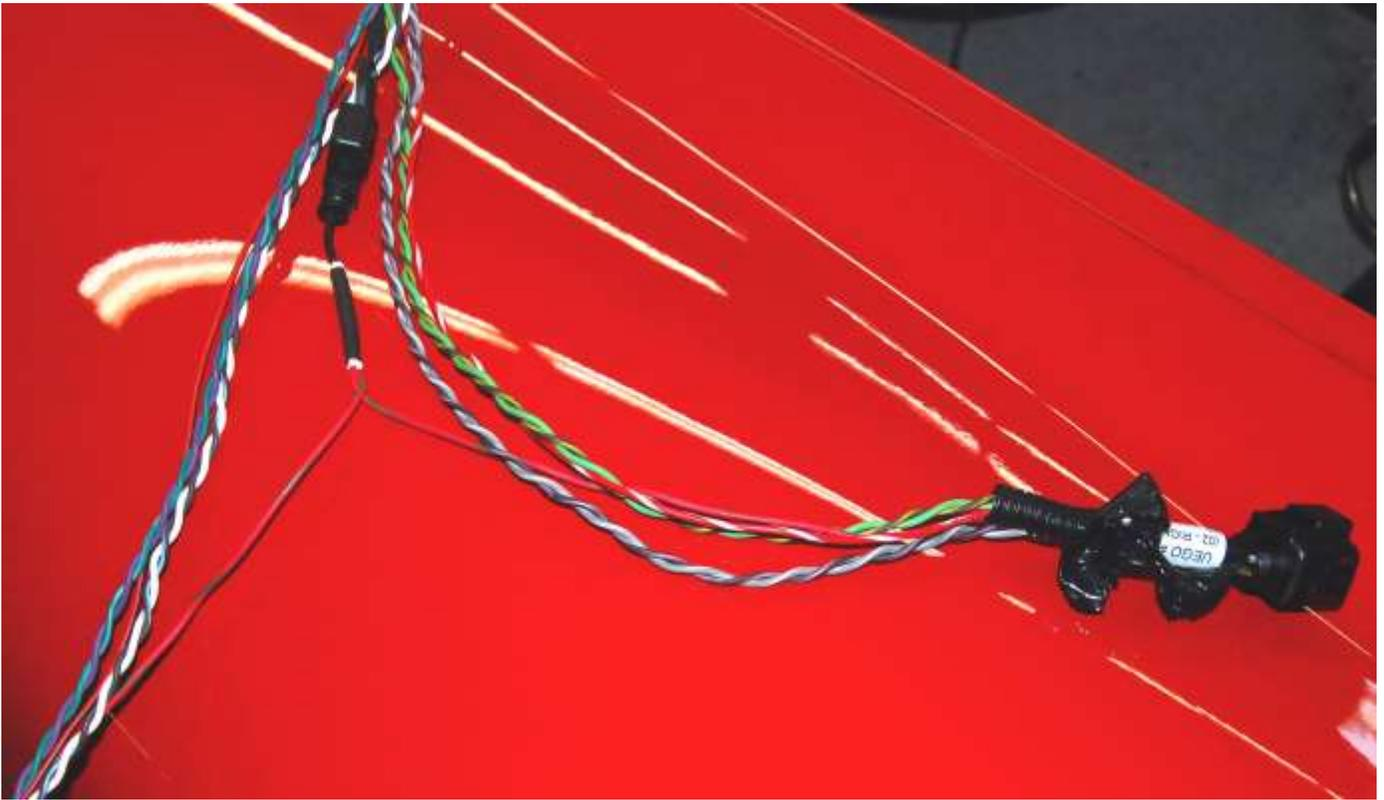
Locate the red/black power wire junction between the two O<sub>2</sub> sensor plugs.
