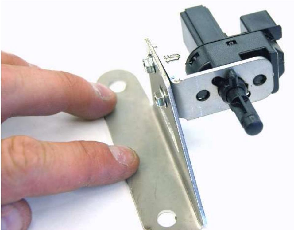
Insert the Top travel (black plunger) clutch switch into the bracket and turn it to the position shown to lock it into place.
