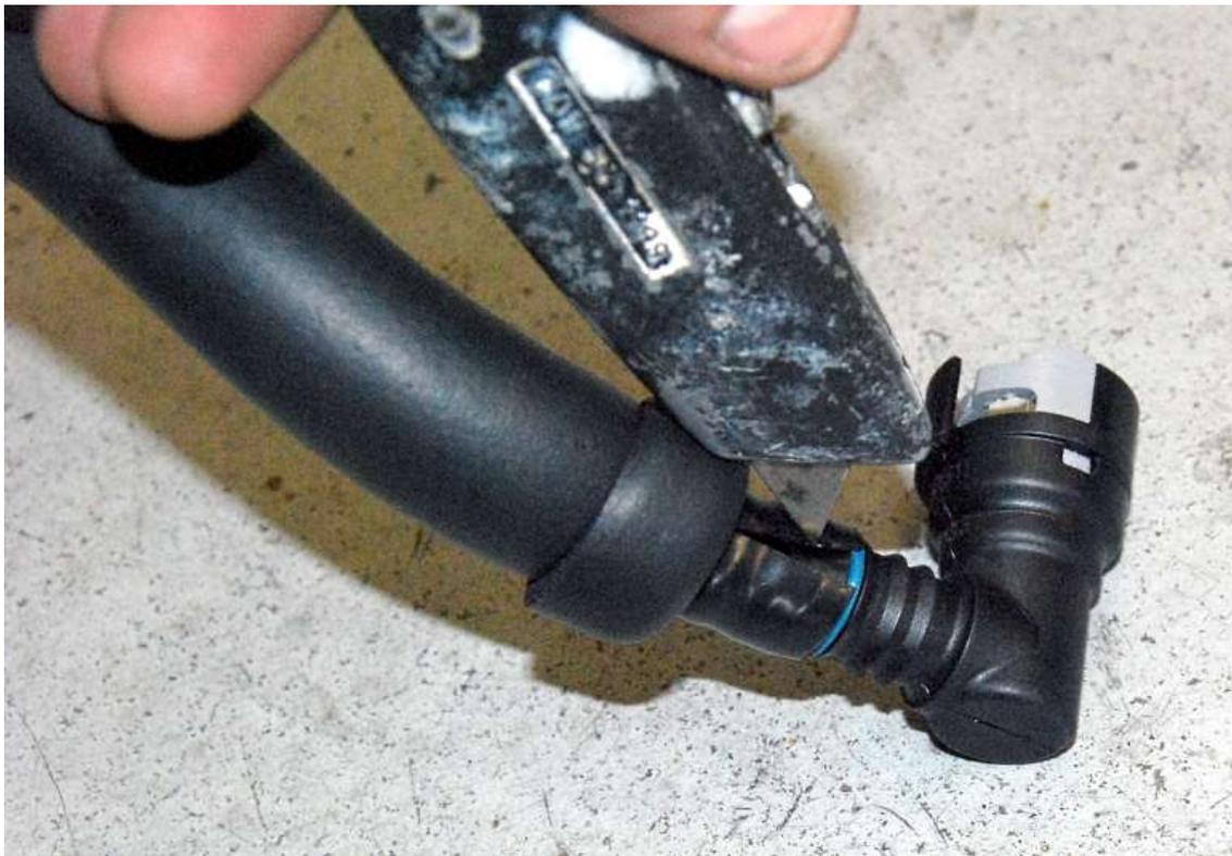
Carefully cut the 90° PCV fittings out of one of the pcv lines without damaging the barbs.
