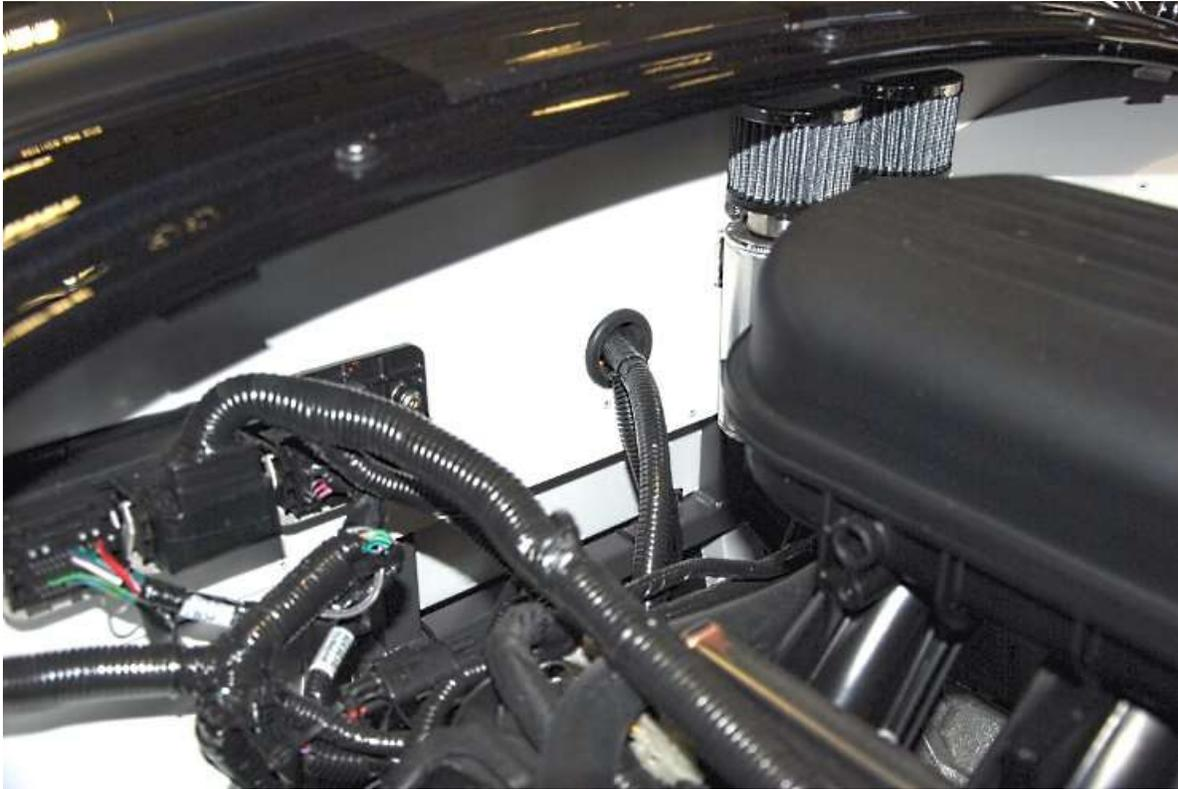
Drill a 1" hole at the bottom in the center of the firewall then insert the expandable grommet.
