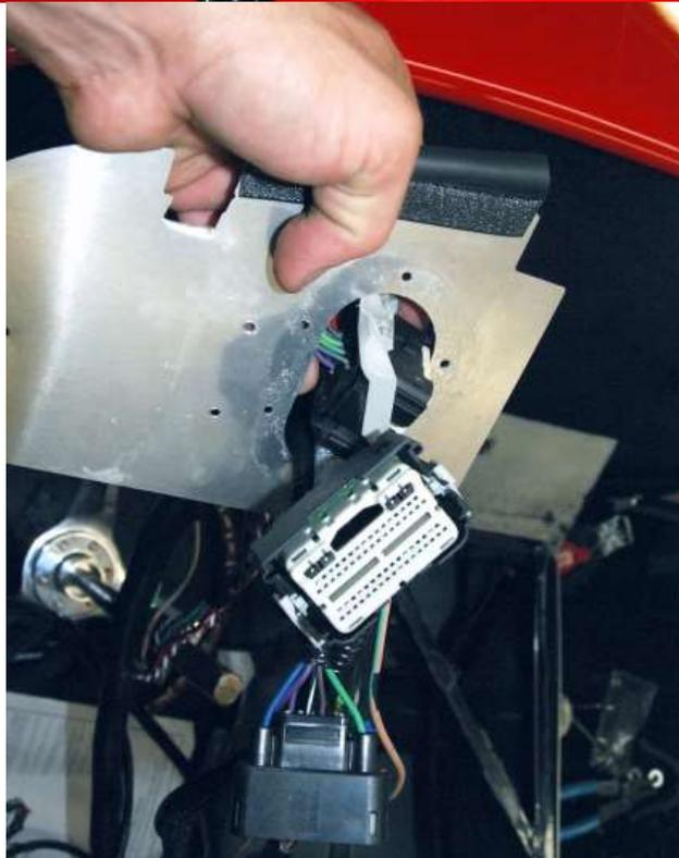
Pass the O<sub>2</sub> harness, computer plugs and other wires in the engine harness through the firewall extension hole into the engine bay.
