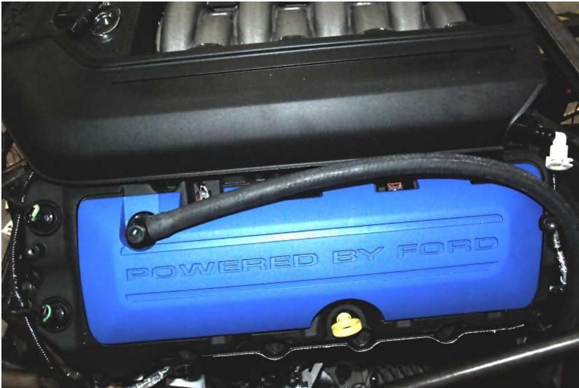
Push the fitting onto the left valve cover and run the hose the back of the engine.
