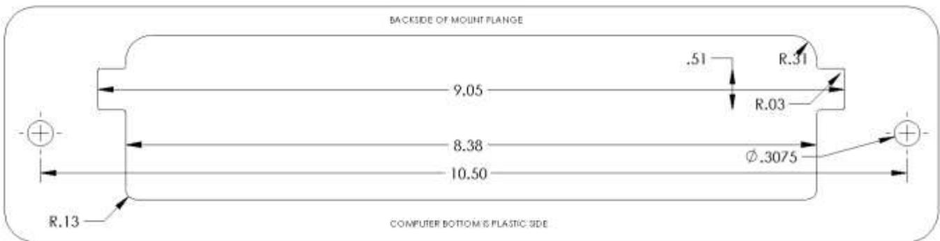
This diagram can be scaled on a copier to create a template. Measurements are in inches.
