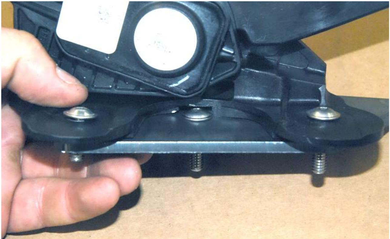
Check the fitment of the mount screw by putting the pedal on the pedal mount with the screws.
