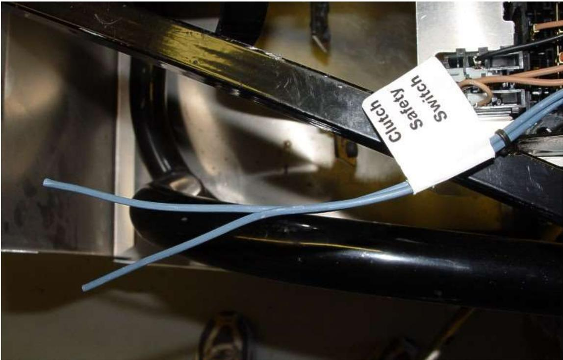
If a neutral safety switch is not going to be used, connect the two blue chassis harness wires together by either soldering the wires or using a butt connector from the “misc. electrical components” assembly in the Factory Five Racing main kit pack.
