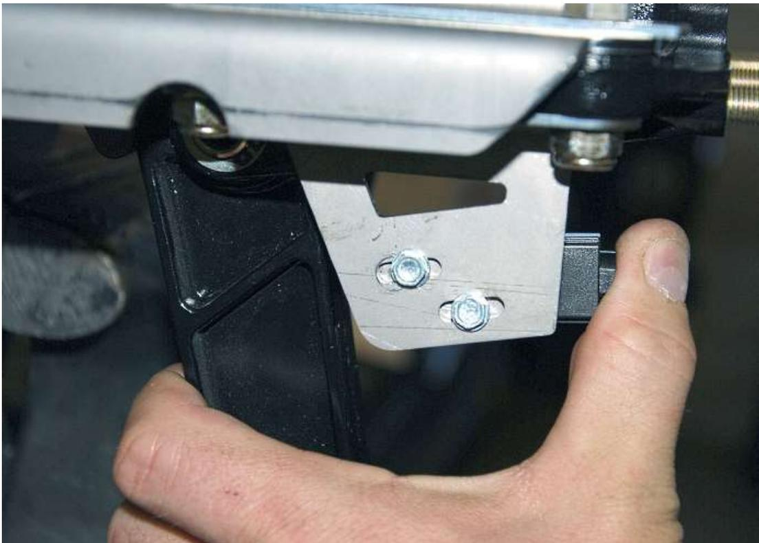
With the clutch pedal in its normal position, push the top travel switch in until it bottoms out on the pedal then tighten the #8 screws with a 1/4" socket and ratchet.
