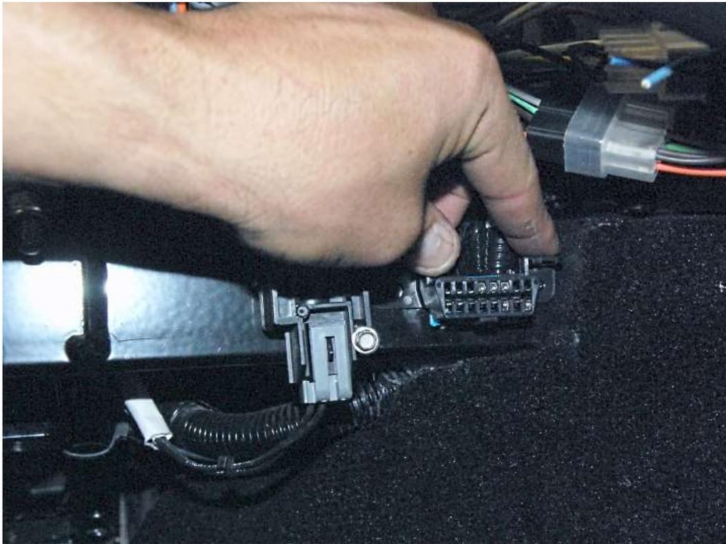
Locate the OBD 2 port on the 2"x 2" tube to the right of the steering wheel.
