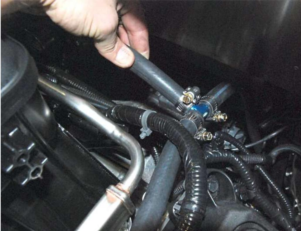
Push the remainder of the hose onto the third leg of the “T” and run it down the side of the bellhousing and zip tie it to the transmission tunnel tube.
