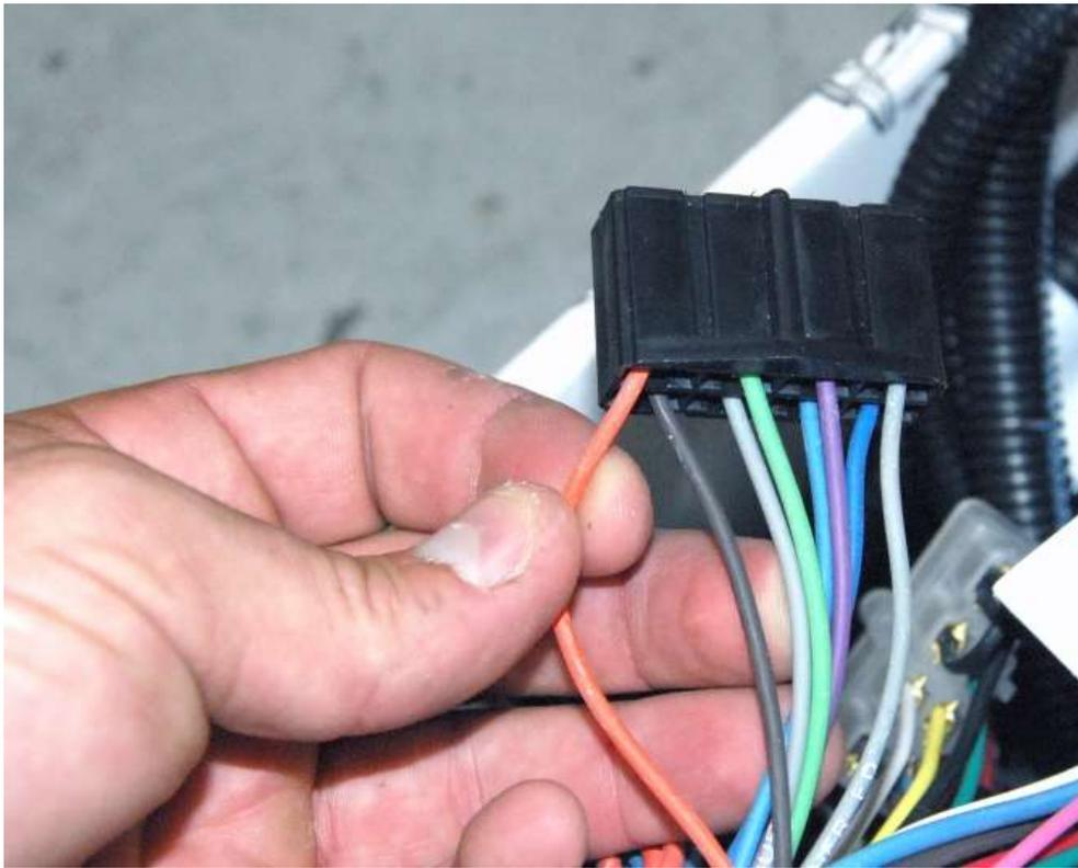
At the top of the footbox area, find the chassis harness orange fan wire in the dash harness plugs.
