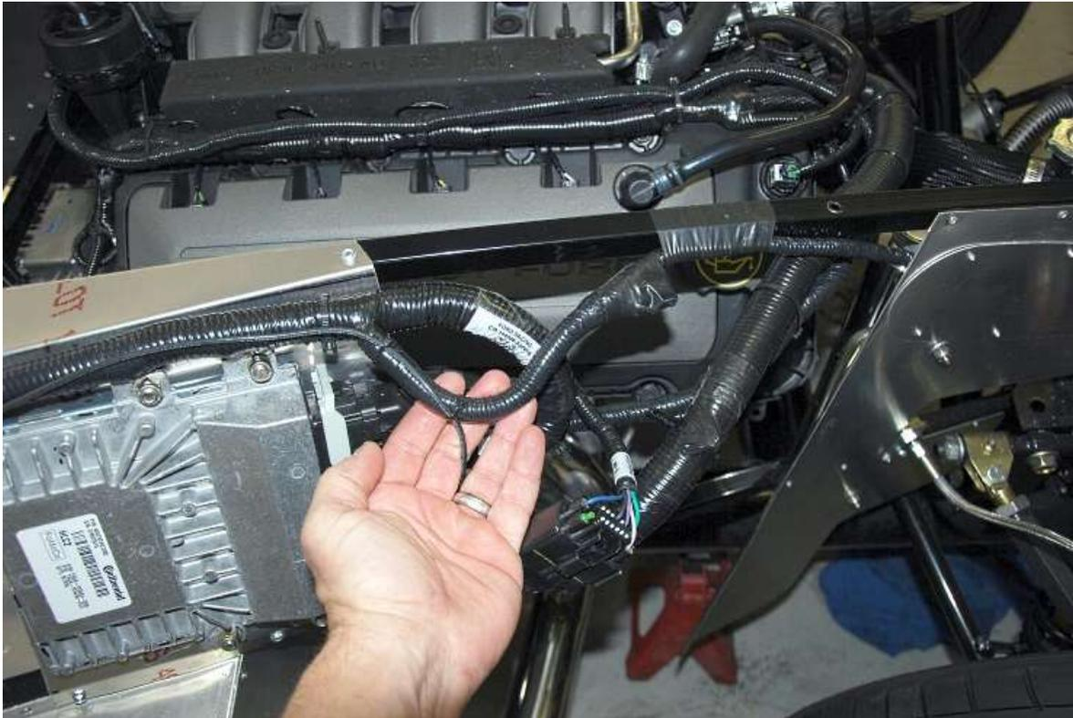
From the computer area, run the harness with the orange fan wire forward to the fan and connect to the blue fan wire.
