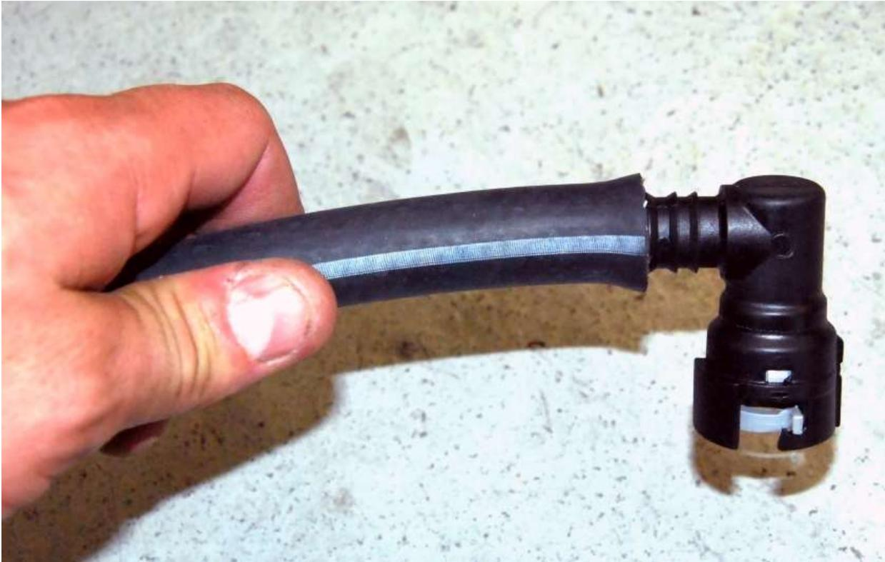
Push the ½” heater hose onto the PCV fitting.
