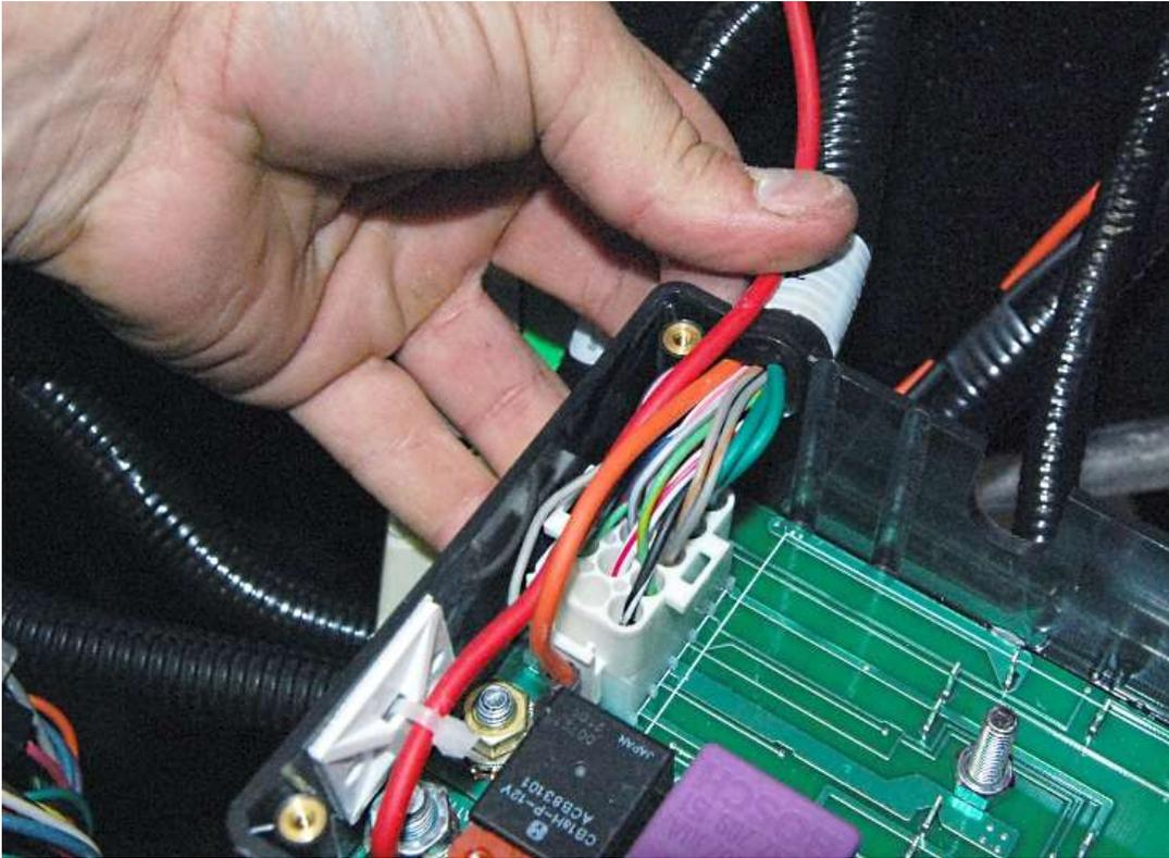
Run the white plug wires and the orange fan plug out of the box in the slot provided near the plug.
