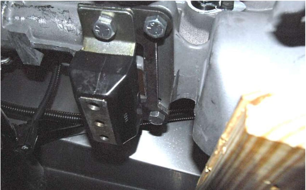
Attach the polyurethane transmission mount assembly to the transmission.
