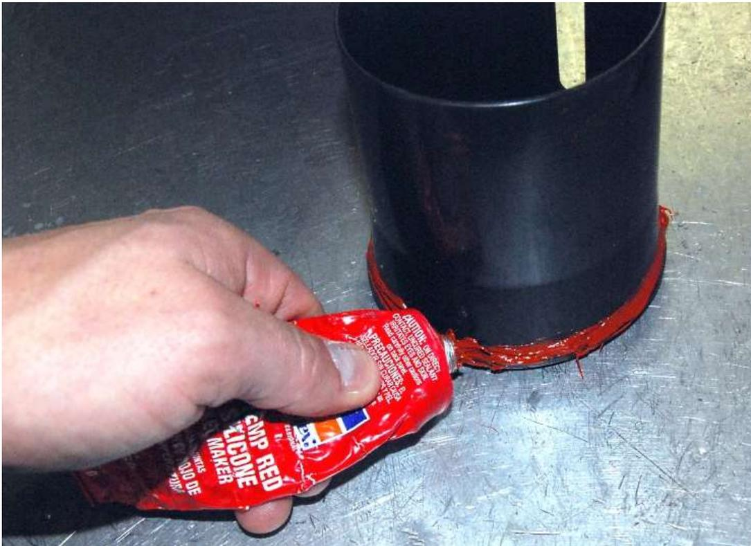
Run a bead of Sensor safe RTV silicone around the flange of the large plastic reducer.
