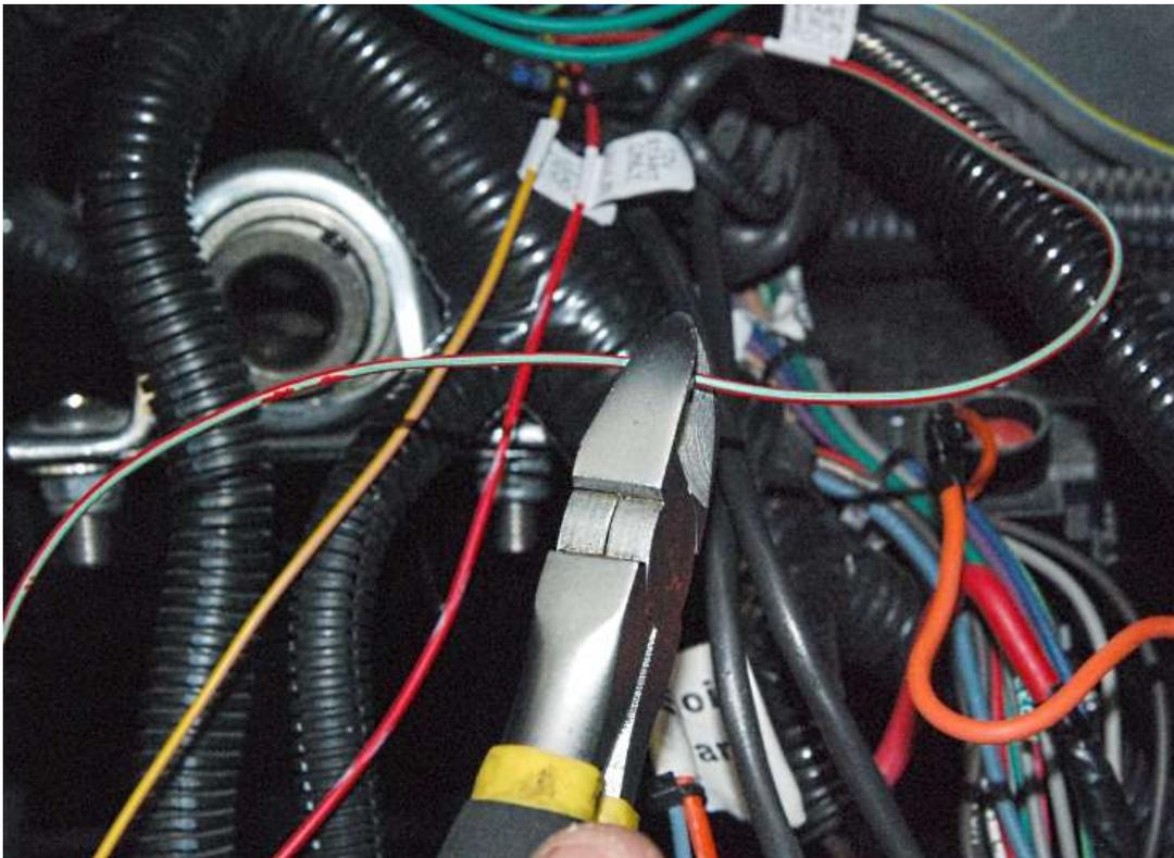
Route the Coyote 12v start/run wire (red/green) and 12v start (red/blue) wires to the chassis harness EFI wires and cut to length.
