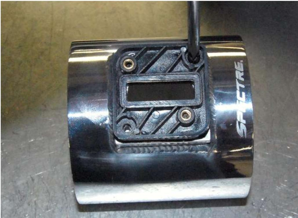
Attach the mount to the intake tube using the long screws so that the flat side of the sensor will face the “Spectre” writing.
