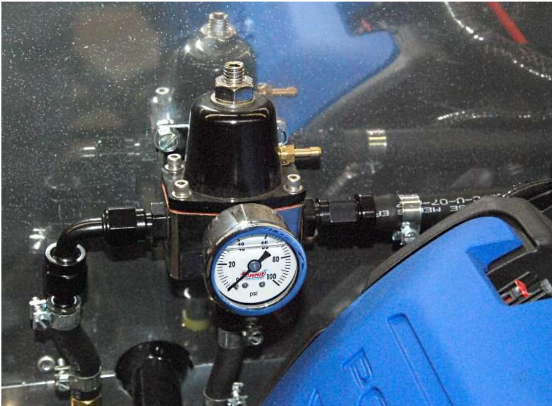
Push the  $\frac{3}{8}$ " fuel line onto the right side of the regulator then attach a hose clamp and run it over to the engine fuel rail.
