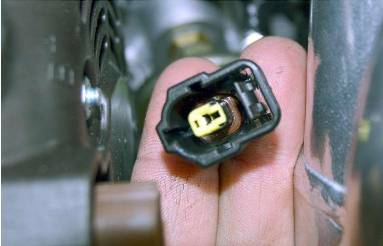
Remove the stock oil pressure gauge sender plug from the block located on the left front side of the engine. This plug will not be used again
