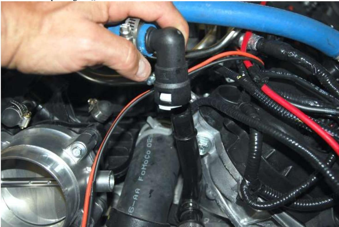
Push the hose onto the top of the tube to the left of the throttle body.
