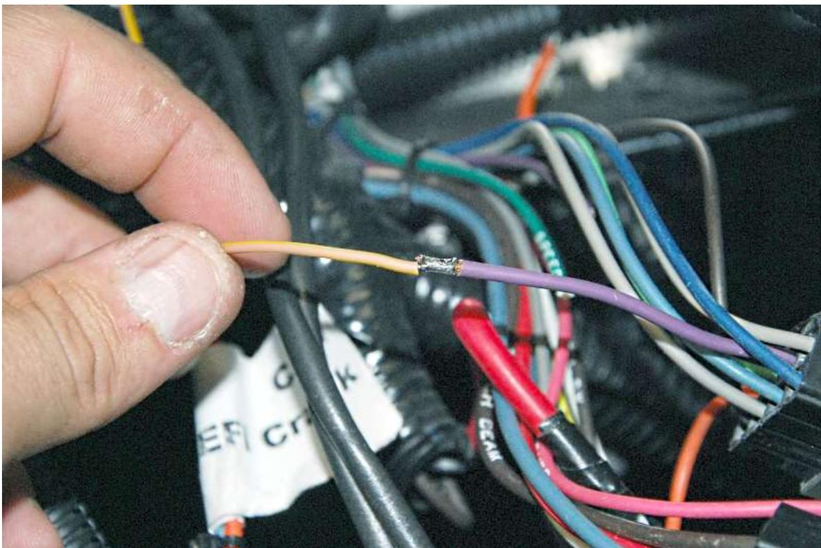
Connect the tach wire to the chassis harness plug and connect it to the purple wire attached to the plug.
