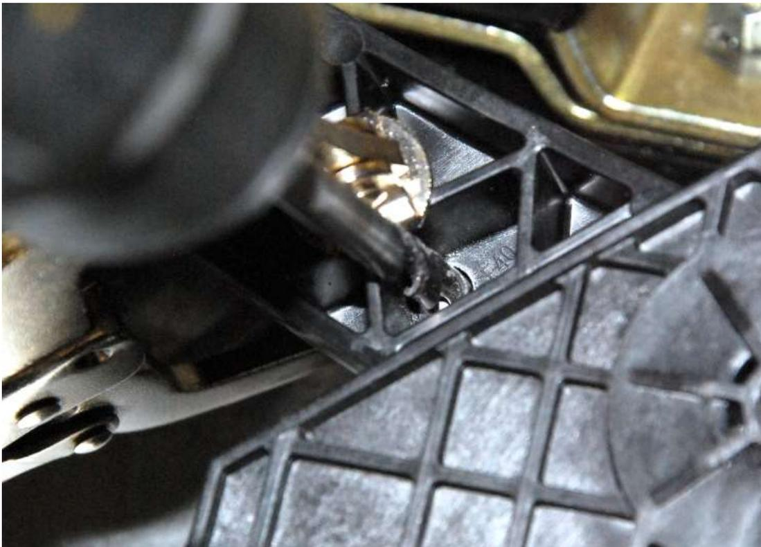
Remove the locknut and enlarge the hole using a  $\frac{1}{4}$ " drill bit.
