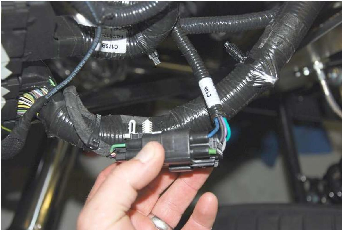
Connect the Engine harness plug to the control pack plug.
