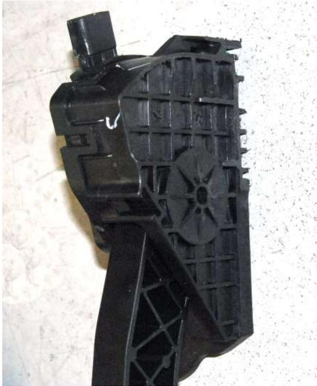
Use a hack saw to cut the right mount off the accelerator. Cut right against the flat section of the pedal so it also cuts the top Webbing off.
