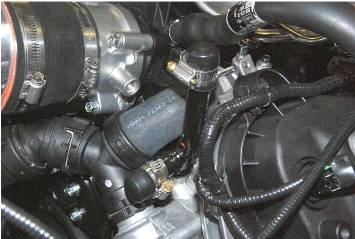
If not already done, fill the engine with coolant through an inline filler or radiator cap. To help remove air from the system, remove the top cap until coolant starts going up the tube then recap and hose clamp.
