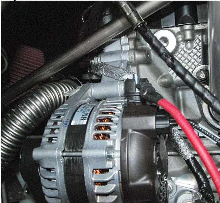
Crimp on a ring terminal and attach the red wire to the Alternator.
