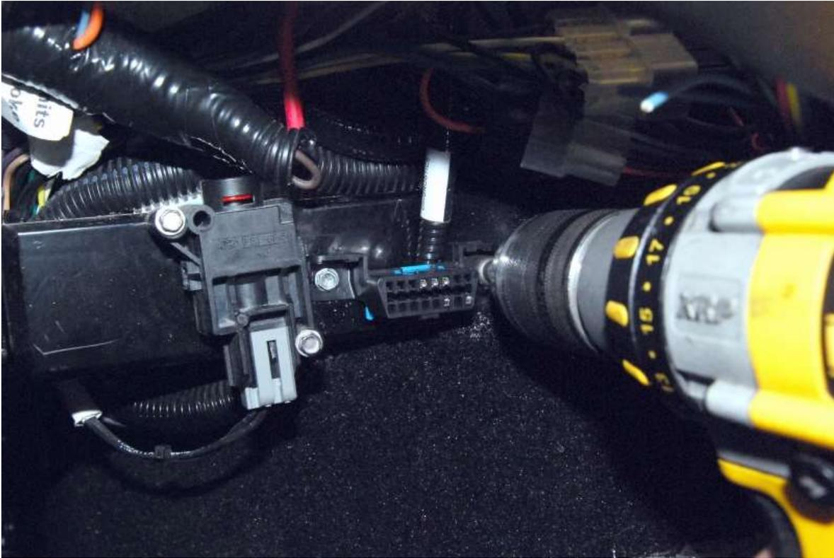
Use some of the aluminum panel #6 screws to attach the OBD 2 plug to the frame.
