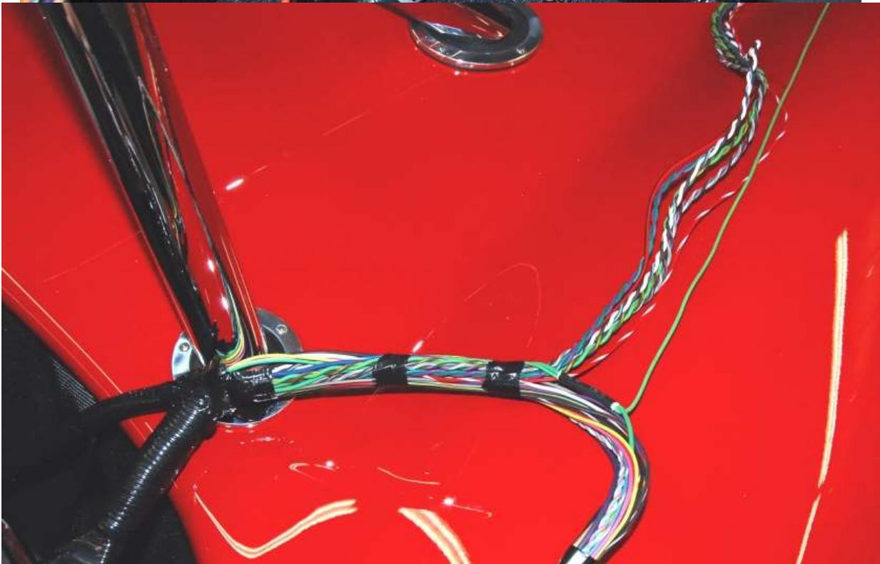
Remove the harness wrap and pull the wires back to the first harness branch. This will allow them to get routed in the engine bay with enough length.
