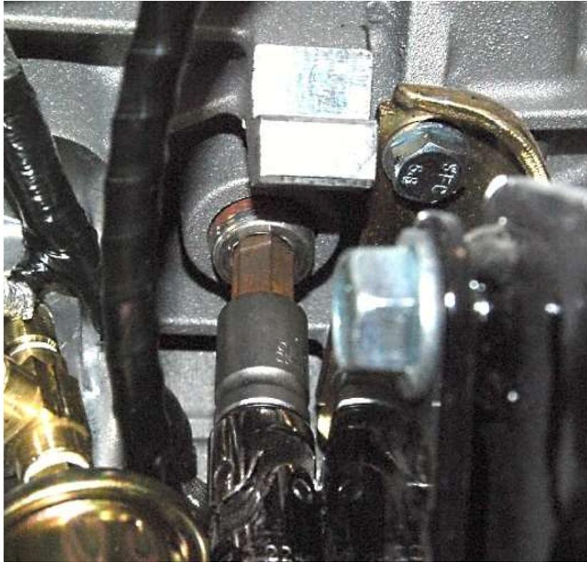
Remove the  $\frac{3}{4}$ " NPT plug from the side of the block using a H14 Hex key or socket.
