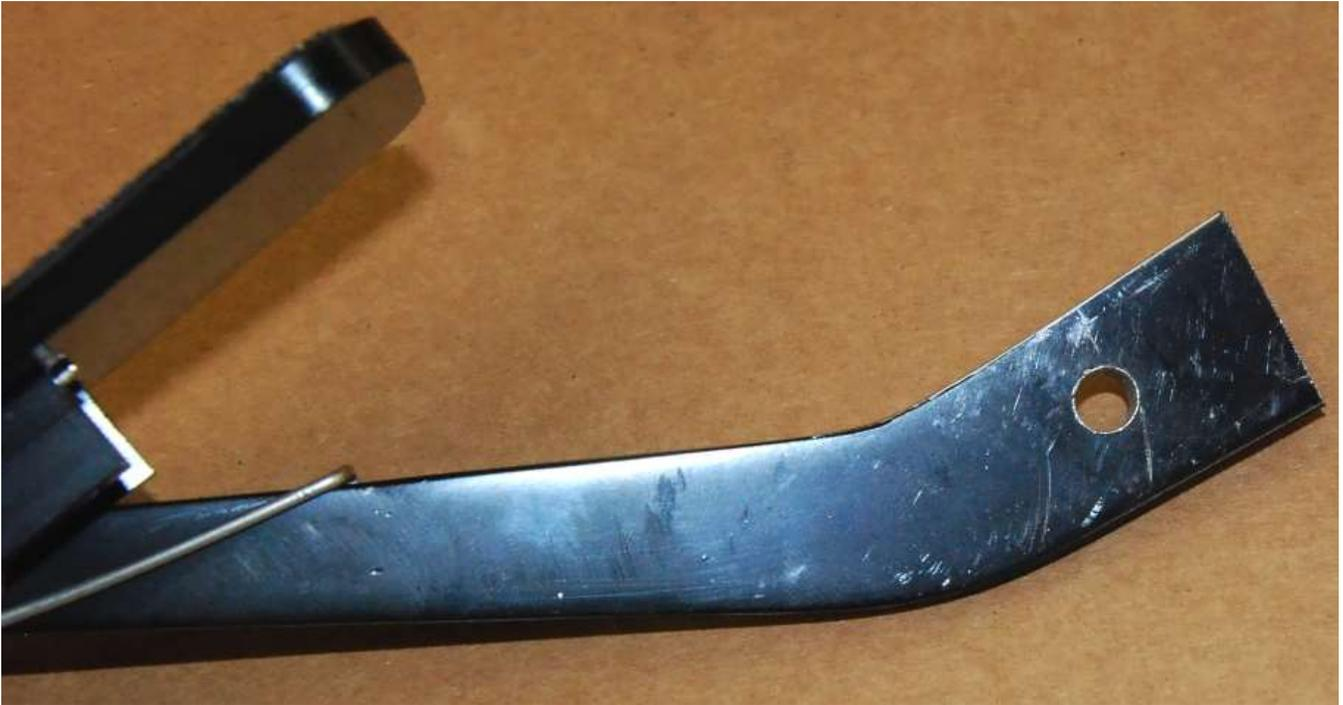
Check the alignment of the metal pedal on the plastic pedal then drill through the metal pedal using the plastic hole as a guide.
