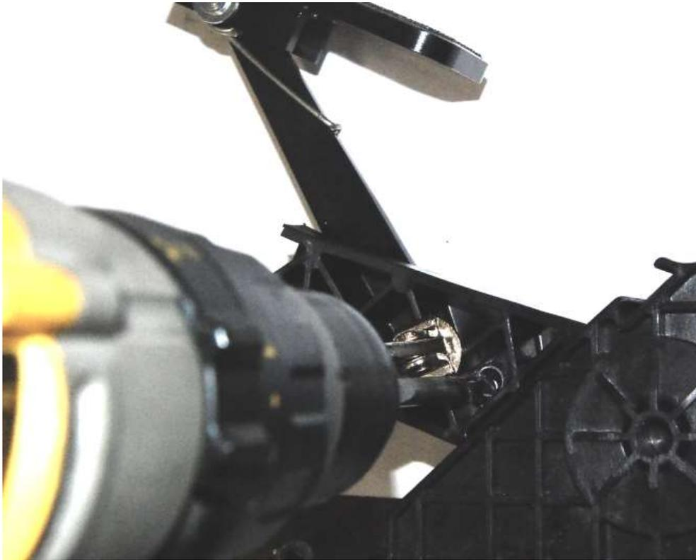
Using the locknut nylon as a guide, drill a  $\frac{3}{16}$ " hole through the plastic pedal.
