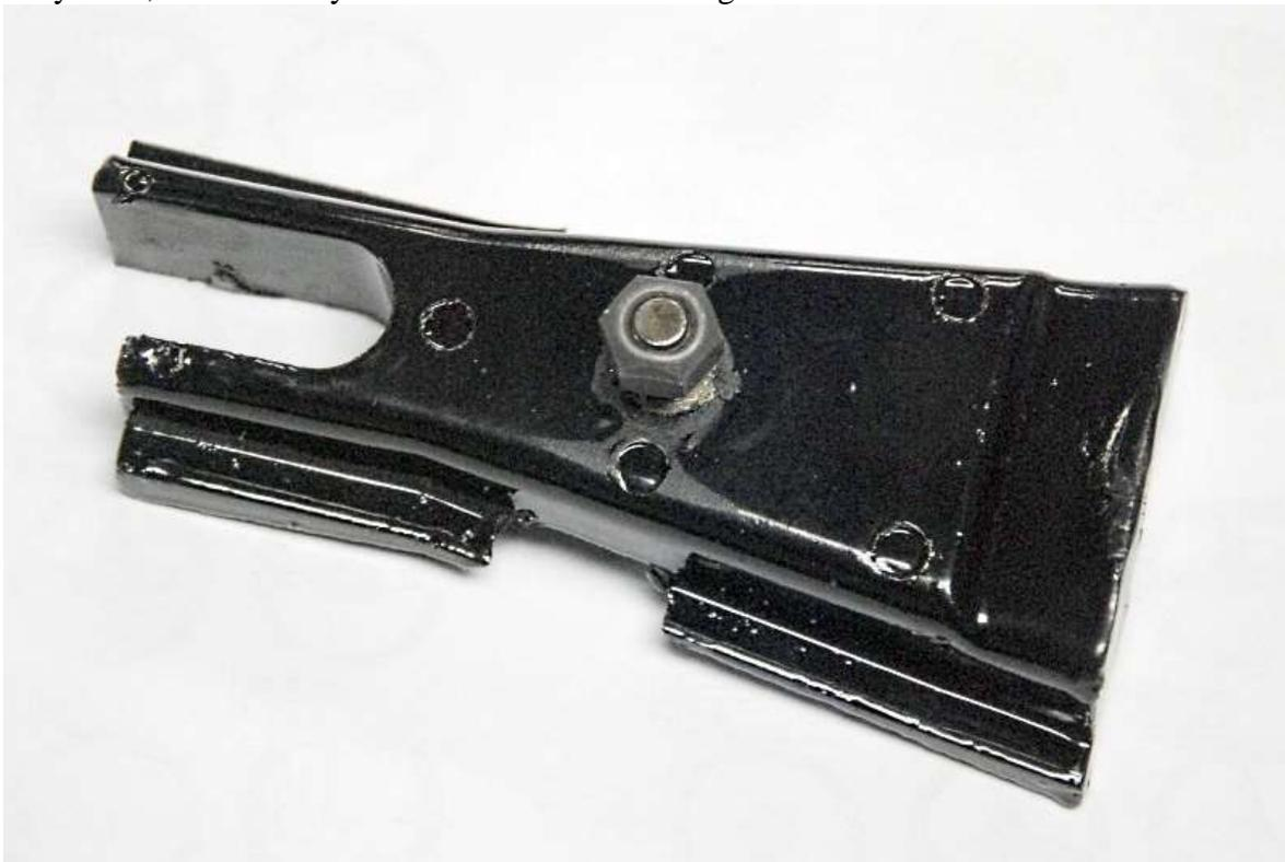
Remove the vibration damping weight from the clutch fork, it is not needed.
