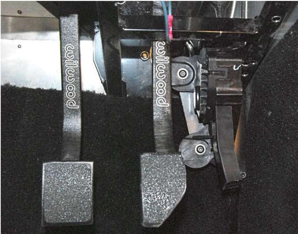
Attach the Coyote accelerator pedal to the new pedal mount.
