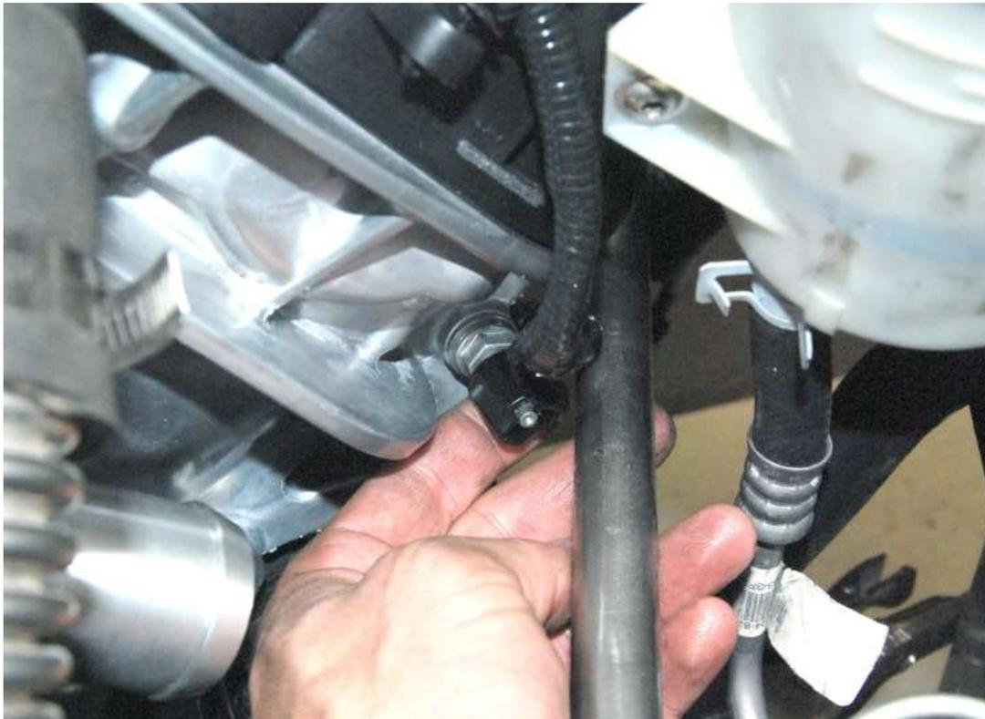
On the left side of the engine, remove the wiring harness holder from the stud on the front of the head; it will hit the steering shaft after install.
