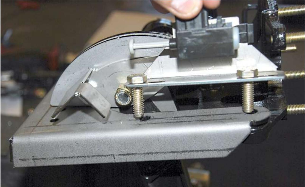
Insert the new  $\frac{5}{16}$ " x 1.25" bolts through the bottom travel switch mount then through the pedal box bracket and pedal box.
