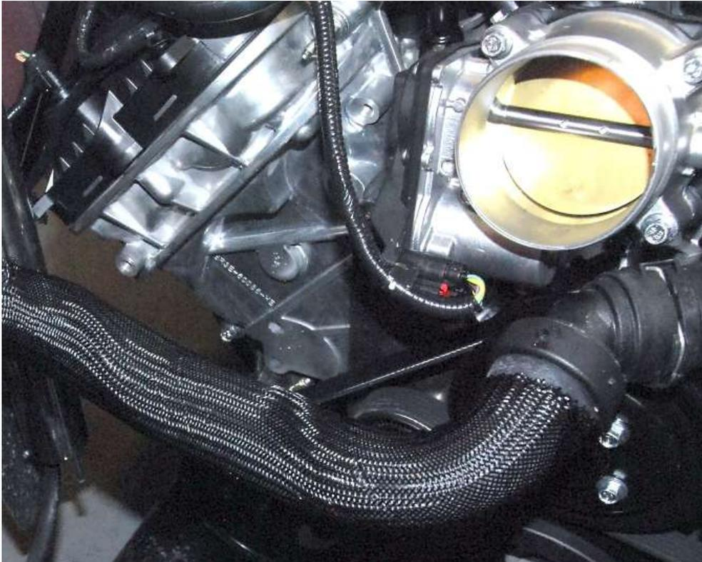
Push the Ford supplied hose onto the outlet under the throttle body.
