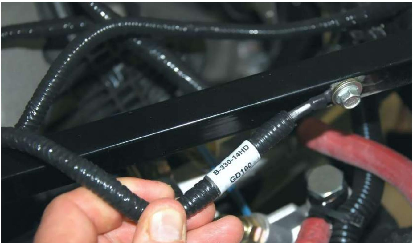
Ground the control pack harness to the frame, make sure to remove any frame coating to ensure a good ground.
