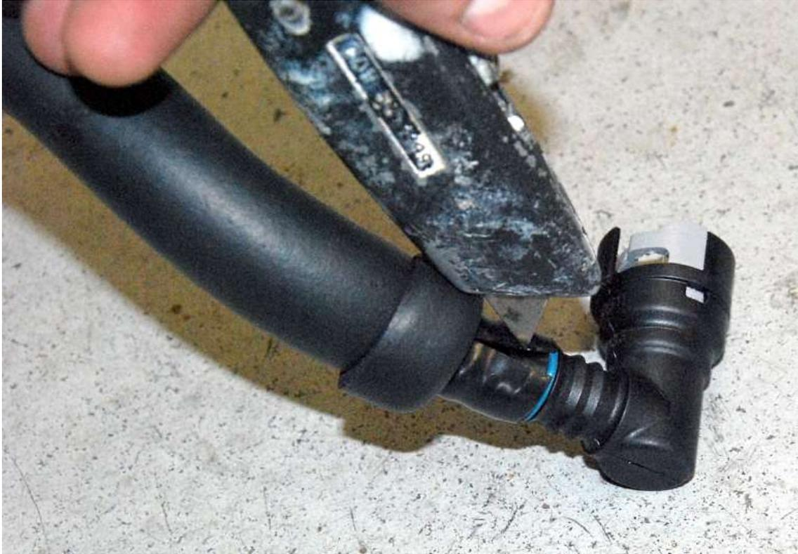
Carefully cut the 90° PCV fittings off the pcv lines without damaging the barbs.
