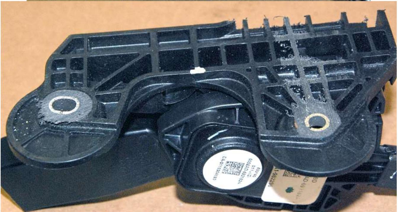
Align the mount holes of the pedal on the pedal mount and mark the pedal through the upper frame mount hole.
