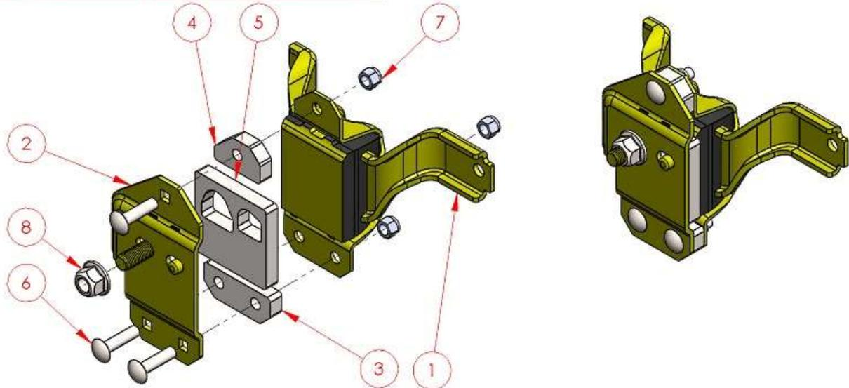
Reassemble the left engine mount using the 1/2" thick spacers, 3/8" x 1.50" carriage bolts and a 9/16" socket with ratchet. Reuse the 3/8" locknuts.
