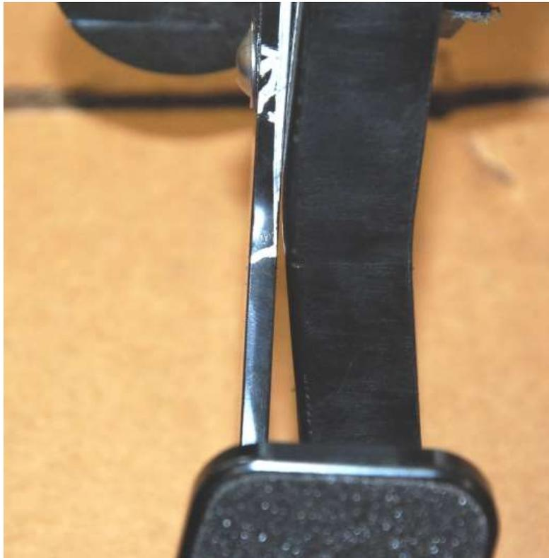
If your pedal location requires bolting below the bend in the plastic pedal, mark the location of the bend.
