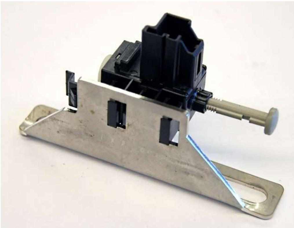
Attach the Bottom travel (gray plunger) clutch switch to the bottom travel switch mount as shown.
