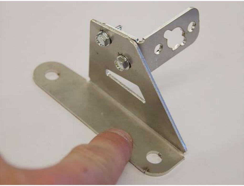
Hold the clutch pedal switch mount in a vise and screw the top travel switch mount to it using the #8 self-tapping screws and 1/4" nut driver. Leave the screws loose enough so that the switch mount can slide in the slots.
