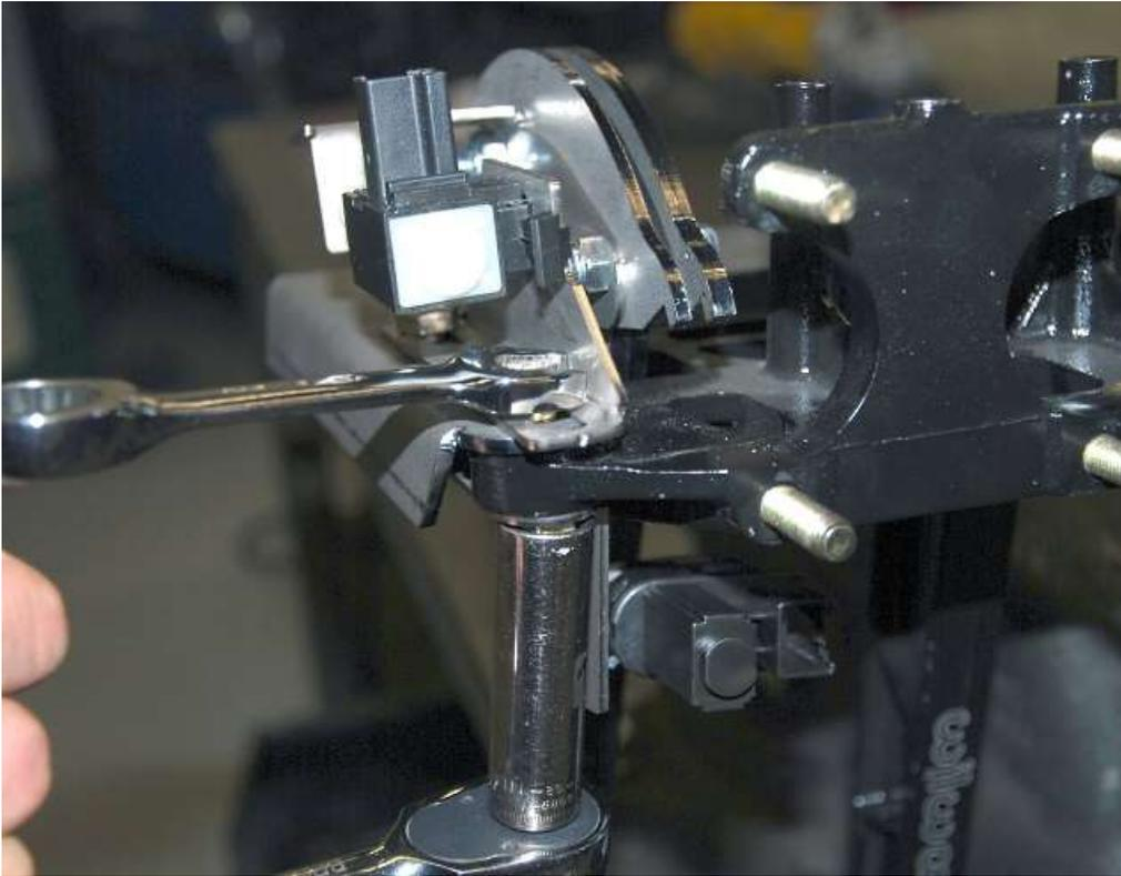
Snug the bolts up with a 1/2" wrench and socket so the bottom travel switch bracket can still move.
