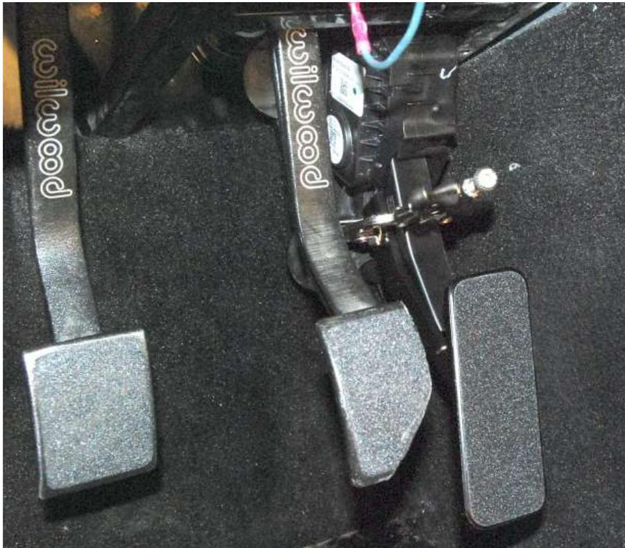
Clamp the FFR pedal to the Coyote pedal with a small clamp so that the accelerator pad is  $2\frac{1}{8}$ " back from the brake pedal.
