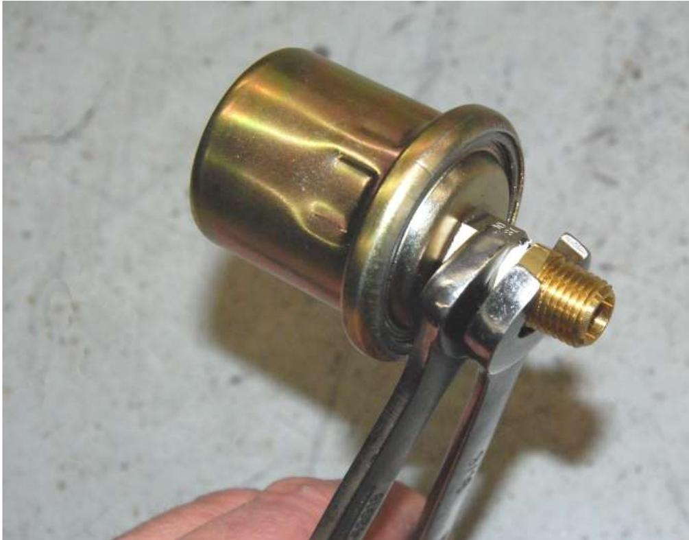
From the gauge box, screw on the 1/4" NPT adapter.
