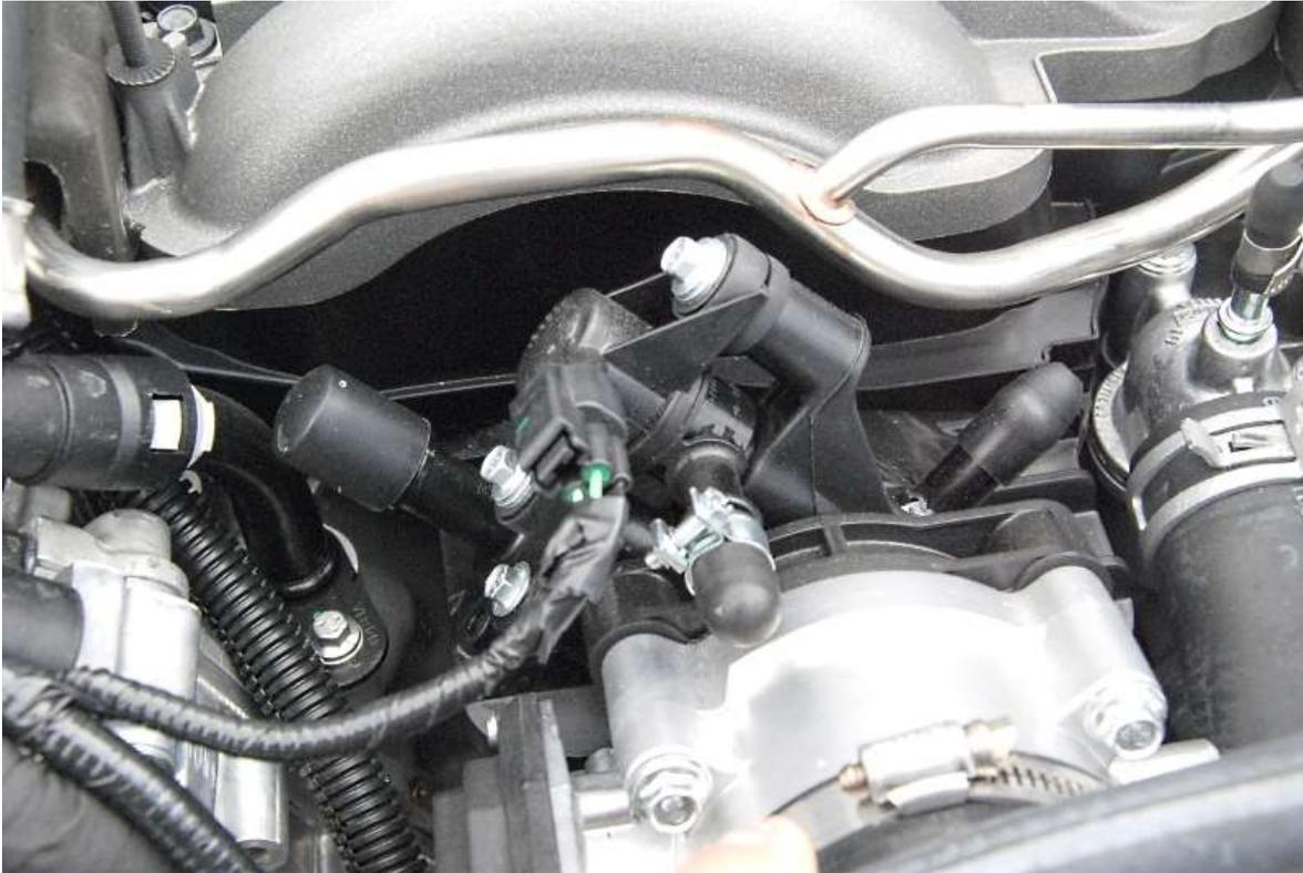
Block off the vacuum ports and fuel evaporator intake tube just behind the throttle body.
