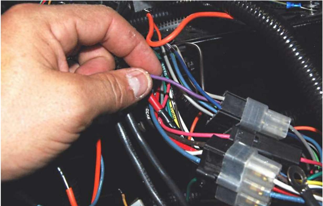
Find the purple tach wire in the sending unit plug and cut it so the engine harness can get connected to the purple wire.
