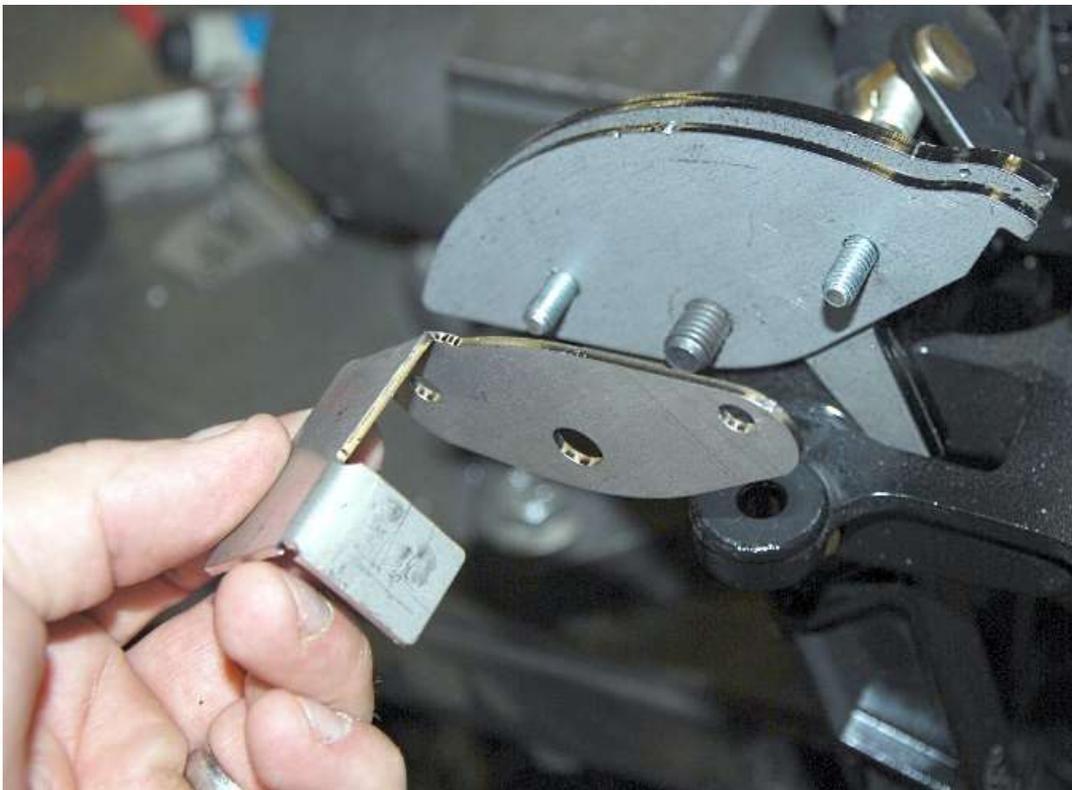
On the clutch pedal, remove the last  $\frac{1}{8}$ " clutch quadrant end plate and replace it with the stainless bottom switch clutch quadrant plate.
