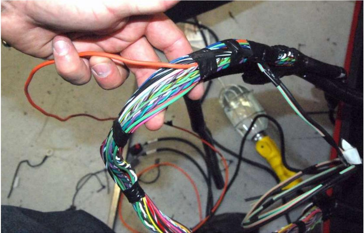
The orange wire in the engine harness needs to either be taped back along the harness or, a better way is to remove the engine harness wrap tape and pull the orange wire back to the last junction.
