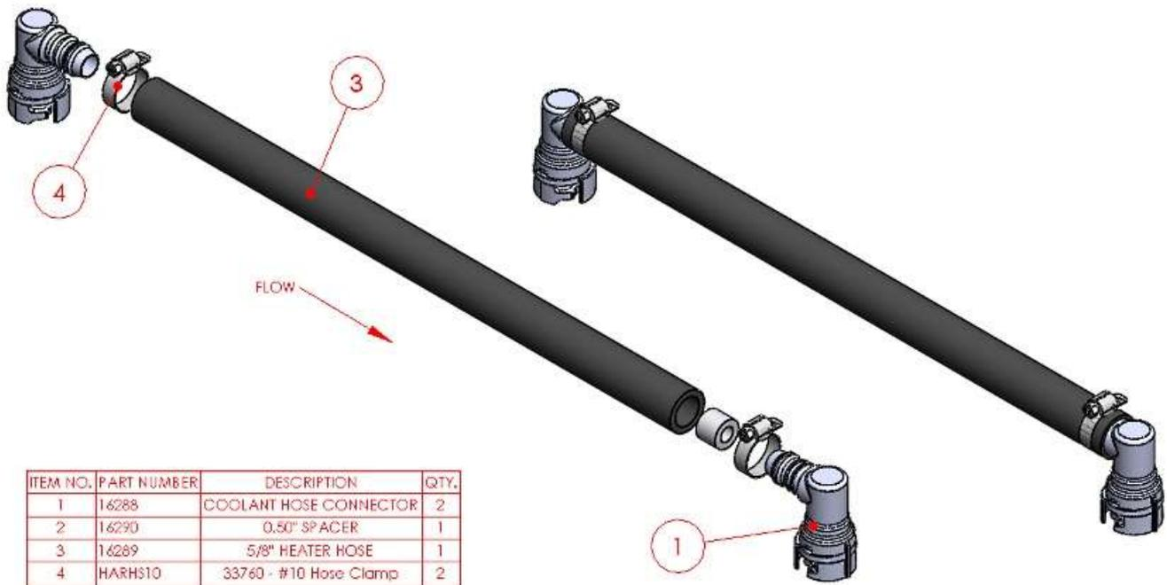
Assemble the right side of the heater bypass hose, insert the 0.50" aluminum spacer into the 5/8" heater hose followed by a hose clamp then push one of the 90° plastic coolant hose adapters.
