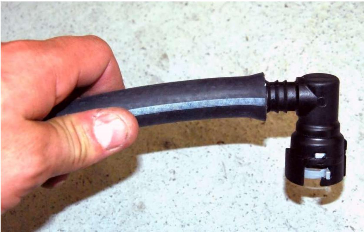
Spray some WD40 into the end of the hose and push the ½" heater hose onto one of the PCV fittings.
