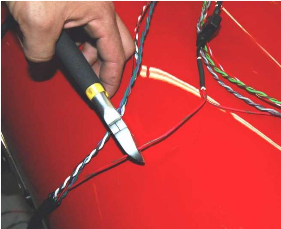
Cut the wire for the left side O<sub>2</sub> sensor a few inches from the junction.
