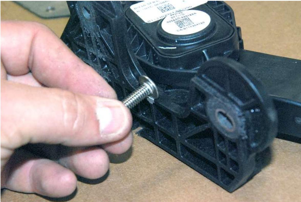
Hold up the mount screw to the pedal at the point marked.
