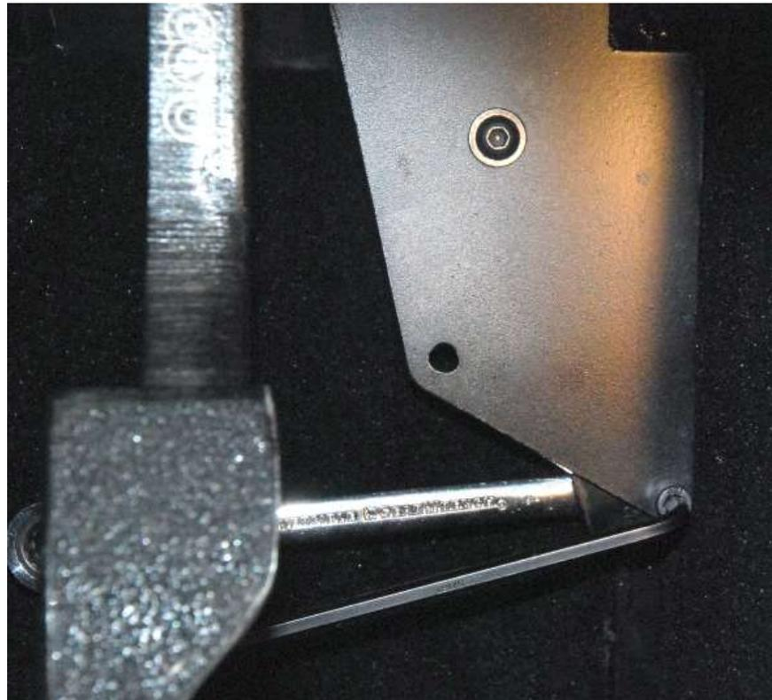
Attach the Accelerator pedal mount to the frame accelerator pedal mount using the 1/4" screws provided and the ones from the standard kit.
