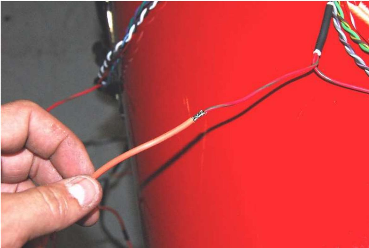
Use one of the extra wires pulled out of the harness or chassis harness to extend the wire. Start by soldering the wire to the end near the junction.
