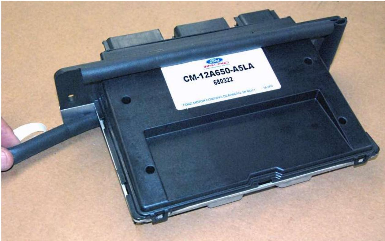
Use weatherstripping or silicone around the flange of the computer to seal the hole.
