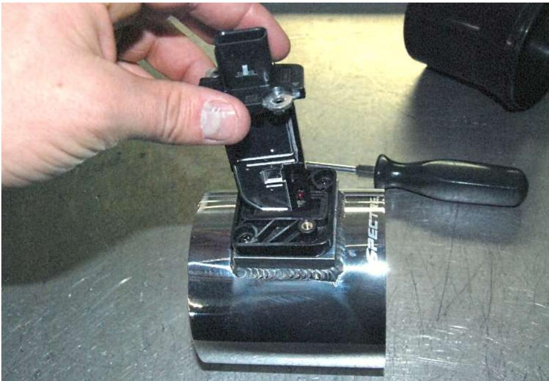
Install the sensor on the mount using the short screws so the flat side of the sensor will face the “Spectre” writing.
