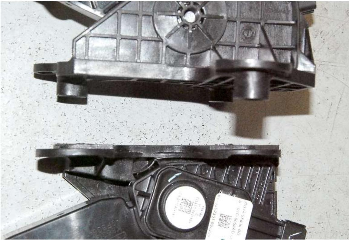
On the underside, cut the bottom mounts off with a hack saw so that the bottom is flat.
