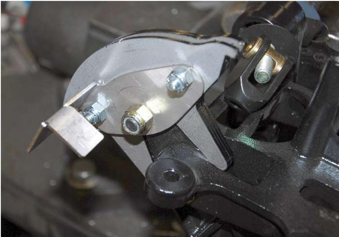
Tighten the locknuts.
