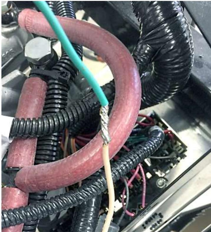
Solder and tape the tan wire and Fuel pump relay out (green) wires together.
