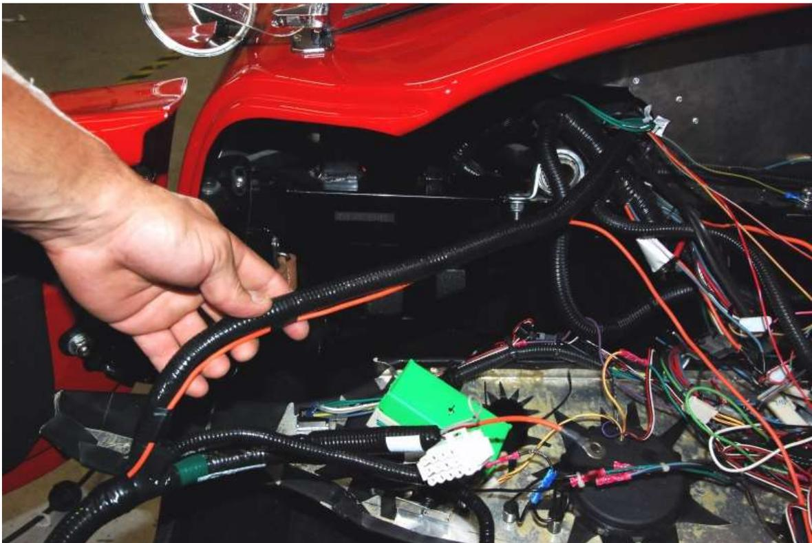
Run the orange wire along the outside of the harness going to the accelerator pedal.
