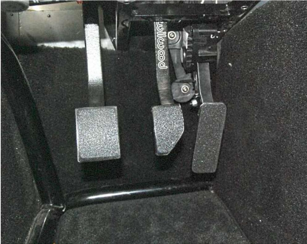
Mount the pedal to the new pedal mount in the footbox.
