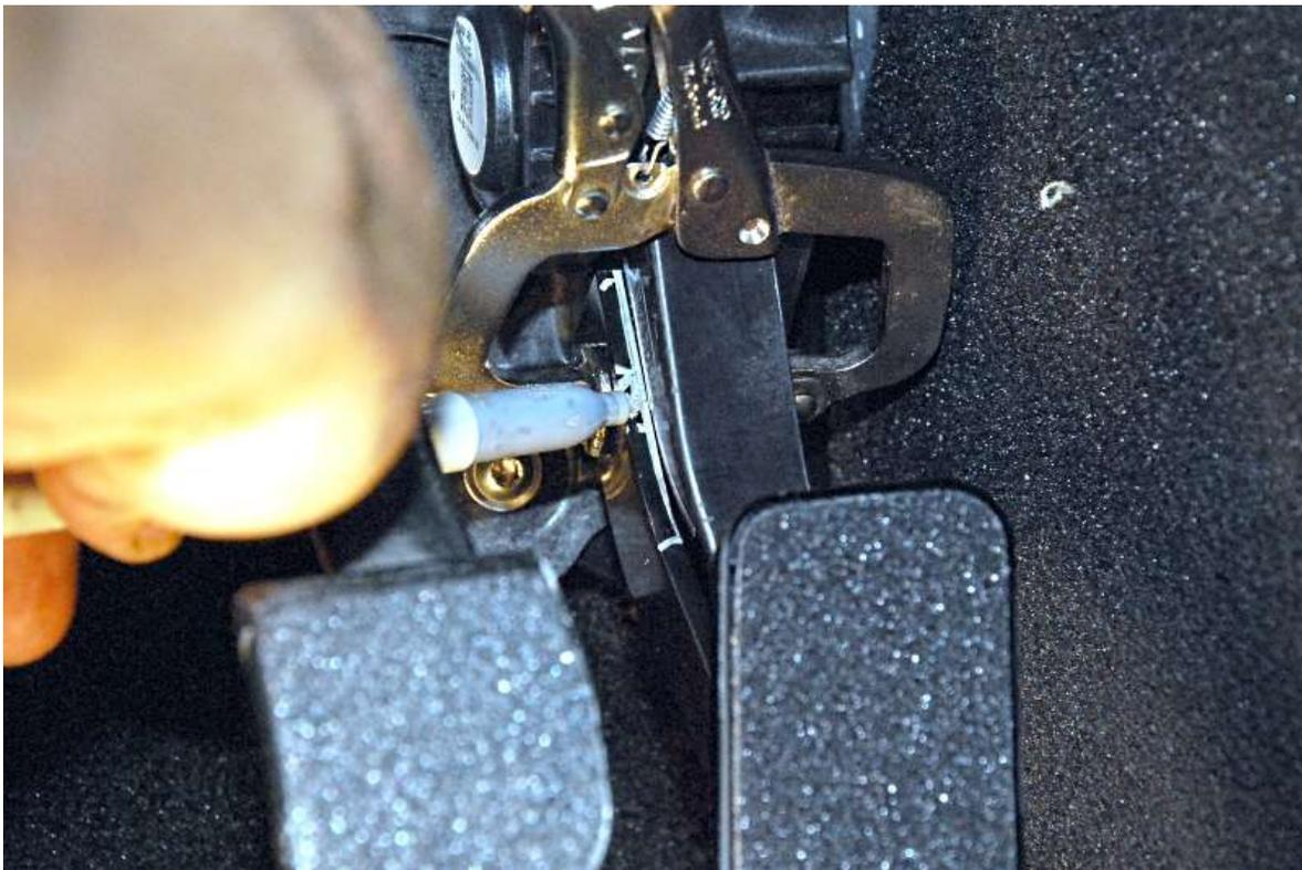
Sit in the car and push the brake pedal down as if you were stopping the car. You should be able to push the pedal down without hitting the gas pedal but be able to rock your foot (heel/toe) onto the gas pedal.
