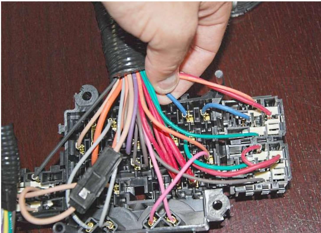
Locate the blue wire going into the harness on the opposite side of the cooling fan fuse from the blue wire coming from the fan relay.
