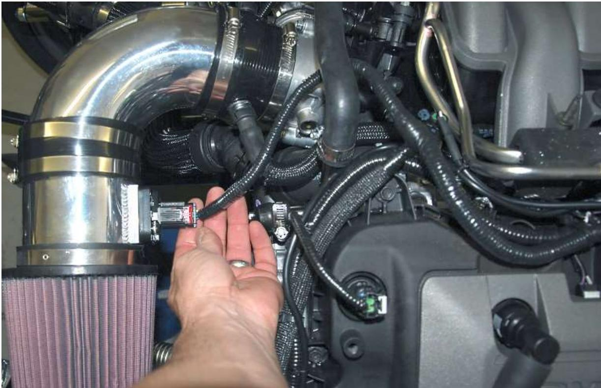
Plug the mass air meter connector into the mass air meter.
