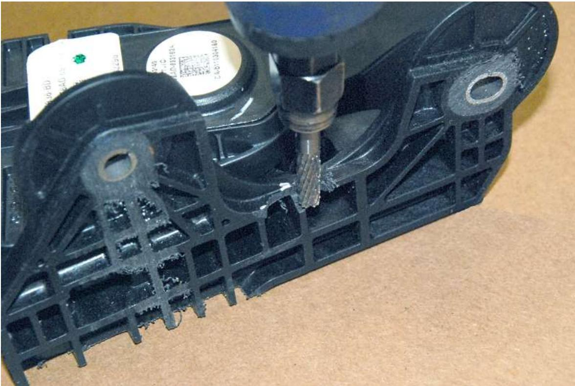
Use a grinder, hack saw or drill bit to remove material on the pedal for screw clearance.
