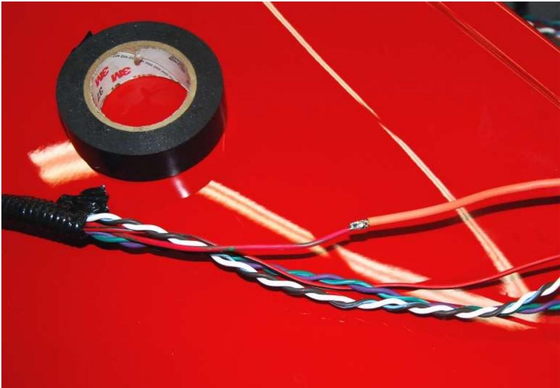
Solder the other end of the extension wire to the O<sub>2</sub> sensor wire.
