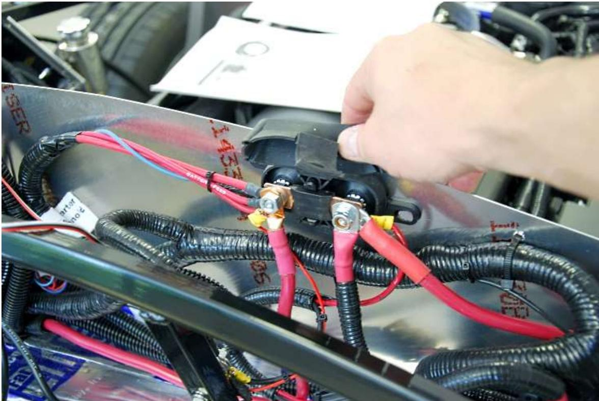
Locate and mark the inline fuse just to the left of the dash support post on the firewall or on the 2" tube.
