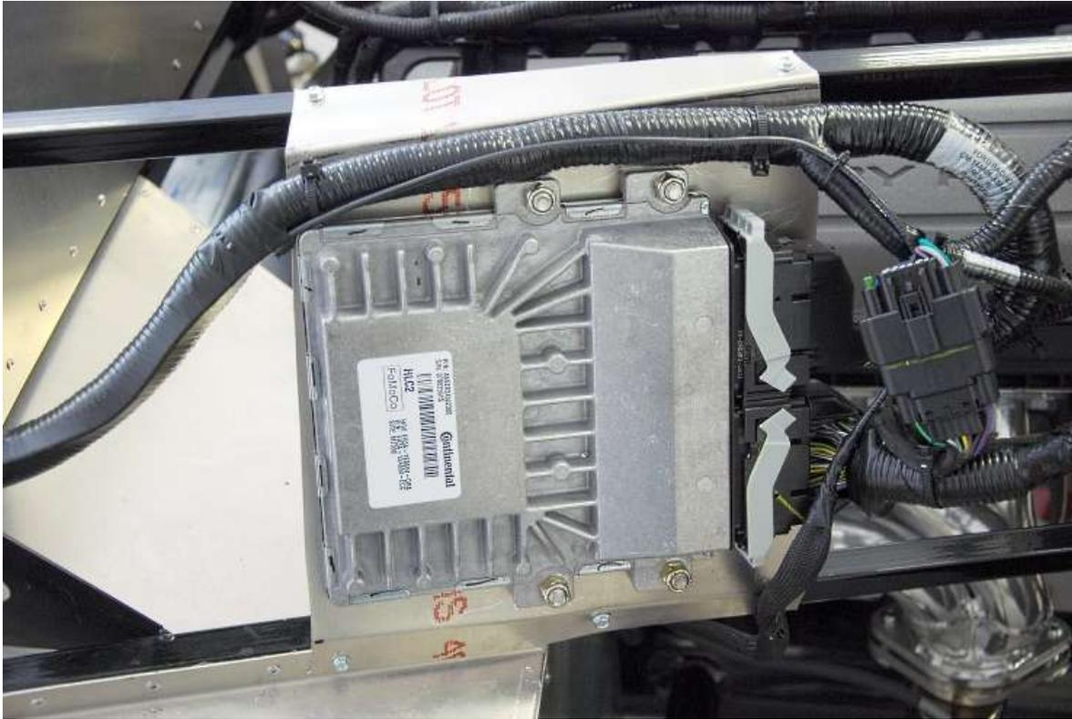
Locate the aluminum computer bracket so that it spans between the upper and lower  $\frac{3}{4}$ " tubes that go down to the front suspension on the right side of the chassis and the rear bottom computer hole lines up with the front of the right footbox.
