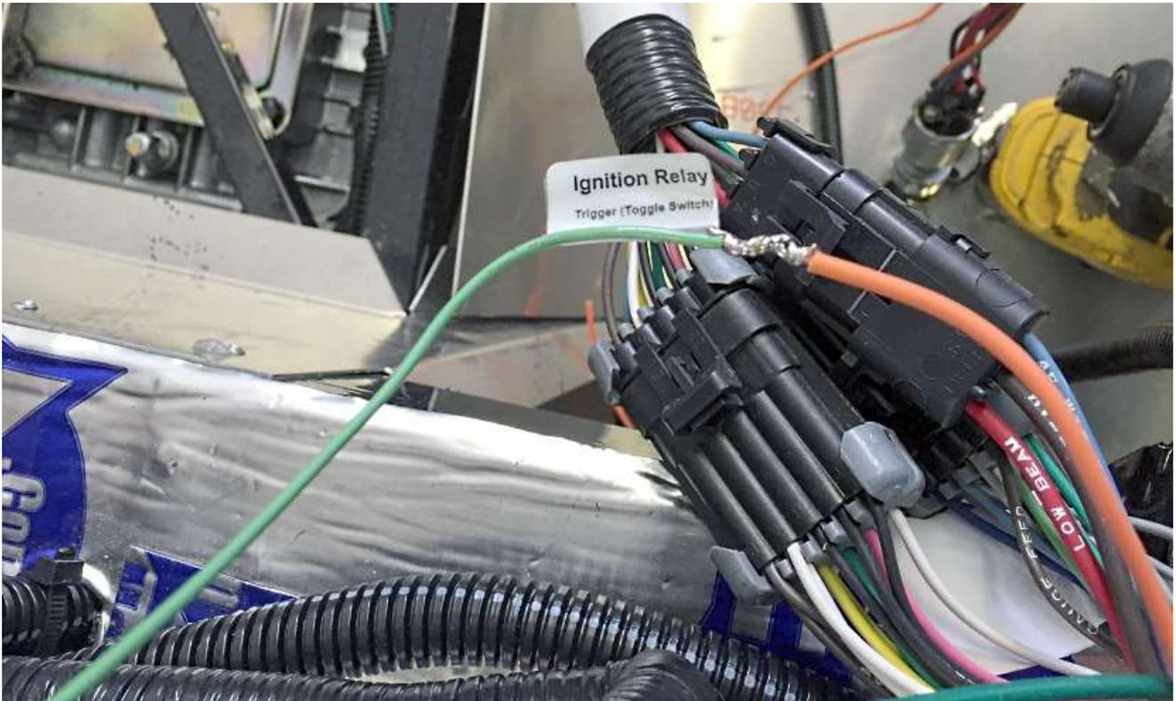
On the 16 way connector, connect the 12v Ignition relay trigger wire (light green) wire to the orange coil wire.
