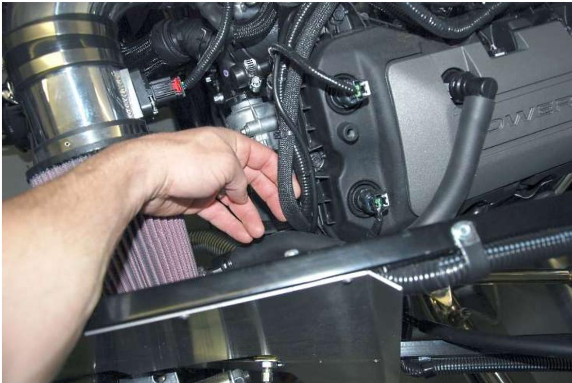
Run the alternator plug down to the alternator.
