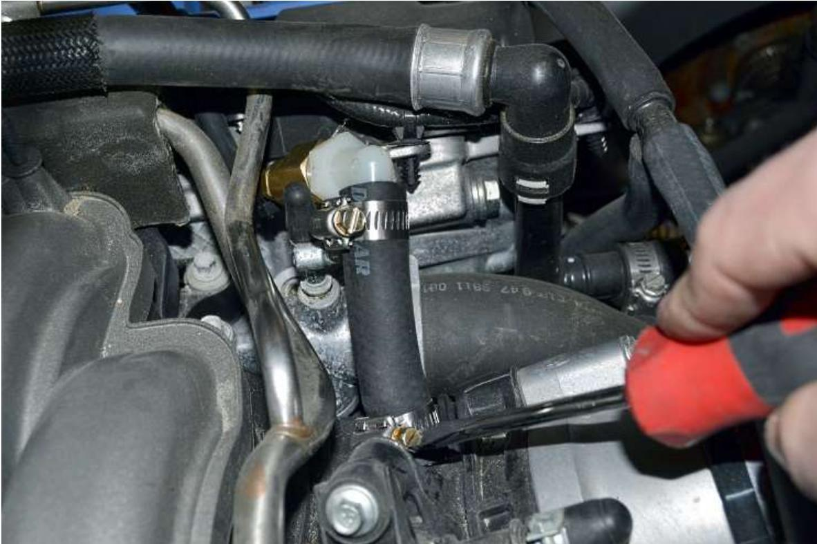
Push the ½" hose onto the vacuum port on the right side of the throttle body so the small end points towards the firewall and tighten the hose clamp.
