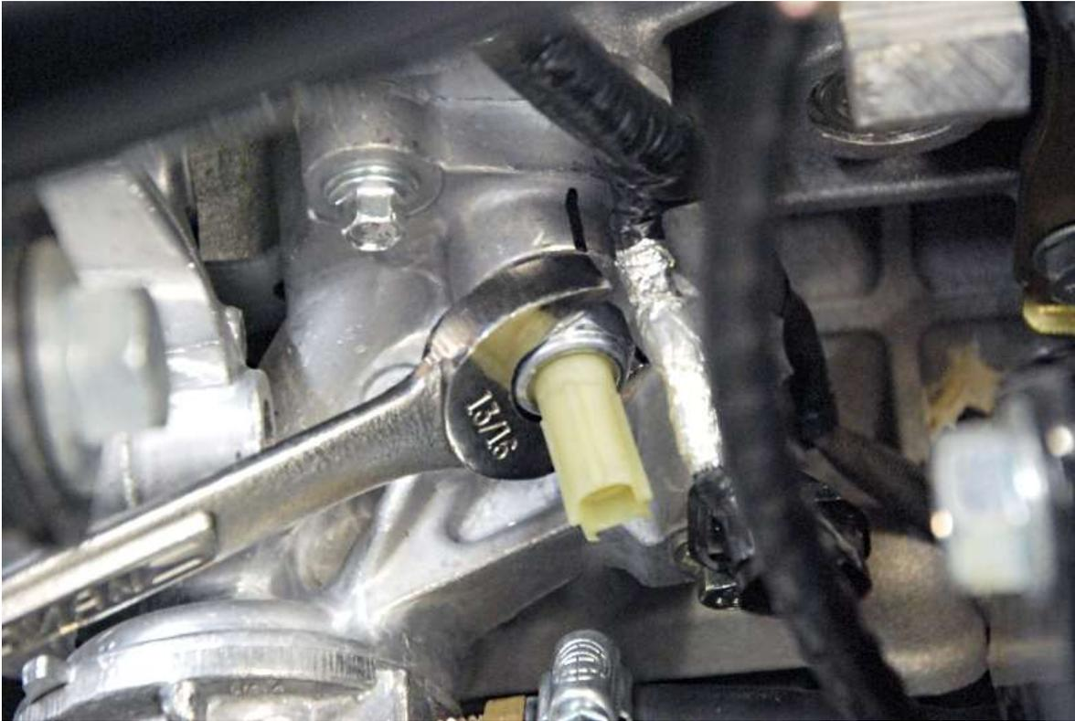
Remove the stock oil pressure gauge sender from the block located behind the alternator. This Sending unit will not be used again.
