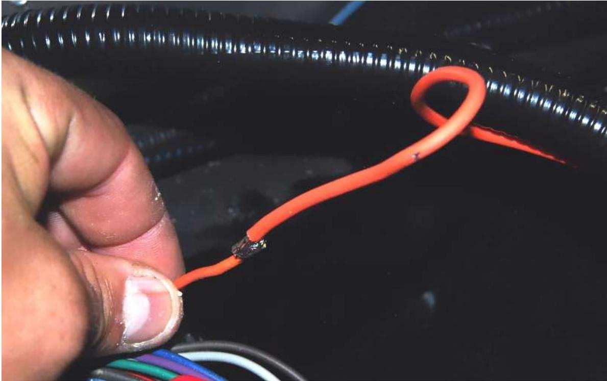
Solder or butt connect the orange fan wires together.
