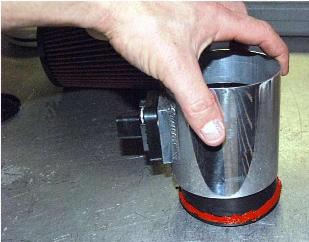
Slide the Mass Air Meter tube flat sensor side first (Spectre writing) down onto the plastic reducer.
