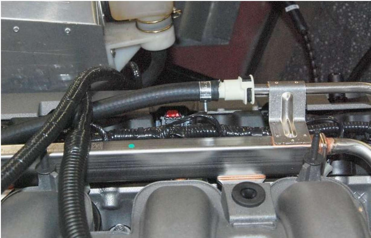
Push the white connector onto the fuel rail.
