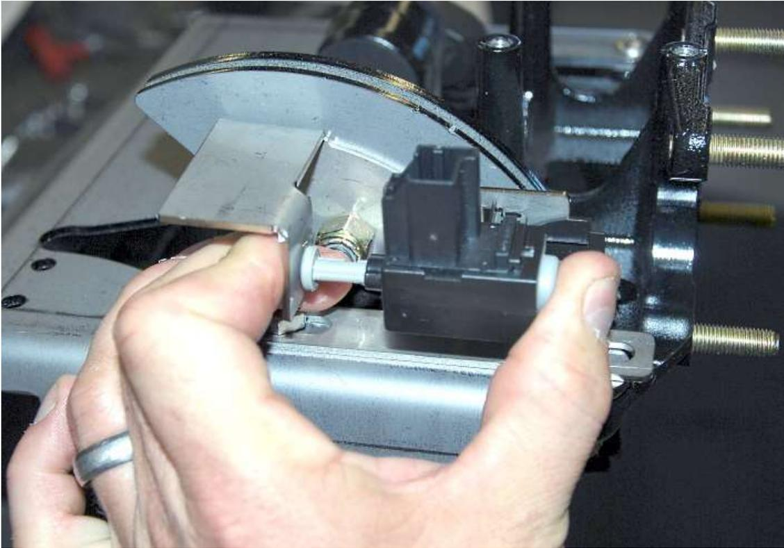
Have someone push the clutch pedal all the way in then slide the bottom travel switch mount so that the bottom travel switch is pressed in all the way against the quadrant plate. Hold the switch mount so that it does not move and let the clutch out then tighten the pedalbox mount screws with a ½” wrench and socket making sure the switch mount does not move.
