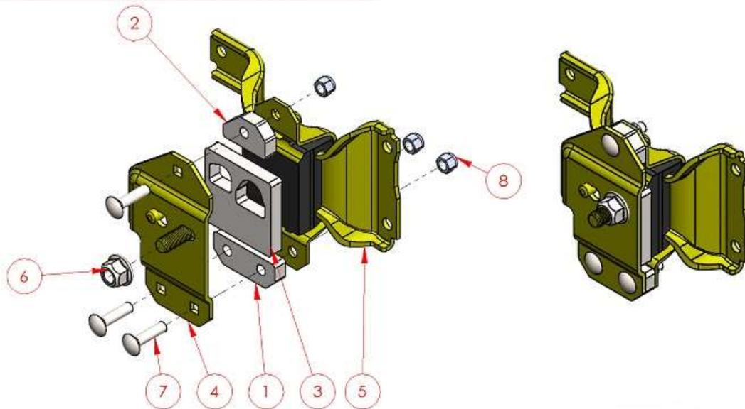
Reassemble the left engine mount using the 1/2" thick spacers, 3/8" x 1.50" carriage bolts and a 9/16" socket with ratchet. Reuse the 3/8" locknuts.
