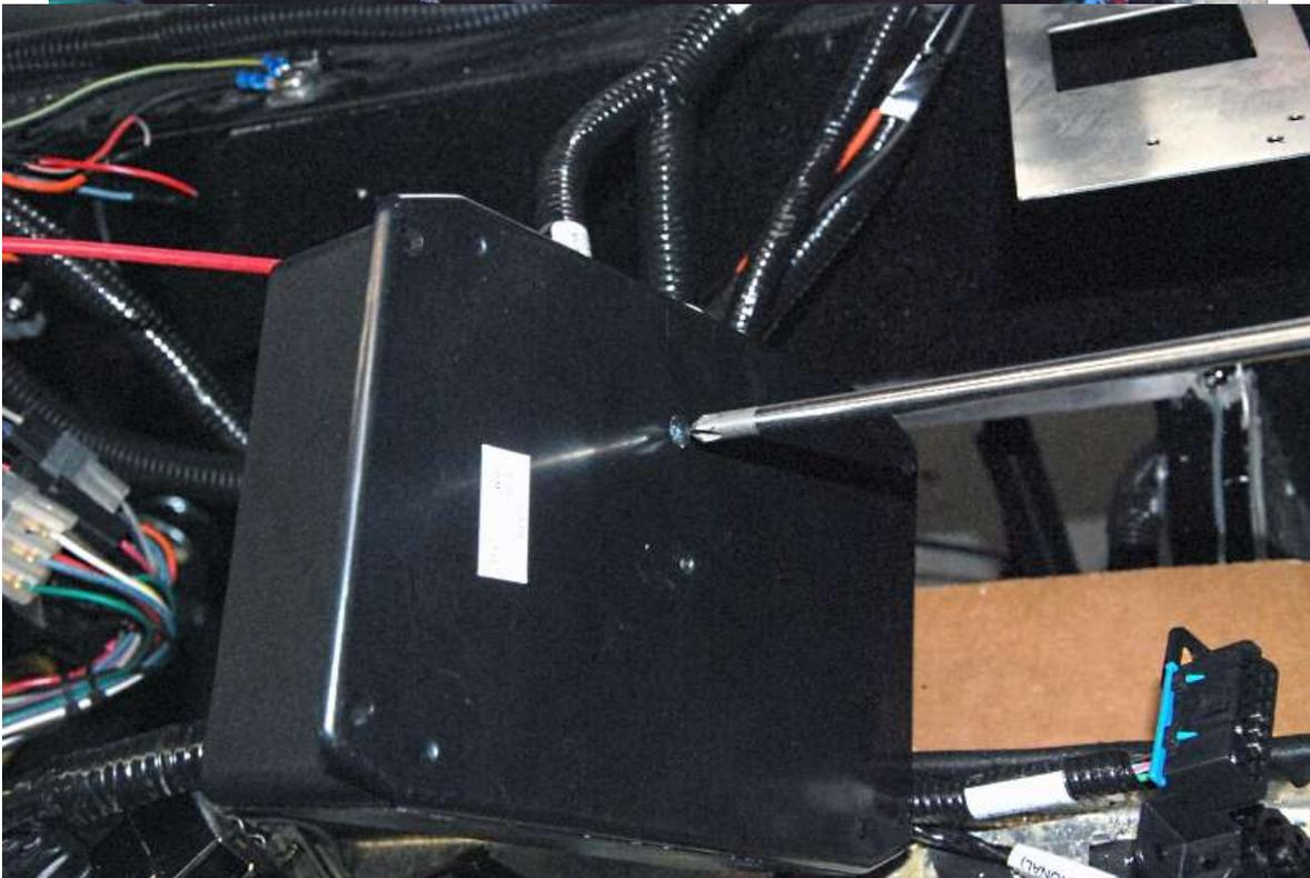
Connect the green power plug inside the box. It gets attached using a large Philips head screwdriver through the bottom of the box.
