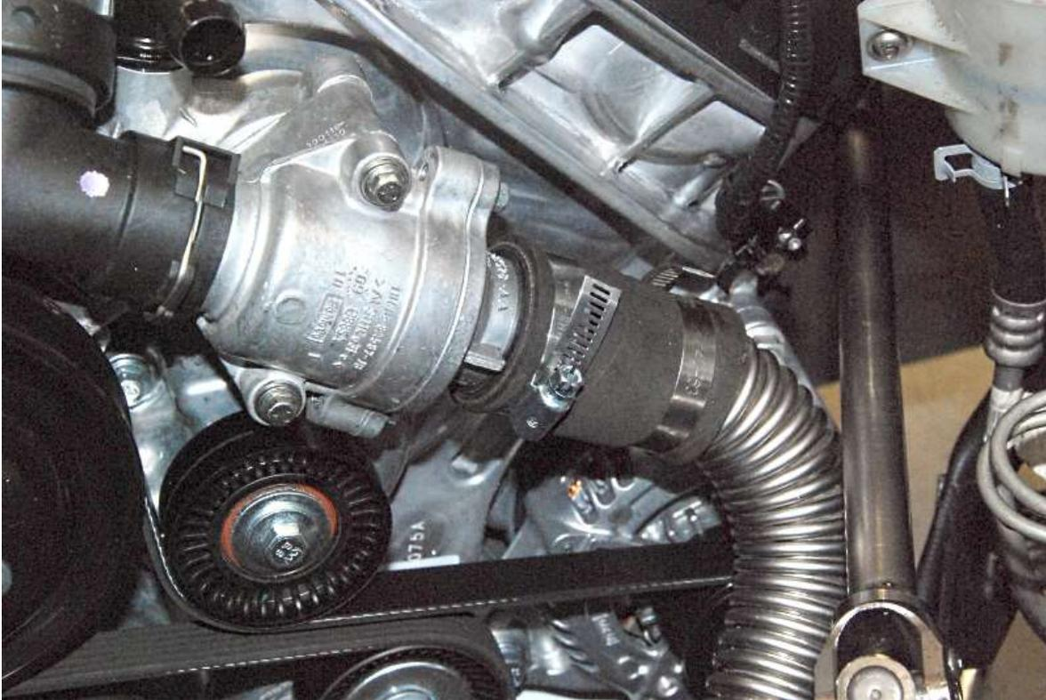
Push the correct size adapters onto to the thermostat housing with a length of the stainless hose.
