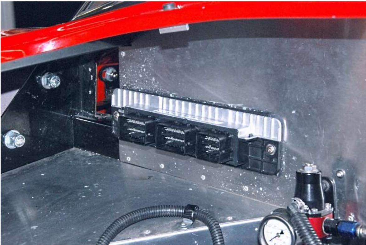
Mount the computer to the car using the #10 x 1" screws in the wiring harness mounting hardware or nutserts if you have them.
