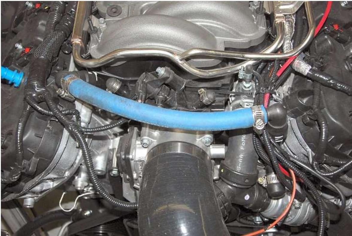
Put a hose clamp on the hose, push it onto the coolant adapter and tighten the hose clamp.
