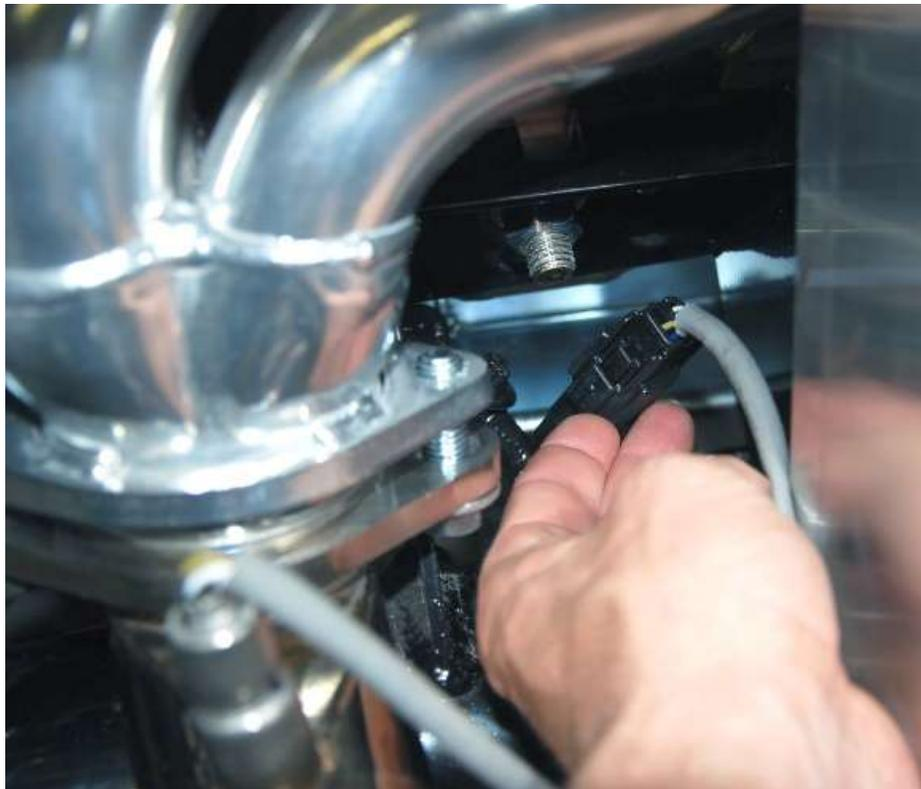
Connect the left O<sub>2</sub> sensor to the connector down near the engine mount
