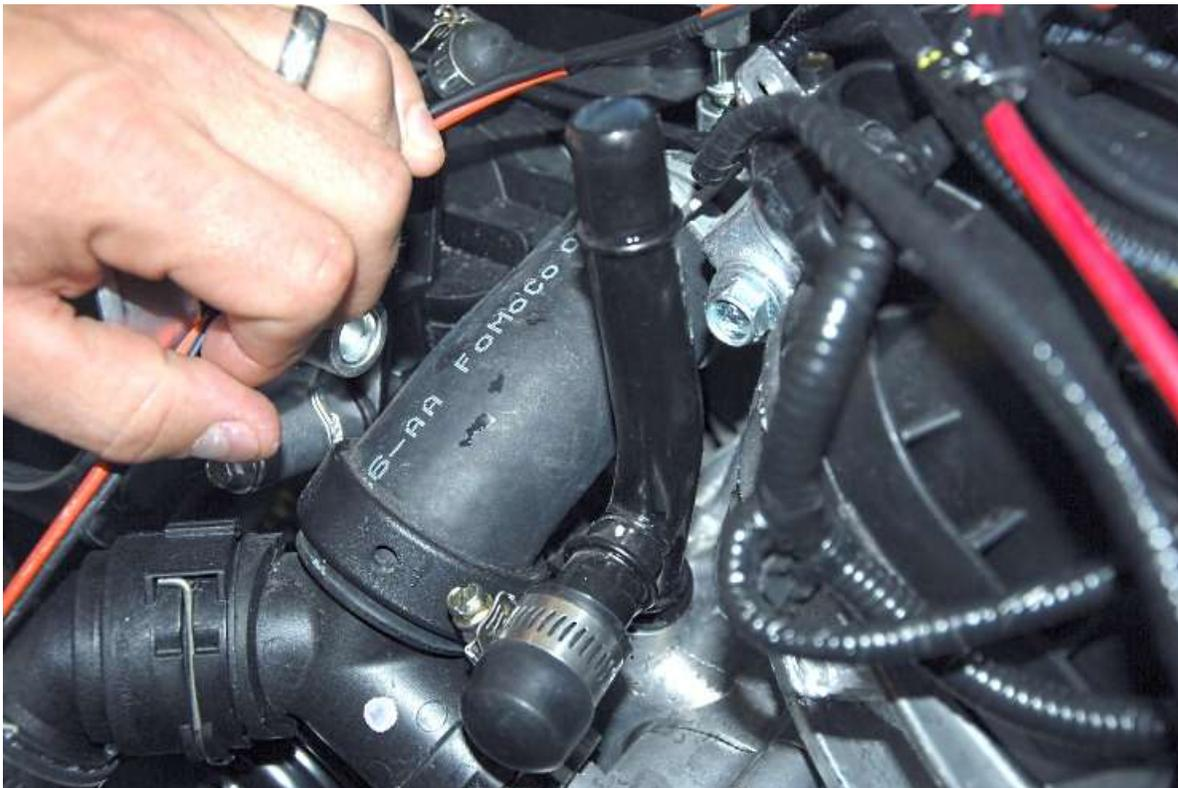
Push the bypass caps onto the lower tube to the left of the throttle body and hose clamp it.
