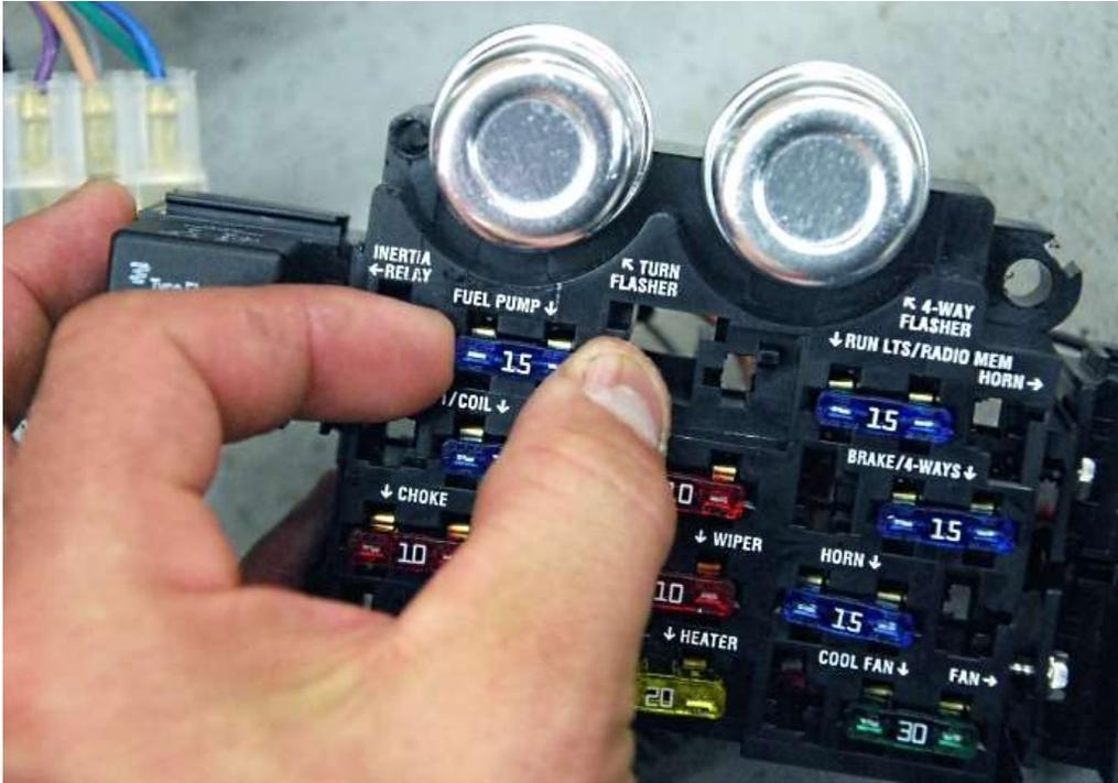
Remove the fuse from the fuel pump circuit on the chassis harness fuse panel.
