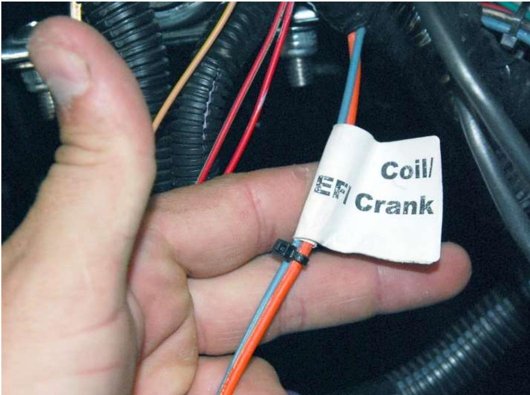
Locate the EFI/crank and coil wires in the chassis harness.
