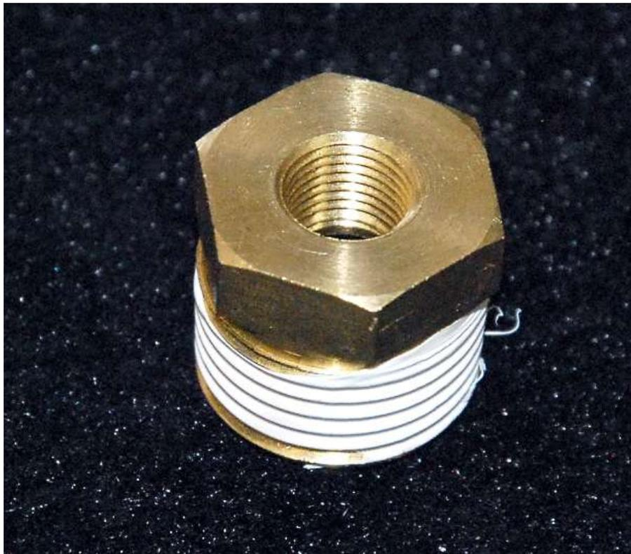
Use Teflon tape on the 1/8" NPT to 1/2" NPT adapter included with the gauge.
