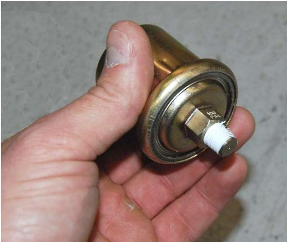
Use Teflon tape and install the oil pressure gauge sender.
