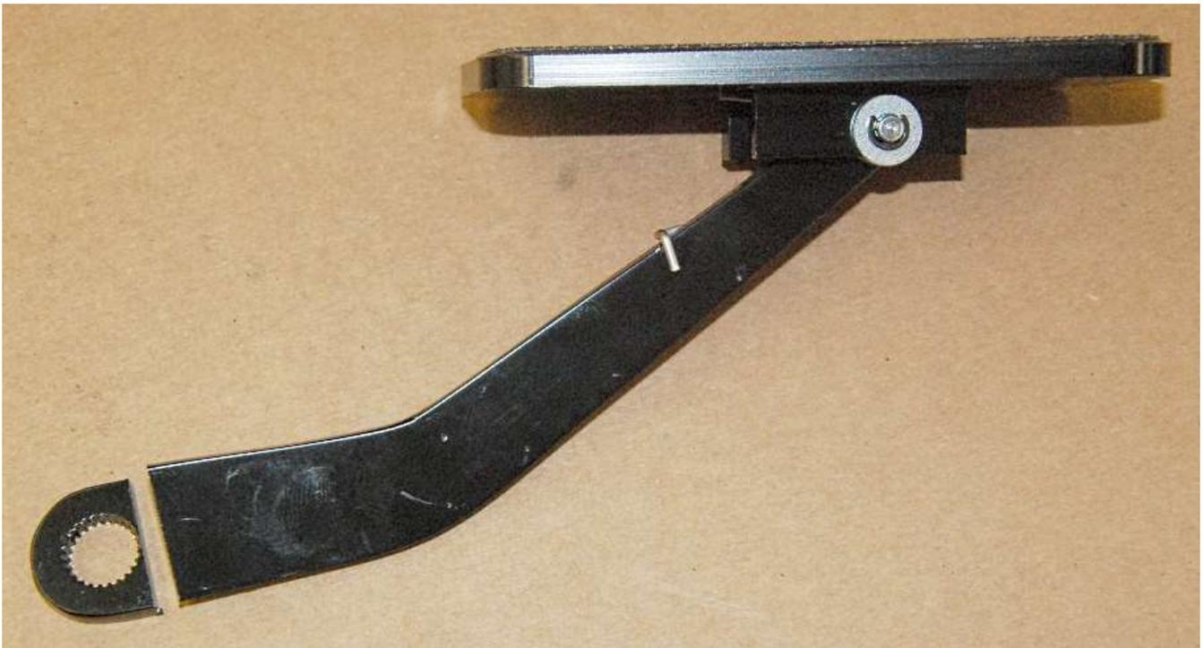
Cut the FFR accelerator pedal at the bottom of the existing mount hole using a hack saw.
