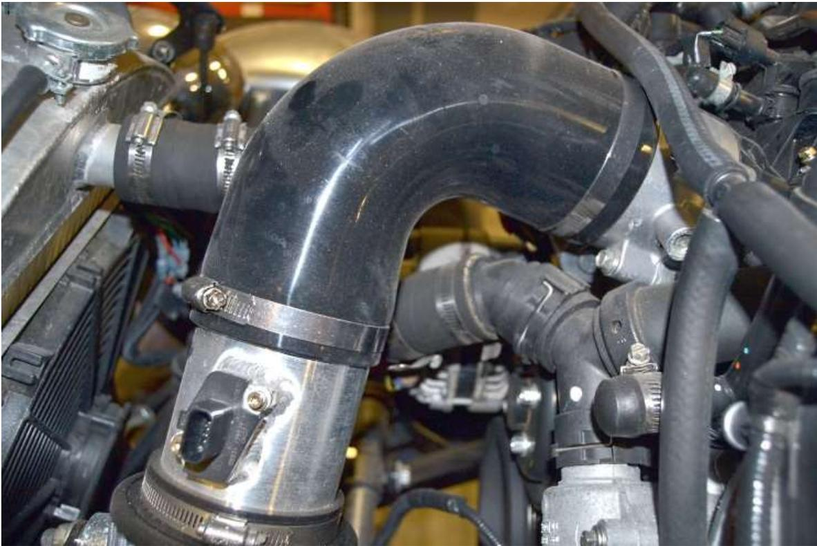
Test fit the 90° Silicone hose on the mass air meter and the throttle body, if necessary cut the legs of the hose for radiator and frame clearance.
