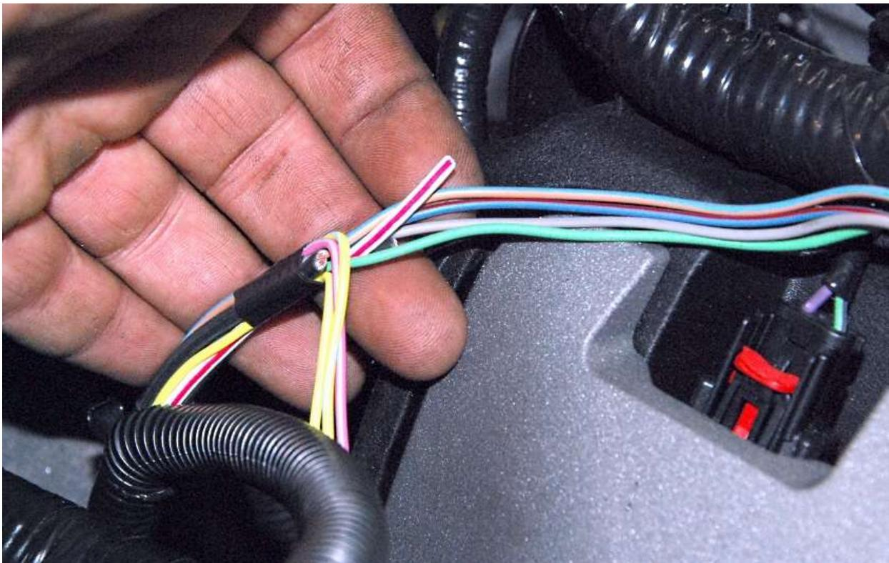
Cut the white/red Intercooler pump wire as far back in the harness as you can. It is not needed or used.
