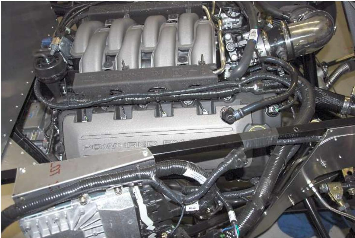
Route the BB harness (harness leg with the alternator and Mass air plugs at the end) to the front of the engine and run it across to the engine with the engine harness. Loosely zip tie the harnesses together.
