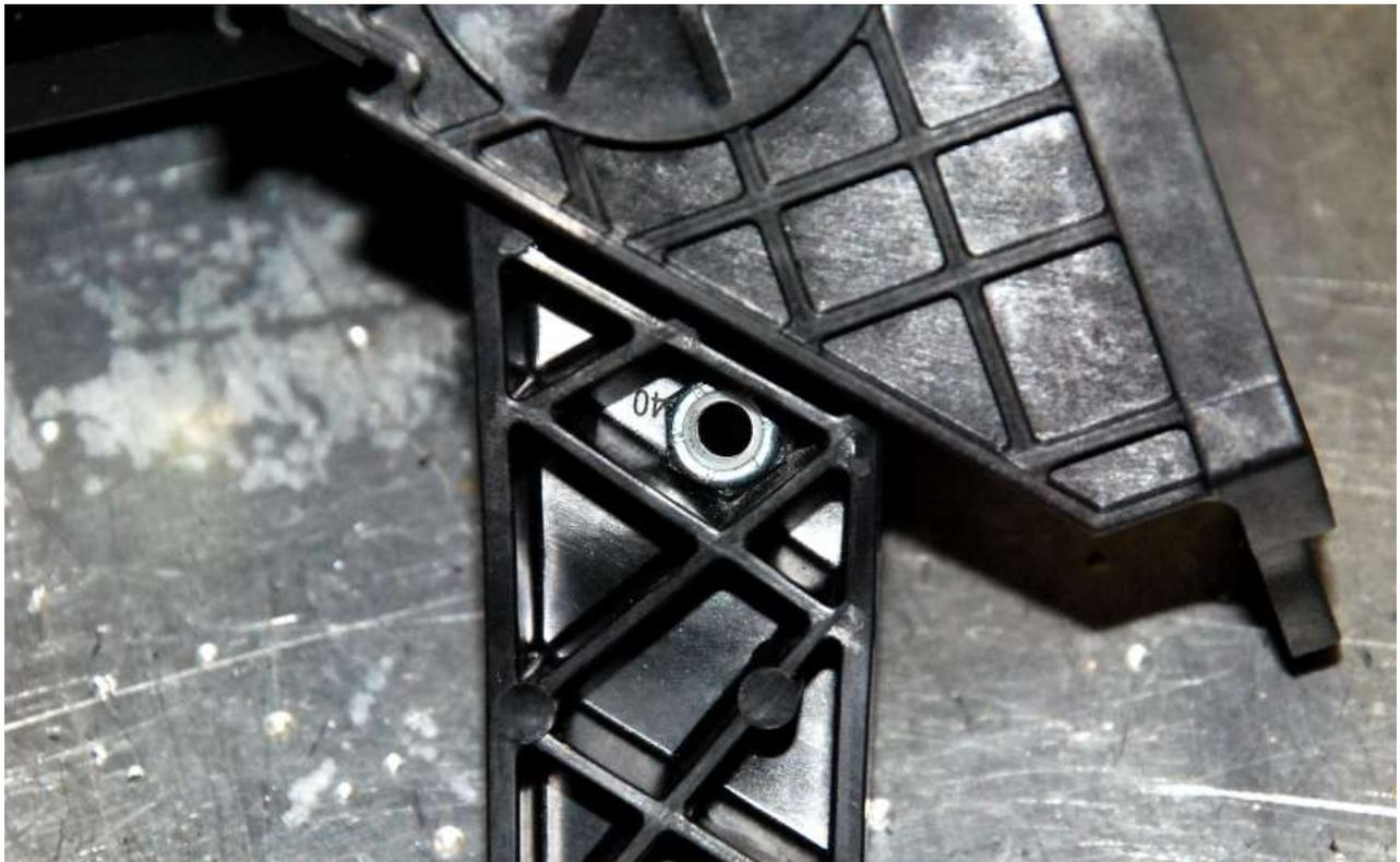
On the backside of the pedal insert one of the 1/4" locknuts into one of the recesses so that the bolts will be as far apart as possible and still go through both the FFR pedal and the Coyote pedal.
