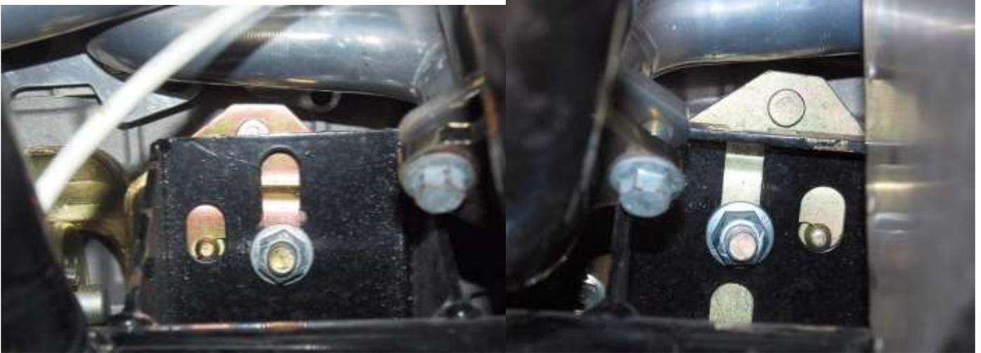
The engine will sit low in the engine mounts.
