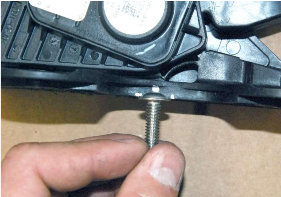
Mark the pedal where the screw starts, stops and the height of the screw.
