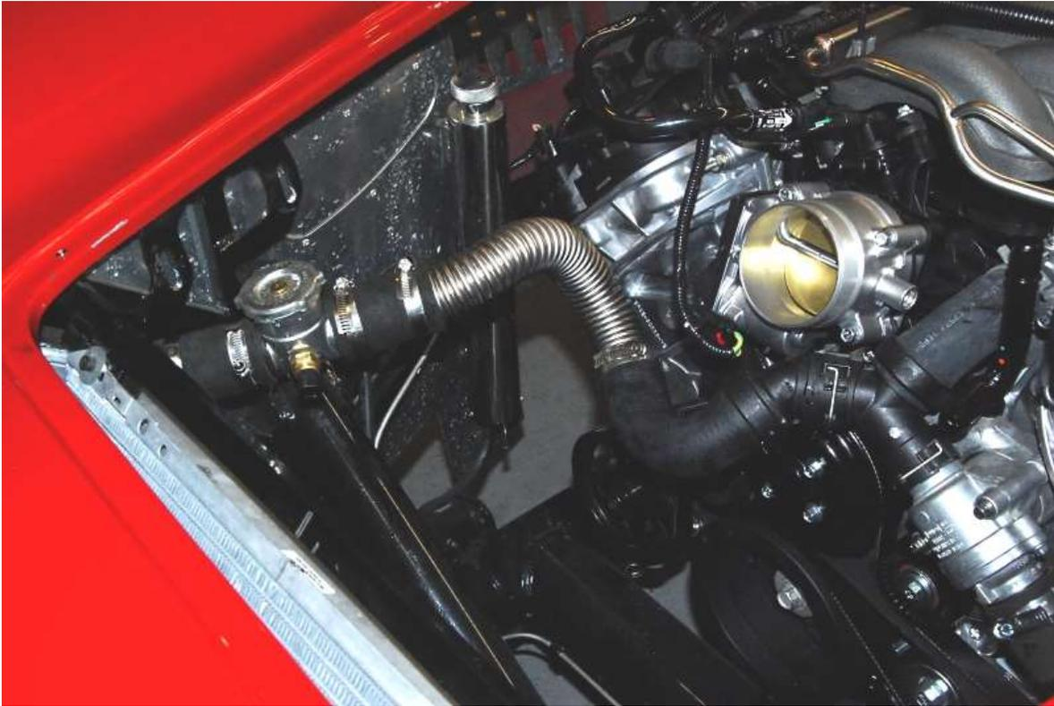
Push the stainless hose into the end of the rubber hose and run the hose to the right side upper radiator inlet.
