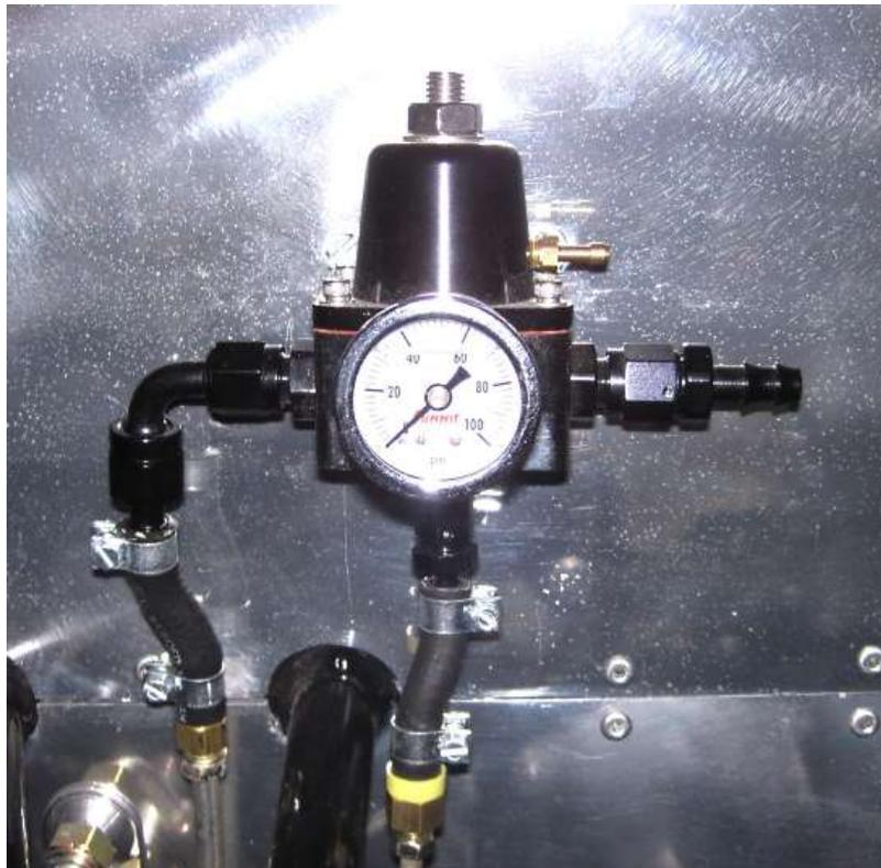
Mount a fuel pressure regulator to the firewall and connect the appropriate fittings, the return is on the bottom.
