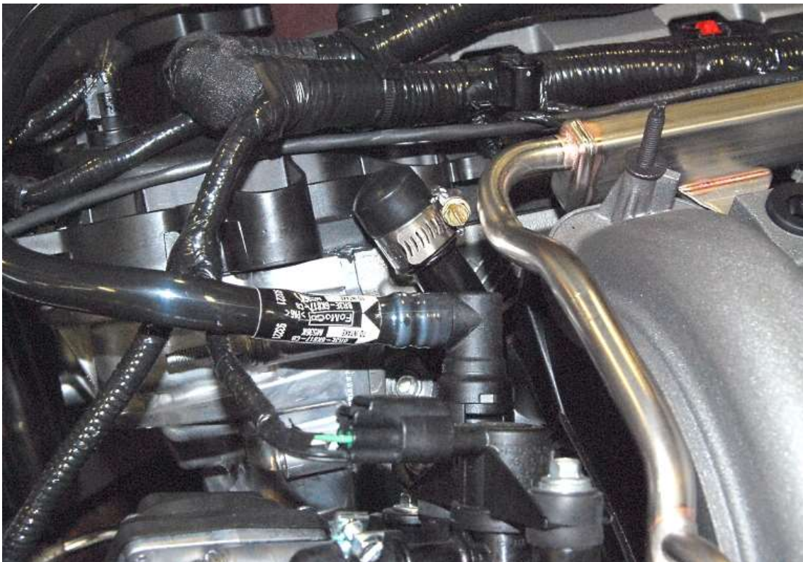
Cap and hose clamp the 3/4" coolant.
