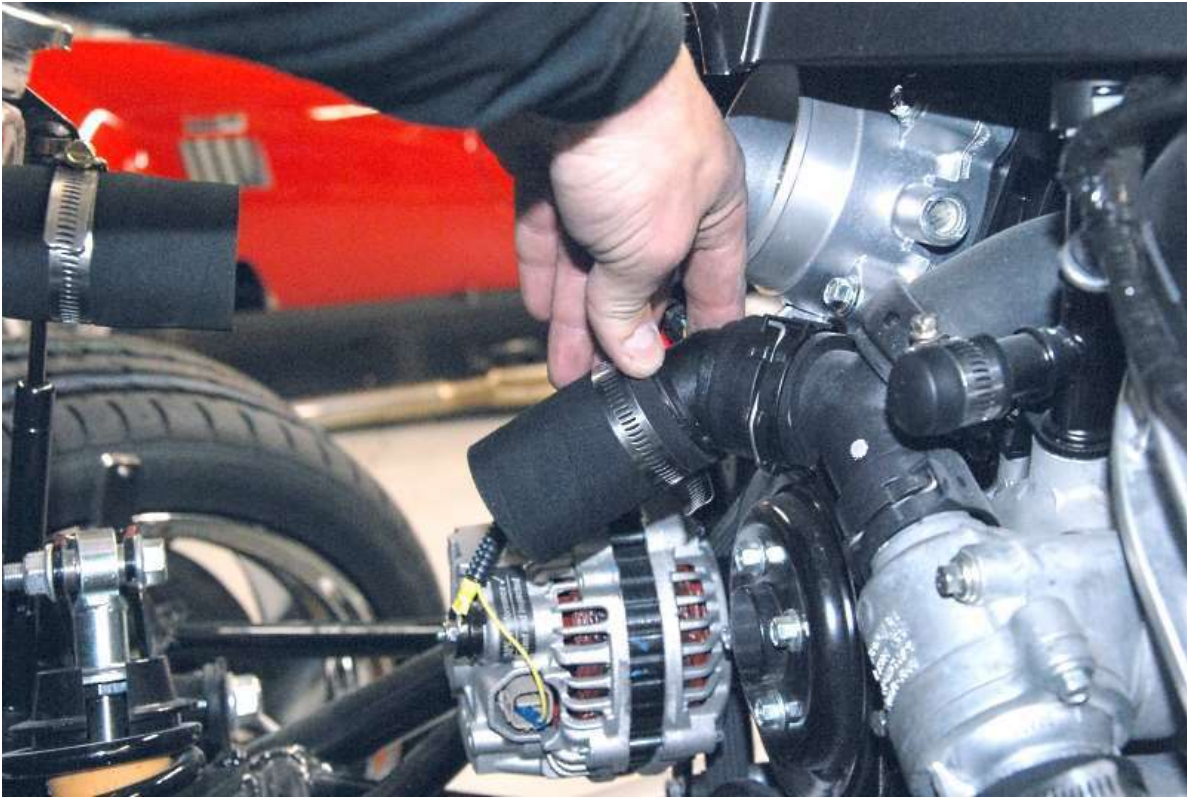
Push the adapter onto the engine.
