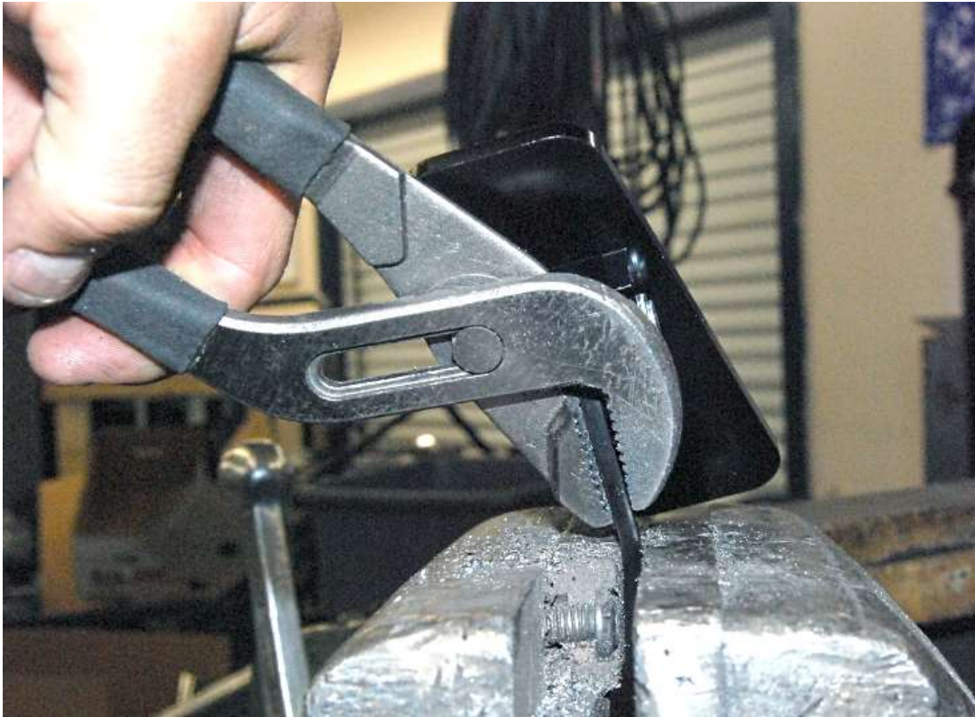
Use a pair of pliers and a vise to slightly bend the metal pedal to match the plastic.
