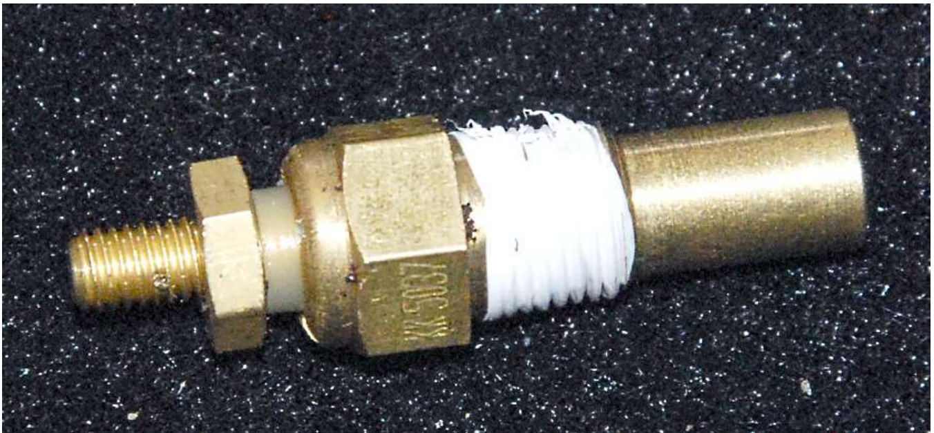
Put Teflon tape on the sending unit.
