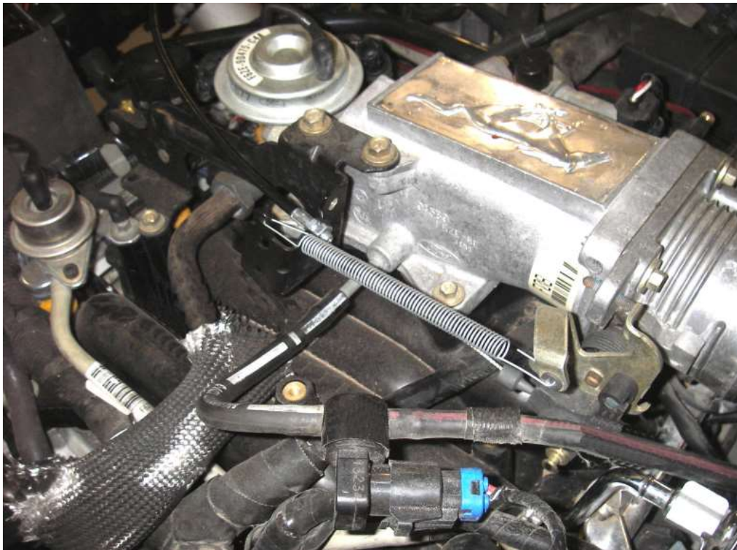
Accelerator cable mounted on 1996 2 valve Intake.
