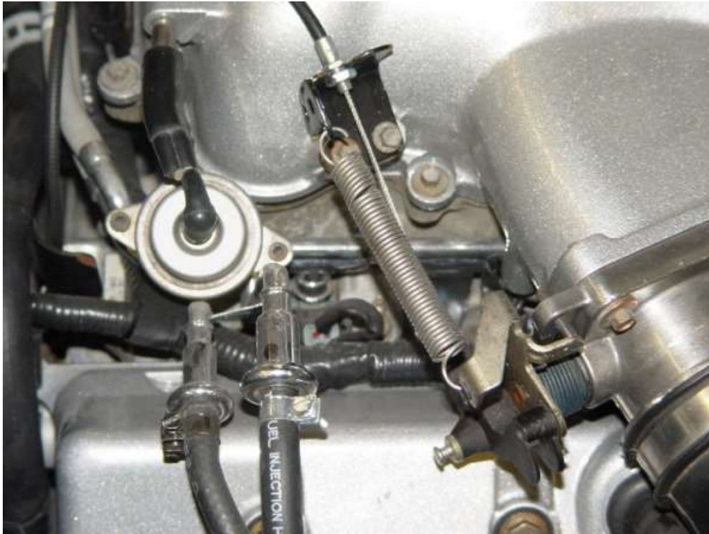
Accelerator cable mounted on 1998 4 valve Intake.
