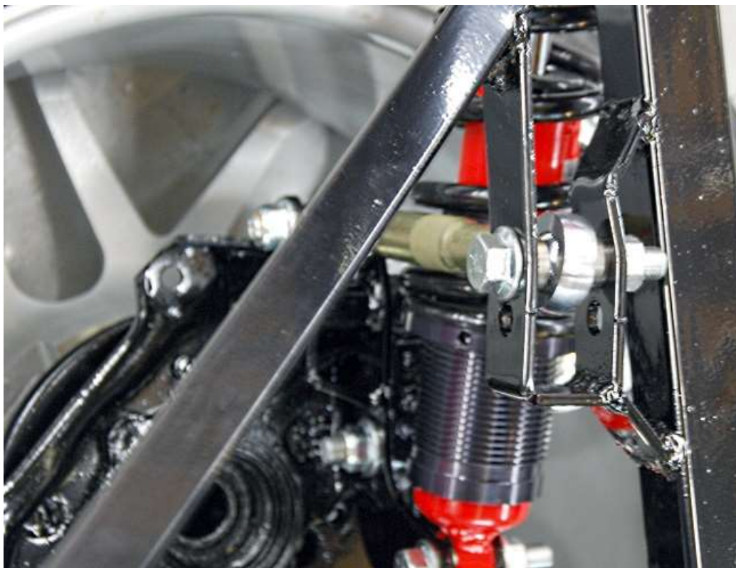
The upper link mounts to the upper hole in the chassis as well.
