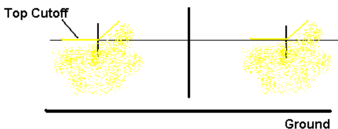
Figure 3: Headlight alignment aim
