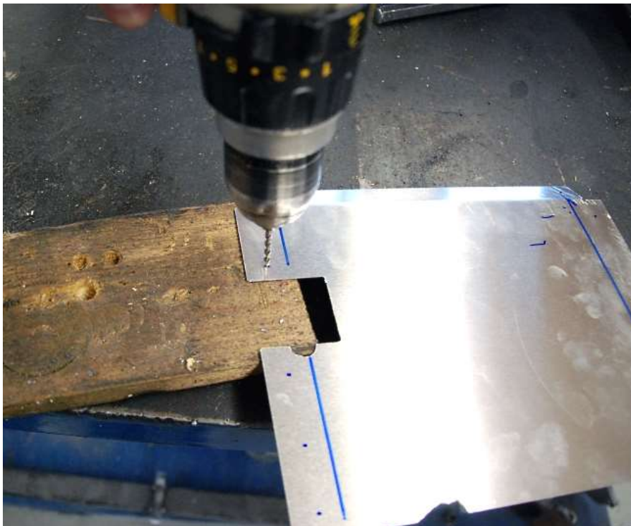
Drill all of the holes out using a \frac{1}{8} inch drill bit.
