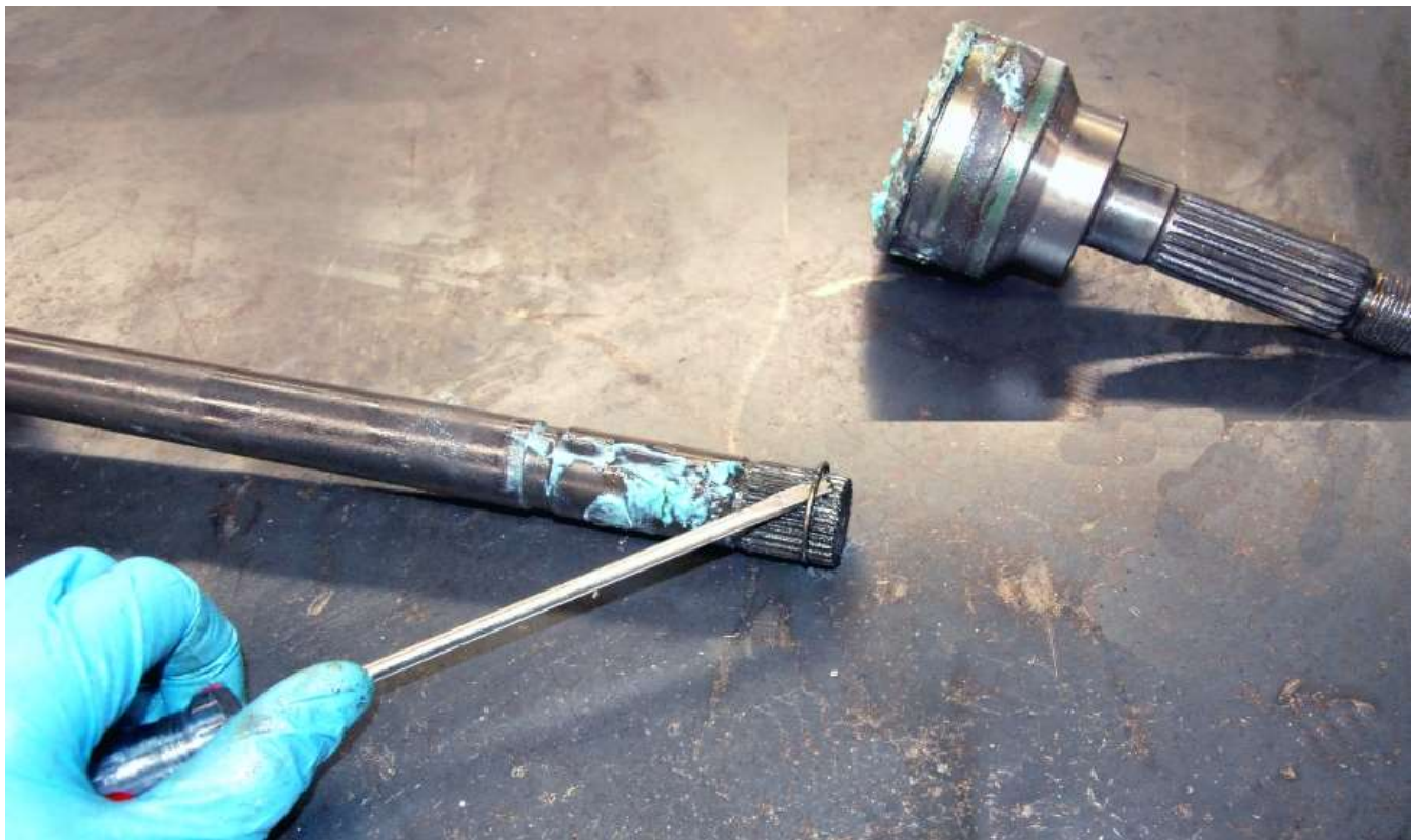
Remove the retaining clip from the axle and save it for the new axle.
