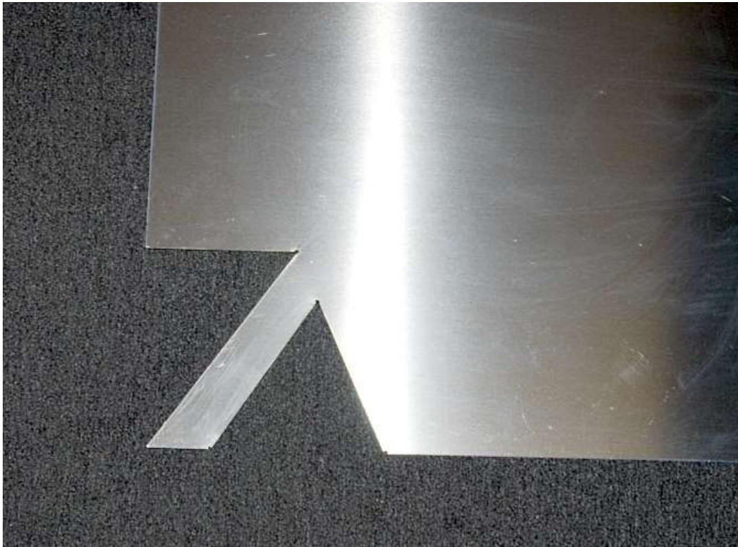
Panel cut for two coolant tubes. (note: Only the lower triangle is needed for single coolant line per side)
