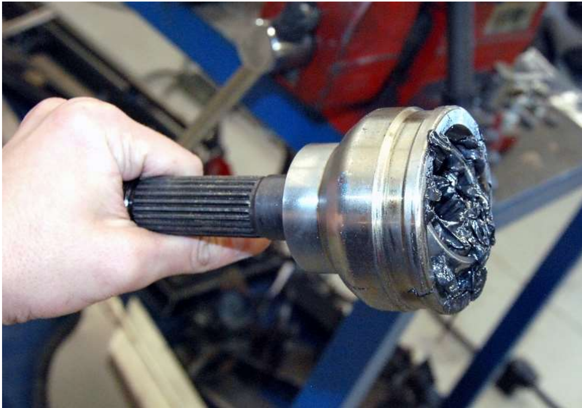
Outer CV joint removed from the axle.
