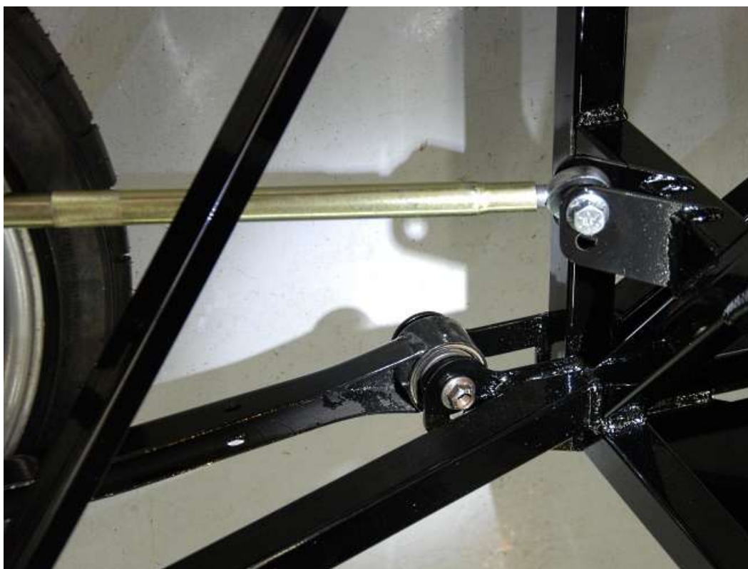
Upper and lower trailing arms mount in the upper mounting holes.
