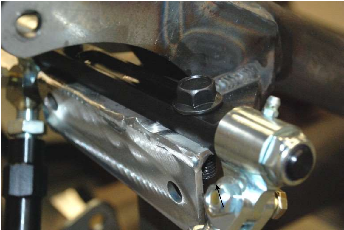
Front upper control arm mounting with FFR Spindles
