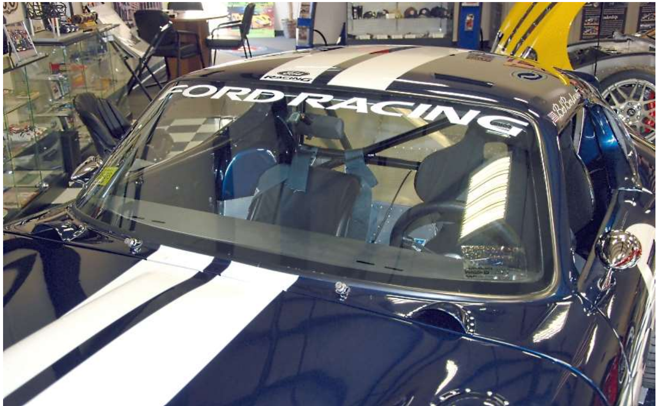
Windshield mounted on the body with 409 T 102 weatherstrip
