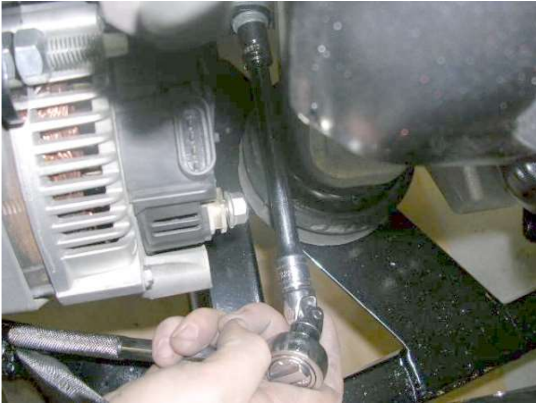
Rear bolt (the engine harness clamp bolt – 13 mm).
