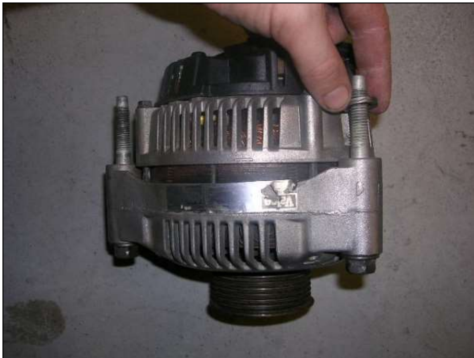
Insert the alternator bolts through the alternator then put the supplied spacers (FFR# 13210) on.
