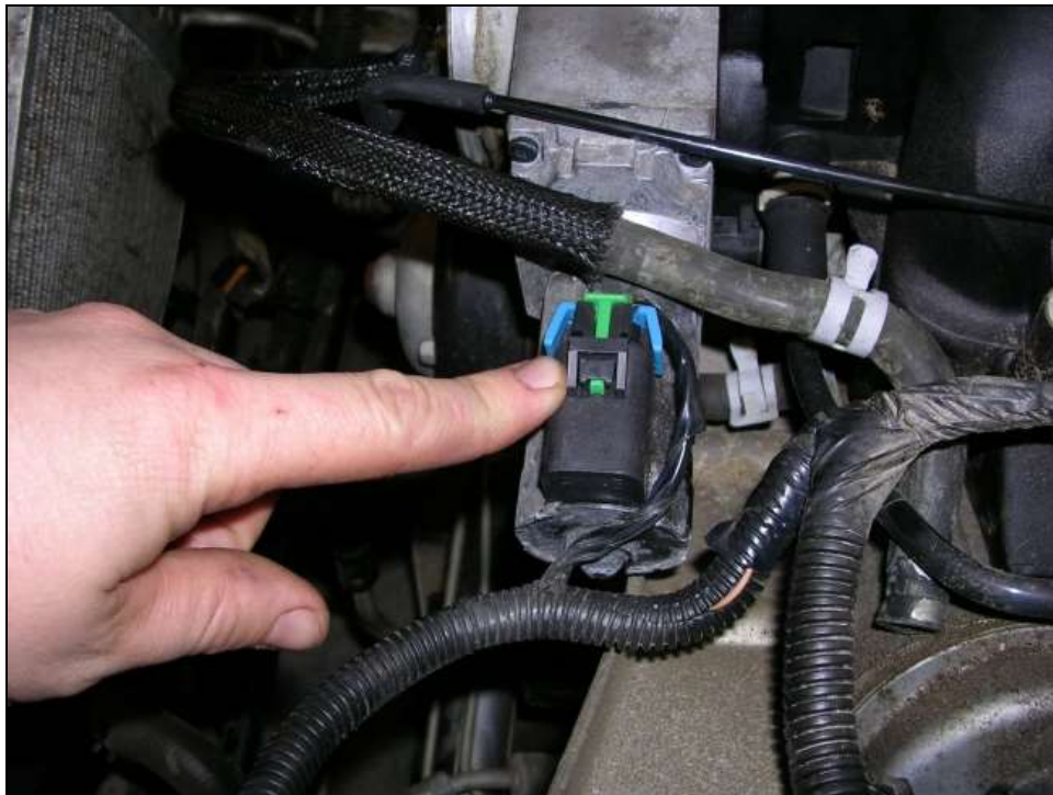
Disconnect the throttle body motor electrical plug.
