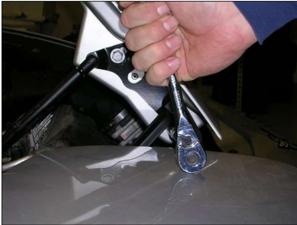
Remove the lower hinge bolts at the hood (13mm socket).
