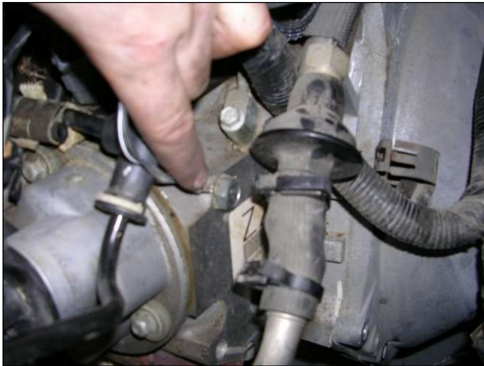
Ground and harness Clamp at rear of Driver Side.
