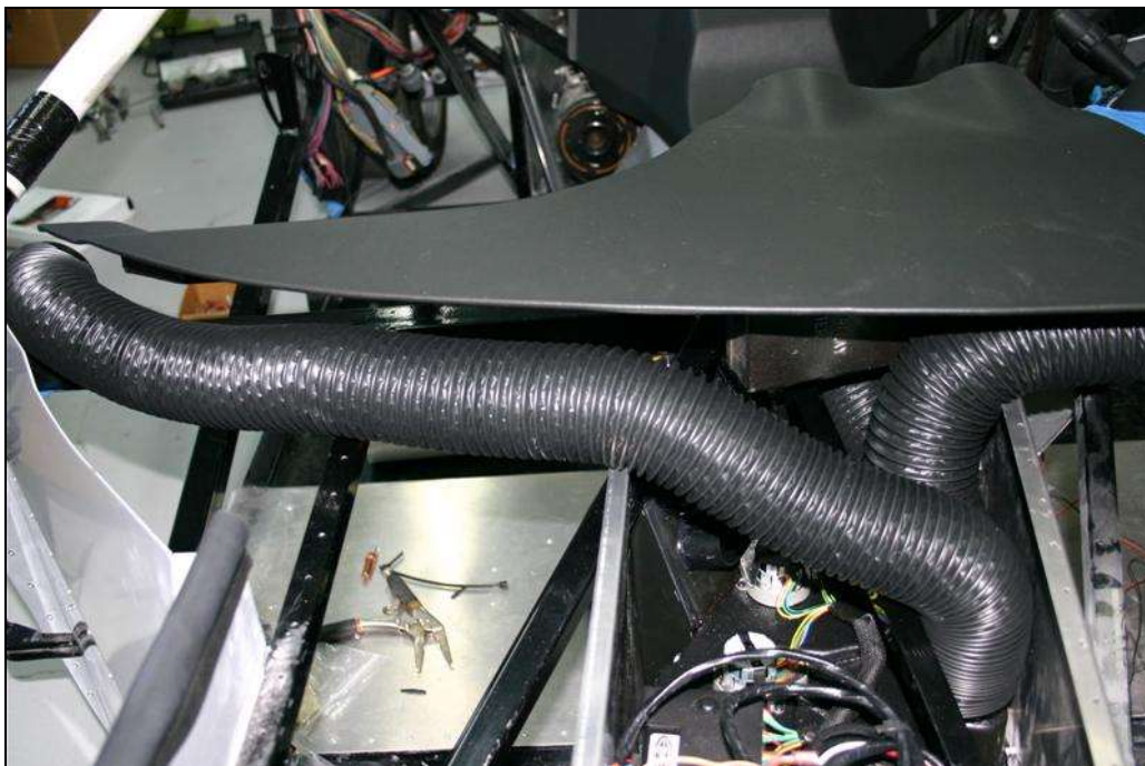
Routing the hoses with footbox roof panel already trimmed.
