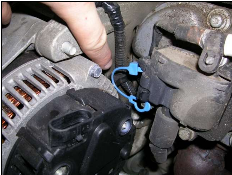
Disconnect the alternator connections (13 mm), wiring clamp behind the alternator.
