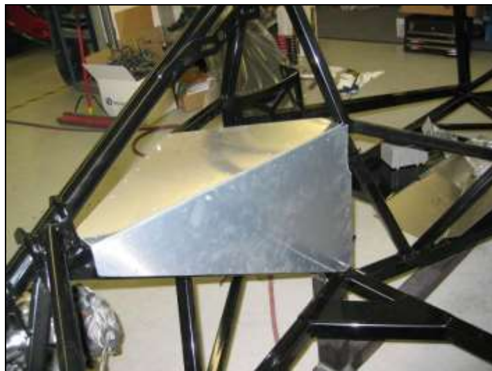
These panels are riveted to the 1" frame members. Make sure to pre-fit these panels before drilling.
