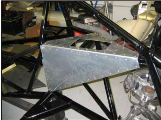
The cutout on the passenger side houses the Corvette fuse panel.
