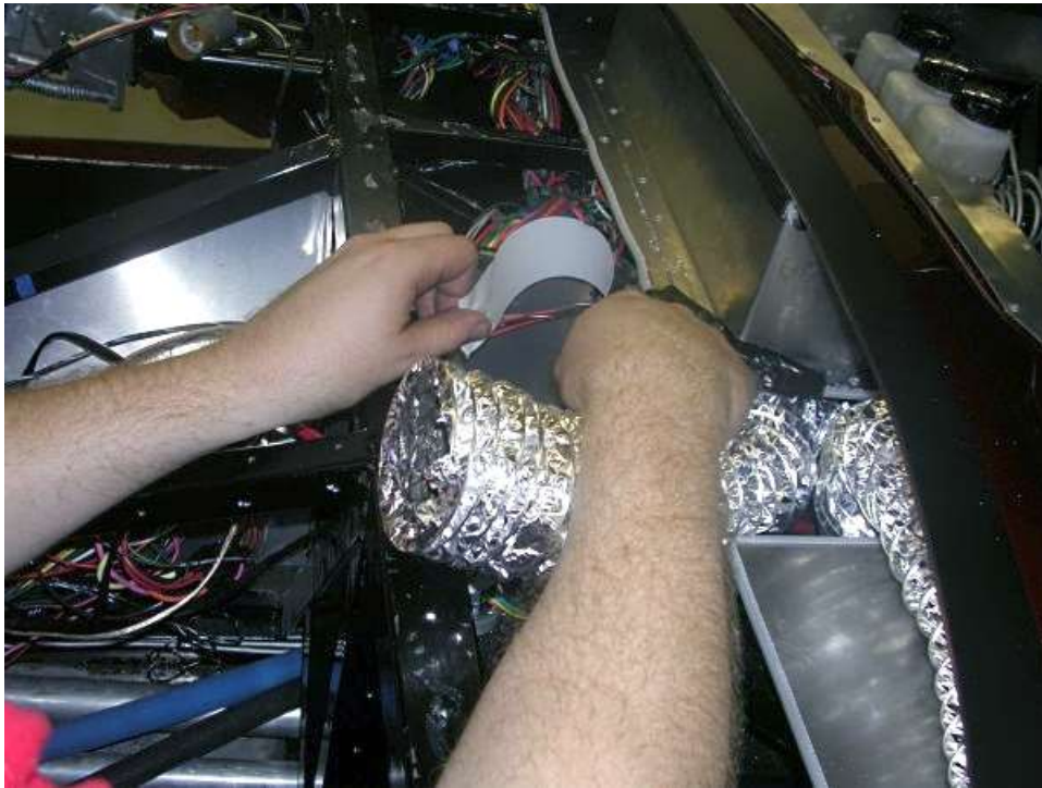
Routing the hoses with footbox roof panel already trimmed.
