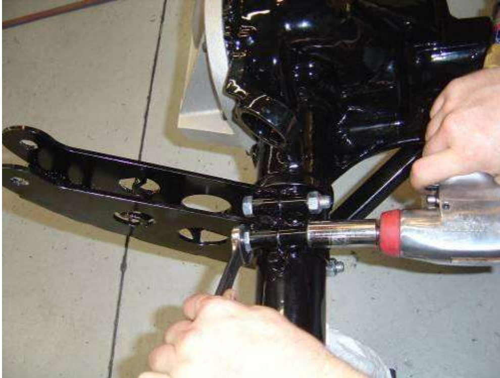
Install the upper link bracket onto the axle using the fine hardware (FFR# 12217 & 12218)
