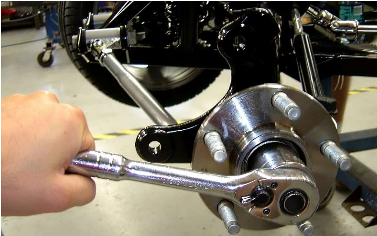
Install the hub nut onto the spindle. Torque the hub nut to 305-338Nm (225-250 lb-ft) .
