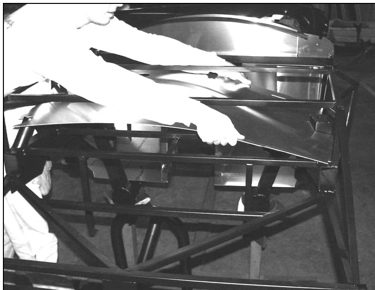
Fitting the mid-trunk panel. Bend the panel as shown and insert the passenger's side first.
