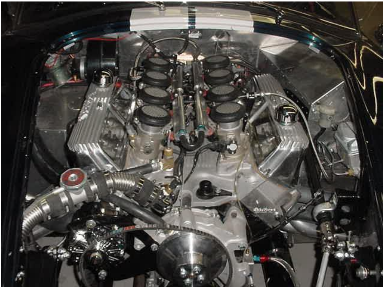
427 Shown here with fuel injection.
