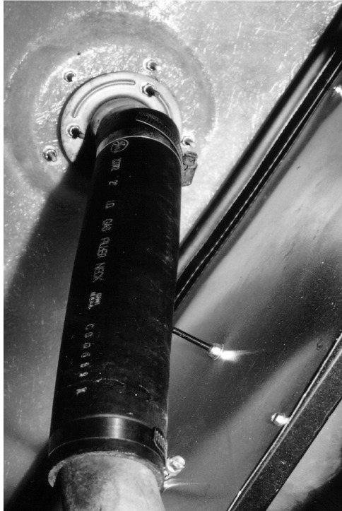
Underside view of installed fuel filler neck extension. Mustang neck bolts up to, and through, the composite body.
