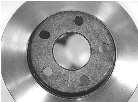
Wheel Stud holes elongated
