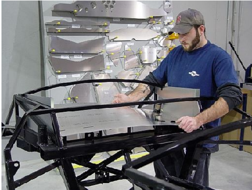
Fitting the mid-trunk panel. Bend the panel as shown and insert the passenger's side first.
