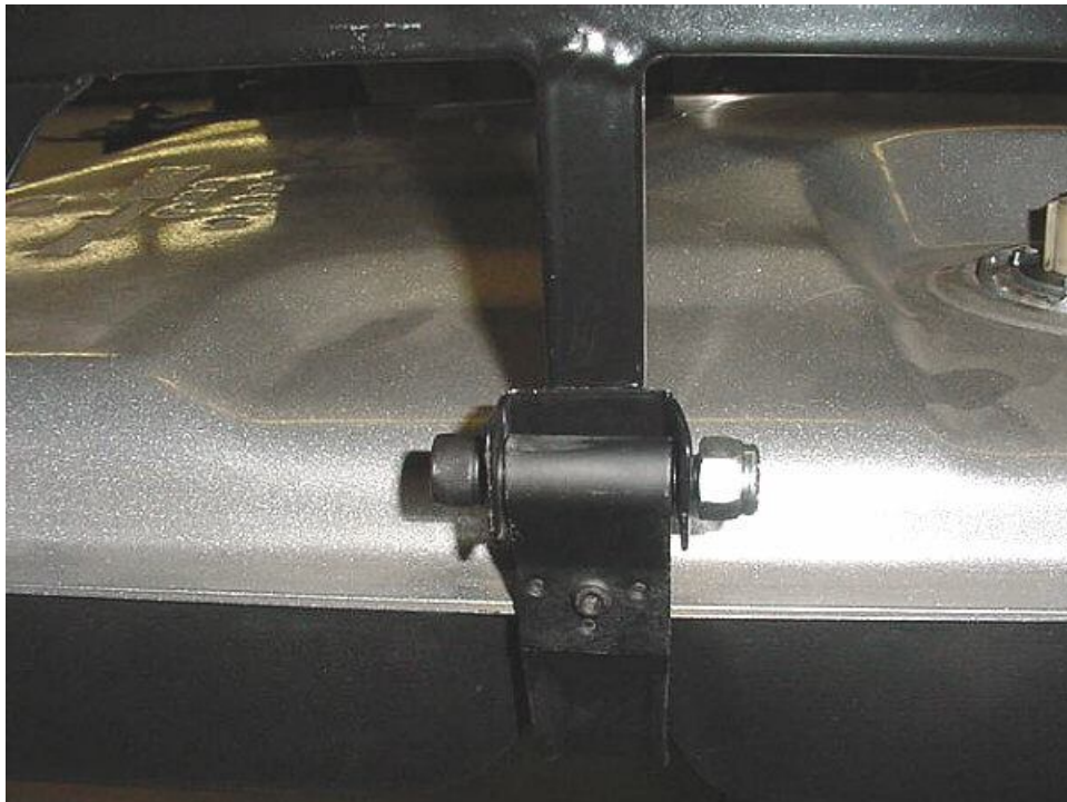
Driver side rear tank strap mount.
