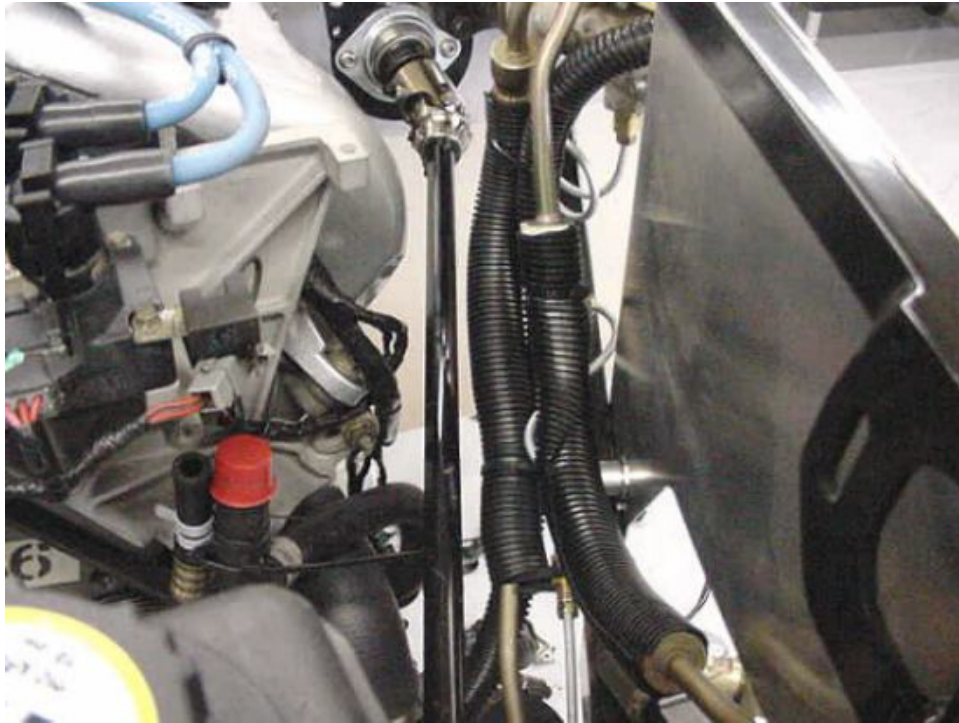
Lines running from booster, along steering shaft to steering rack.
