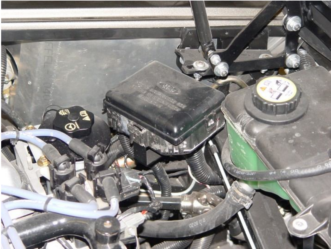
Fuse Panel mounted in the engine Bay.
