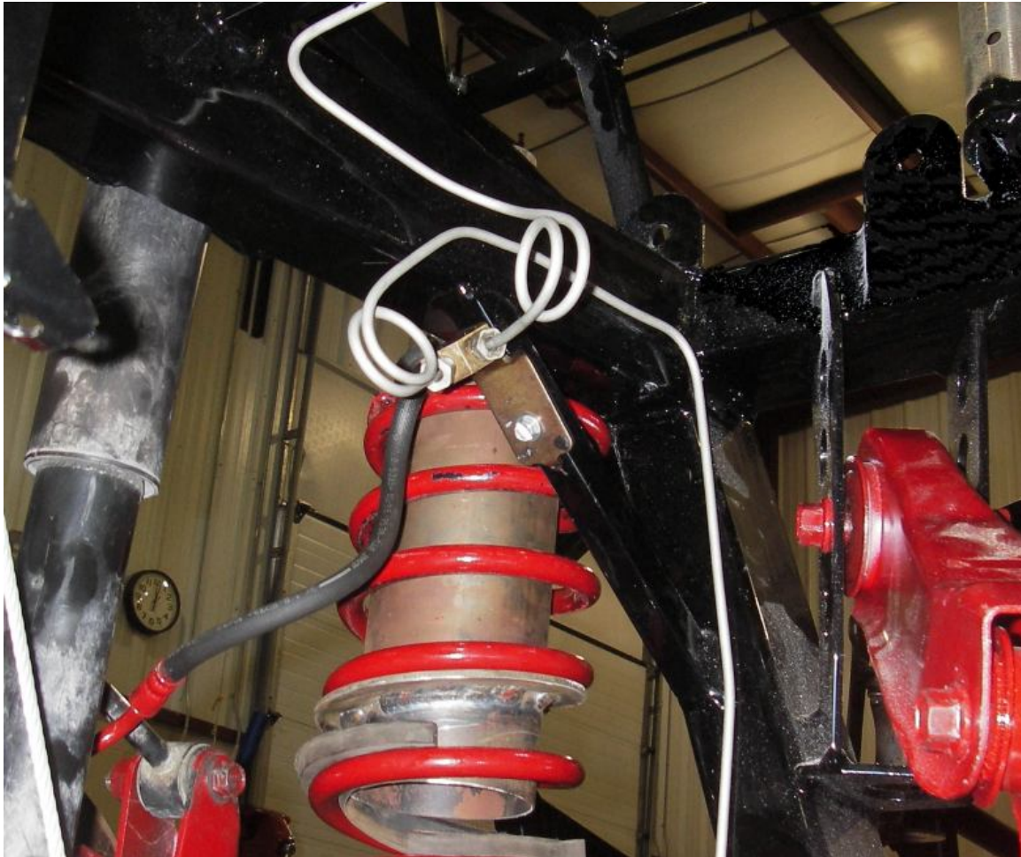
Driver side brake line mount. Note the loops in the line.
