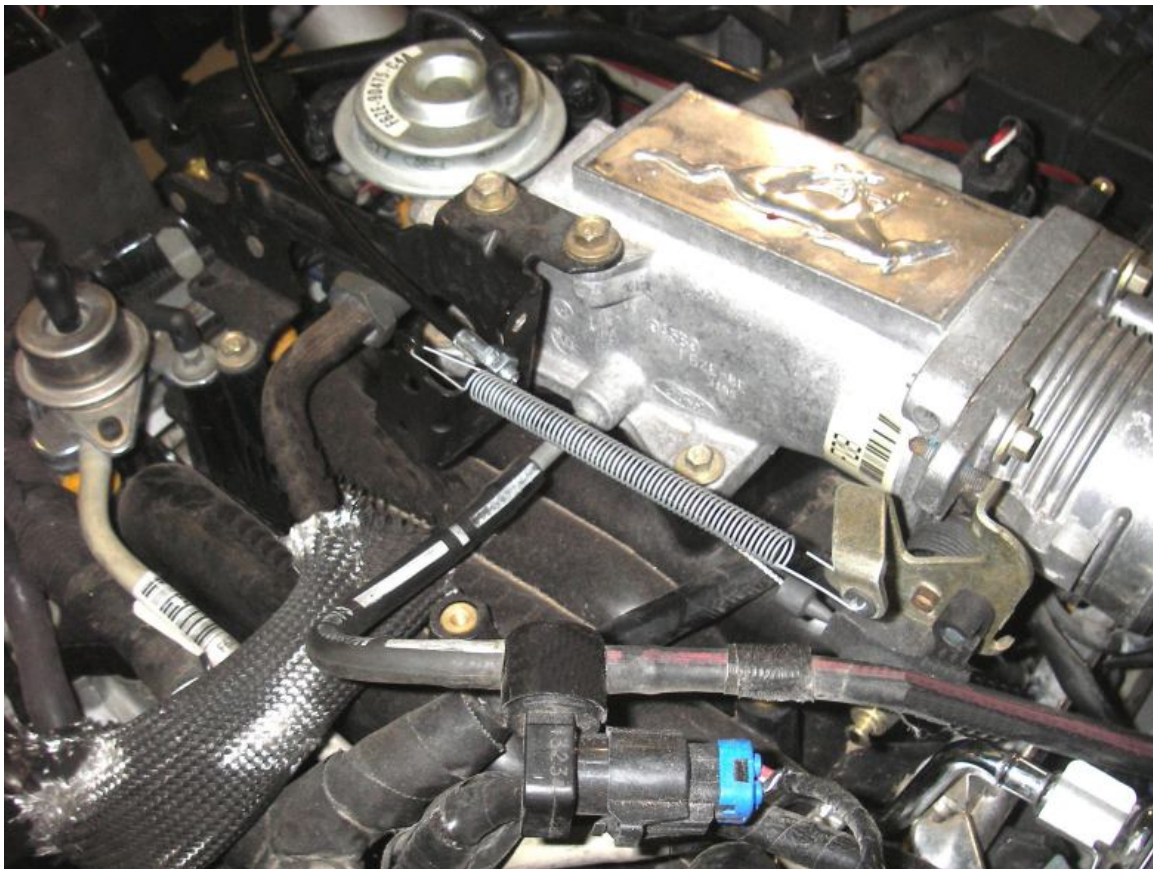
Accelerator cable mounted on '96 2 valve intake.
