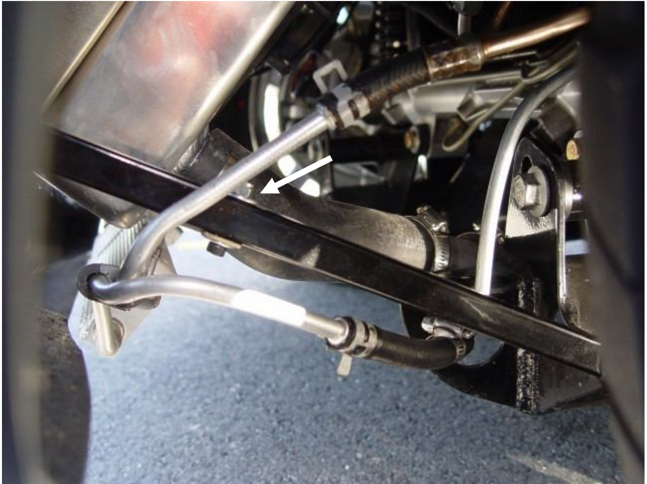
Driver side mount of the cooler mounted to \frac{3}{4} " tube and inlet/outlet tubes bent.
