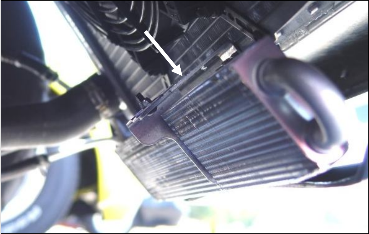
Power steering cooler mounted to the bottom of the radiator. Note the 90 degree bent mount bracket.
