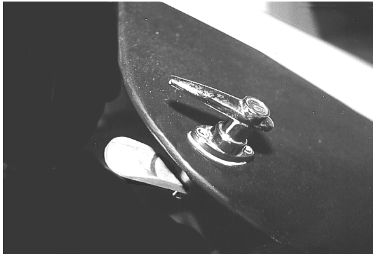
Mounted L-shaped hood handle with cam wedge.
