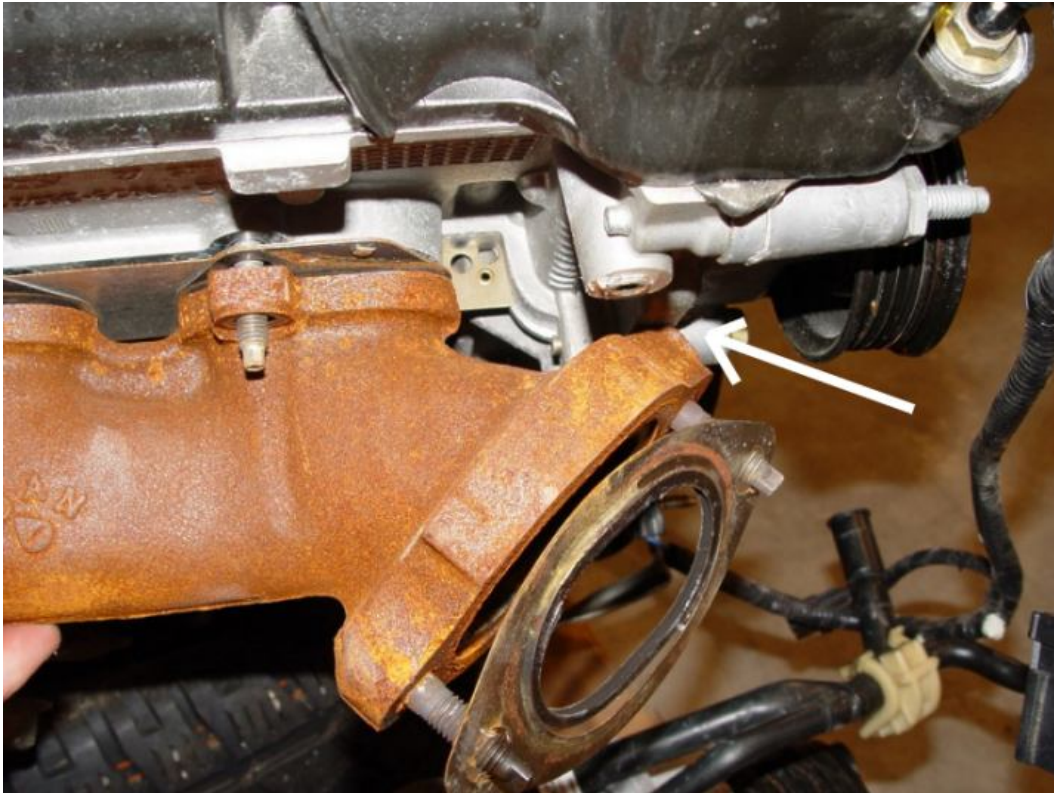
Passenger side manifold. Note the casting touches the block.
