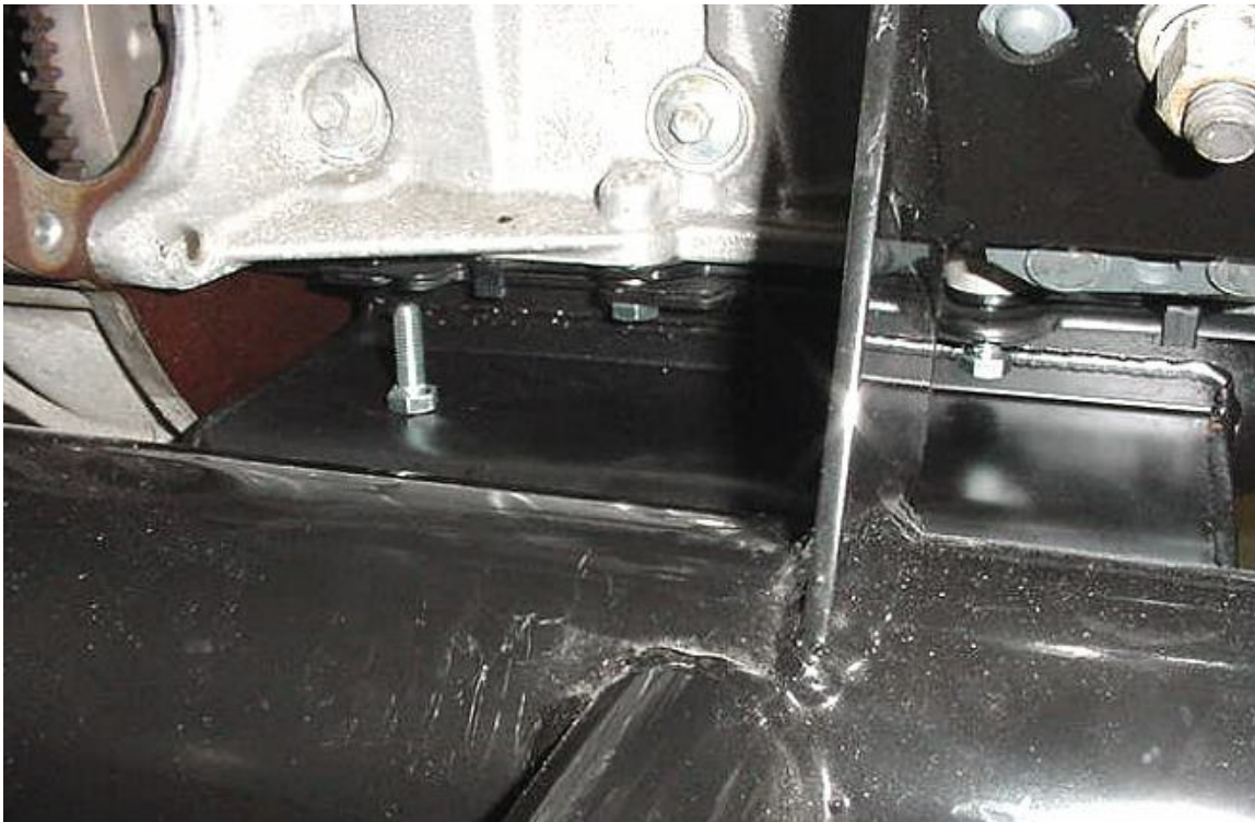
Short oil pan attaching bolts over kick out.
