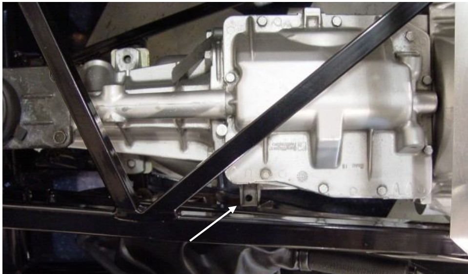
T-5 mounted in frame. Note the tab to be removed.
