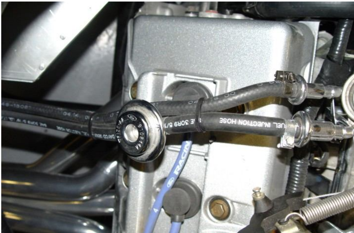
Fuel lines coming off the intake. Surge dampner shown.
