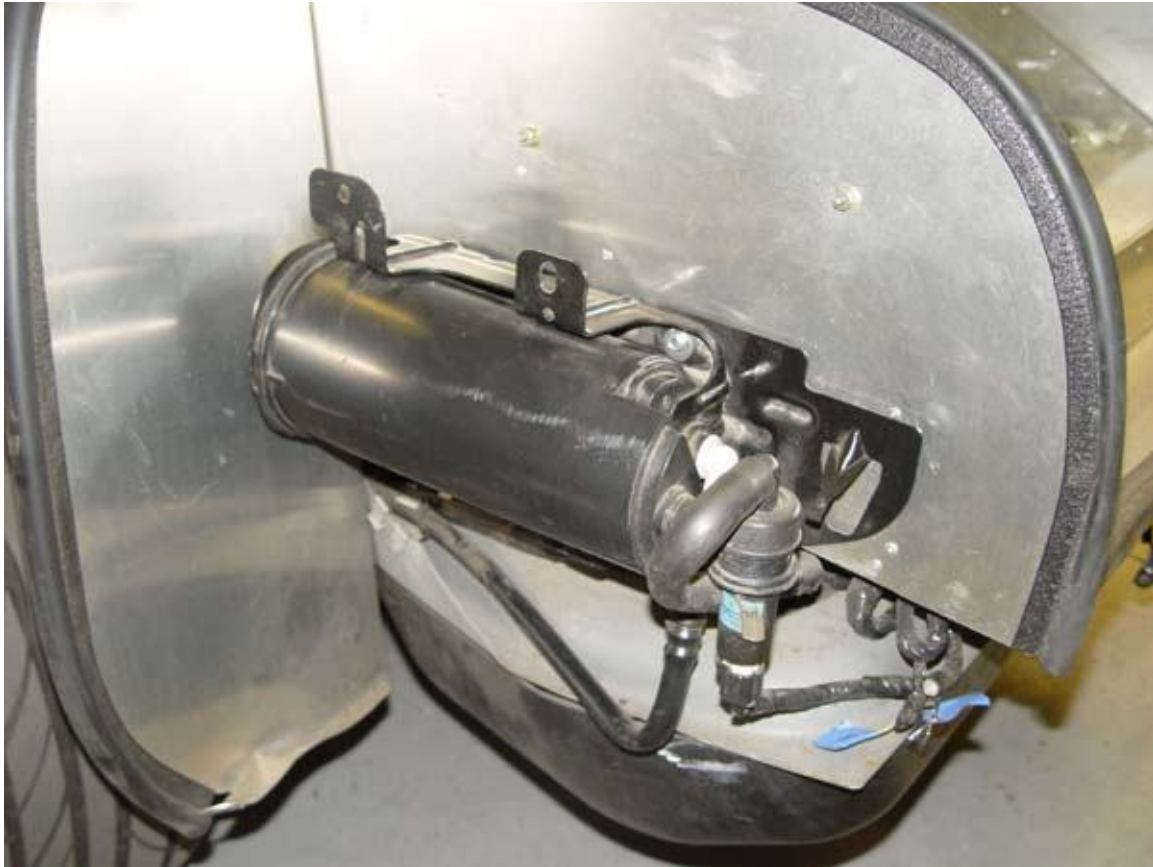
Charcoal can mounted on drivers side rear. Note: Splash guards are not mounted until after the body is on.
