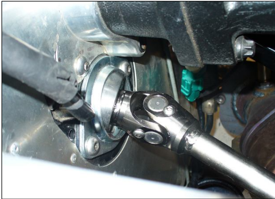
Flange Bearing mounted to front of footbox.
