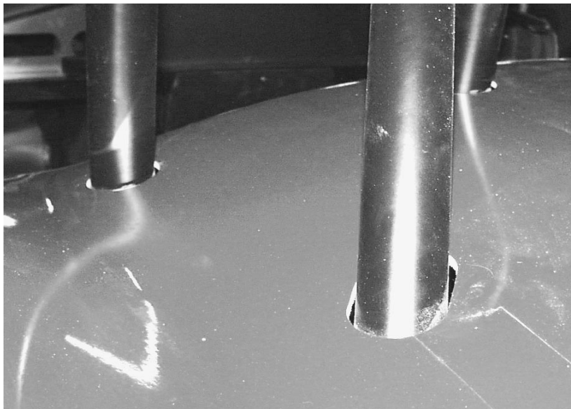
Roll bar holes cut out with roll bar installed.
