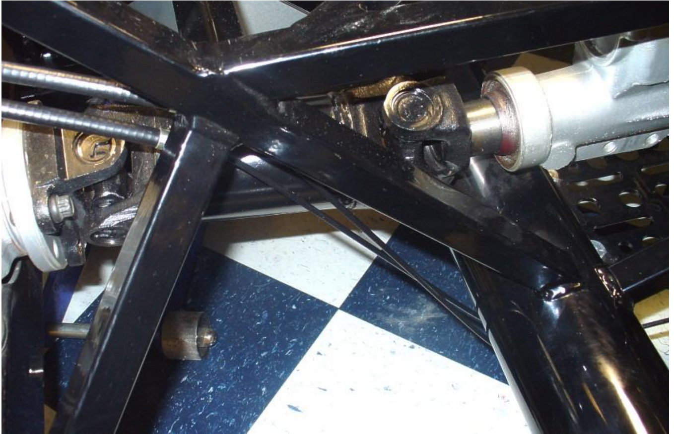
Brake cables running under the 4" crossmember.
