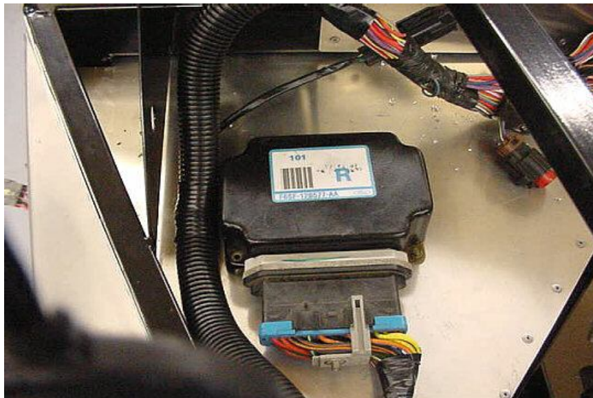
Constant control relay mounted to the top of the passenger footbox.
