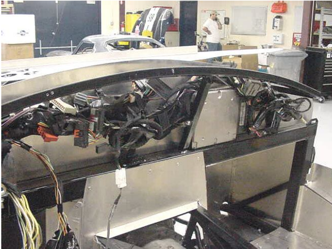
Dash wiring showing computer mounted on the passenger side of the firewall.
