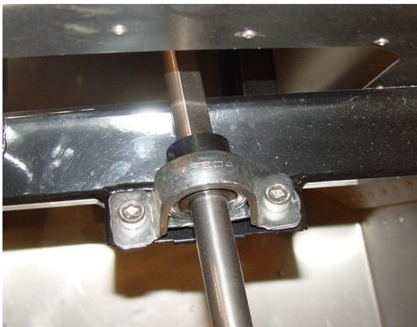
Overhead view looking down onto upper steering pillow block installed on frame 2"x 2" dash support.
