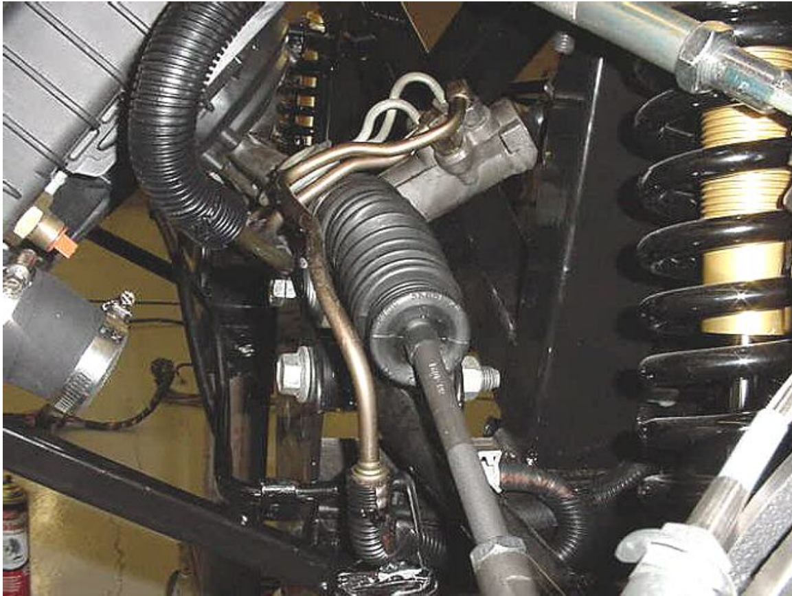
Power steering line for steering rack. Note stock line bent.
