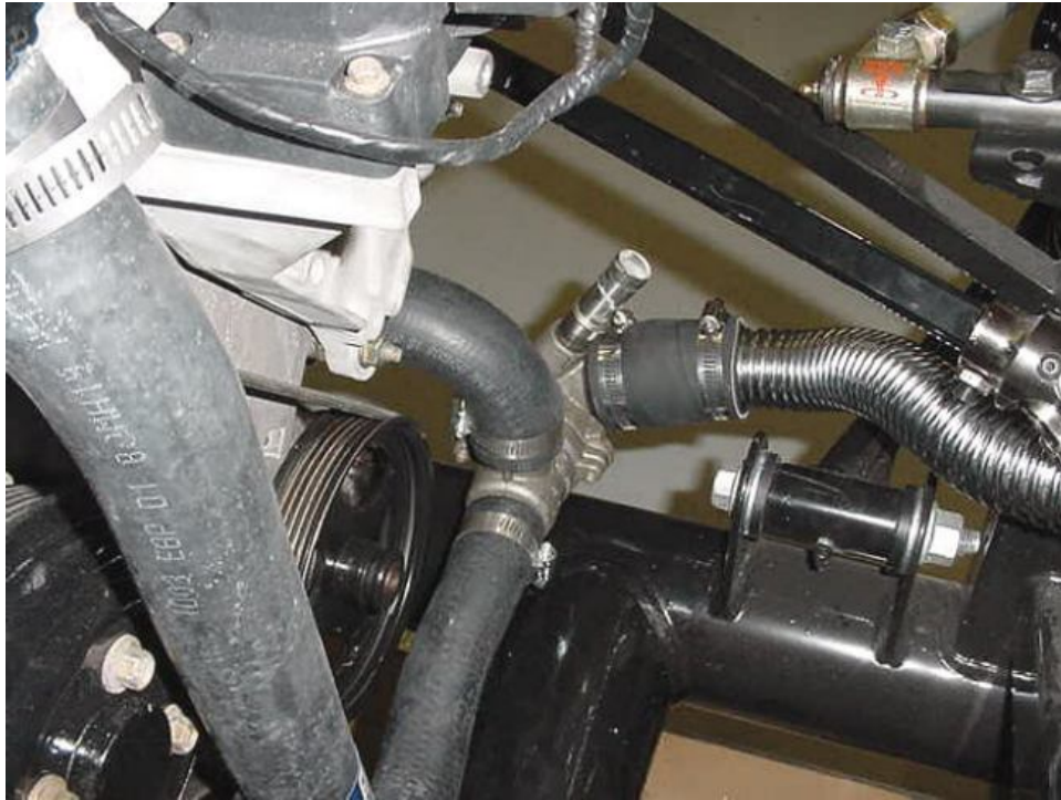
Lower radiator hose from engine to thermostat housing and bypass tube from DOHC engine to radiator housing.
