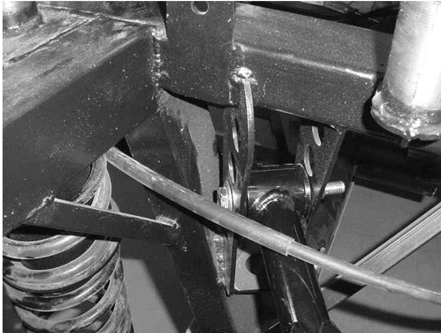
Parking brake cable passing through triangle and in front of coil spring on driver's side
