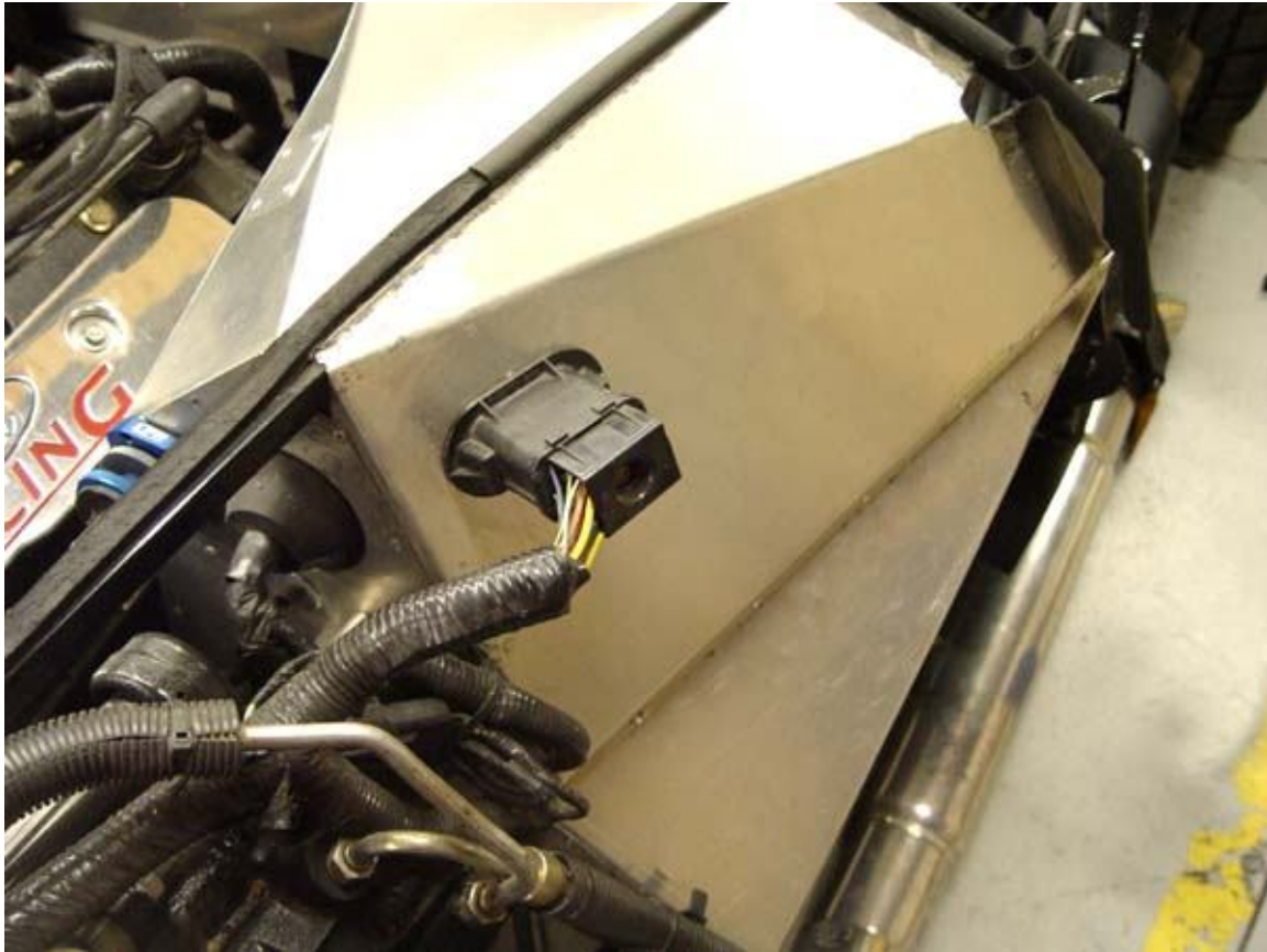
Optional way to run the dash harness so the conical rubber bushing does not need to be cut.
