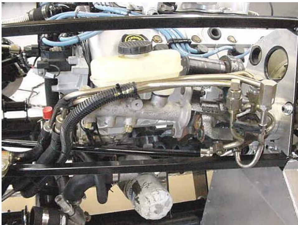
Hydro-boost lines shown in stock location. Lines must be bent and re-routed to fit behind aluminum
