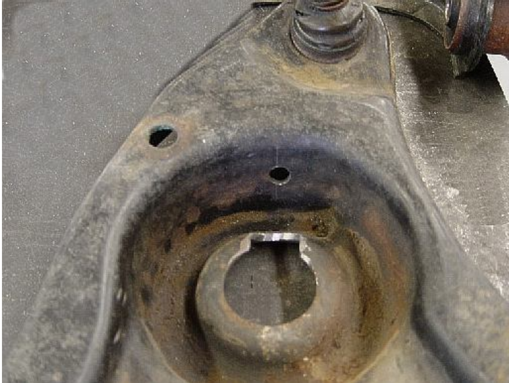
Drilled and modified front lower control arm.
