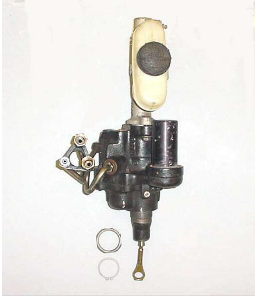
1997 Hydro-booster, Master cylinder, Hydro-boost retaining nut and snap ring.
