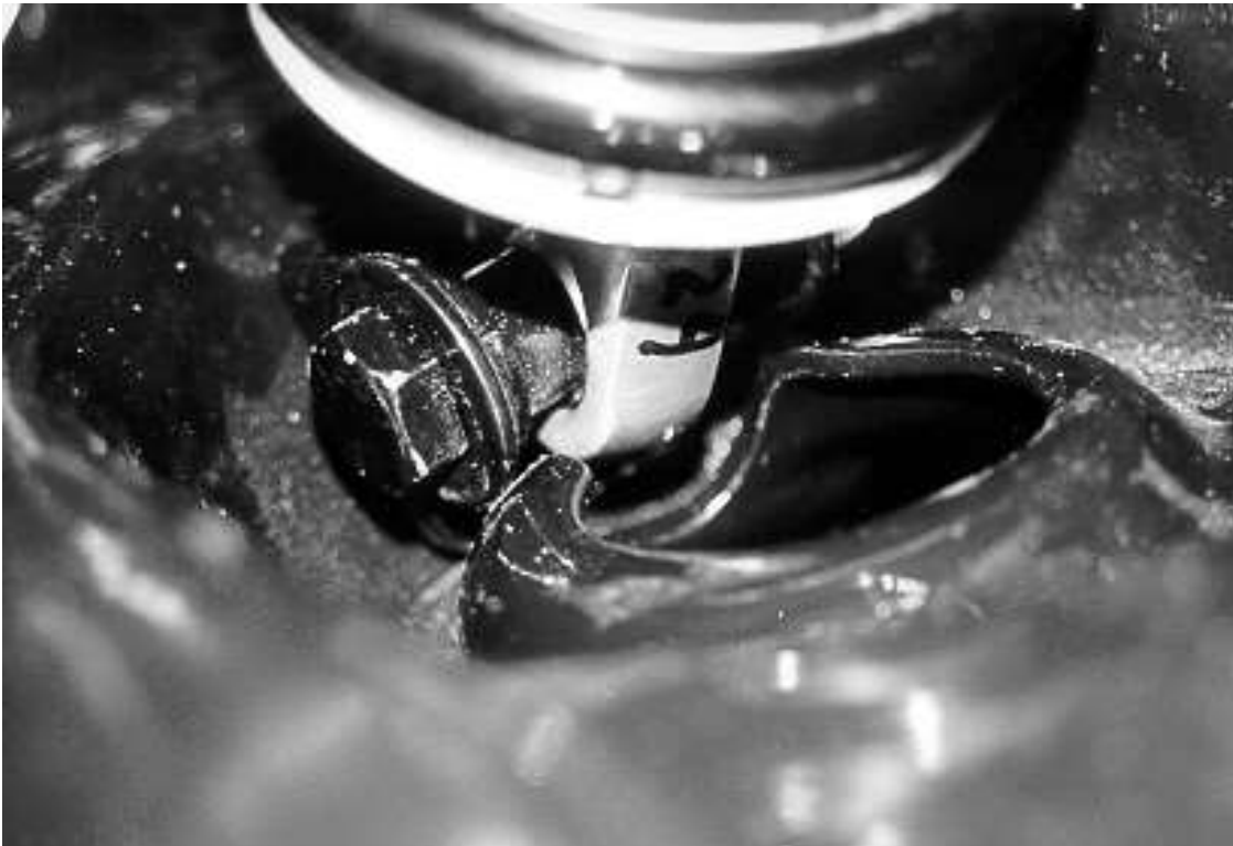
Coil-over mounted in lower arm with clearance hole.
