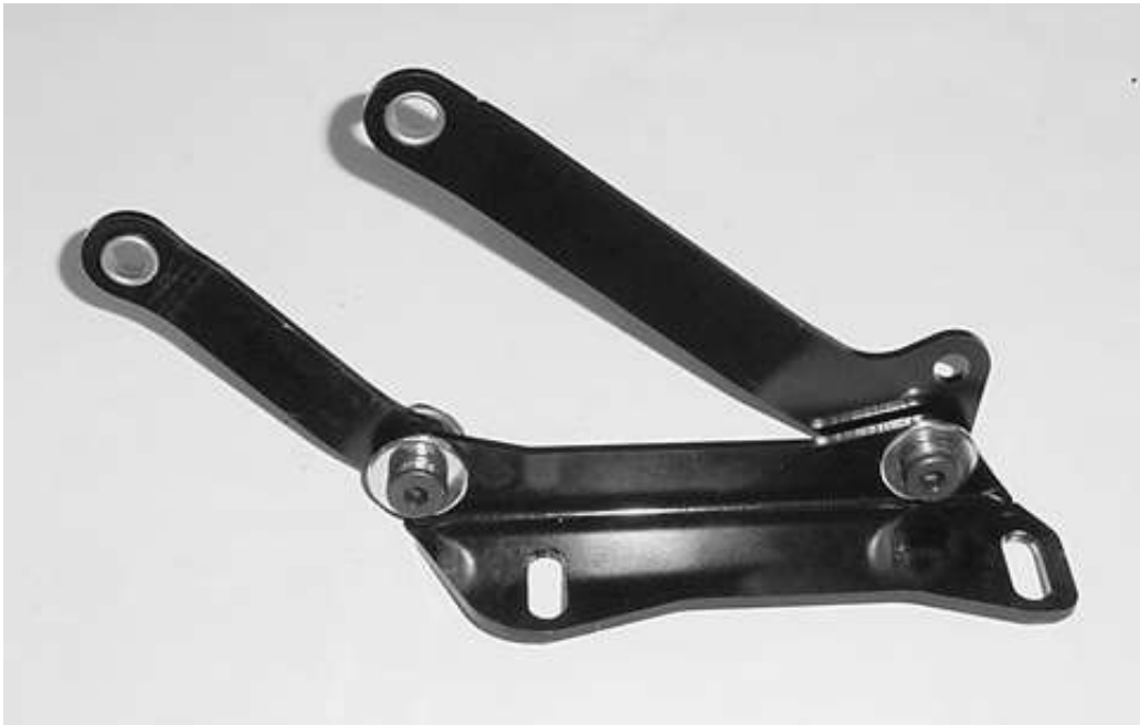
Drivers side arm plate with arms attached
