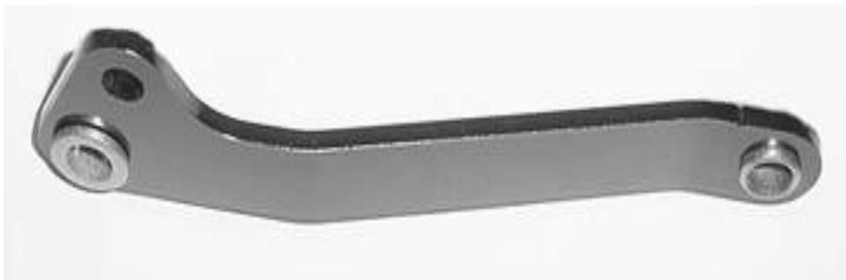
Passenger side long arm with bushings pressed in
