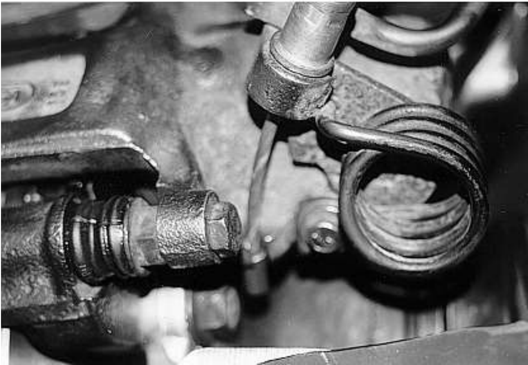
Emergency brake cable in caliper bracket.
