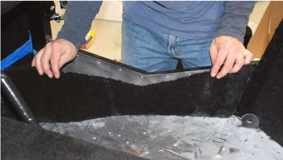
Fit and glue the under-door piece.
