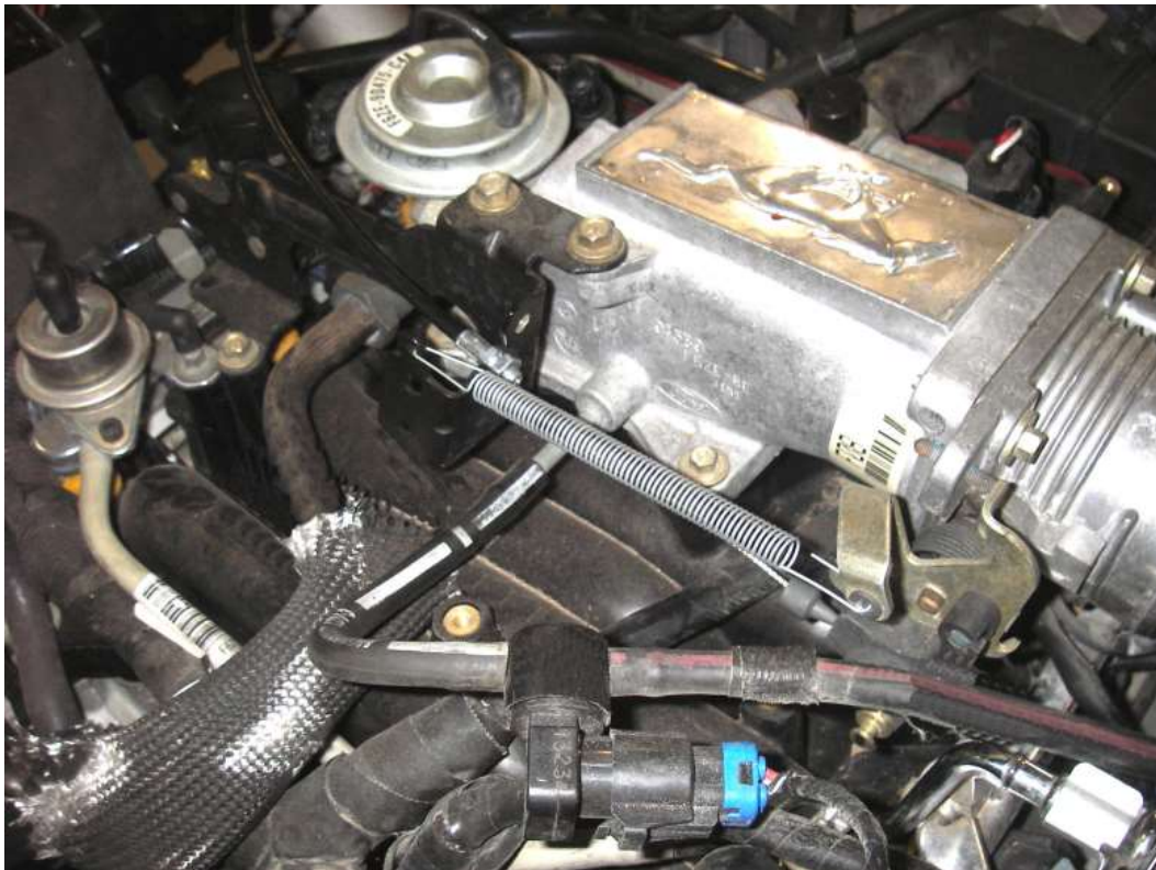
Accelerator cable mounted on '96 2 valve intake.
