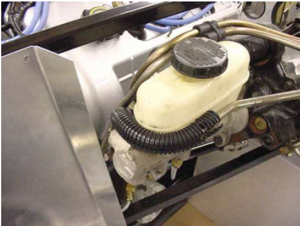
Tubes bent around inside of Master cylinder.
