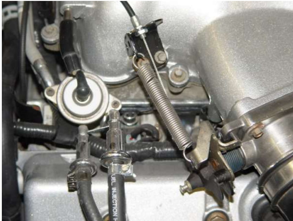
Accelerator cable mounted on '98 4 valve intake.
