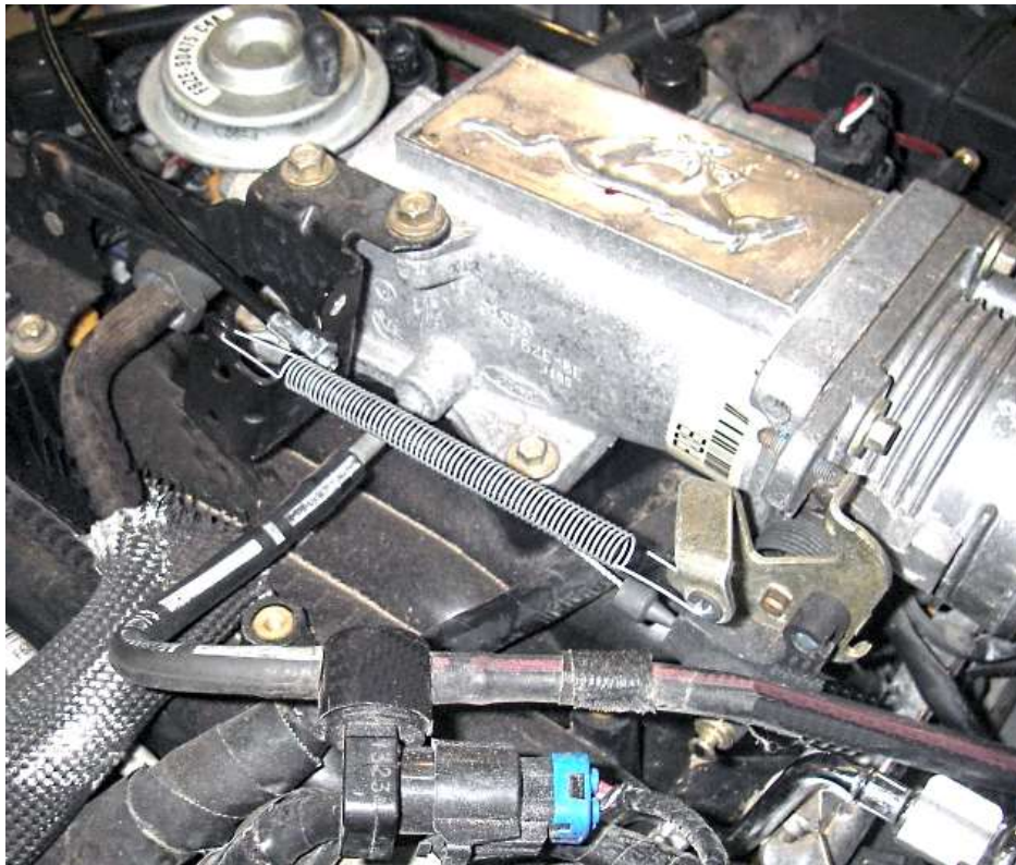
Accelerator cable mounted on '96 2 valve intake.
