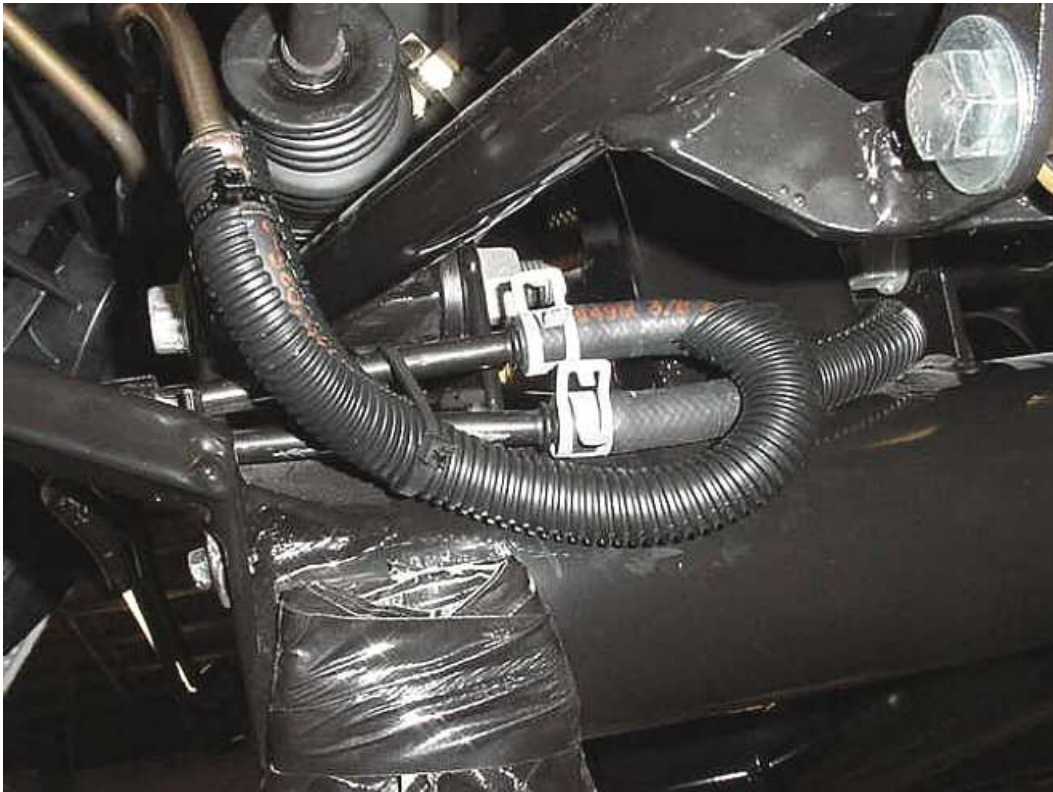
Hose routing for 96-2000 power steering cooler.
