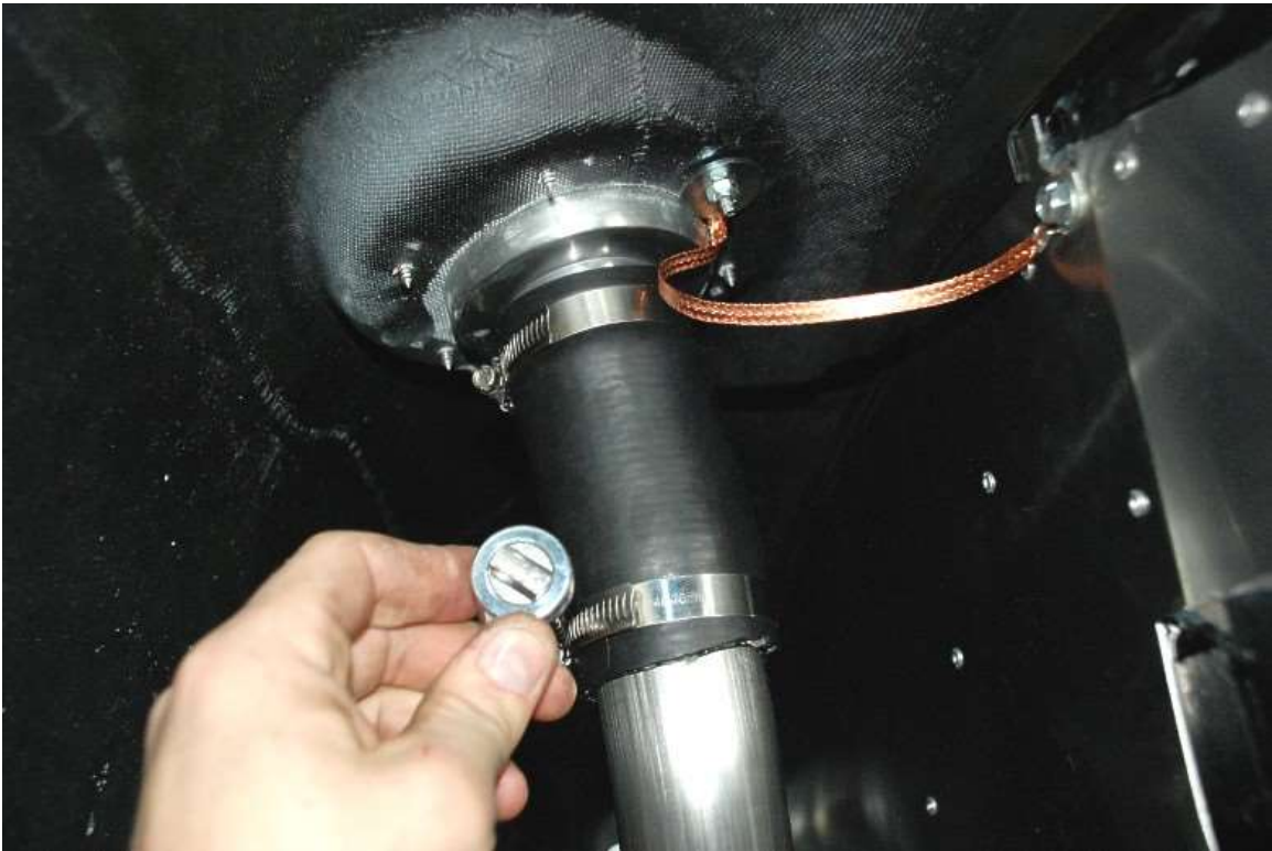
Install the hose between the filler neck and gas cap with the clamps that came in the cap hardware.
