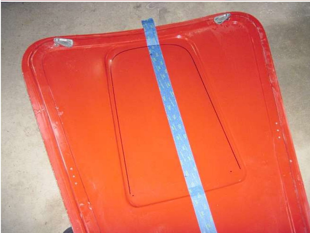
Mark around the edge of the hood scoop
