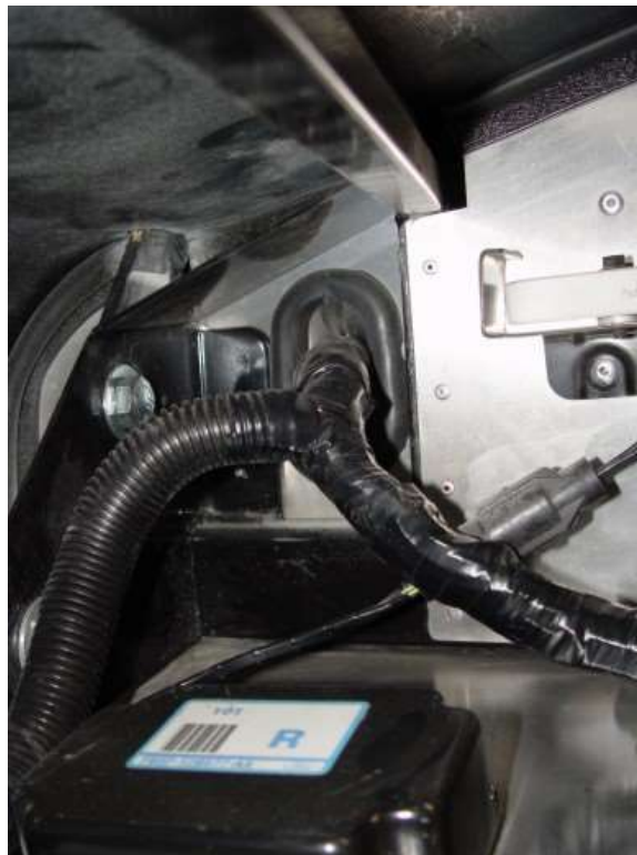
The engine harness begins in the passenger foot box. The computer plug is pushed through the oval shaped hole on the Firewall extension from the engine bay side.
