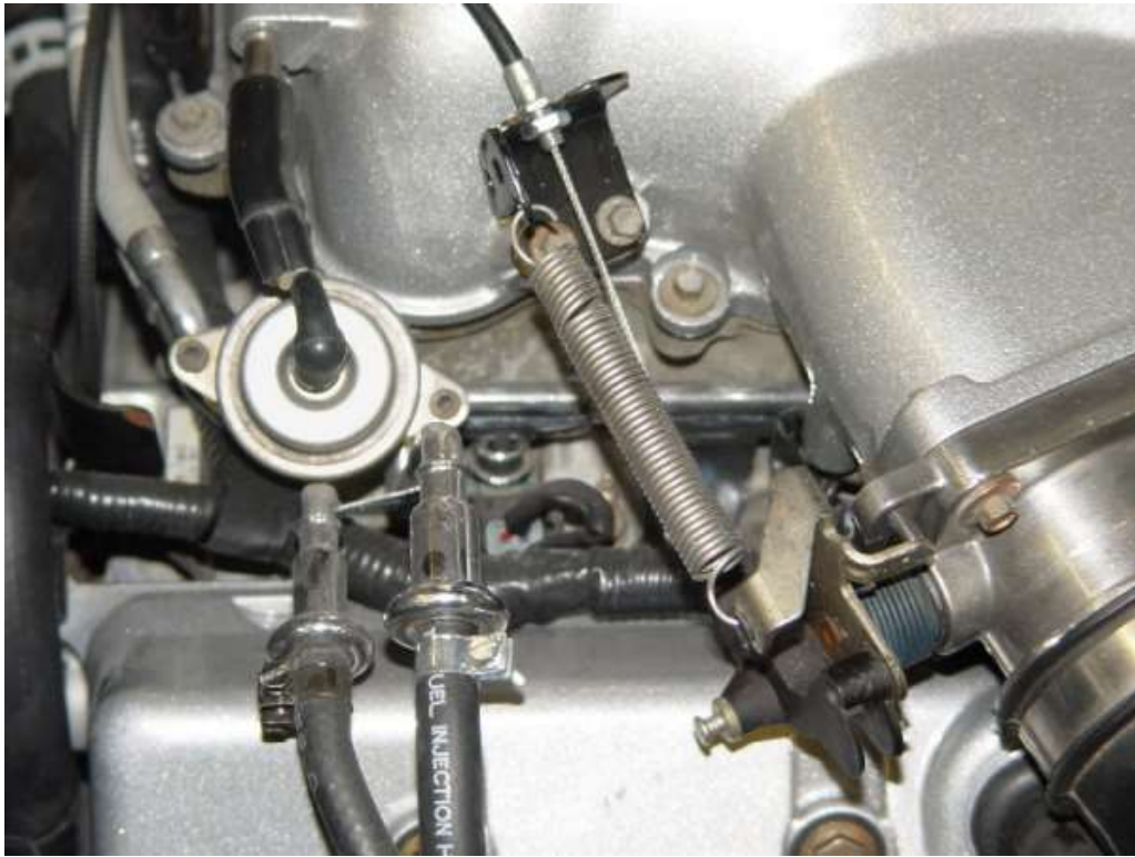
Accelerator cable mounted on '98 4 valve intake.
