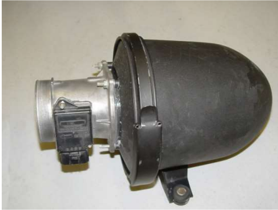
95-04 Mass Air Meter and Air Filter housing.
