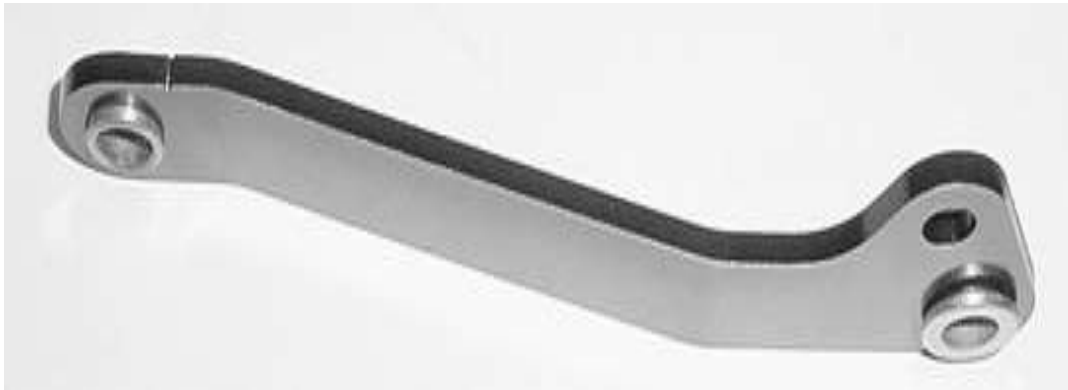
Drivers side long arm with bushings pressed in
