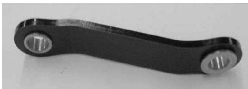
Passenger side long arm with bushings pressed in
