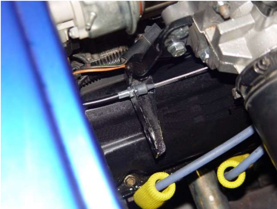
87-93 mounted accelerator cable.
