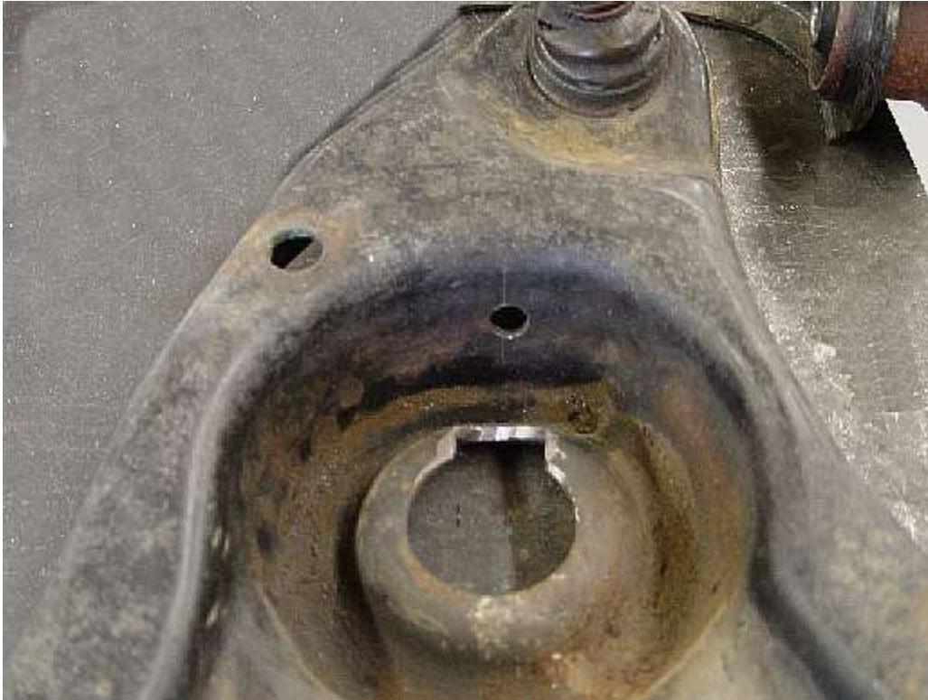
Drilled and modified front lower control arm.
