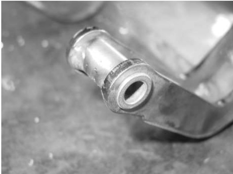
Bushings inserted into hinge arm.
