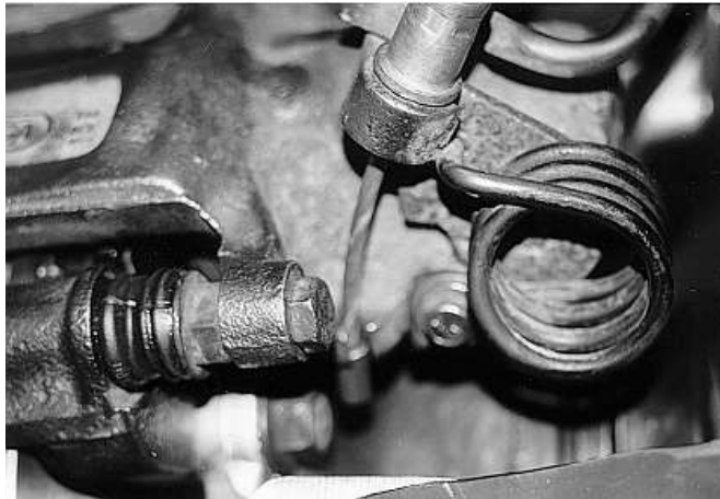
Emergency brake cable in caliper bracket.
