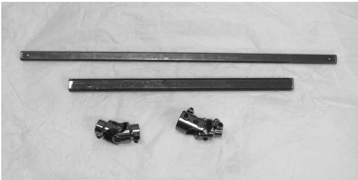
Top to Bottom: \frac{3}{4} " DD Lower Steering shaft, 1" DD tube, lower U-Joint, Upper U-Joint.
