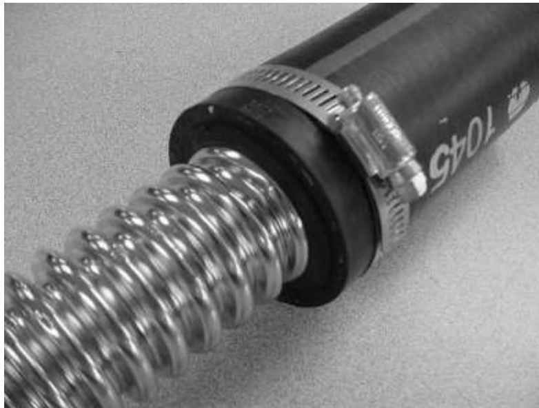
Filler hose clamped over the adapter hose.
