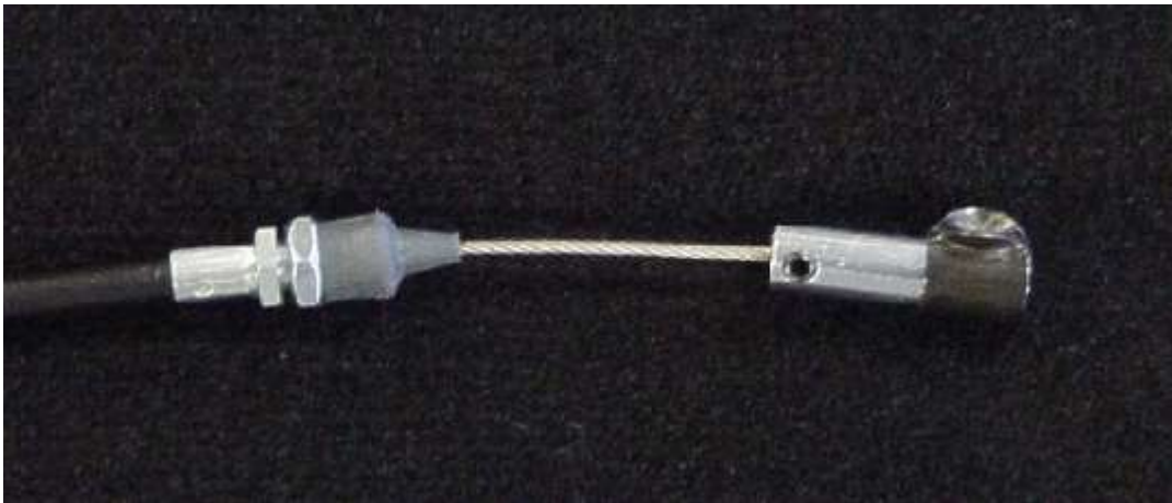
Ball stud retainer pushed onto cable.
