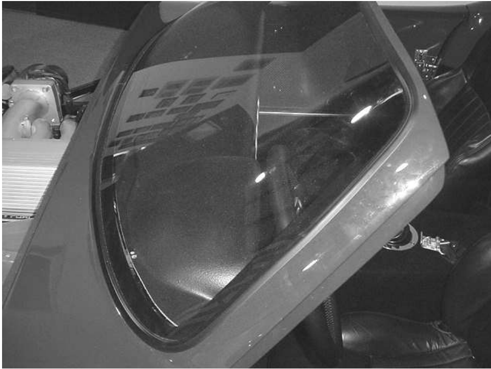
Windshield mounted on the body.
