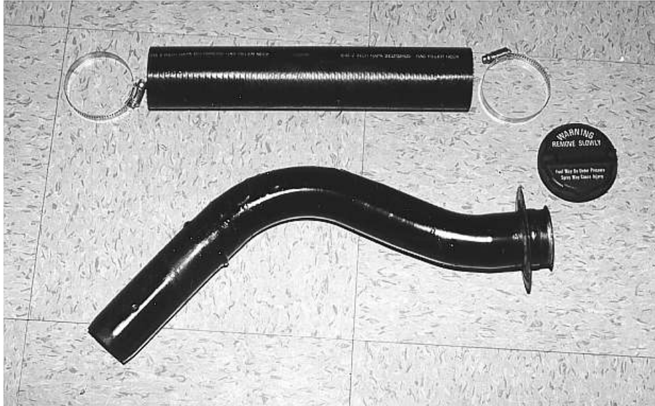
Mustang fuel tank neck with kit extension tube.
