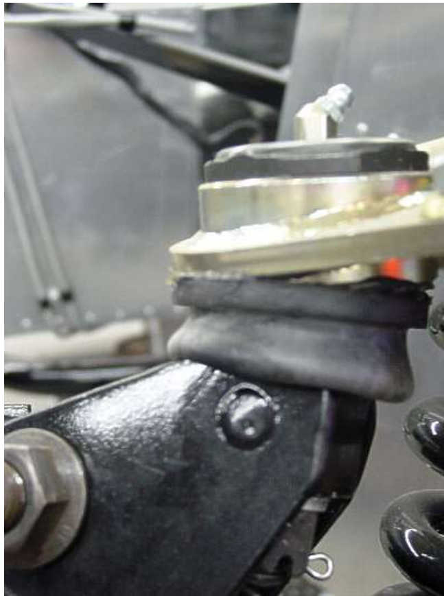
Ball joint in IFS Bracket.
