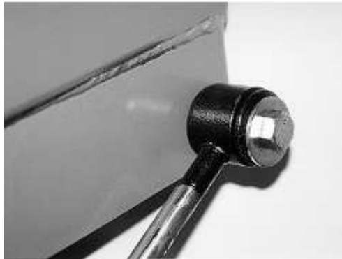
Quadshock mounted to frame bracket.
