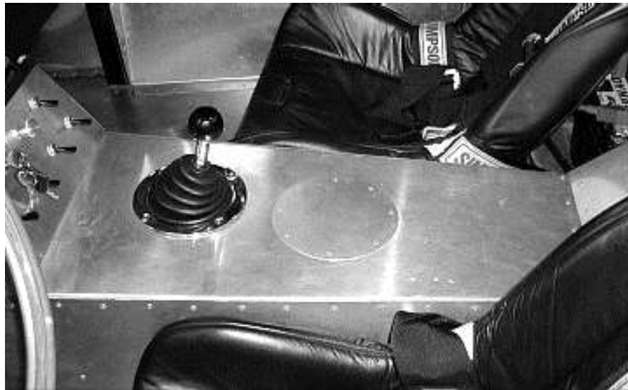
Transmission tunnel top panel mounted (FFR Coupe shown).
