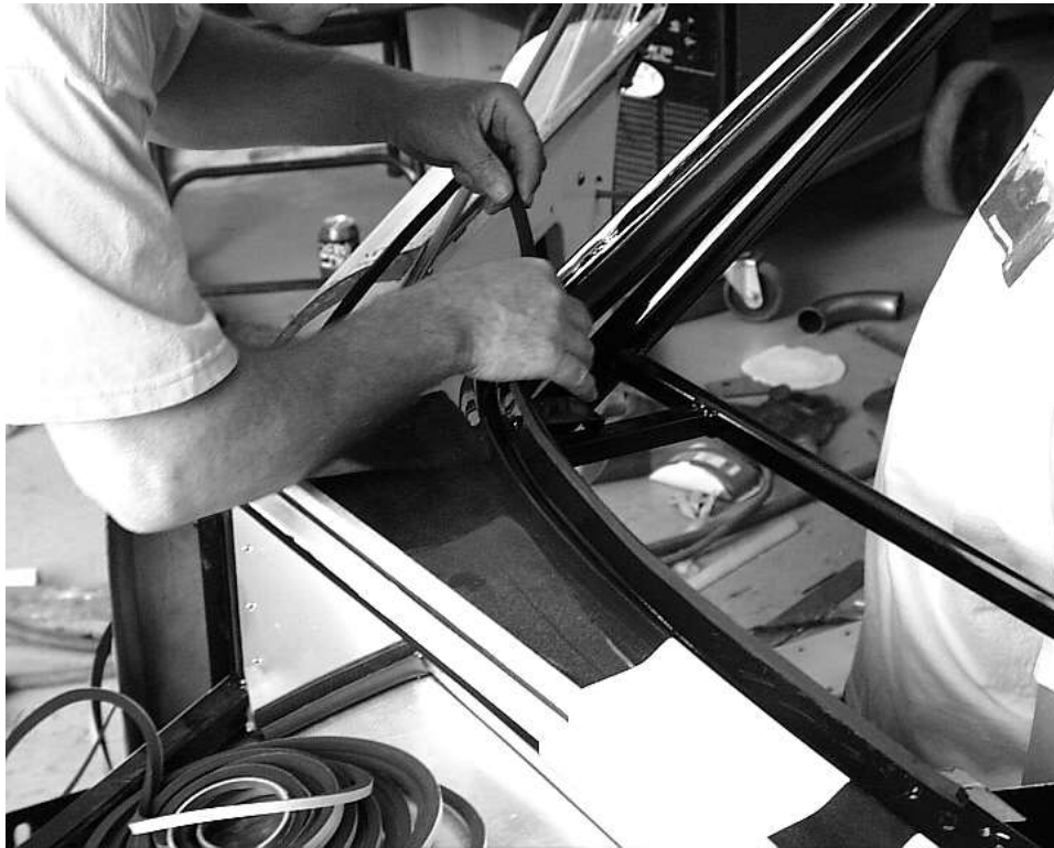
Sticking the foam dam to the windshield flange.
