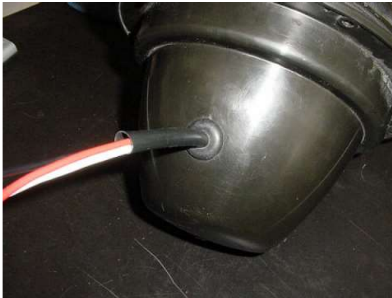
Pigtail wires and covering pulled through grommet.
