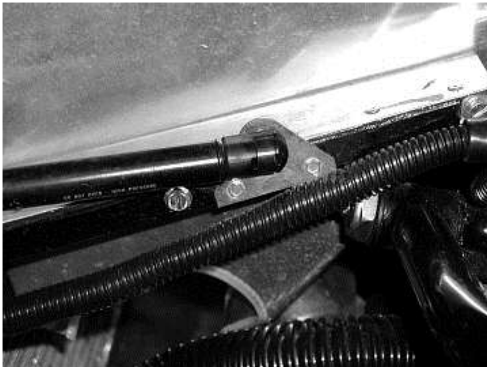
Nose strut mounted on frame.
