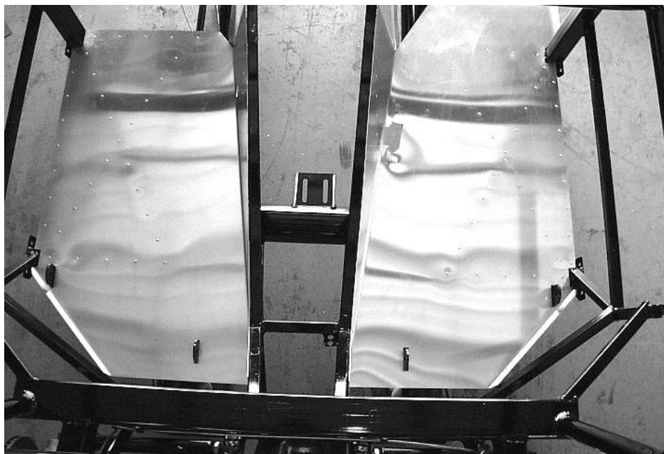
Cockpit floors riveted in position.
