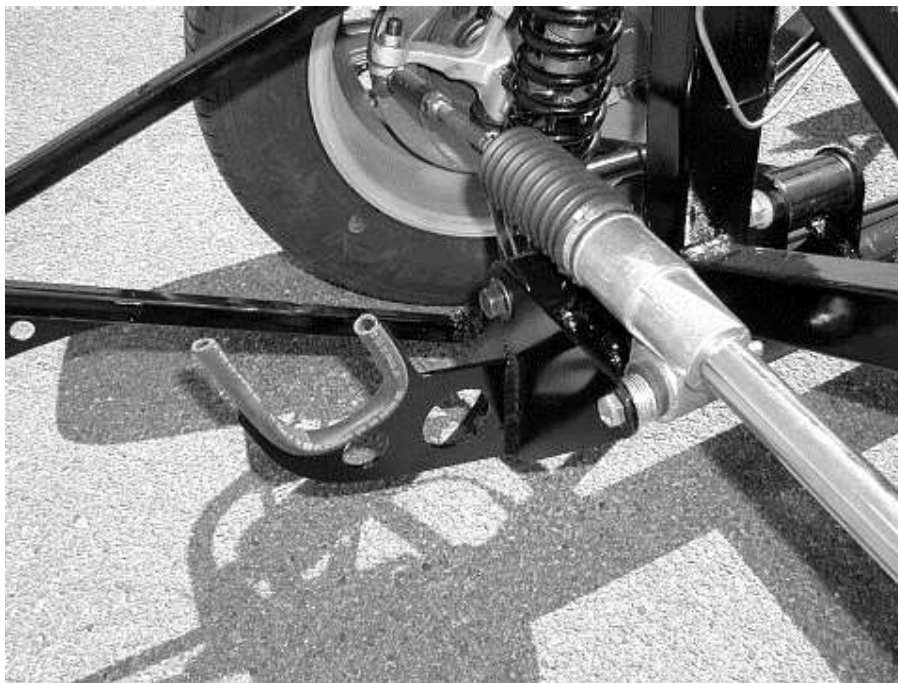
Lower radiator mount with fuel line pressed on.
