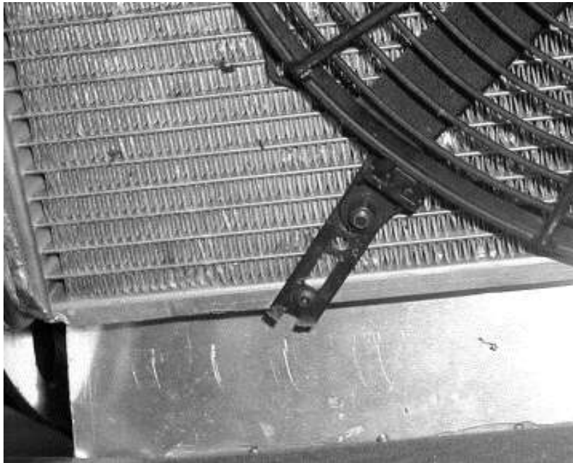
Lower fan mount before trimming.
