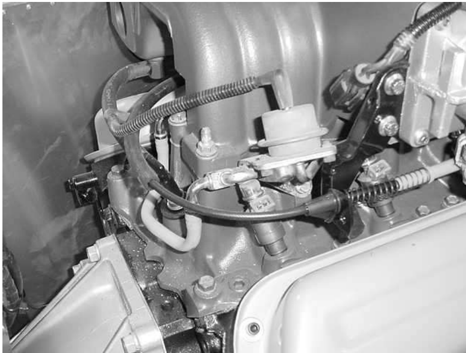
Accelerator cable attached to the throttle body.
