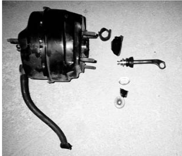
Power booster with the rod removed.
