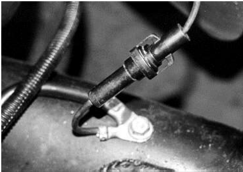
Computer ground near Master Cylinder.
