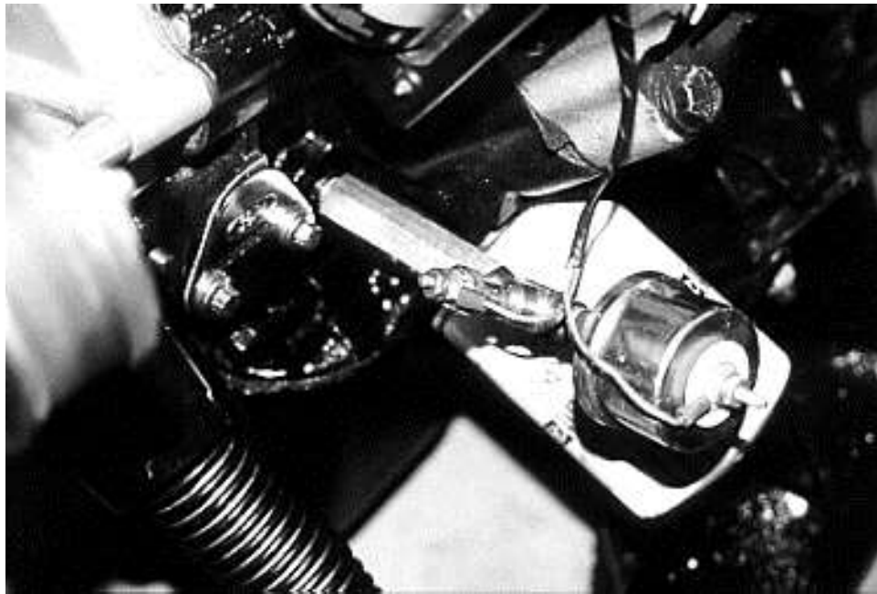
Oil Pressure and temperature senders mounted.
