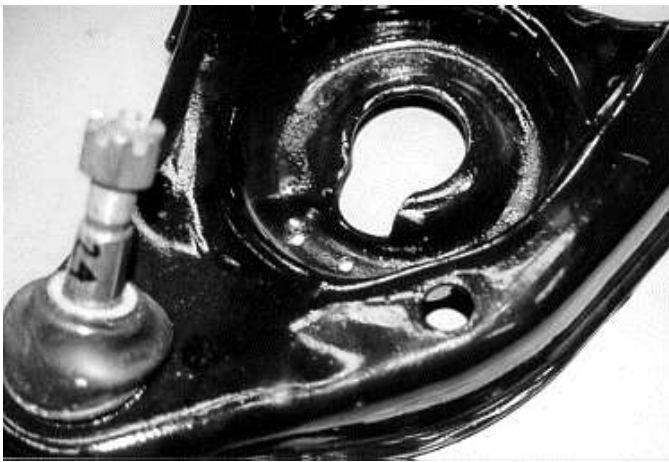
Section removed from front lower control arm.
