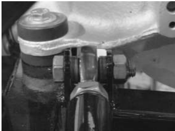
Alignment shims in place.
