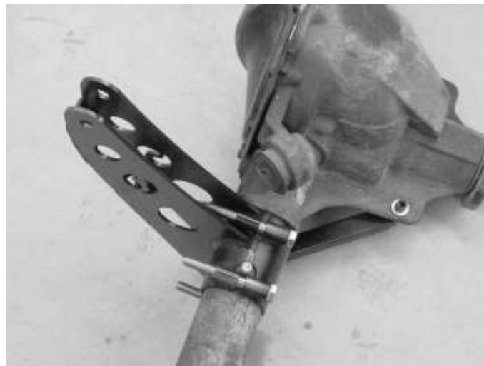
Upper axle mount attached to axle.
