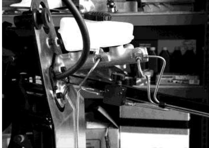
Master cylinder mounted and plumbed.
