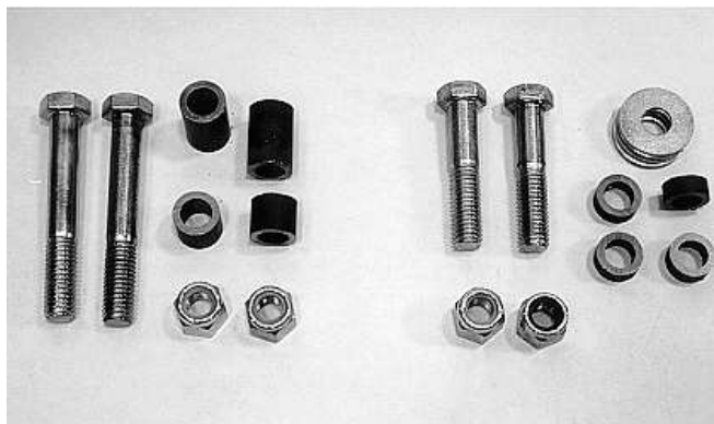
(Left) Lower shock-mounting fasteners/spacers. (Right) Upper shock mounting fasteners/spacers.
