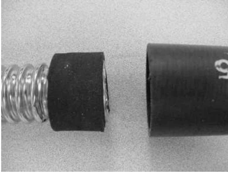
Corrugated hose with adapter hose slipped over the end.
