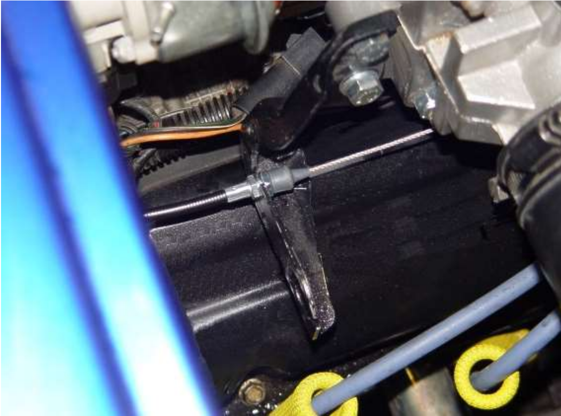
Accelerator cable attached to engine.
