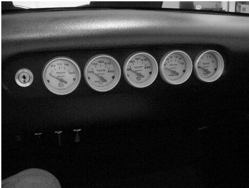
Optional ignition switch, Oil Pressure, Water Temp, Oil Temp, Volts, Fuel Gauges (Left to Right).
