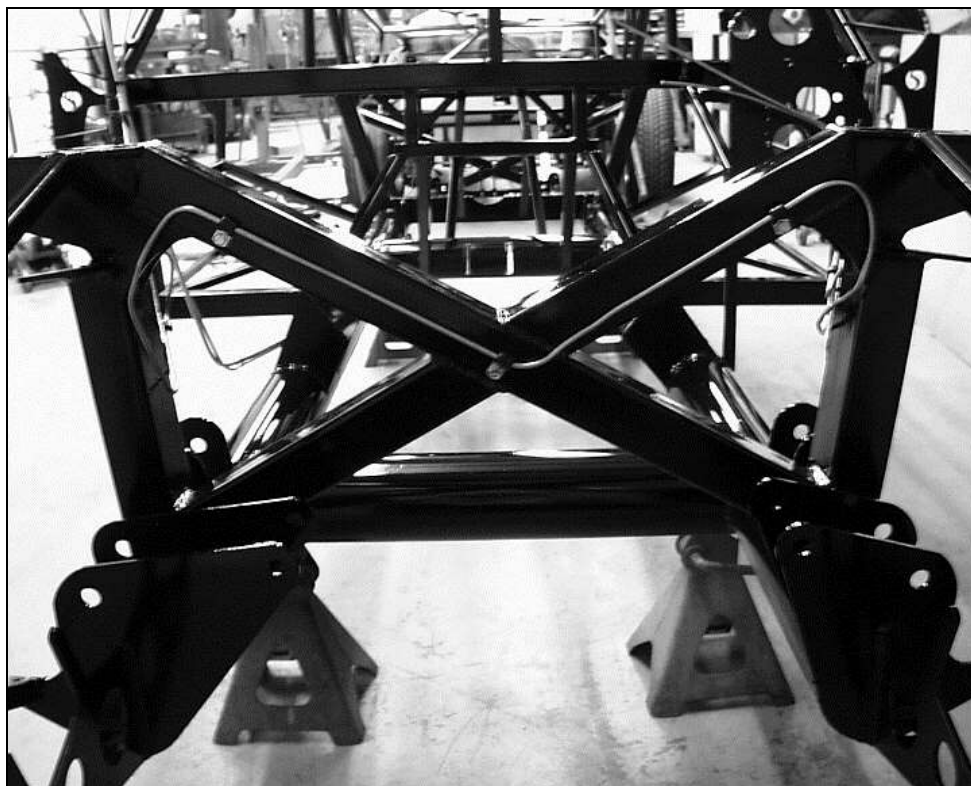
Brake line routing along frame X-member.
