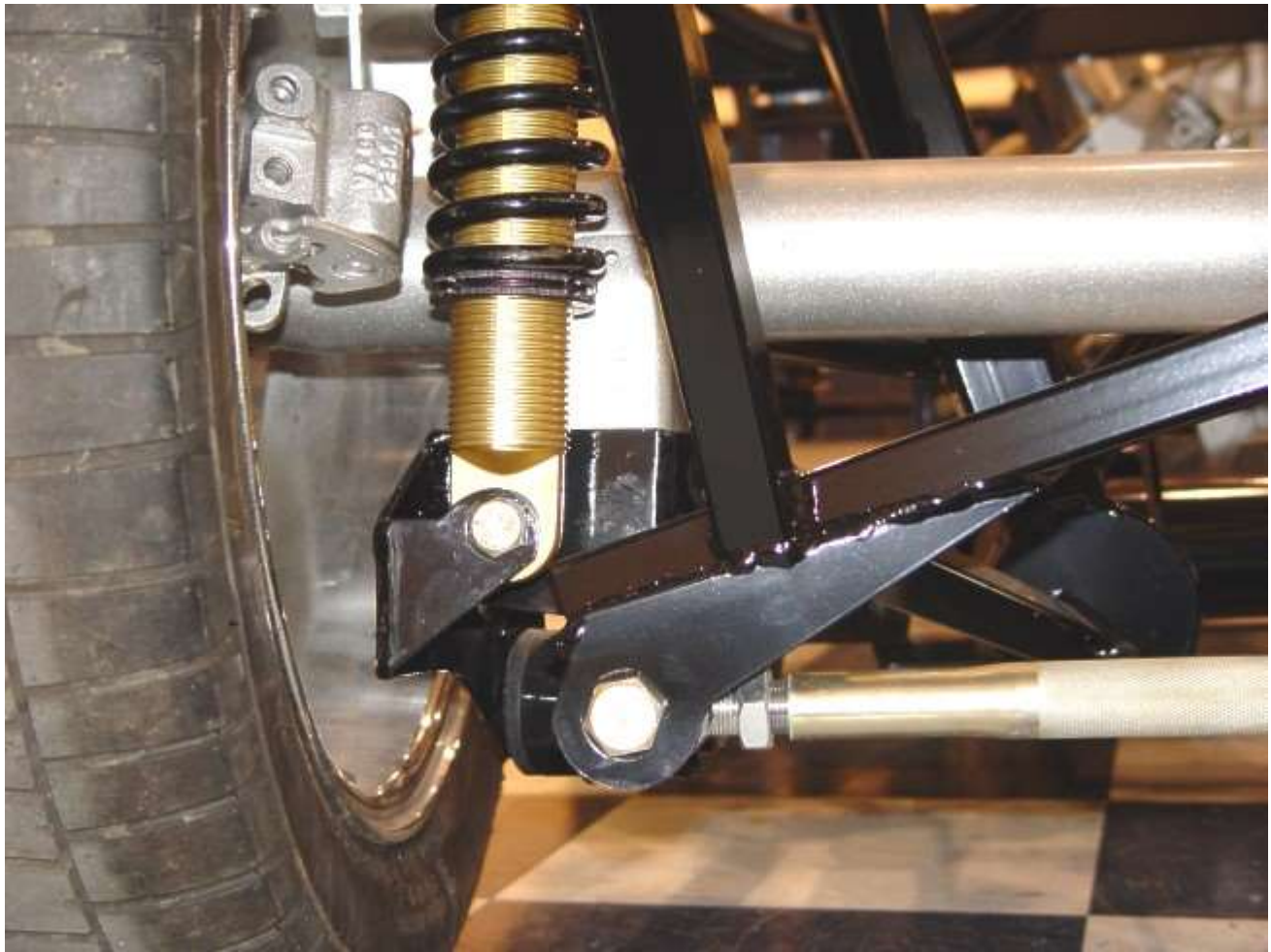
Rear traction lock bracket installed with rear coil-over and 3-link options.
