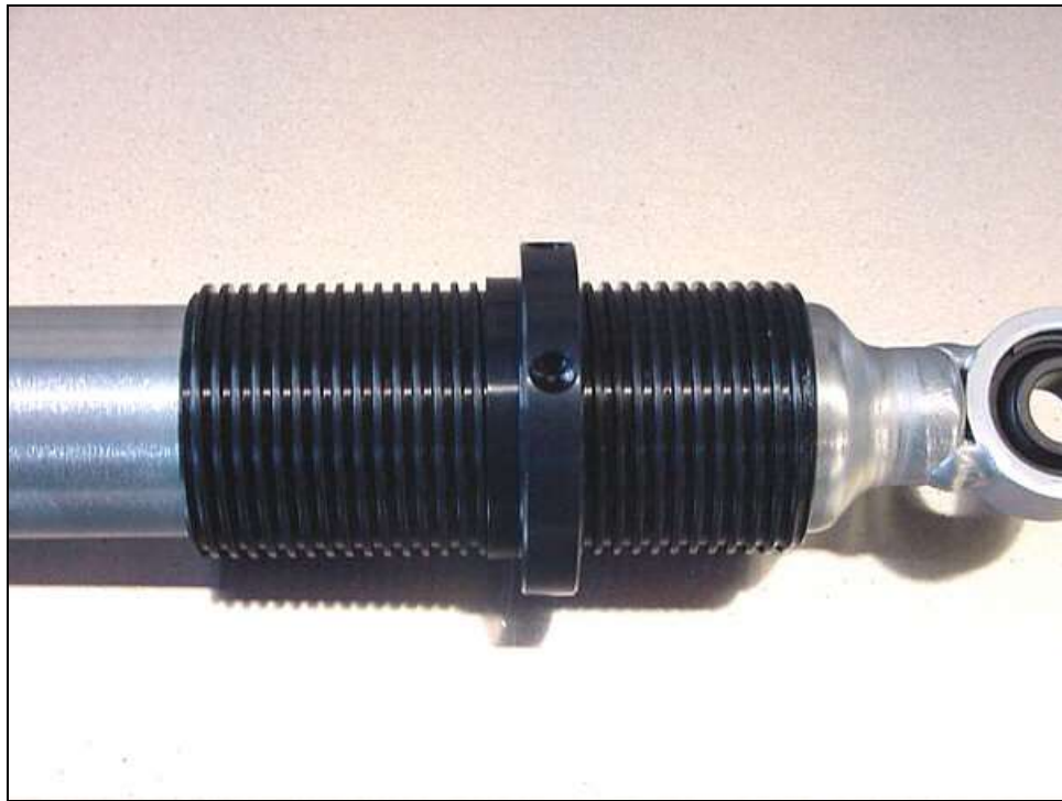
Threaded tube assembled on shock with spring seat screwed on correctly.
