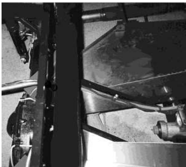
Battery cable routing.
