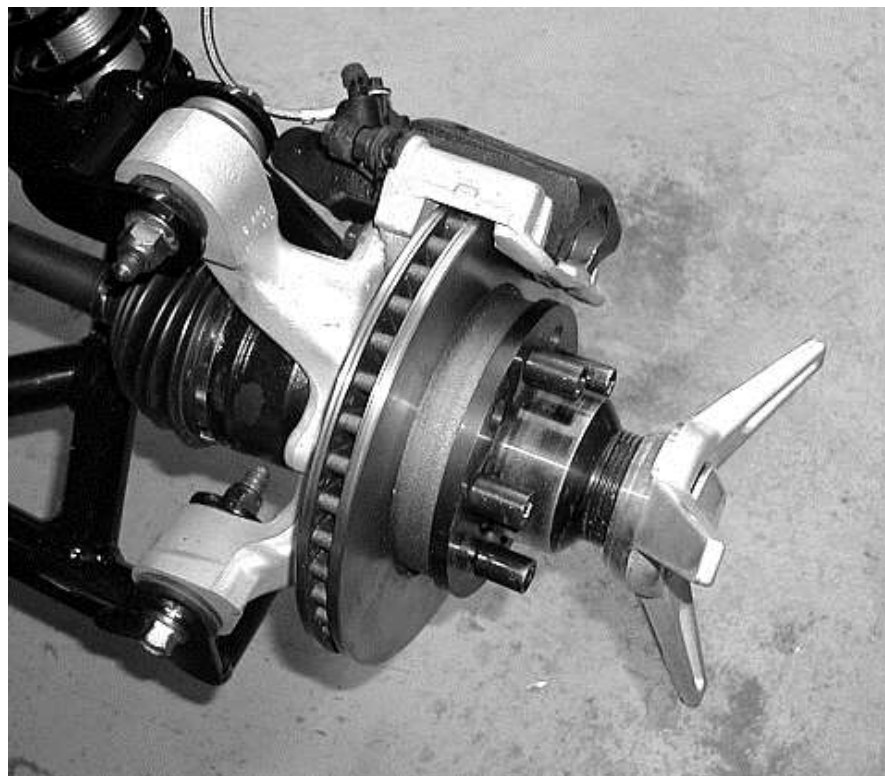
IRS spindle with knockoff adapter and spinner.
