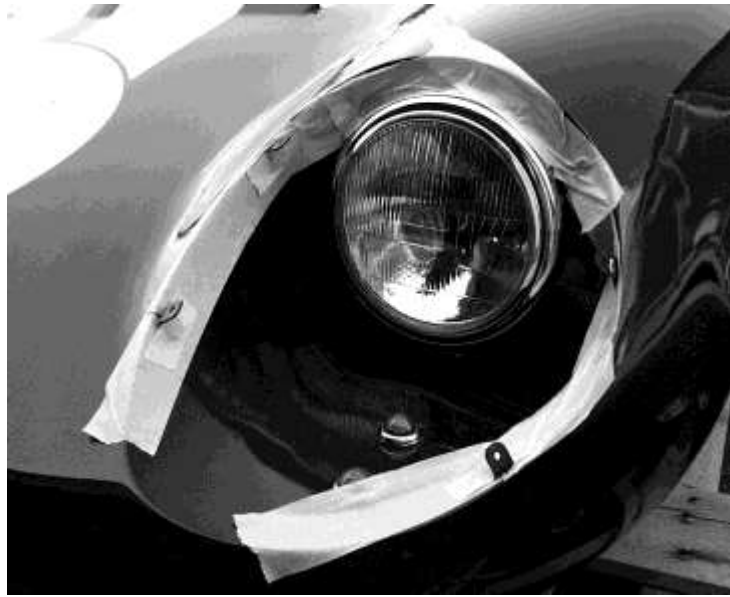
Mounting tabs taped to headlight bucket sides.
