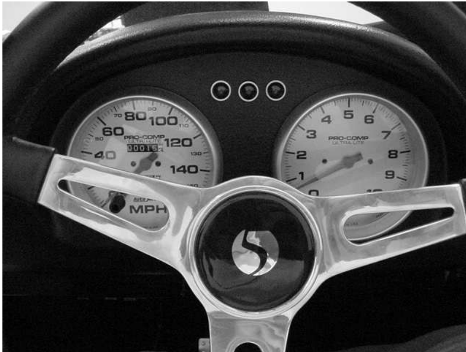
Speedometer and Tachometer mounted.
