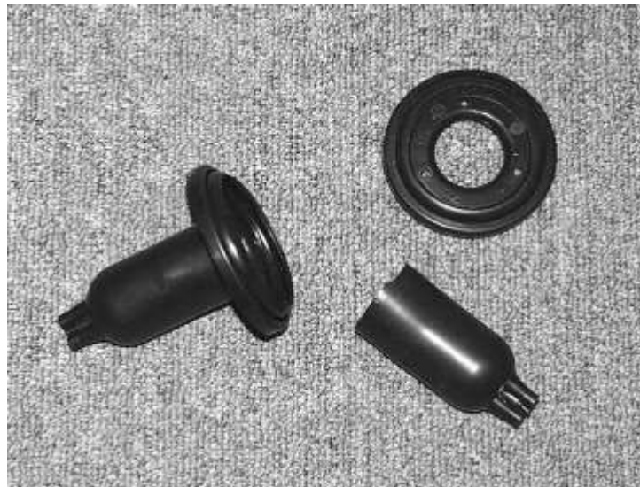
Cutting the protruding rubber seal.
