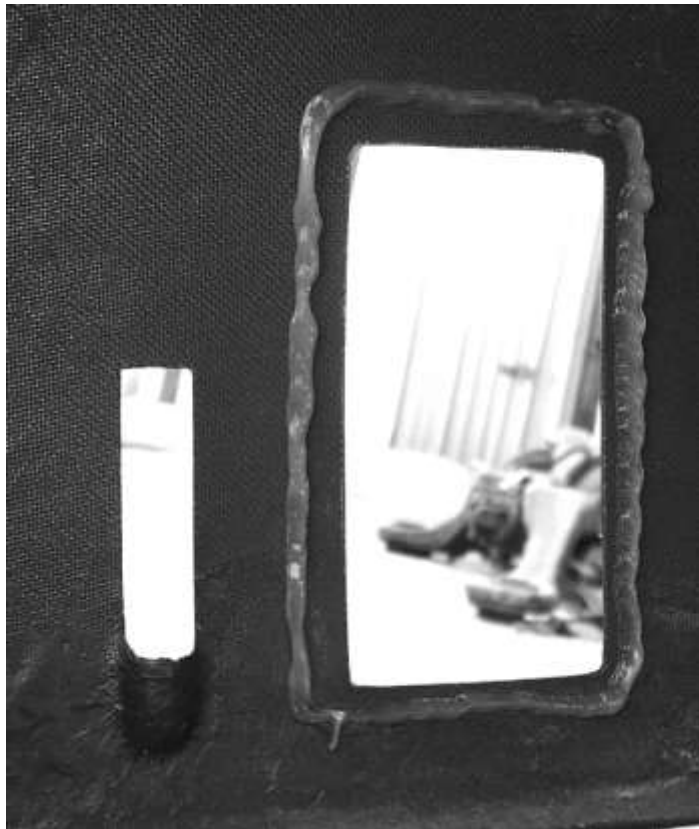
Apply silicone bead in place for the mesh screen.
