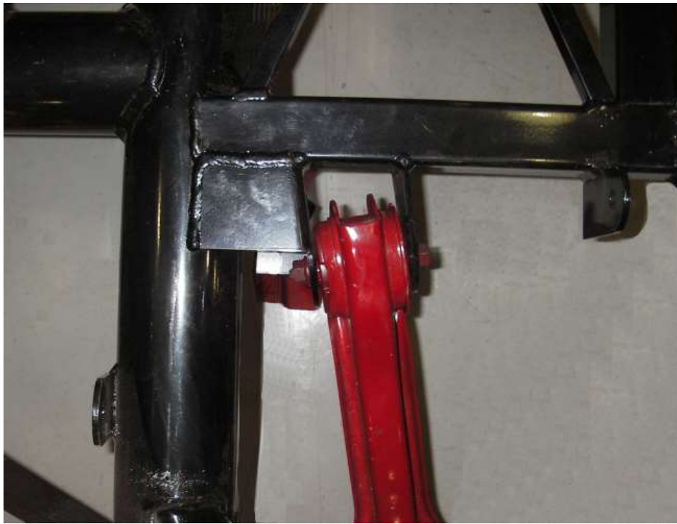
Passenger side stock rear lower control arm in the frame mount.
