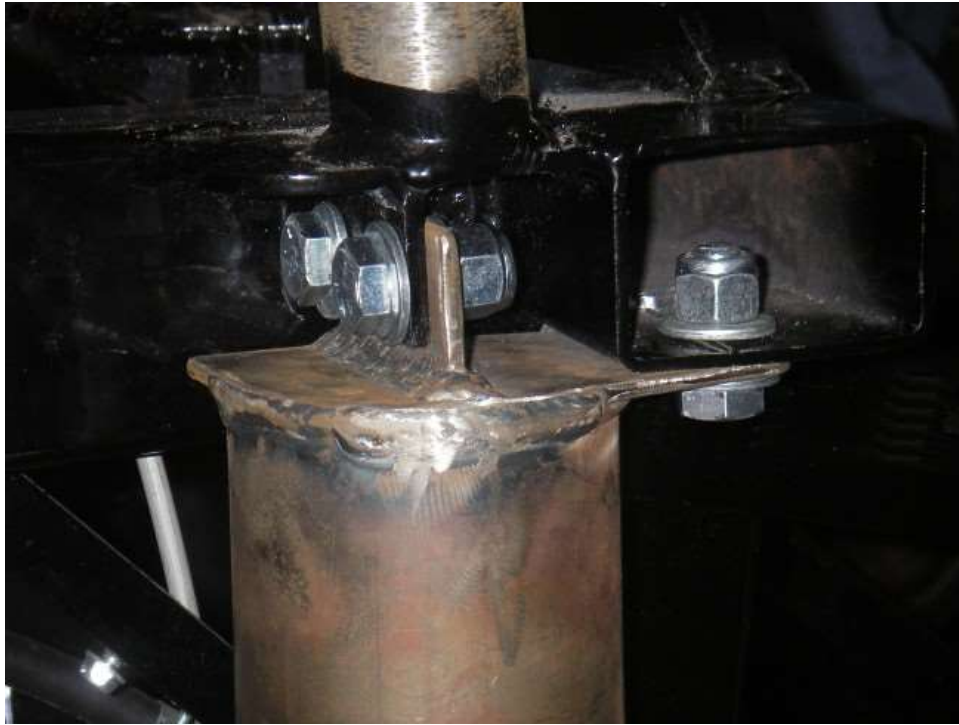
Spring perch mount bolted on frame.
