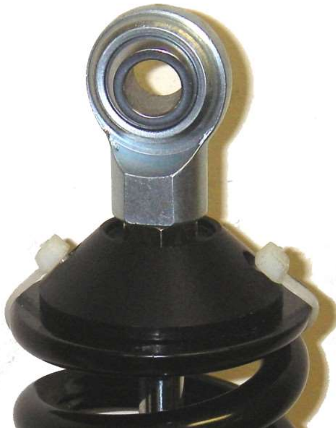
Spring hat attached to spring
