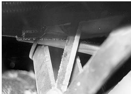
Old hose slit and covering new hose. Zip tied in place.
