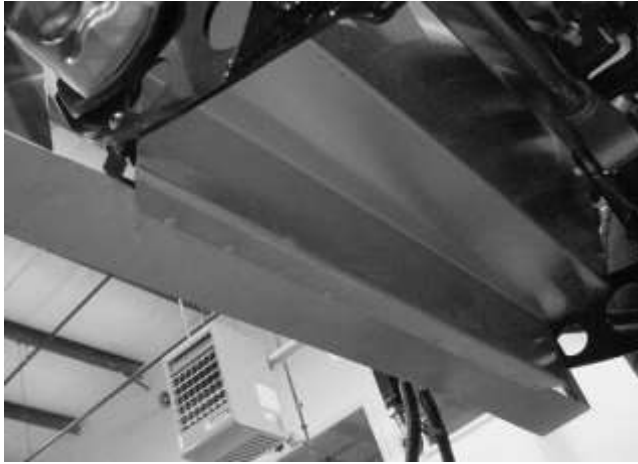
Large radiator duct mounted.
