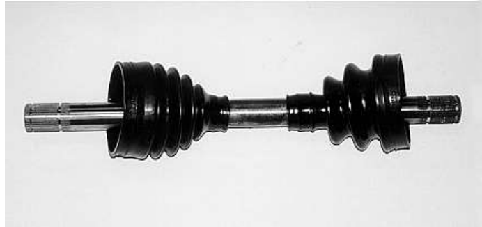
Boots pushed onto the new shaft
