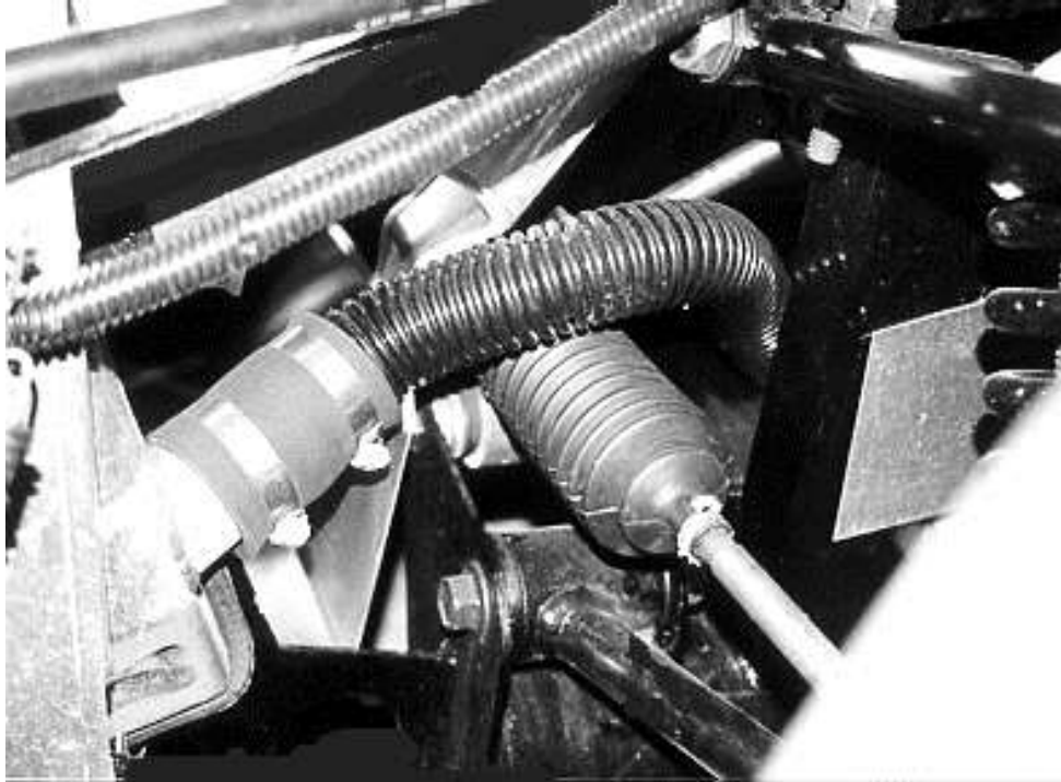
Lower radiator hose passing over the steering tie rod.
