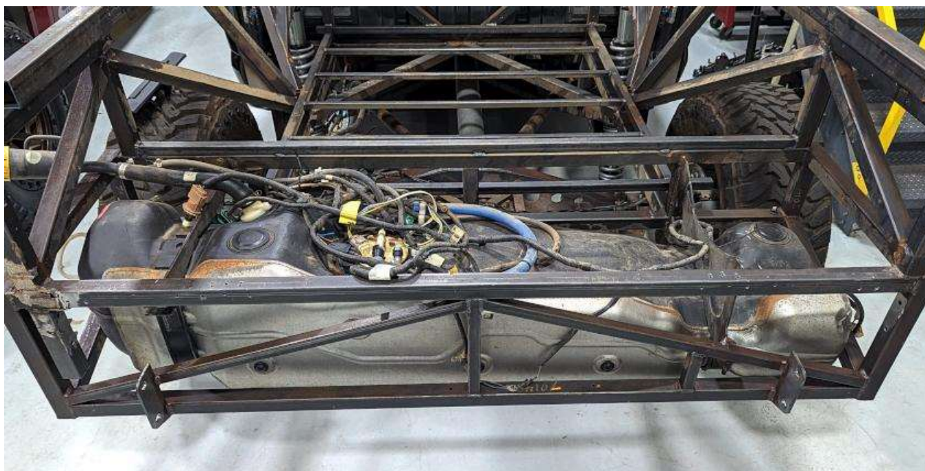
Raise the 26-gallon fuel tank into position with the fuel filler on the left side.
