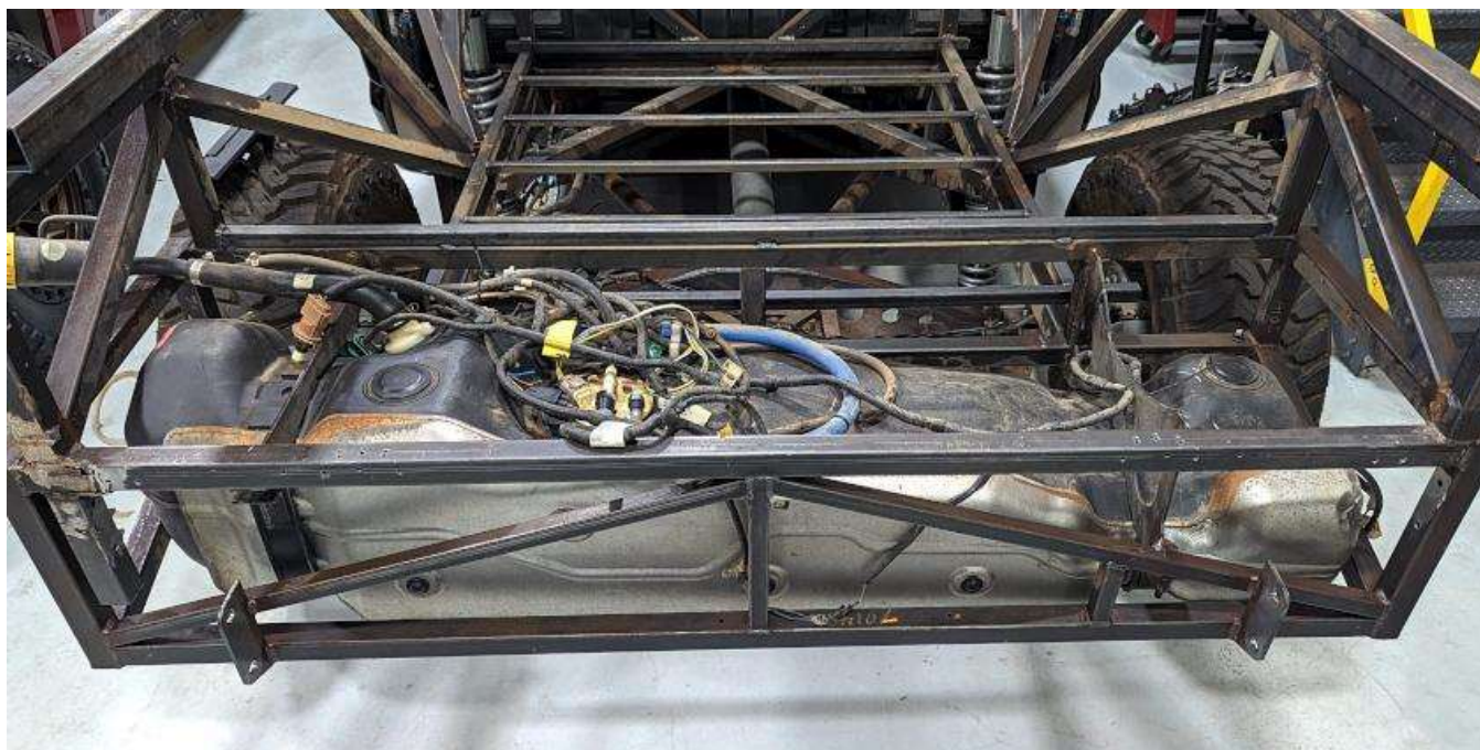
Raise the 26-gallon fuel tank into position with the fuel filler on the left side.
