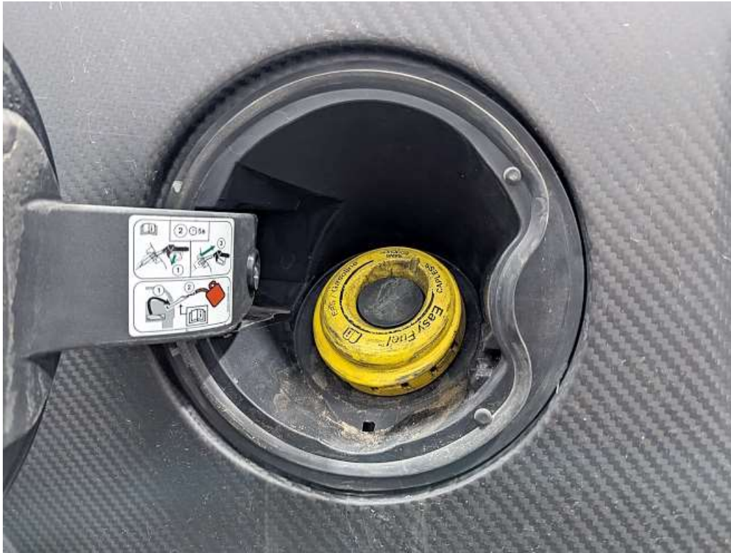
Filler neck in the filler cap.
