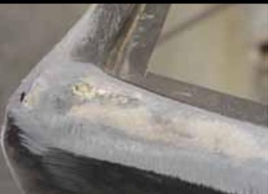
> Expect to find a few thin spots and air voids with the initial seam grinding. You need to rough these up so they'll provide some tooth for the filler material to adhere to, but there's no need to dig the hole any deeper than it is.
