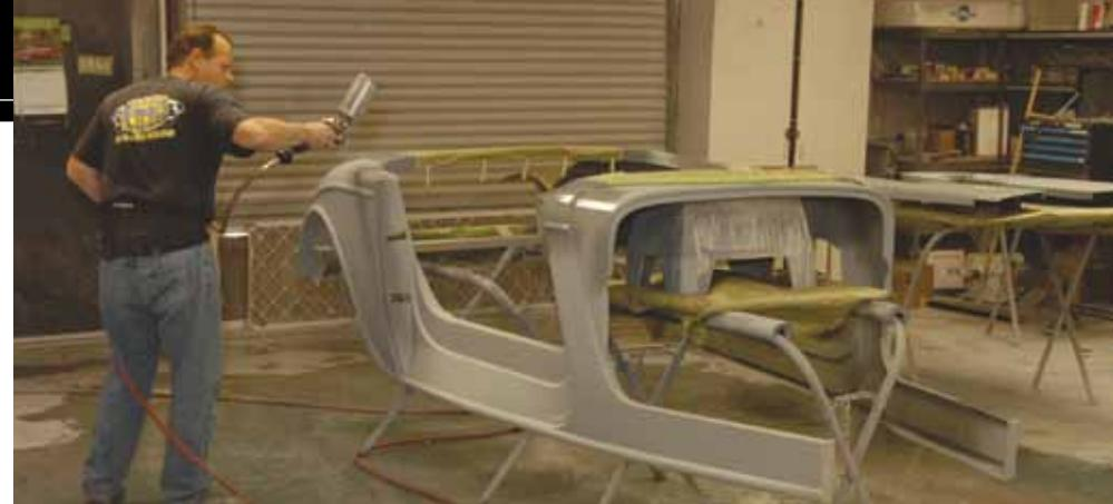
> Miller's final step is to spray black epoxy sealer over the feathered edges of the gloss-black paint. That's because the gloss paint is still fresh and sanding it can release solvents that will foul the matte black he'll be spraying in a few minutes.
