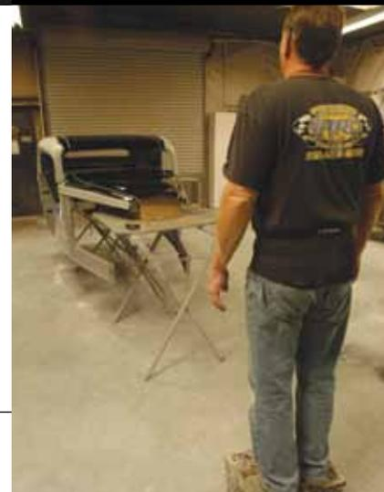
> "Tape twice and paint once" could be the two-tone painter's credo. No matter how much doodling and planning takes place on paper or a computer screen, being there when the tape lines go on is the only way to account for the complex interplay of body lines and paint breaks. This is the last time Miller can adjust his paint lines, so he gives the body a critical visual hose-down.
