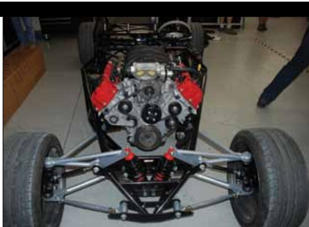
> The front suspension uses unequal-length control arms actuating inboard Koni coilovers mounted right behind the radiator.
