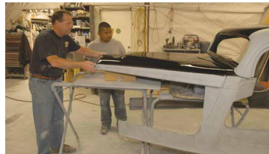
> Applying our two-tone gloss and matte-black scheme requires mocking the body a couple of times. Here Miller and Castillo carefully assemble the bodywork on stands, so the final step—applying the matte black—can be accurately laid out. It's worth noting the chassis was never at the paint shop, so all the lines and paint breaks were established like this. Set all panel gaps as carefully as possible for this step.
