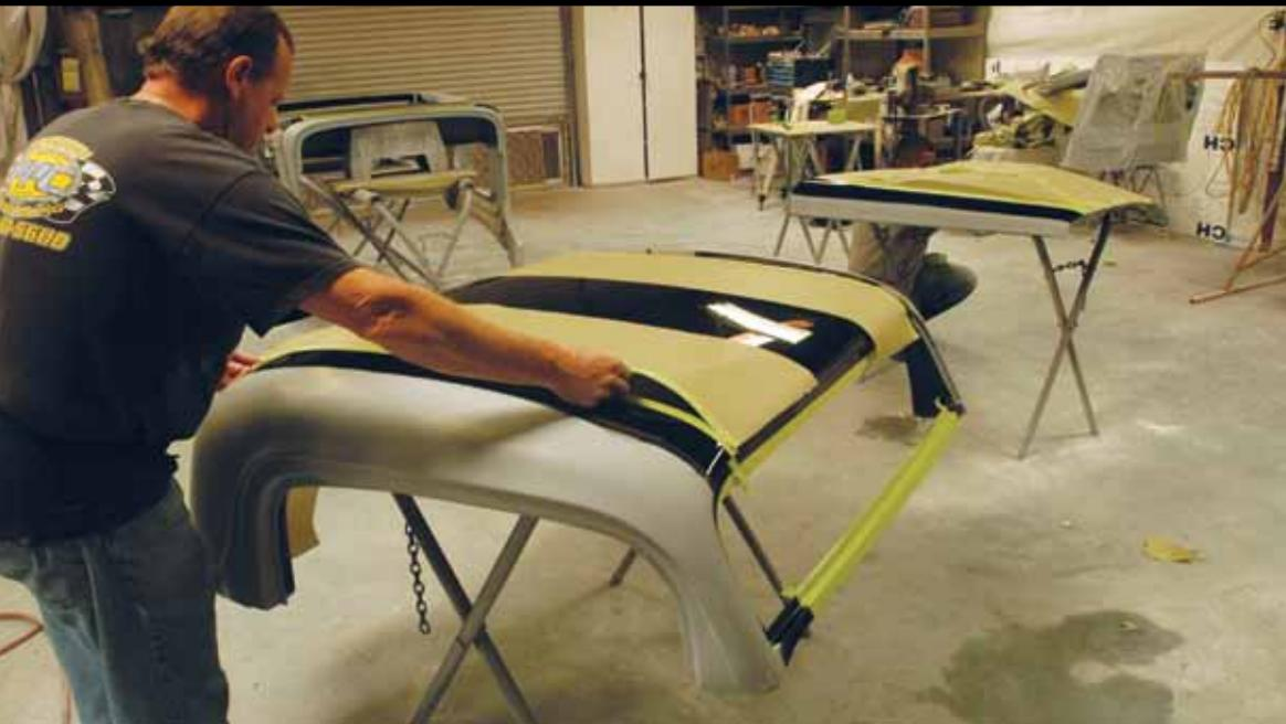
> With the break between matte and gloss black set, a 6-inch-or-wider secondary masking job goes on. This doubling up on masking paper over the edges of a finish paint coat keeps solvents from leaking through the paper and causing evil to the first finish coat below.
