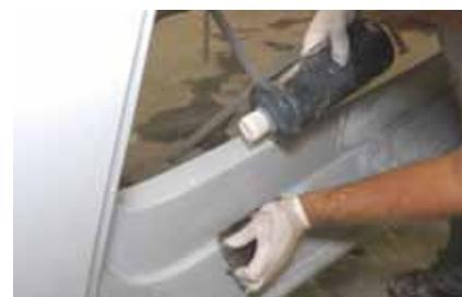
> For the final smoothing of the primed surface, wet-sand the entire body with 600-grit. This makes a wet mess, but flushing with water lets you see the work progressing. Getting the primer to a scratch-free, even, matte finish is the goal.
