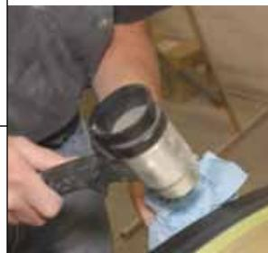
> Miller uses this nifty dryer to speed away residual water so he can get on with painting the '33. The dryer is just a venturi that augments the shop's compressed air with ambient air. It helps limit the number of towels that get wet and dirty drying the car and works fine for water-based paint jobs.
