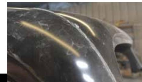
> Out of the box, the raw body panels are marked by mold parting lines. These are where the various sub-panels were joined to form a fender, or a roof panel in this case. They look hideous standing up in a jagged line, but they buzz off easily enough and are an unavoidable characteristic of fiberglass construction.
