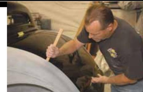
> With paint on the panels, this is obviously taking place later in the game, but getting the hinges on moving panels correctly aligned is part of checking body panel fit. Here, Miller uses a paint stir stick as his panel fit gauge. Typically, a bit of edge trimming of the door or lid sets the panel gaps equally around the opening. Nubs and resin globs are the typical offenders, but occasionally, slightly altering a door or lid edge is required. Quick grinding or sanding does the trick.
