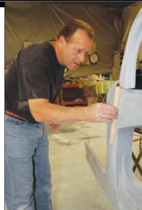
> Step one is to make sure the body panels fit the chassis and each other. A dry fit of the Factory Five kit uncovered no body panel issues, but Jeff Miller did reshape the trunk hinges for more clearance.
