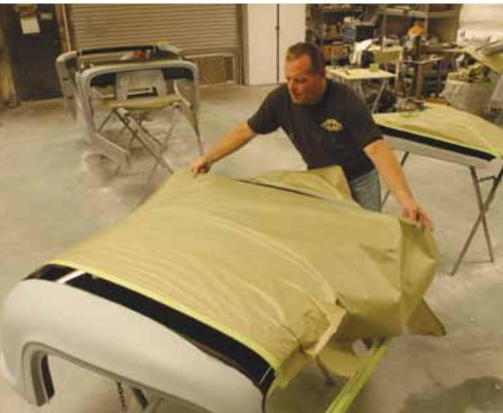
> With the doubled-edge masking paper in place, the general run of masking paper is applied. On smaller areas, such as the narrow edges of the window frame, Miller skips the paper and tapes the whole area. Getting the edges down firmly is important to avoid paint leaks.
