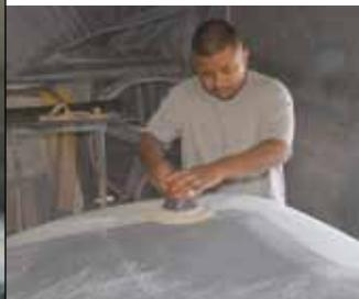
> Now the filler is made smooth using a double-action sander and 80-grit paper. The sander is run along all the filled seams to get them generally smooth, and then the entire panel is roughed with the same 80-grit. Make sure the filler is smoothly feathered at its edges as Castillo is doing here.
