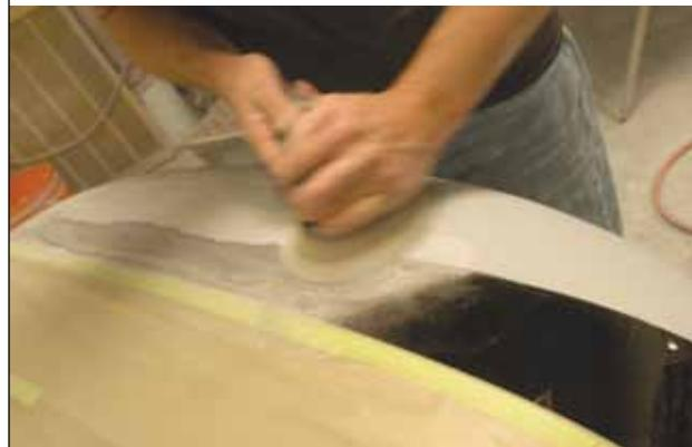
> Lap joints are for roofers; painters always need to feather any point where sprayed layers join or the hard line will show through the finished paint. Miller does this dry with the double-action sander and 500-grit paper. Be very careful not to brush the tape with the sander or paint will definitely leak through, causing a wavy edge. It's best to stay an inch away from the tape.
