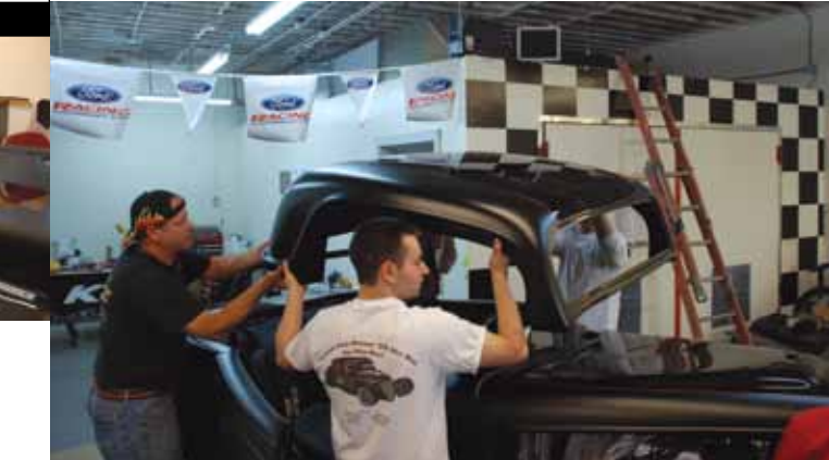
> The roof was lowered into place and bolted down. We doubt we'll ever remove it since it looks too cool installed. You can see part of the rollbar. The kit comes with double-hoop bars, à la Cobra. But with the roof in place, that would look weird, so we converted it to a single bar the width of the interior.
