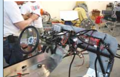
> Some of the aluminum panels were installed before the body went on and some afterward. Cleco pins are a brilliant way to hold them in place to make sure all the holes are correct and everything lines up. This photo also shows how the pedal box was mounted. Notice the hanging Wilwood pedal and three master cylinders (two for brakes, one for the clutch). The trick reservoirs mounted in front of them are an LK Motorsports setup, and once the body is mounted, they're accessible from a removable panel on the cowl.
