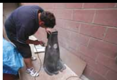
> Mark Dougherty prepped the fiberglass transmission tunnel to clear the trans.
