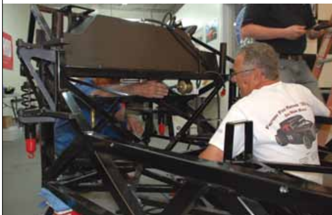
> The front suspension is the first area of attack. The kit uses inboard-mounted Koni coilover shocks mounted just behind the radiator.
