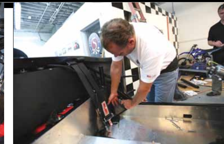
> Miller installed the door hinges and doors. Five-point Simpson harnesses are included for both sides and attach to a chassis mount before the rear bulkhead and seats go in.
