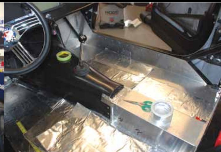
> The stainless steel mufflers sit right under the seats, so we covered the floor with Damplifier Pro insulation.
