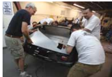
> With the body mounted, the remaining trunk panels were installed. The kit includes pre-cut carpet to cover all the aluminum panels.
