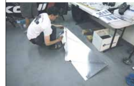
> There are quite a few aluminum panels for the floor, trunk, and other areas. They are precut to fit, but you still have to drill the mounting holes in the panels and the frame.
