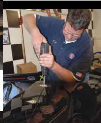
> The roof is held on with about 10 bolts and Rivnuts and is removable. Here, Dougherty drills the cowl for the Rivnuts.
