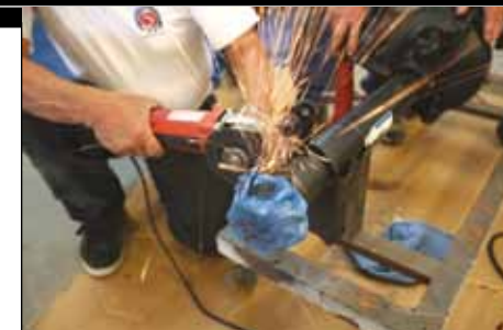
> Some of the stock rearend brackets were not needed and were removed.
