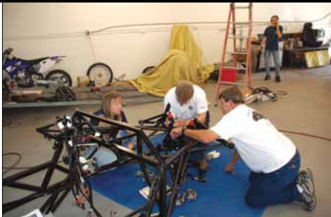
> The front suspension is the first area of attack. The kit uses inboard-mounted Koni coilover shocks mounted just behind the radiator.
