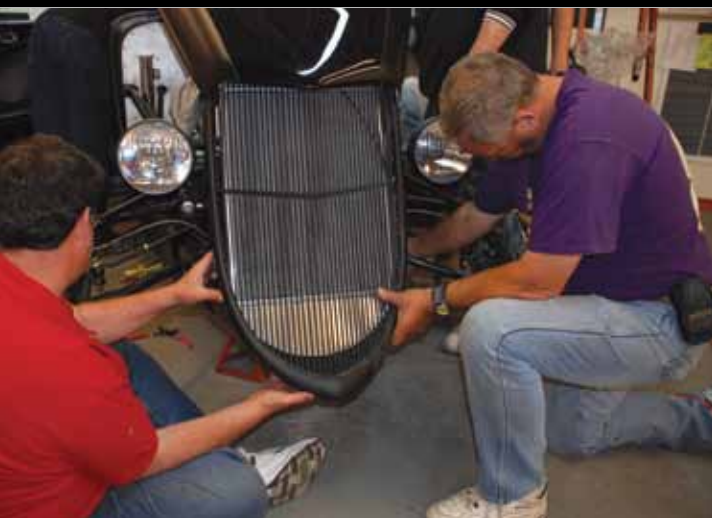
> After assembling the grille/radiator/fan assembly, it was installed. The kit comes with hoses and everything else needed.
