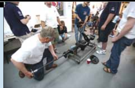
> The kit is designed to use a Ford 8.8-inch rearend from a Fox or SN-95 Mustang, and you can choose from a stock-style four-link or a more race-oriented three-link suspension. This car uses the three-link, and we loaded the 8.8 with 3.73:1 gears. That big bracket bolted to the housing is the upper link mount.
