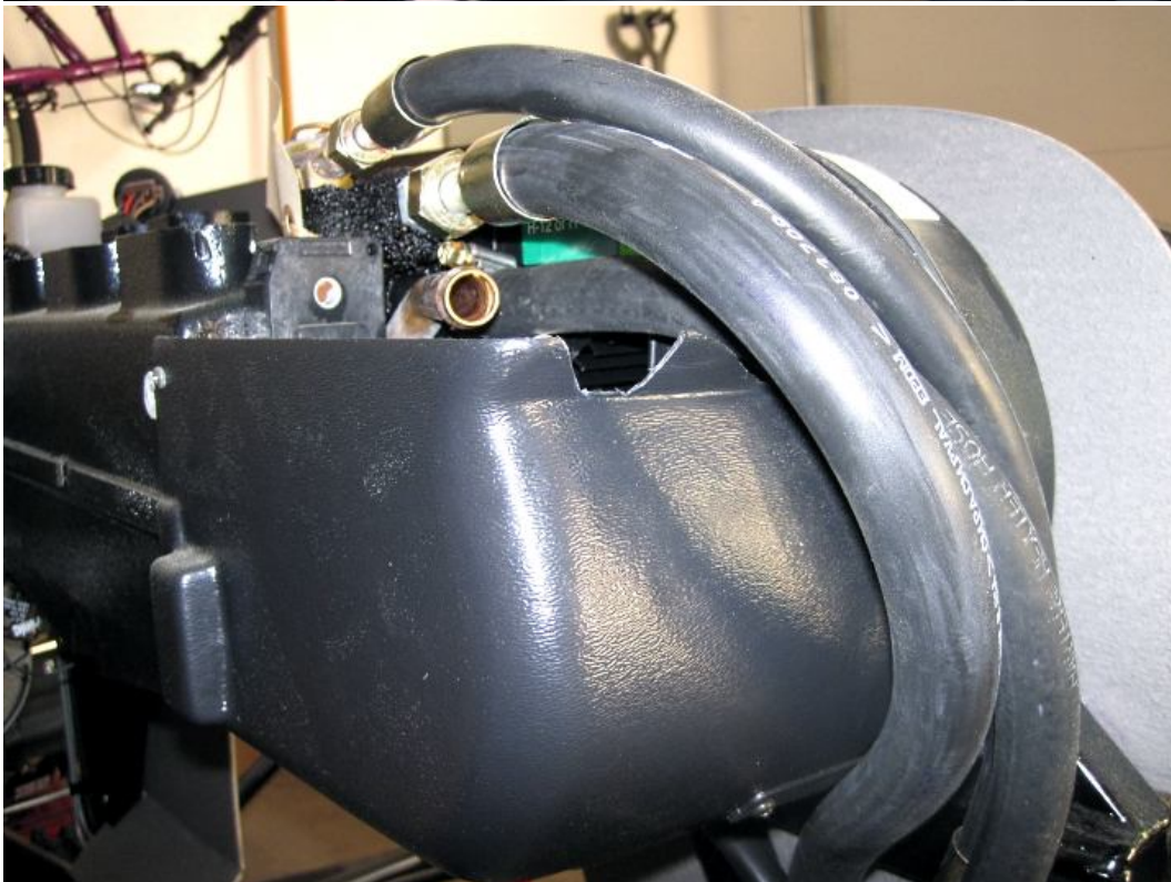
Cut the plastic cover again where the hose will touch it.
