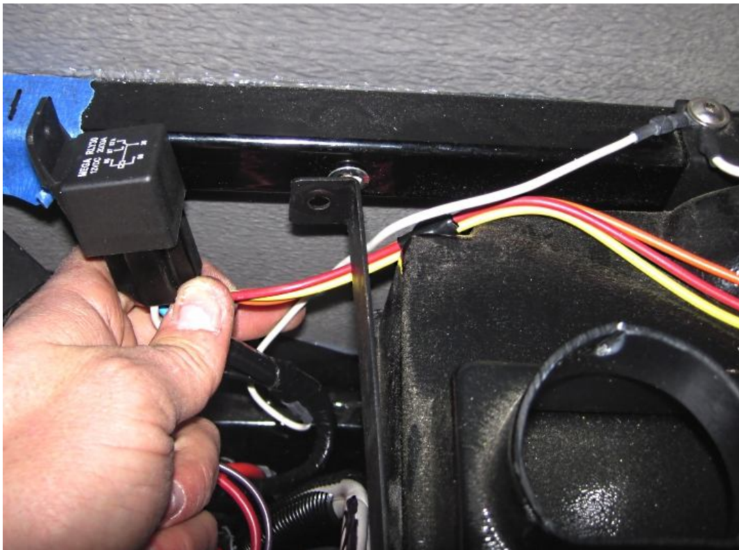
Undo the left evaporator screw and slide the relay wires under the mount.
