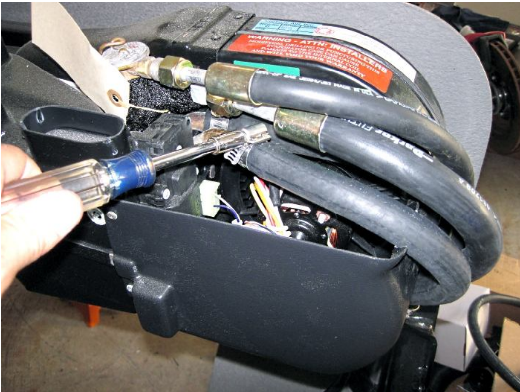
Attach the second heater hose to the heater core with a hose clamp and a \frac{5}{16} " socket.
