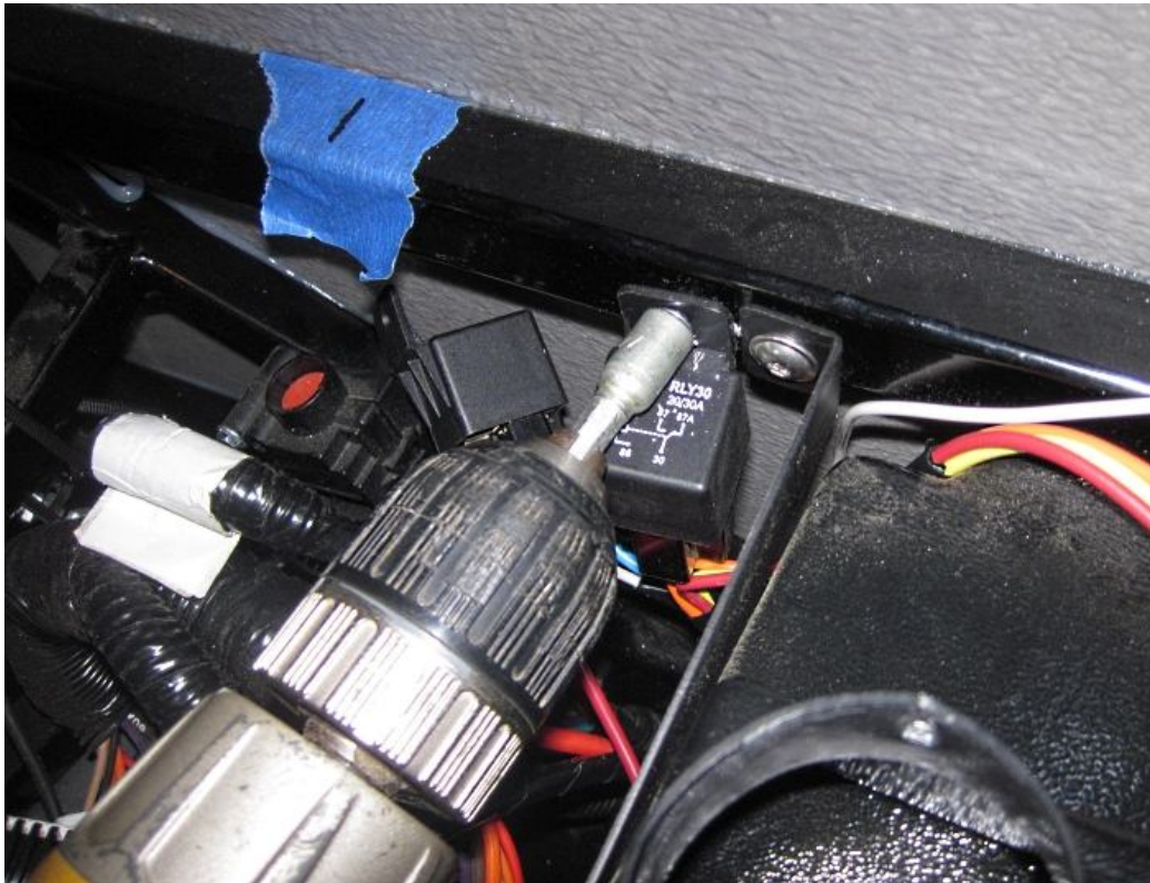
Reattach the mount screw.
