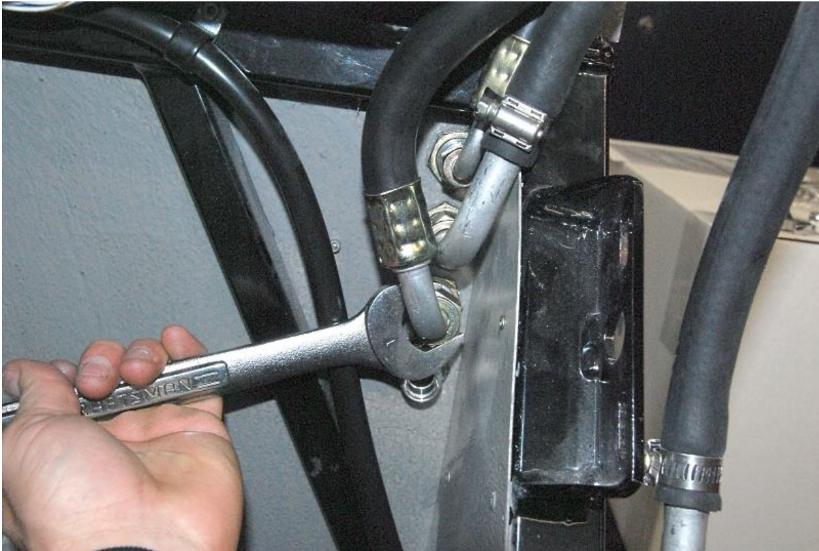
Screw on the third inside A/C fitting by hand then tighten using a 1" wrench.
