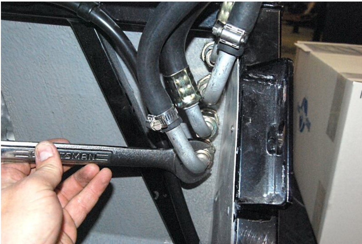
Screw on the bottom inside heater fitting by hand then tighten using a 1" wrench.
