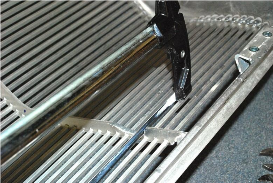
Use a saw or grinder to remove the material from the crossbar.
