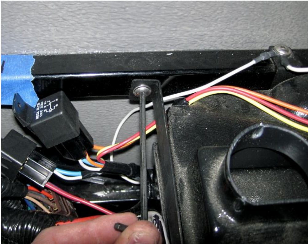
Reattach the mount screw.
