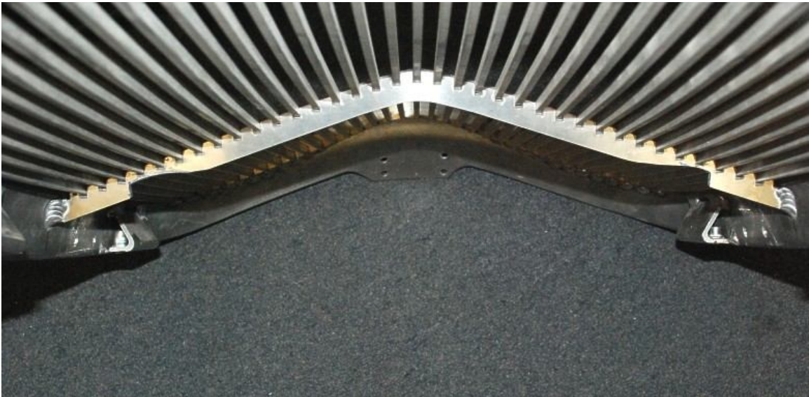
Use a saw or grinder to remove the material from the crossbar.
