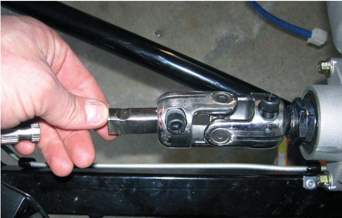
Insert the small \frac{3}{4} " DD shaft into the joint on the front of the electric steering unit.
