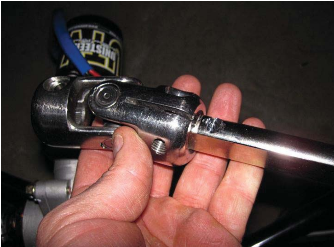
Remove the locking bolt from the remaining splined joint with a 6mm hex key and insert the 15 \frac{1}{16} " middle steering shaft into the joint.
