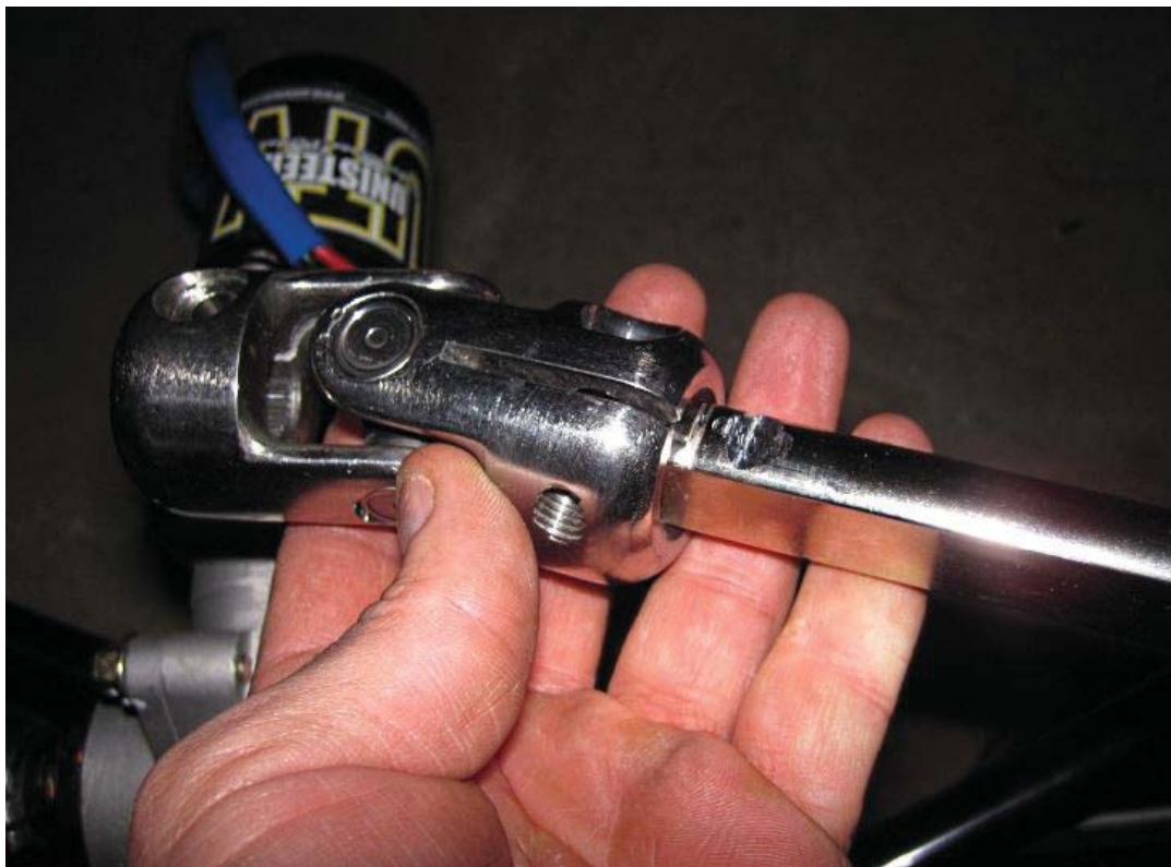
Remove the splined joint from the electric steering unit and push it onto the shaft.
