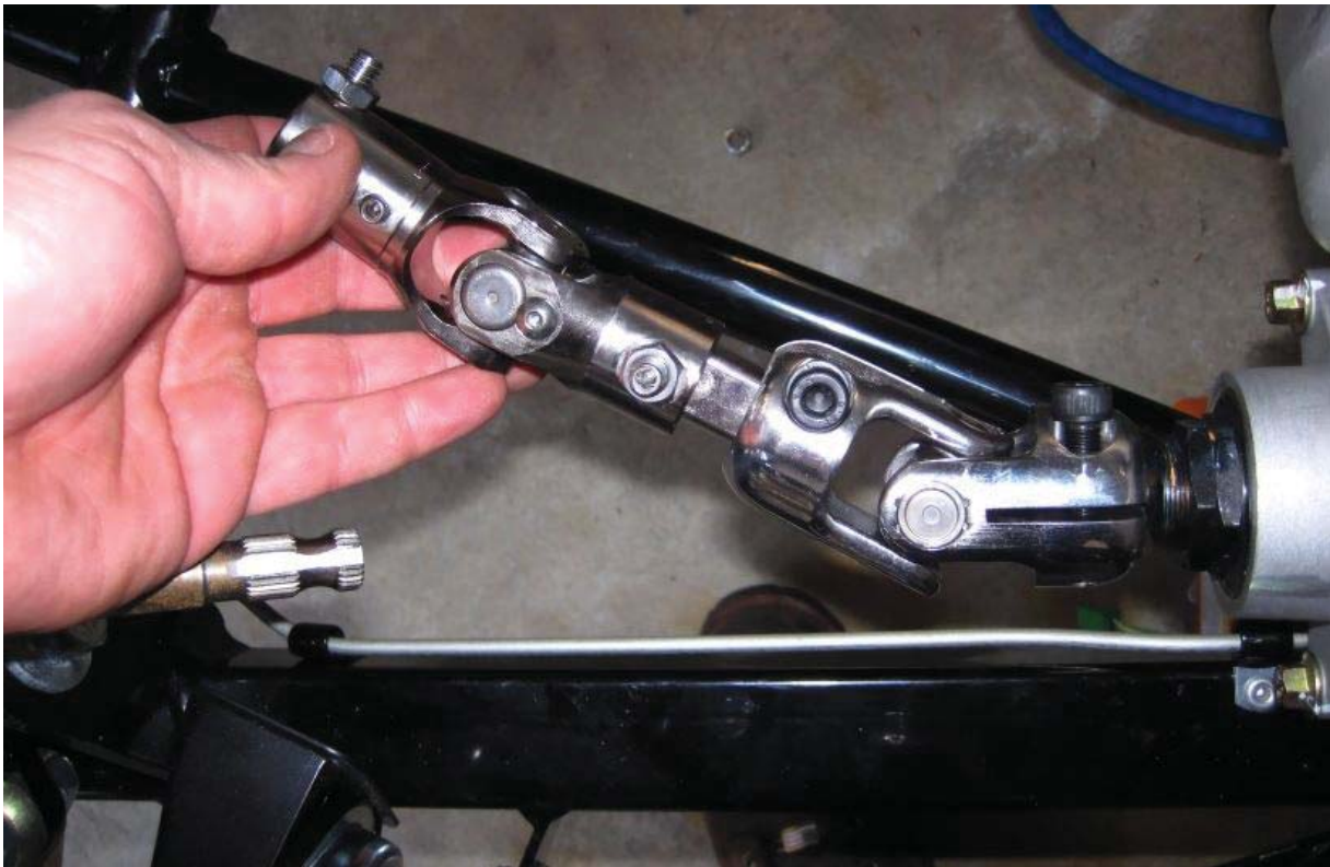
Insert the \frac{3}{4} " DD shaft into the steering rack joint.
