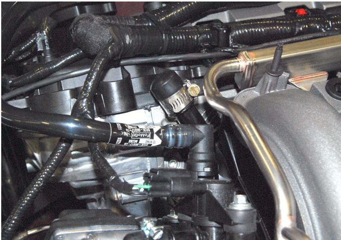
Cap and hose clamp the 3/4" coolant.
