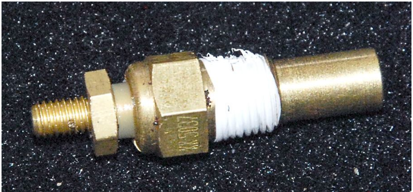
Put Teflon tape on the sending unit.
