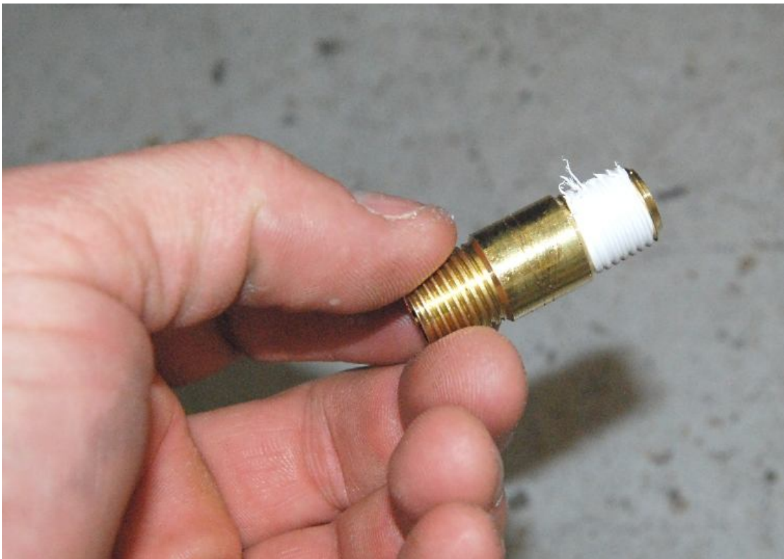
Put Teflon tape on the 1.50" NPT tube.
