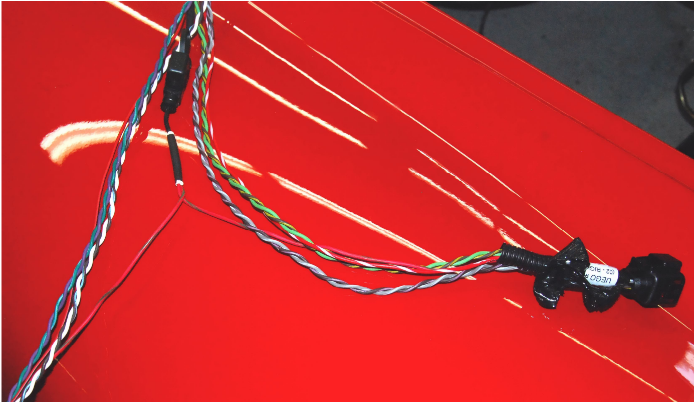
Locate the red/black power wire junction between the two O 2 sensor plugs.
