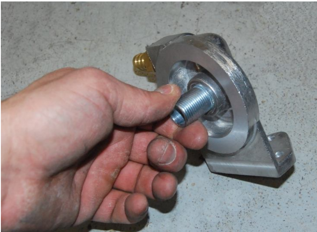
Screw the threaded nipple into the relocater.
