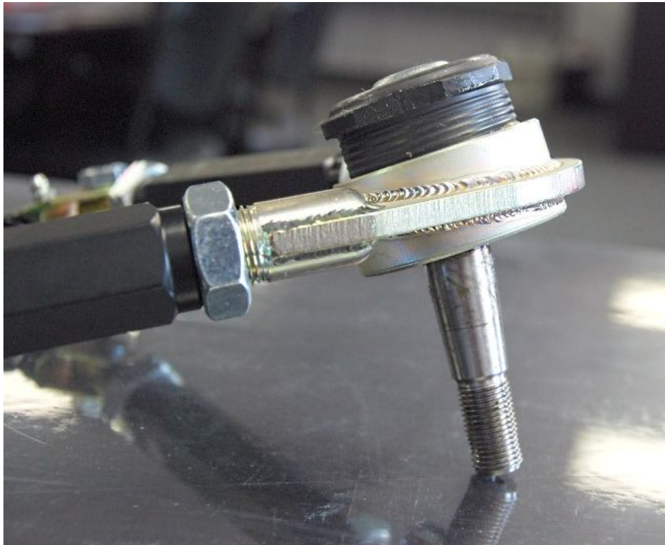
Screw the upper ball joints into the control arms so that the balljoint angles out on the bottom
