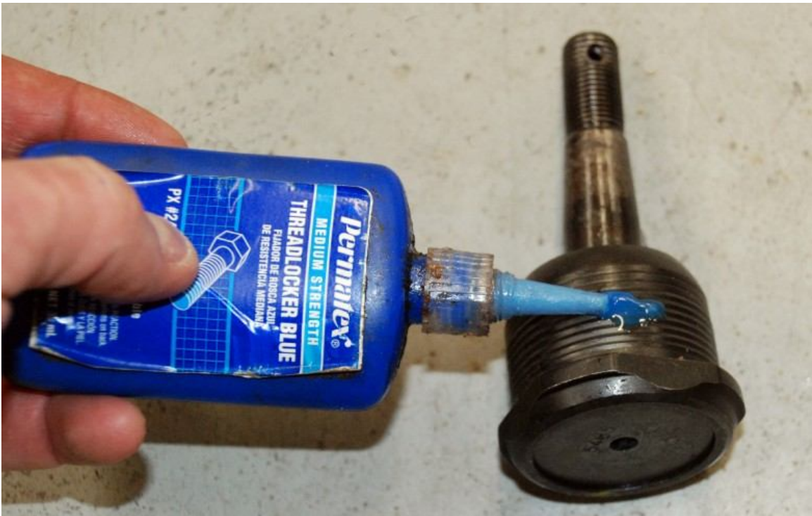
Put thread locker on the upper balljoint threads.
