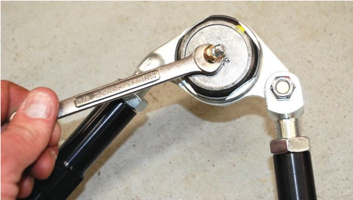
Screw the grease fittings in to the ball joints and tighten with a \frac{3}{8} " wrench.
