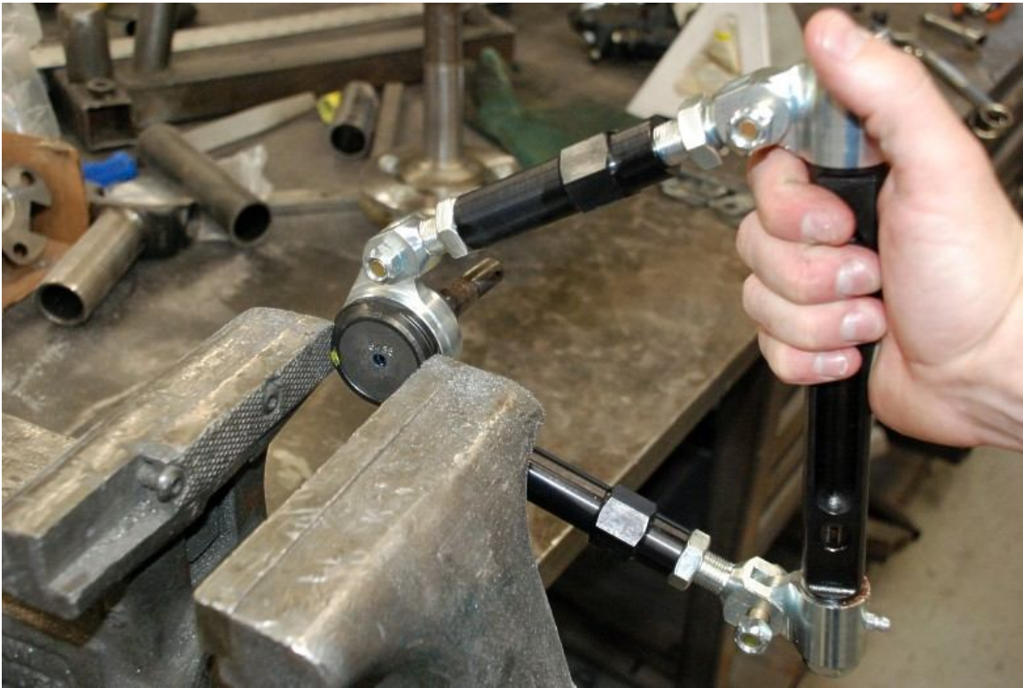
Tighten the balljoint using the arm for leverage with a Vice holding the ball joint.
