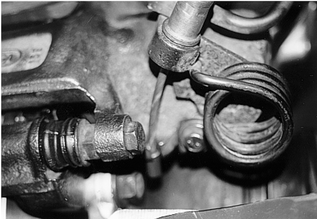
E-brake cable holder on caliper modified to fit cable
