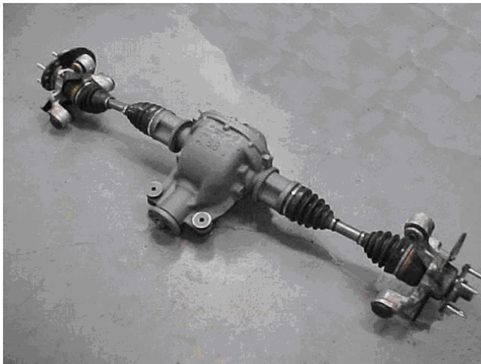
Donor fasteners needed: (Upper) Spindle attaching bolts. (Lower left) Center Section front mounts. (Lower right) Center Section rear mount bolts.
