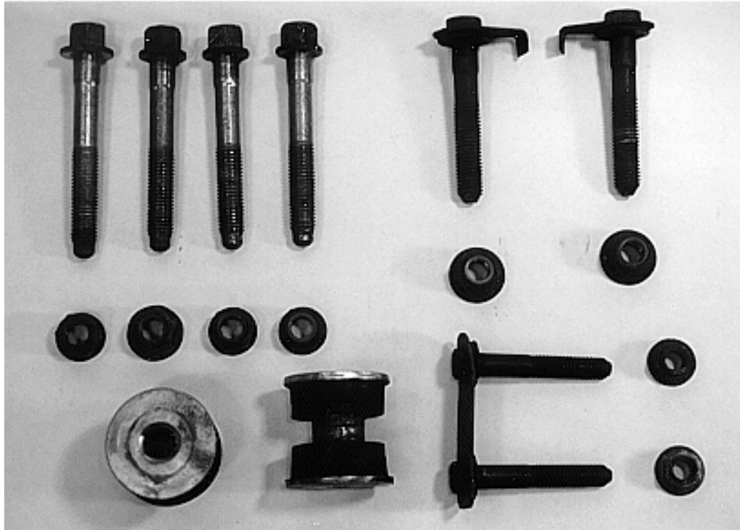
Donor fasteners needed: (Upper) Spindle attaching bolts. (Lower left) Center Section front mounts. (Lower right) Center Section rear mount bolts.
