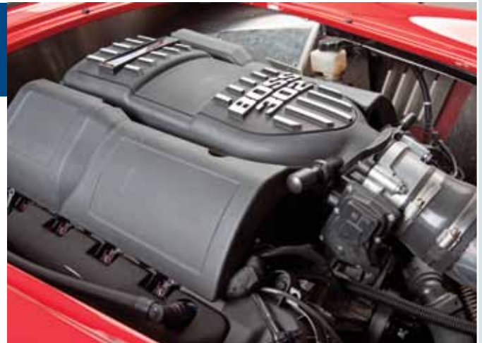
The Summit 5.0L Coyote combo ships with the production intake manifold and plastic engine "halo" cover. However, Dave Smith, President of FFR wanted a little more rpm for his personal Mk4 Roadster and upgraded his Coyote build with a Boss 302 composite intake manifold and matching injector/wiring covers.
