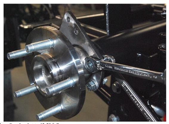
Torque the caliper bracket to 45-50 ft-lbs.
