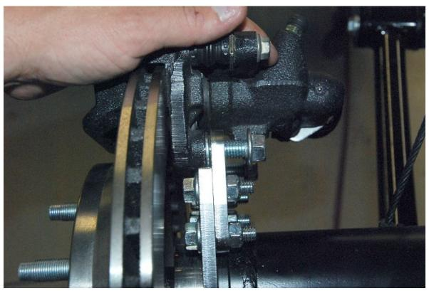
Recheck the clearance between the caliper bracket and rotor.
