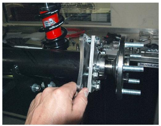
Slide the caliper mount bracket onto the four bolts.
