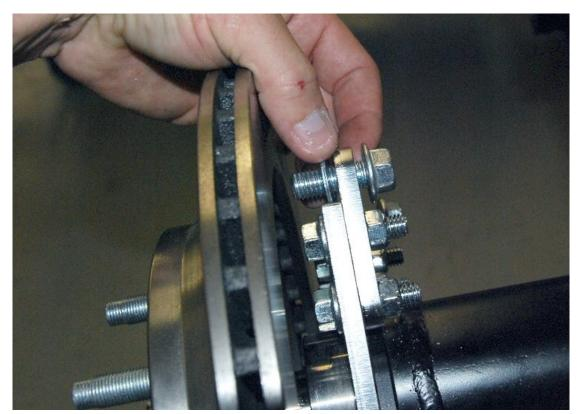
If needed remove the caliper and slide the shim onto the bolt.
