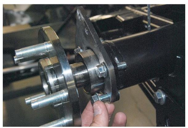
Insert the caliper axle mount bracket bolts from the outside in.
