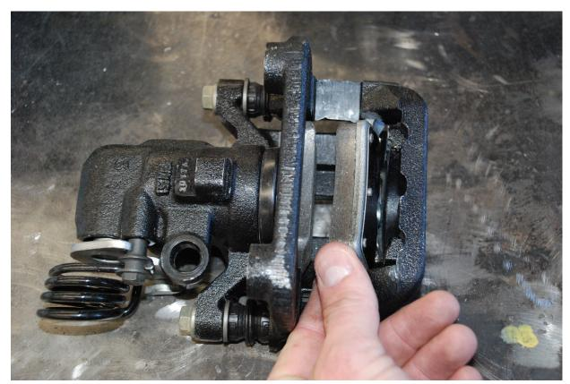
Put the brake pads in the caliper by pushing down on the pad to compress the wire springs on the top of the pad, and then slide them into the slots in the caliper bracket.
