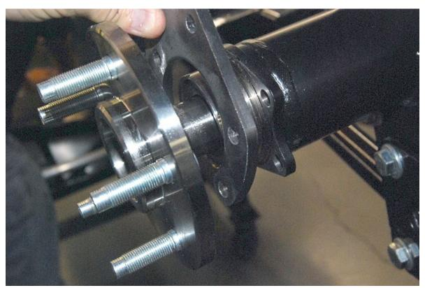
Place the caliper "C" shaped caliper axle mount bracket over the Axle so that the open part of the bracket is facing down.
