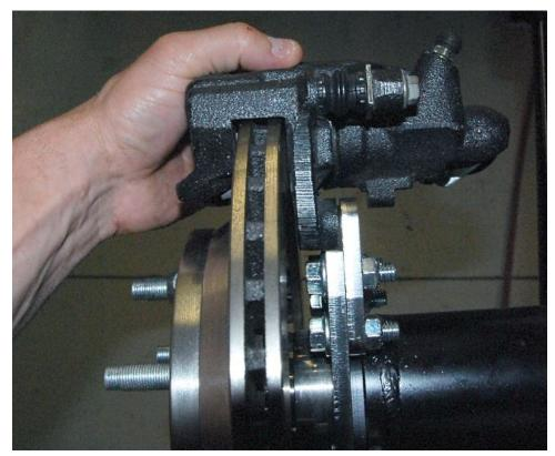
When installing the caliper make sure that the brake fluid bleed screw is on the top side of the caliper. Do not worry about the LH/RH markings on the calipers.
