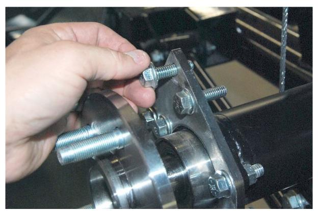
Insert the caliper mount bracket bolts from the outside in through the four remaining bracket holes.
