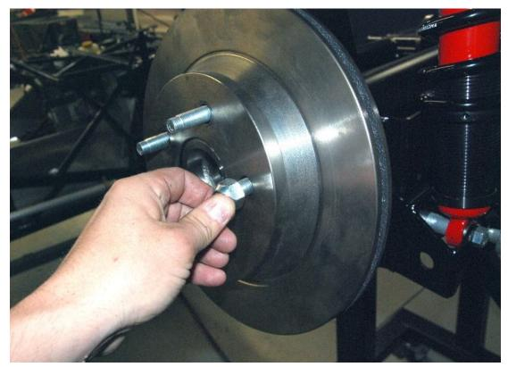
Next install the brake rotor using one lug nut to hold it in place. Make sure to clean the surface of the rotor with brake parts cleaner before installing the caliper.
