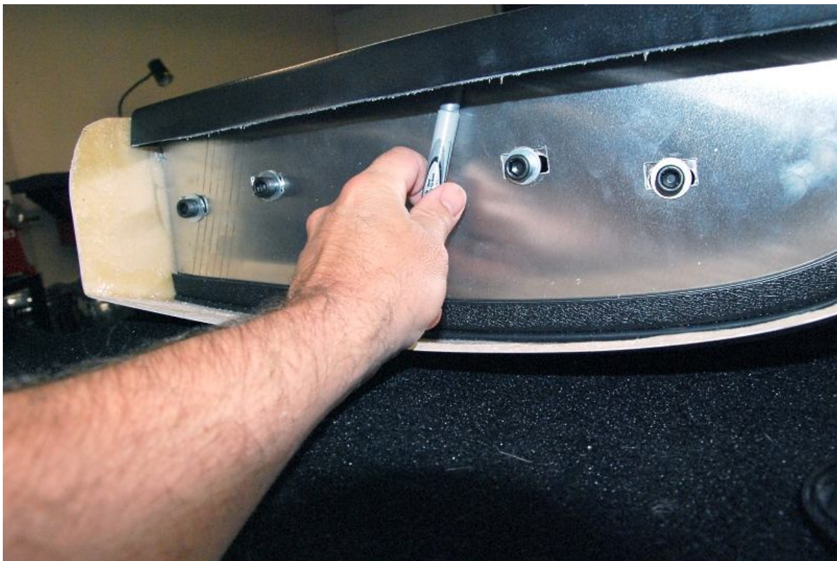
Trim front of door liner to the front aluminum.
