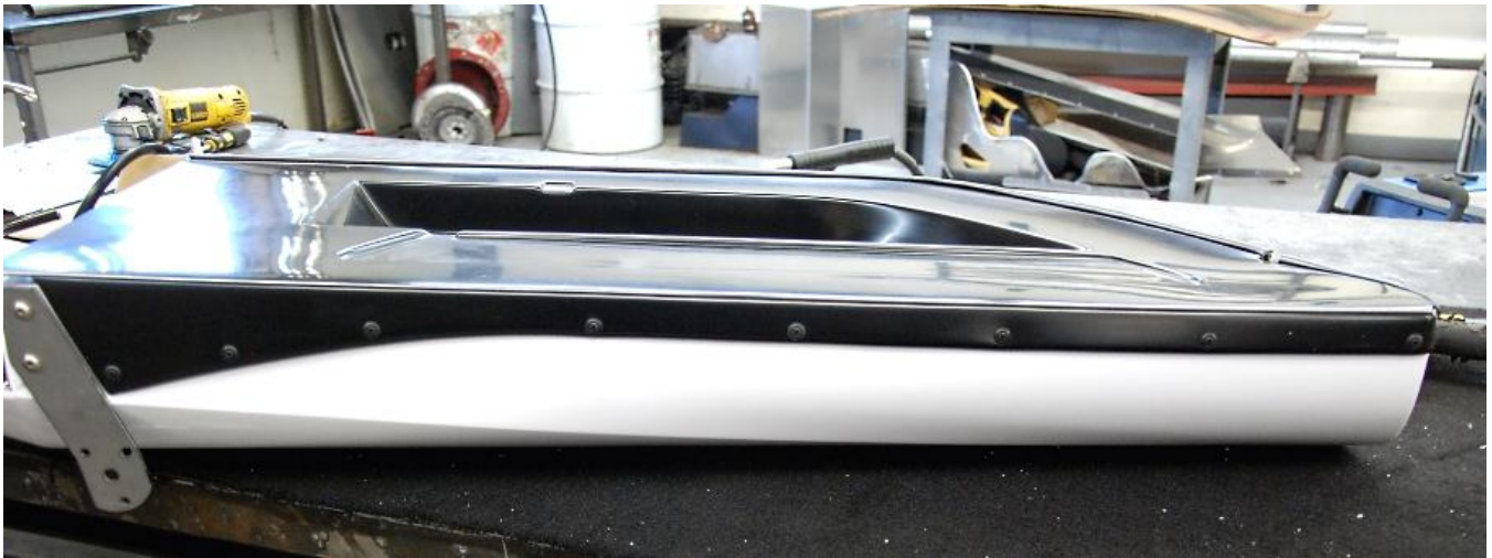
Install oval head screws and countersunk washers on top flange.
