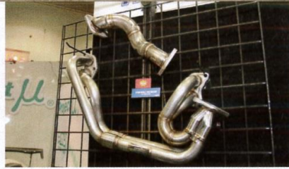
Mackin does more than just high-end wheels. They also import the MXP line of exhaust products, including this equal-length header setup for the Scion FR-S and Subaru BRZ.
