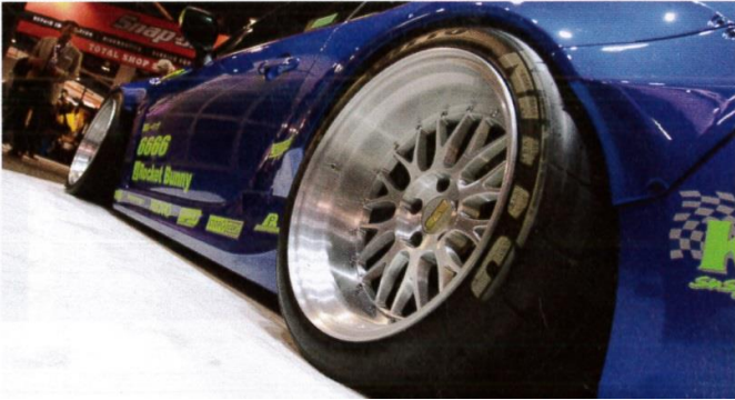
The latest evolution of the popular Volk TE37 forged wheel is the TE37 RT—those last two letters stand for Rigid Tune. Mackin Industries, importer for the line, says that updated manufacturing methods produce an inner rim that's 4- to 6-percent stronger. Look for 17- and 18-inch sizes for Porsches as well as popular Japanese cars.
