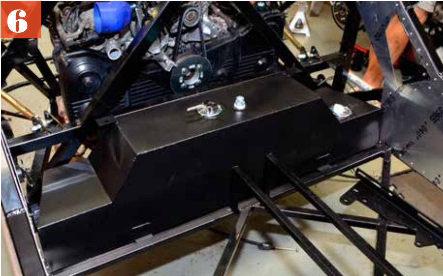
6 The last step was plumbing the fuel tank. Factory Five provides everything needed to transfer the Subaru sending unit and fuel pump to the supplied tank.
